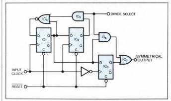
Fig 1—This circuit produces selectable, symmetrical divide-by-2 and divide-by-3 outputs.
