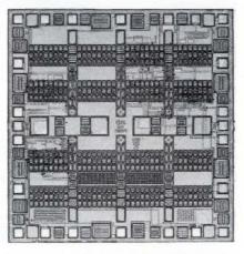
This analog ASIC array uses dielectric isolation to offer both npn and pnp transistors with cutoff frequencies of greater than 600 MHz. Besides including more than 400 transistors of varying sizes, the Sipex SP-1104 gives you programmable capacitors and thin-film resistors, zener diodes, and pinch resistors, so you can create a variety of designs without using external components.
