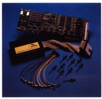
Putting a 40-channel logic analyzer on a single PC bus card is no small feat, as BitWise Designs' LAC shows. You can add RAM to capture 64k-word samples and add cards to achieve as many as 320 channels.
