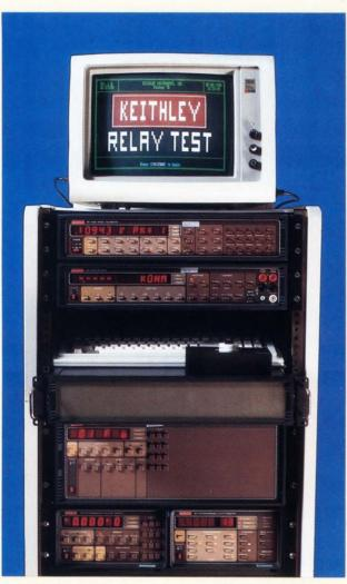
Each Keithley switching system is backed by a quality assurance program dedicated to ensuring reliable system performance. One element of the Q.A. program is the Package 70 Relay Test System shown above which is available as a complete system.
