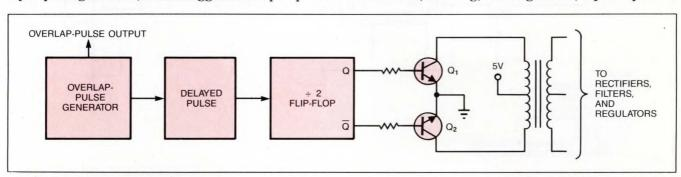
Fig 2—By sending an overlap pulse to indicate an impending noise pulse, this circuit allows the system being powered to stop any critical operations, avoiding converter noise-related problems.
