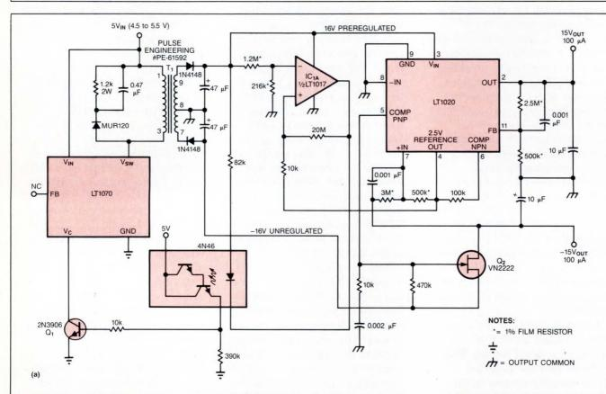
Fig 6—To satisfy the needs of many low-power systems, this converter design (a) supplies  $\pm 15V$  outputs at 100 mA while consuming only 10 mA of quiescent current. As trace D of the scope photo (b) illustrates, the converter has a 40-kHz switching frequency. Compared to conventional designs, this converter's efficiency (c) is far superior at light loads.
