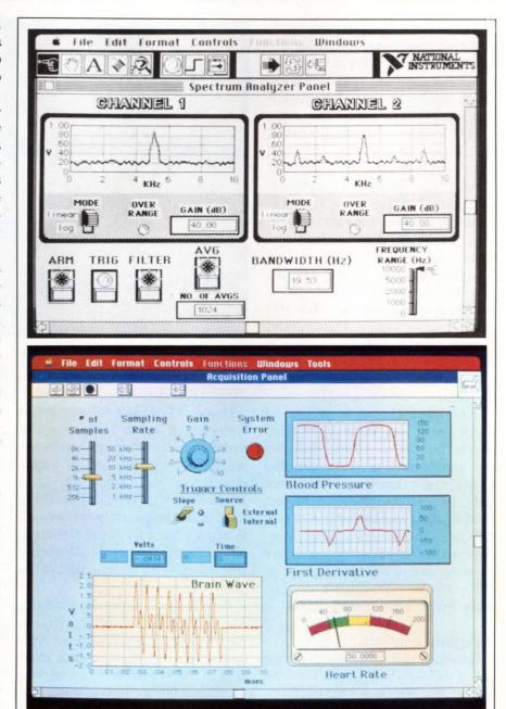
A comparison of the black and white screen of Labview Version 1.0 with the color screen of version 2.0 highlights the enhancements of the later version. Version 2.0 also offers compiled run times that are 10 times faster than previous versions could muster.
