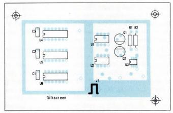
Fig 3—You should be able to create a split ground plane that isolates the analog and digital grounds and provides maximum grounding capabilities.
