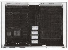
The VSC020 CPU card provides a bridge between the VME and STE Buses. By implementing industrial I/O on the STE Bus, you can dramatically reduce I/O costs.
