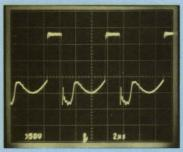
See how the fast rise and fall time of FETs contribute to the 79% efficiency of this 175 Watt model.
