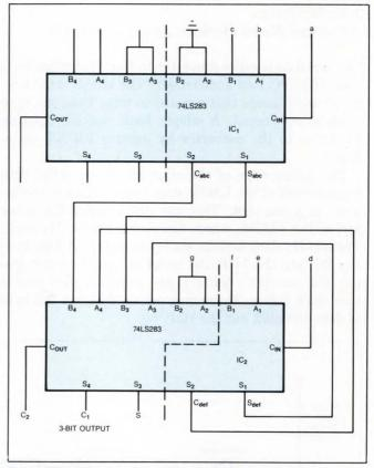
Fig 1—Cascading two full adders, each one configured as a carry-save adder, produces a 7-bit carry-save adder that's faster than its monolithic TTL counterpart.
