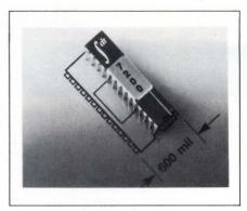
from the first read location. You can cascade the FIFO in depth and width by means of two connections. Maximum supply current is 80 mA for commercial versions and 100 mA for military versions. The IC comes in a 32-pin PLCC, a 32-pin CLCC, or a 28-pin 300-mil DIP. Prices start at \$50.90 (100).
