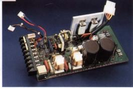
Bottom PC board with FET switches and input EMI filters.
