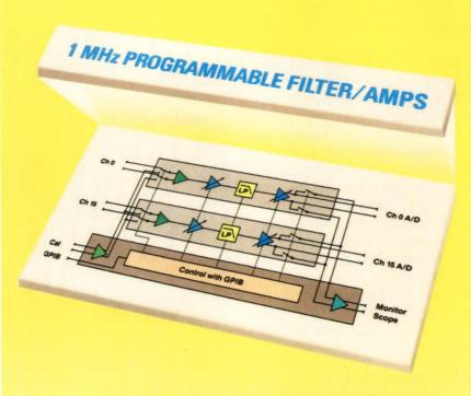
Up to 16 channels, 100 Hz to 1 MHz. HP, LP, TD. 80 dB/octave. 1° phase match. Pre and post gain. Differential input. Calibration input. Output monitor. All in 7" mainframe.
