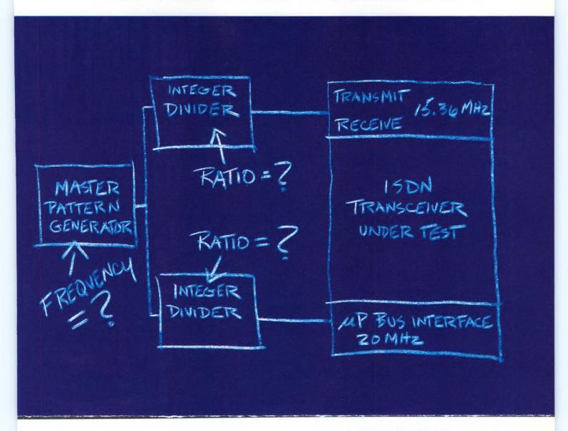
**This ISDN transceiver** requires synchronized transmit/receive data at 15.36 MHz *and* a bus interface pattern at 20 MHz. Given the tester's single master clock, what frequency do you program? What integer ratios do the dividers need?
