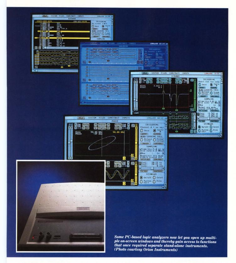
The PC's open architecture and the mix-and-match versatility it engenders provide a partial insight into the reasoning behind the development of PC-based logic analyzers—and other PC-based instruments. First of all, every logic analyzer includes a microprocessor and memory; every logic analyzer requires some sort of keyboard or panel controls; and every logic analyzer needs a display with alphanumeric and graphic capabilities. Because these items are part of a
