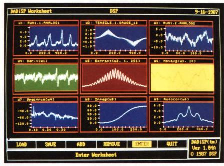
You can work with a waveform instead of just numbers if you use the Dadisp signal-analysis software from DSP Development Corp. The package also has a windowing capability.
