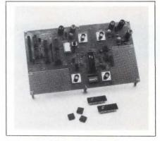
maintains bit weights and ensures no missing codes, provides a differential nonlinearity (DNL) of 0.25 LSB (typ) over the life of the device. The CMOS device, which features a sleep mode for portable operation, is packaged in a 28-pin DIP and dissipates less than 240 mW. \$27.20 (1000).
