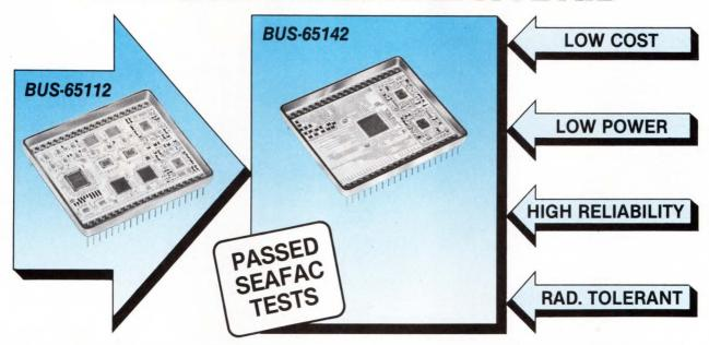
DDC is pleased to announce the new, low cost BUS-65142 MIL-STD-1553B Dual Redundant Remote Terminal Hybrid featuring a single chip CMOS/SOS monolithic RTU protocol and Bipolar low power Mark II transceivers. Incorporating small size (1.9" x 2.1") with low power and high reliability, the low cost BUS-65142 is ideal for most MIL-STD-1553 applications requiring hardware or microprocessor subsystems.
