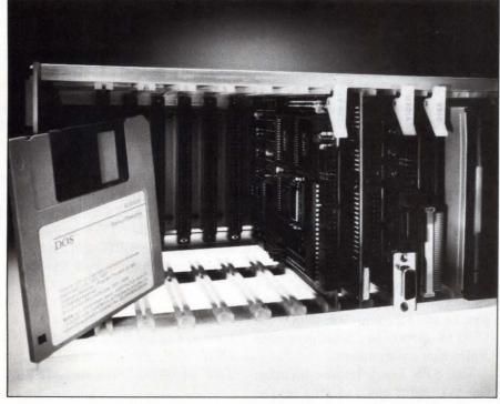
**Providing 80286-based PC/AT compatibility on STD Bus cards,** the 16-MHz STD-AT registers an 18.7 performance index relative to an IBM PC/XT computer, based on the Norton benchmark speed test.
