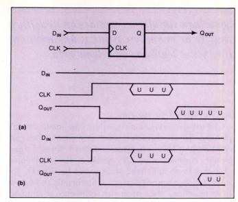
Fig 1—Simulators have different ways of propagating an undefined state. On simulator A, an unknown clock state causes the flip-flop's output to go undefined after a CLK-to-Q<sub>OUT</sub> propagation delay. The same input condition on simulator B causes the flip-flop's output to become unknown only after the CLK signal, which has become undefined, has a potential rising edge.
