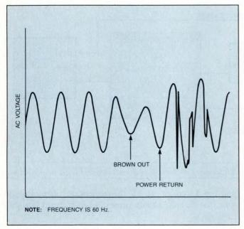
Fig 2—Fault-tolerant systems need to wait for the power line to settle before resuming mains power to protect themselves from surges that often occur at the end of many power-line disturbances.
