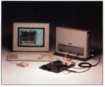
This briefcase-size unit may provide a glimpse of PC-based logic analyzers' future. Orion's Omnilab 9420A contains, besides the analyzer, a scope, an RLC meter, a pattern generator, and an arbitrary-waveform generator.
