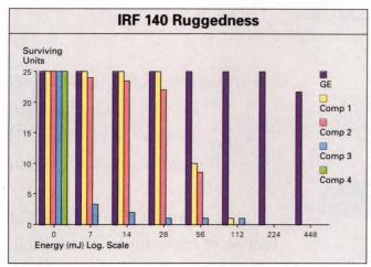
In this test conducted by Associated Testing Laboratories, Inc., the ruggedness of 25 GE IRF-series MOSFETs was compared with 25 devices from each of four competitors. As you can see, the GE parts significantly outperformed the others.
