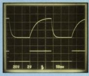
No delay at turn-on, no holding at turn-off. This remote control (RC) feature allows the output to be cycled on and off with TTL logic signals without any input current surges.
