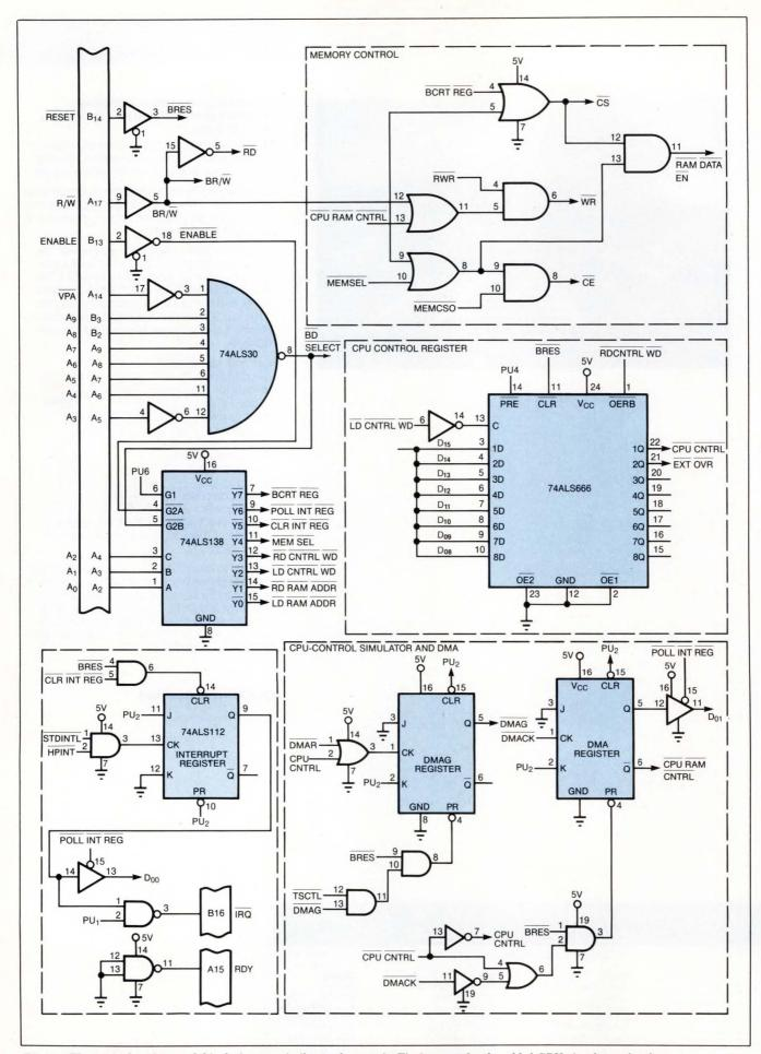
Fig 5a—The control registers of this design are similar to the ones in Fig 2 except for the added CPU simulator circuitry.
