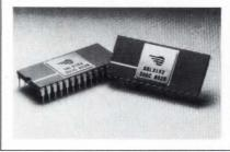
CISC and RISC systems. The ICs have TTL-compatible inputs and outputs and are cascadable in memory depth and word width. The SSL2152 has a totem-pole output; the SSL2154 has an open-drain output. Available packages include DIPs and PLCCs. Prices, which depend on the speed selection and
