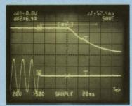
Power continues undiminished for a minimum of 20 milliseconds (30 ms typical) after loss of a-c power. Test sample measured for this photograph held up for more than 50 ms.
