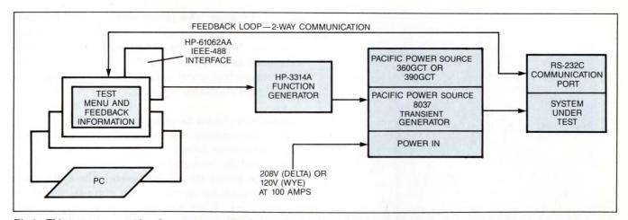
Fig 1—This test setup provides clean power, precise timing, characteristic testing, and simulates various worldwide power configurations.
