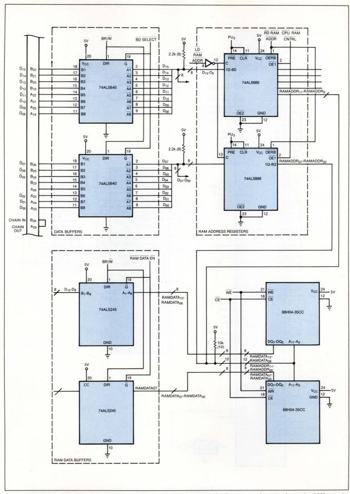
Fig 5b—Like the cirucit in Fig 2, this design uses buffers and latches to couple the local memory to the system bus under CPU control.
