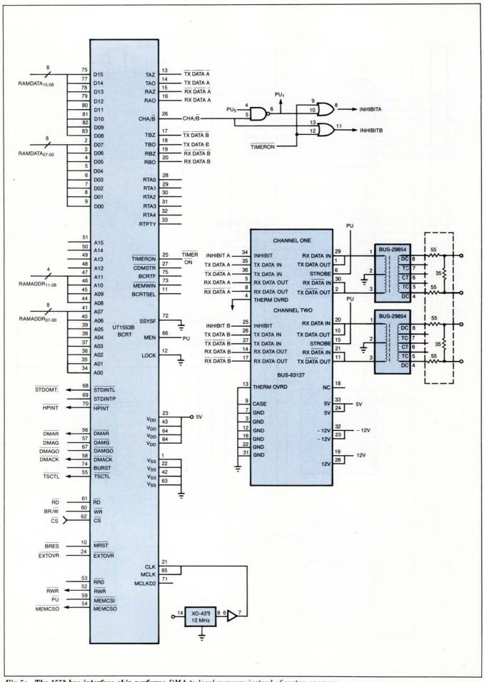
Fig 5c—The 1553-bus interface chip performs DMA to local memory instead of system memory.
