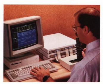
A PC allows the addition of artificial intelligence to a logic analyzer. Array Analysis' Expertest 1000 "learns" how to diagnose faults in boards.
