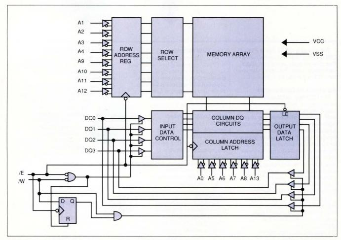
Fig 1—Integral address and data latches on a pair of SRAMs ease timing problems in high-speed, pipelined applications.
