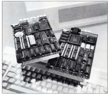
ICs created for clone mother boards and a standard BIOS ROM allow this 2-card computer for the STD Bus to use any software developed for the IBM PC.
