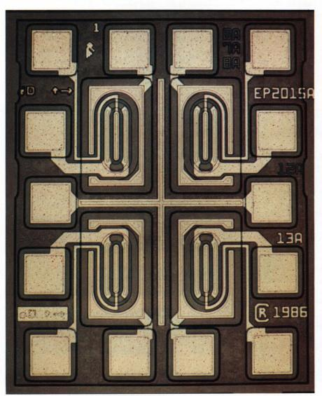
You can see the isolation barrier as dark rings around the transistors in this quad transistor array from Elantec. The glass forms a cup underneath the transistor, separating it from the substrate.
