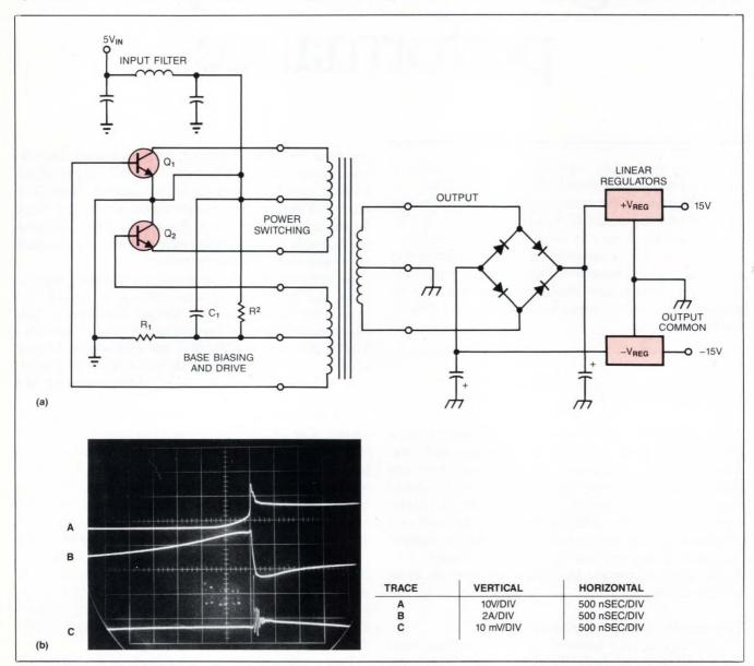
Fig 1—Although its efficiency and short-circuit characteristics are good, this converter (a) suffers from poor noise performance. The waveforms (b) show that a current spike (trace C) generated during the switching sequence is the problem source.
