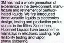
Fluorinert Liquids, used as a direct contact heat transfer medium, offer a range of physical properties that make them particularly suitable for electronic uses. They are non-polar and exhibit no solvent action. They are colorless, low in toxicity, non-flammable and offer exceptionally high dielectric strength plus thermal and chemical stability. Most important, they have almost no chemical reactivity and they evaporate without leaving a residue on parts.
