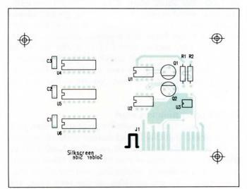
Fig 1—Grounded copper areas and guarded traces can help to eliminate noise problems in analog circuits.
