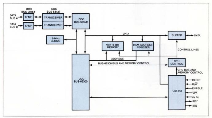
Fig 1—Adding the CPU-control circuitry to its manufacturer's application recommendations allows the system CPU to set up and test the 1553 interface.
