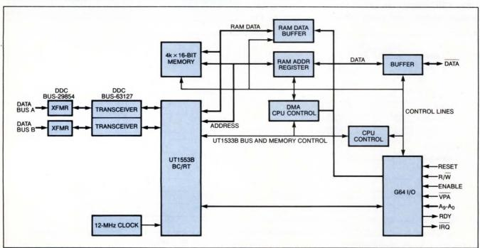
Fig 4—Like Fig 1, this block diagram has extra circuitry to transform a DMA bus controller into a DPMA bus controller that can be put under CPU control at will.
