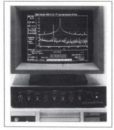
from dc to 250-kHz signals. It features software-selectable gains from 2 mV to 32V, and pretrigger and post-trigger capabilities. The 32k-byte memory/channel—expandable to 64k bytes—and the turnkey operation of the software provide the programming facilities. You access the software from C, Turbo Pascal, or Basic. The vendor provides samples of data-acquisition and data-display software with source code. \$2995.
