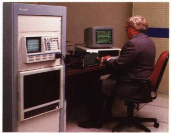
**PC-based logic analyzers** such as Gould's K450M can accommodate 40M 64-bit words of RAM.
