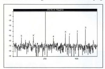
Fig 1—This FFT of an A/D converter's output has some spectra, X and X', that indicate a bad converter, buried among other, out-of-order spectra.
