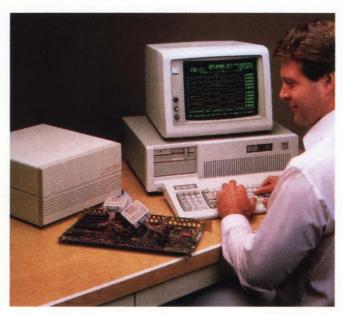
An external cabinet housing Microcase's Logic-Analysis Workstation (LAW) Series connects to the PC bus through a proprietary parallel interface.
