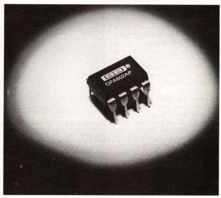
This dielectrically isolated precision op amp (the OPA-602 from Burr-Brown) features a 35V/nsec slew rate, a 6.5-MHz bandwidth, and a 2-pA bias current. The device is available in a plastic DIP for \$2.80 (100).
