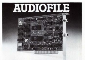
Sing it! Say it! Play it!...now in high fidelity! The new enhanced VP620E Voice Processor converts 20Hz to 7.0 kHz audio inputs into ADPCM encoded digital data for hard disk recording on your PC/XT/AT/386 or compatible. Playback flawless, authentic audio when and where you want it from background DOS commands.
