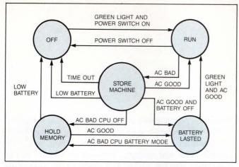
Fig 3—This state machine controls the operation of the faulttolerant computer.
