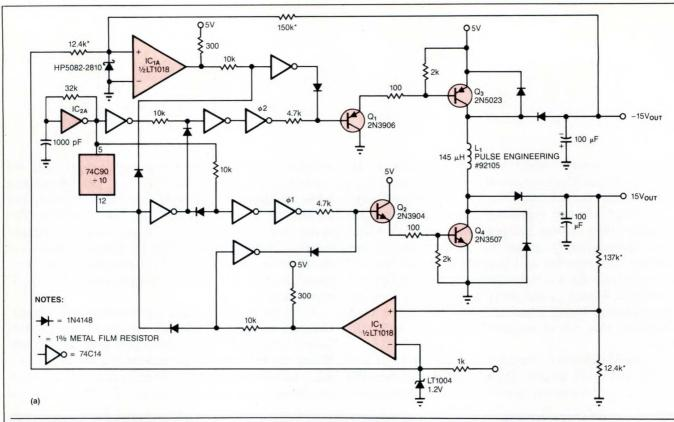
Fig 5—For circuit simplicity and economy, the drive scheme in this converter (a) uses a 2-terminal inductor in place of the usual transformer. The waveforms (b) show that although the inductor sees irregularly spaced shots of current (trace K), the multiplexed operation has no effect on the inductor's performance.
