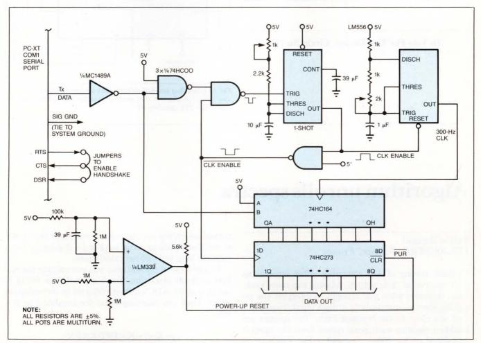
Fig 1—This serial-to-parallel converter allows your IBM PC's serial port to control low-speed (1 byte/sec) processes.
