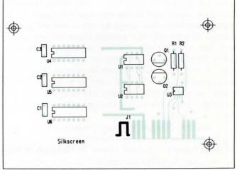
Fig 2—Analog circuits usually require a greater variety of trace widths than digital circuits. The trace from the top end of R1 was narrowed to pass between the pads for R1 and R2.
