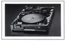
matic disk rejection, and a dual-color LED to indicate which mode (1M or 2M byte) is in operation. The drive uses CMOS circuitry and requires a 5V supply to operate. Evalution samples and documentation, \$100.
