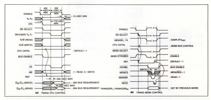
Fig 3—The I/O board's circuitry must meet MIL-STD-1553 timing specifications.
