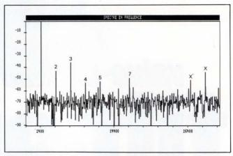
Fig 2—After performing the artifical-oversampling transformation of the A/D converter's output, a second FFT unrolls the spectrum and isolates the error components clearly.
