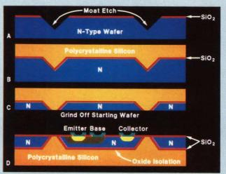
Fig A—Dielectric isolation includes four preliminary steps that other semiconductor processes don't use: You etch the silicon (a), oxidize its surface (b), grow a polysilicon layer on top of the oxide layer (c), and finally mill away the original silicon (d).
