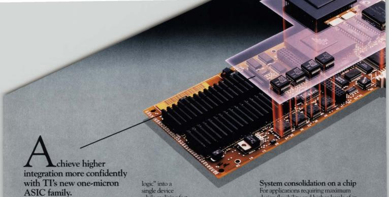
Now, you can integrate more of your systems logic using TI's new one-micron CMOS ASIC (application-specific integrated circuit) family—the TGC100 Series gate arrays and the TSC500 Series standard cells. Each offers different degrees of design flexibility and system integration. The result is significantly reduced component count which cuts board size and system cost while improving reliability and performance.
