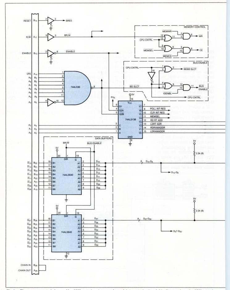
Fig 2a—The memory-control, bus-enable, CPU-control register, ready, and interrupt circuits of this diagram form the CPU-control circuitry, while these data buffers and address demultiplexers form the heart of the design's dual-port memory.
