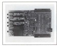
A/D converter with a 5-µsec conversion time. Two 16-bit D/A converters, which settle in 5-µsec, generate analog signals for two analog output channels. The interface for the input and output channels takes place through standard phone
