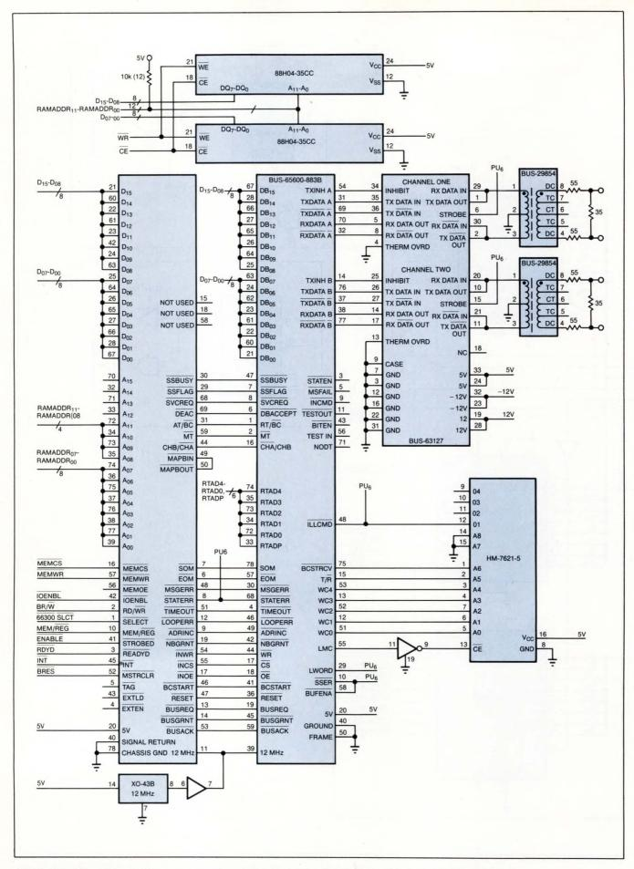
Fig 2b—The Bus-66300 and its associated chips can handle 1553-bus transactions to and from local memory.
