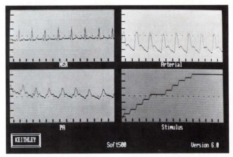
Although its output display is rather plain, Keithley Instruments' Soft500 Version 6.0 software outperforms its prettier competitors with data-acquisition speeds of 50,000 samples/sec and a 16-bit resolution for as many as 32 channels.
