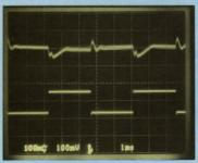
The fast switching frequency allows recovery within 1.0 msec.
