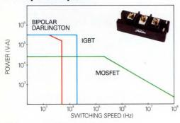
The choice is now obvious when you require both power and switching speed in your power systems. Insulated Gate Bipolar Transistors (IGBTs) offer both.
