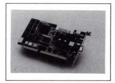
provides a resolution of  $800 \times 600$  pixels with 16 simultaneous colors and a resolution of  $640 \times 400$  pixels with 256 simultaneous colors. The card works with all VGA analog displays and multifrequency monitors. The manufacturer provides a specifically stated 1-year parts and labor warranty period. The card also features 256k bytes of dynamic RAM, 16-bit access to memory and I/O, and compatibility with the EGA, CGA, MDA, and Hercules standards. \$399.
