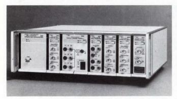
Virtual instruments such as these from Heath Zenith plug into a chassis that is an extension of the IBM PC/AT bus. The chassis also accommodates the instruments' signal connectors.
