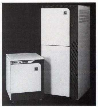
The Symmetry Series computers have a shared-memory architecture, which can have as many as thirty 32-bit processing elements. These systems, from Sequent, can deliver from 6 to 81 MIPS.
