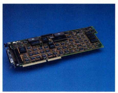
A 16k-byte read-ahead cache created in system memory by the driver software supplied with Western Digital's 7000-FASST2 board eliminates disk-access and data-transfer delays on consecutive disk reads of contiguous data.
