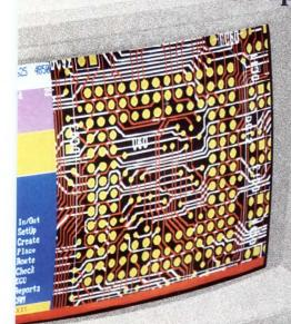
he Integrated PADS-Superstation is a new and powerful PC-Based Design Station that allows the Engineer or Circuit Designer to perform the entire design sequence from cradle-to-grave. Every decision required in the design effort, from Logic Capture to Printed Circuit Design, to 100% Connection Routing, to Checking, to generating Manufacturing Aids is made by the responsible engineer and implemented on a single, fully integrated CAE/CAD SUPERSTATION!
