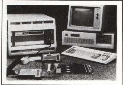
comes in two basic versions of the tester: the 635A and 635B. The 635B provides both test- and program-generation facilities, but the 635A can only execute test programs. You program the 635B,
