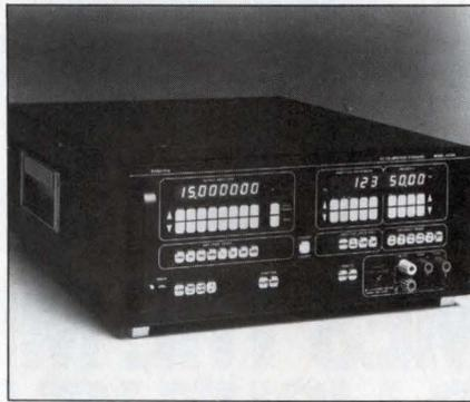
at 1 MHz or 1000V at 75 kHz. Its output-current capability is 50 mA for the 1, 10, and 100V ranges and 60 mA on the 1000V range from 10 Hz to 1 MHz. The 6400A's total
