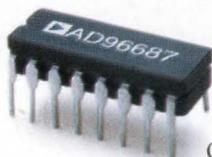
If the output from your present comparator makes it difficult to use, take a look at the incomparable AD96685 and AD96687. They're the only comparators whose propagation delays remain constant to within 50 picoseconds for any overdrive from 100mV to 1V, so you always get consistent output.
