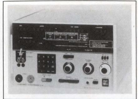
rms—that is, 1W to 35 kW, at 50, 60, and 400 Hz. It maintains its  $\pm 0.015\%$  error spec at power factors as low as 0.01. You can obtain units with an IEEE-488 interface. \$12,000 to \$14,000. Delivery, 90 to 120 days ARO.
