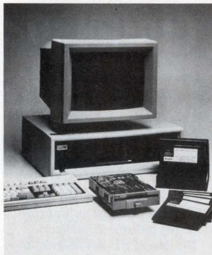
that provides a recording density of 24 kfc/i (thousand flux changes per inch). The disk drive's formatted capacity of 20M bytes is 55 times
