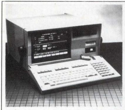
as a remote terminal on the bus, or as a monitor of all bus traffic. When used as a monitor, it provides extensive diagnostic displays; for off-line analysis, it can store bus-traffic records as long as 2.3M bytes. RS-232C, IEEE-488, and Centronics-parallel interfaces are standard, thus facilitating the unit's use in ATE systems. \$22,950 for rack-mount version; \$25,950 for portable version. Delivery, eight weeks ARO.
