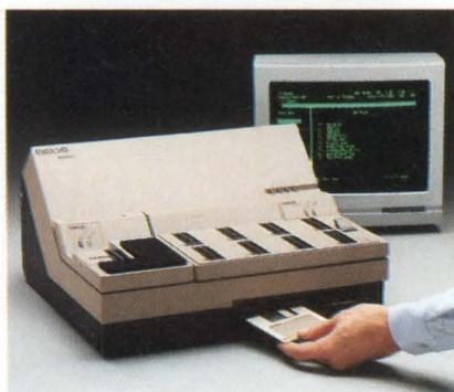
electronics stores device-specific instructions on a 3 1/2" micro diskette. To update your UniSite 40 with the latest device releases, simply load a new master diskette.
