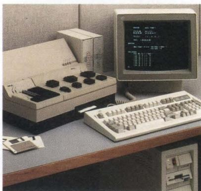
**UNIVERSAL PROGRAMMING TOOLS.** The UniSite™ 40, our most sophisticated programmer, handles all devices—memory, logic, and microcontrollers—in a single site. The modular approach to logic programming is the 29B with a LogicPak™. Or for portable convenience, the 60A programs popular logic and memory devices. Add our handler and workstation soft-
