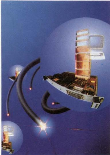
*On the cover: Intelligent Ethernet boards include a local  $\mu$ P and memory and actually perform front-end execution of the network protocol without impacting the host CPU's performance. See pg 114. (Photo courtesy Interphase Corp)*
