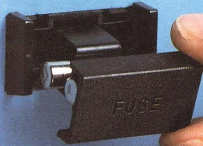
Pull out the fuseholders spring-loaded, self-extracting fuse carrier. (It's permanently attached.)
