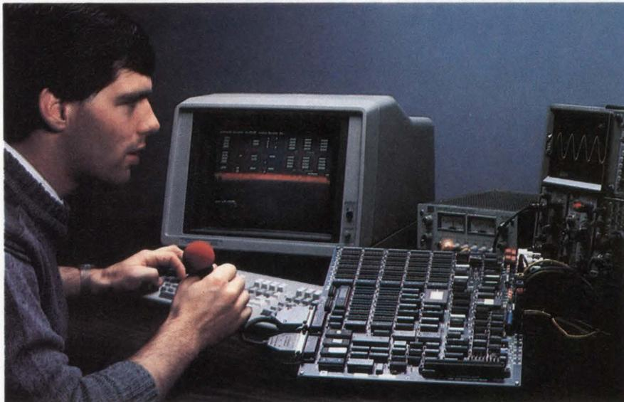
*You can shorten the development time of your next DSP-based system by using a high-level language and an evaluation system. If the evaluation isn't quick enough for your needs, you can use assembly language to speed up the time-consuming portions. (Photo courtesy Analog Devices)*
