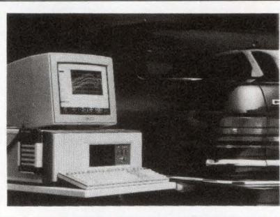
75-dB dynamic range. Two input channels are standard; the controller can accommodate eight. To safeguard the operators, the unit under test, and the test operations, the GR2530 controller performs 13 safety checks. \$27,900.
