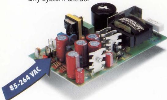
For small to medium systems, check out the NFS110 series 110 watt switchers. The +12V output will deliver up to 9 amps to start disk drives. The small 7.0" x 4.25" x 1.8" size delivers more than 2.0 watts per cubic inch.
