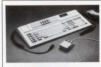
and when shifted, control-shifted, or ALT-shifted. A liquid crystal display provides operator guidance. The 123-key keyboard, equipped with electronic options for bar-code reading, the installation of a mouse, and the use of a magnetic-card reader, costs \$765. Bar-code reader, \$170; light pen, \$45; and mouse, \$45.
