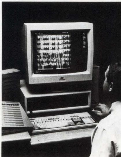
The autorouter handles 16-layer boards and offers user-redefinable strategies and 45° routes. It is re-entrant, operates in single or multiple passes, and supports three algorithms: fast probe, exhaustive search, and rip up and reroute. For each 256k bytes of RAM on the coprocessor board, the autorouter can handle a board area of approximately 56 in.<sup>2</sup> and as many as 89,600 pins. Schematic capture and layout, \$1995; autorouter, \$2995.
