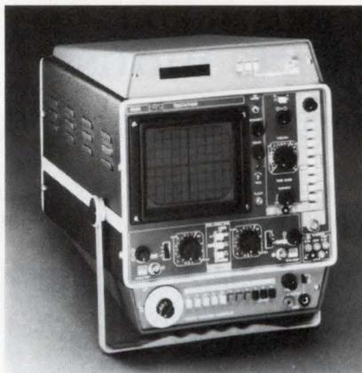
A 2-channel curve tracer lets you display and compare V/I characteristics of components. The scope has single-ended inputs with a maximum sensitivity of 2 mV/div. You
