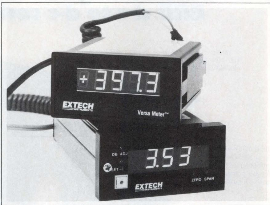
controls include pushbutton set-point display and setting, deadband range (0.1 to 10% of span), and zero and span adjustments. \$249.
