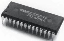
*Samsung's 256K (32K x 8) KM62256 SRAMs are available with access times of 100ns, 120ns and 150ns, all in low-power versions with standby current of only 4 $\mu$ A (typical).*
