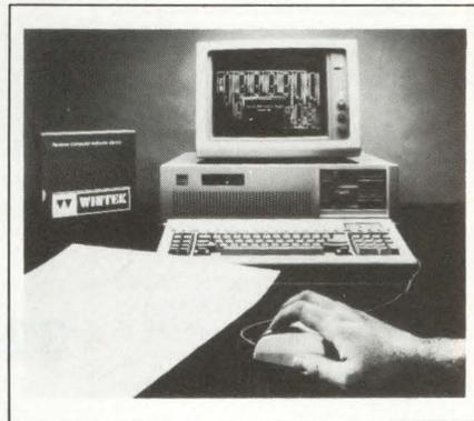
include 0.001-in. resolution, the ability to create pc-board layouts with as many as 250 layers and the ability to handle boards as large as 60x60 in. You can direct output to pen plotters, dot-matrix printers, and laser printers. The package includes utilities for the creation of net lists and a bill-of-materials, and for comparing these with your final board layout. The vendor offers a 3½-in. diskette version of the package for use on the IBM PS/2 family and some laptop machines. \$895.
