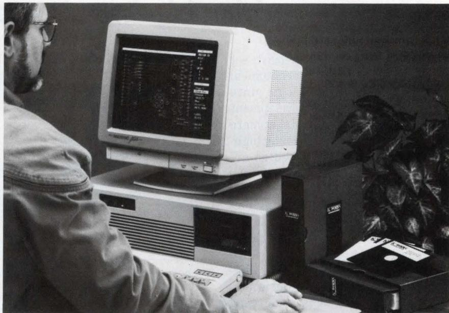
*When you use this automated ASIC-design package, you don't have to deal with the physical details of the design. IC Works can generate 50 placement alternatives from 50 different initially randomized cell placements in order to provide the best solution.*
