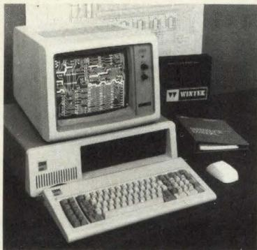
**smARTWORK<sup>®</sup> PCB Software.** In a fraction of the time hand taping requires, you can create double-sided printed-circuit boards with smARTWORK and your IBM PC. The program's features include continual design-rule checking, automatic pad shaving, a silkscreen, and text for all three layers. smARTWORK with autorouting is \$895 (without, \$495) and comes with a 30-day money-back guarantee. Credit cards accepted. Write or call
