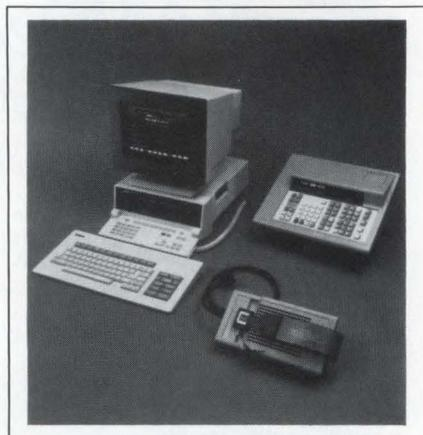
to 25 MHz without adding wait states. You can set hardware breakpoints as an optional means of terminating a Run UUT operation, and 8k bytes of overlay RAM can replace the UUT memory. Six quick-test modes are built-in, as are protection against improper voltages on the UUT pins and self tests to verify pod operation and UUT-cable continuity. \$2995. Delivery, eight weeks ARO.
