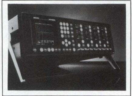
ples/sec with 10-bit resolution; the slowest provides 12-bit resolution. Each has a 64k-sample memory. You can chain or partition all of the modules' memories to achieve record sizes ranging from 512 samples to 0.75 megasamples. The instrument's plug-ins have programmable input amplifiers and can operate under software control. The instrument comes with RS-232C and IEEE-488 interfaces. It has direct outputs for X/Y plotters and matrix printers. \$13,275. Delivery, 30 to 60 days ARO.
