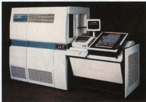
The L210i is Teradyne's first board tester for VLSI in-circuit testing, and in-circuit tester budgets.
