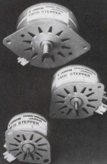
Three frame sizes — 35mm, 42mm and 55mm — in 12 or 24 volt versions. They weigh 100, 150 and 290 grams, respectively. Choose non-grain oriented or multi-pole oriented magnets.
