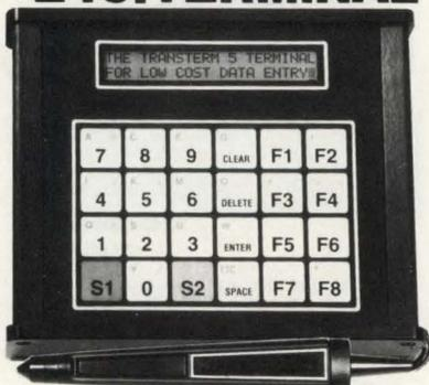
Featuring • Standard RS-232 Serial Asynchronous ASCII Communications
