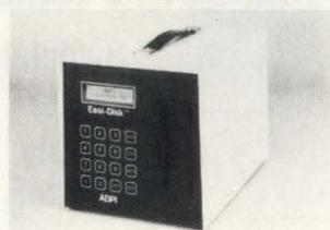
Information Transfer to/from Non IBM Compatible Systems to/from IBM & Compatibles: (Over RS-232 or 488 Interface).
