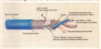
The construction of a 75 $\Omega$  control cable, such as the Belden 9463, is tailored for maximum EMI protection.
