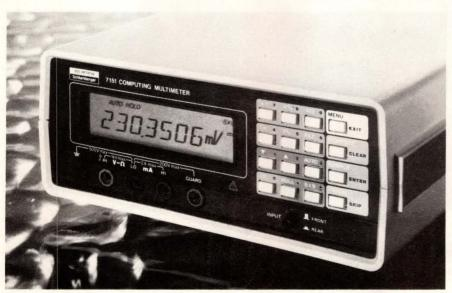
Eight firmware mathematical routines and an alphanumeric display allow the Model 7151 from Solartron to function automatically without a controller.
