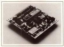
A/D CONVERTERS. These A/D converters digitize video signals at high speeds and accuracy. Model ASA-1205 operates to 12-bit resolution and at rates to 5 MHz. Model ASA-1020 operates to 10-bit accuracy and at rates to 20 MHz. The units are compatible with LS TTL and ECL, respectively. Each features single-board construction and onboard gain and offset-adjustment potentiometers. ASA-1205, \$2895; ASA-1020, \$2795. Addacon Inc, 3708 Alliance Dr, Greensboro, NC 27407. Phone (919) 852-6200.
