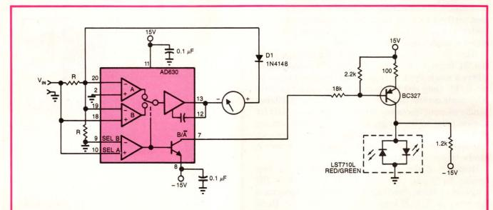
The heart of this absolute-value meter is the AD630 balanced modulator/demodulator. In its absolute-value voltage-to-current mode, meter current is a function of the input voltage and the input resistor, R.
