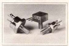
POWER MOSFETs. Switchmos fast-switching power MOSFETs meet MIL standards and feature V<sub>DS</sub>s to 400V and I<sub>D</sub>s to 8A. They employ isolated packaging in TO-61/I, TO-111/I and TO-228AA cases. The manufacturer claims the isolated packaging reduces size and weight. From \$12.85 (1000). Delivery, 6 to 8 wks ARO. Solitron Devices Inc, 1177 Blue Heron Blvd, Riviera Beach, FL 33404. Phone (305) 848-4311. TWX 510-952-7610.
