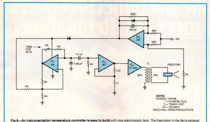
stream is the temperature-sensing element. The circuit features a long time constant, to reduce audible and annoying hunting. The LT1010 easily handles the highly reactive transformer/piezo-fan load.
