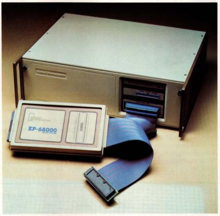
Stand-alone in-circuit emulators like this one from Applied Microsystems assist in hardware software debugging without tying up expensive software-development tools.
