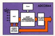
incorporates TRI-STATE® output latches that directly drive the data bus. As a result, the unit can be configured as a memory location—or as an I/O device to the microprocessor. No interface logic is needed.
