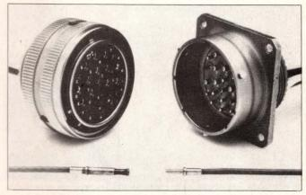
Useful in adding fiber-optic-link capability to conventional circuitry, Cannon's new fiber-optic contacts are interchangeable with size-16 pin and socket electrical contacts in the MIL-C-38999 Series and other connectors.
