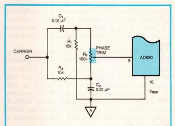
Fig 7—To trim a carrier signal so that it's in phase with the input signal, you can use this lead-lag network. With the transducer at its maximum value, adjust resistor R<sub>3</sub> to maximize the circuit's average dc output.
