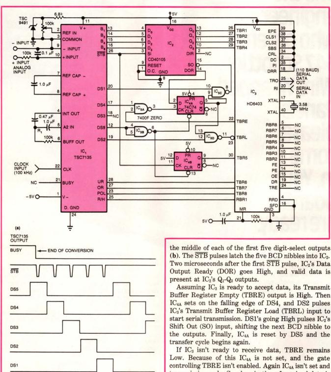
A/D converter IC1 (a) loads five BCD digits into the FIFO, IC2, in 8 msec for transmission over a slow serial data link. Transfer timing. including the STB pulse that shifts the data into the FIFO, is shown in (b). The digit-select outputs then act as a multiphase clock to load the UART, IC4, for transmission at 10 cps.
