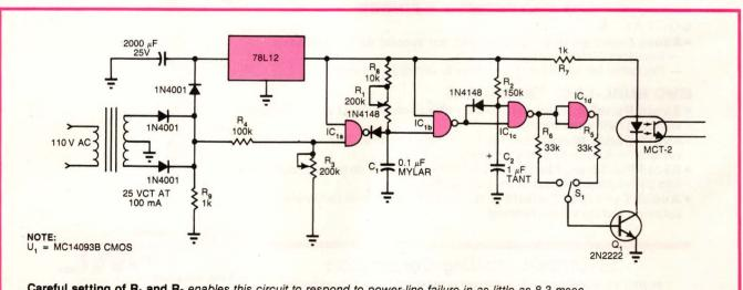
Careful setting of R<sub>1</sub> and R<sub>3</sub> enables this circuit to respond to power-line failure in as little as 8.3 msec.
