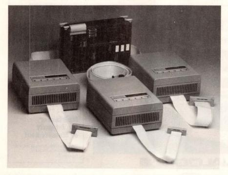
Switching from 68000 to 68010 emulation requires only a control-probe change with the 68XXX emulator from Tektronix.
