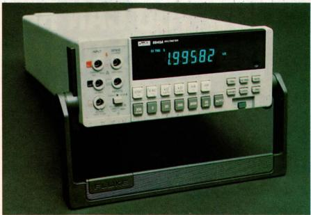
A basic dc-volts accuracy of 0.005% and the ability to take 100 4½-digit readings per second are features made possible by the recirculating-remainder A/D converter used in Fluke's Model 8840A DMM.
