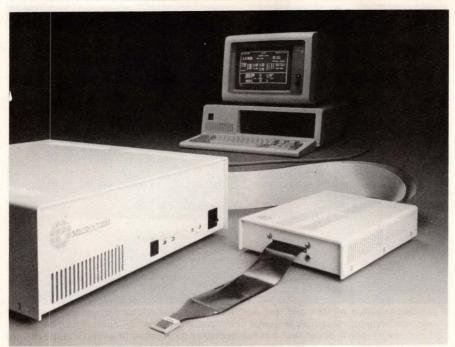
Hosted emulators can use their hosts' capabilities in graphics and fast computing to provide easy-to-use human interfaces and debug tools. Microcosm's user interface utilizes command-line and menu-driven formats to accommodate novices and advanced users.
