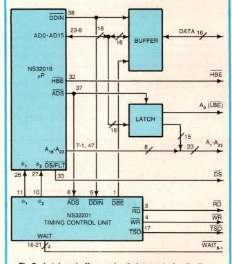
Fig 7—Latches, buffers and a timing-control unit allow a 16-bit CPU board to work with slow peripheral boards. The use of the timing unit provides as many as 15 programmed wait states in a bus cycle.
