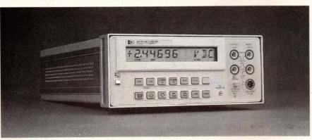
With an MTBF of 50,000 hrs, Model 3478A from Hewlett-Packard employs the multislope A/D technique and comes standard with the IEEE-488 interface.
