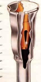
When you're loading boards before soldering, anchor sockets in thru-holes with the OMNI-TACT<sup>TM</sup> Spring Socket. Mark's exclusive bowed-spring design compresses to provide a secure retaining force over a broad range of hole diameters.
