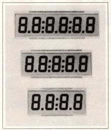
LCD. Three LCDs furnish 25.4-mm-high digits. Each  $25.4 \times 13.2$ -mm digit has seven 3.3-mm-wide segments. Minimum operating voltage is 3V, and operating range spans -10 to +60°C. SP-540 displays four digits, three decimal points and a colon and measures  $94 \times 46$  mm with a  $89 \times 33$ -mm view-
