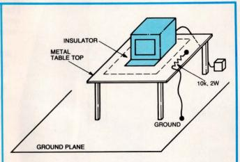
Fig 5—Test table-top units as you would floor-standing units: with and without an insulating spacer. Be sure to use a metal table top grounded through a  $10\text{-}k\Omega$  resistor.
