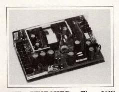
50W SWITCHER. The 50W EP6003 multioutput switching power supply has five output rails: 5V at 6A max and  $\pm 12V$ , +24V and -5V all at 1A max. Line and load regulation is better than 0.1% and
