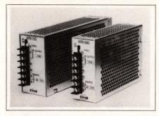
SWITCHERS. Sixty- and 100W KRV Series power supplies feature 100-kHz switching speeds instead of the usual 20 kHz. The faster switching speed results in smaller size. Models are available in 5, 12, 15 and 24V dc versions. All have overvoltage protection. 60W, \$129; 100W, \$176 (1-9). KEC Electronics, 20817 Western Ave, Torrance. CA 90501. Phone (213) 320-3902.
