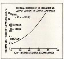
Matching the TCE of the metal core of a PC board to chip carrier ceramic is accomplished by bonding the correct ratio of copper to Invar.
