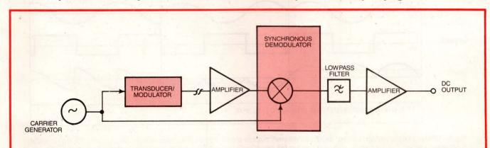
Fig 1—A typical instrumentation system can include a synchronous demodulator that removes the carrier signal from a transducer's modulated output. Using balanced modulation/demodulation removes system offset, drift and noise too.
