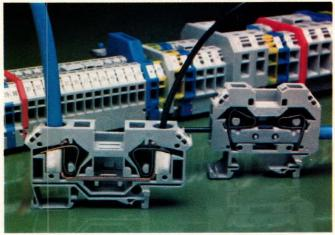
**For limited working space**, the Wago cage-clamp connectors are terminated by pushing the stripped wire end into a stainless-steel clamp assembly. They pass stringent vibration and corrosion tests.
