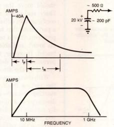
Fig B—The graphs depict a worst-case short-circuit human-ESD event. The peak current is 40A, minimum rise time is 1 nsec, and maximum fall time is 100 nsec.
