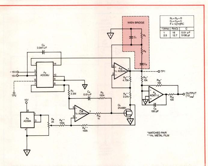
Based on a Wien bridge that supplies a sine wave with little distortion, this oscillator circuit also employs automatic gain control to stabilize amplitude.
