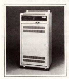
FAULT-TOLERANT MINI. The fault-tolerant Parallel 300 minicomputer runs UNIX and uses Multibus. Users need no training or tools to restore the system to operation; components can be removed and replaced quickly. The system has duplicate MC68010 virtual-memory
