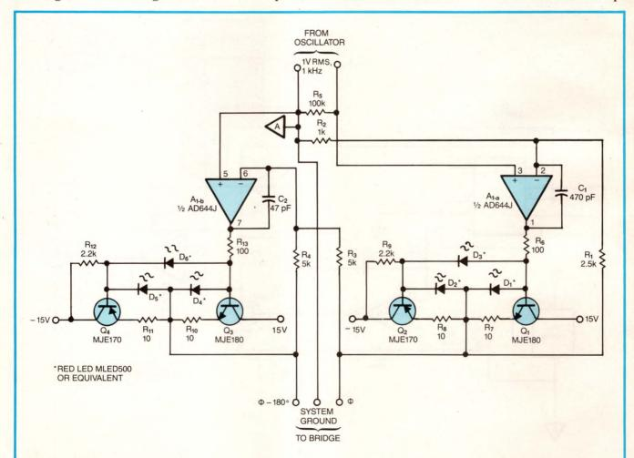
Fig 9—To drive the ac bridge in Fig 8, this driver circuit produces two 5V peak sine waves that are 180° out of phase. Using these balanced signals maximizes system sensitivity.
