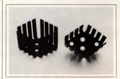
HEAT SINK. Providing efficient cooling for TO-3 and TO-66 transistors while conserving board space, Model M1622 measures 1.4×1.88 in. Fin heights of 0.5, 0.75, 1 and 1.25 in. are available. Tests indicate that while dissipating 4W of power, the device experiences a temperature rise of 22 to 40°C above ambient, depending on fin height. The standard model is made from black anodized aluminum. \$0.50 (10,000). Tran-Tec Corp, Box 1044, Columbus, NB 68601. Phone (402) 564-2748.
