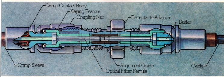
If you're looking for a quality SMA-style connector that's great in mating/unmating cycles, reliability and performance, you want the newest innovation from ITT Cannon's Micro Division, the Fiber Optic Single-Channel connector (FOSC). Its polarized shell allows positive alignment time after time, for repeatability of data transmission and minimum light loss.
