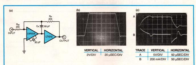
Fig 1—Inserted in a feedback loop, the LT1010 effectively isolates an operational amplifier from highly capacitive loads. The photos show the circuit's response with a 0.33-μF (b) and a 2-μF (c) load.
