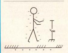
Movement can produce a charge buildup, creating a potential V<sub>ESD</sub> for an electrostatic discharge (ESD).
