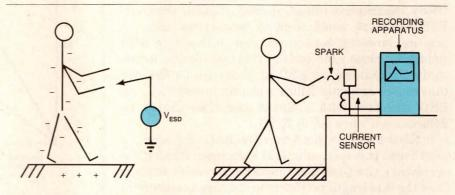
Fig A—By first measuring the open-circuit voltage on a human's finger tip and then recording the current as the charge is discharged, you can model a human-ESD event.
