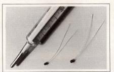
NTC THERMISTOR. The M841 negative - temperature - coefficient thermistor furnishes  $0.1^{\circ}\text{C}$  accuracy (which corresponds to a resistance tolerance of  $\pm 0.4\%$ ) over a 30 to  $50^{\circ}\text{C}$  temperature range. It comes with 20-mm silver-plated leads and operates from -40 to  $+100^{\circ}\text{C}$ . Rated resistance values are either 3 or  $5 \text{ k}\Omega$ . An epoxy-coated version, the M861, is available for operation
