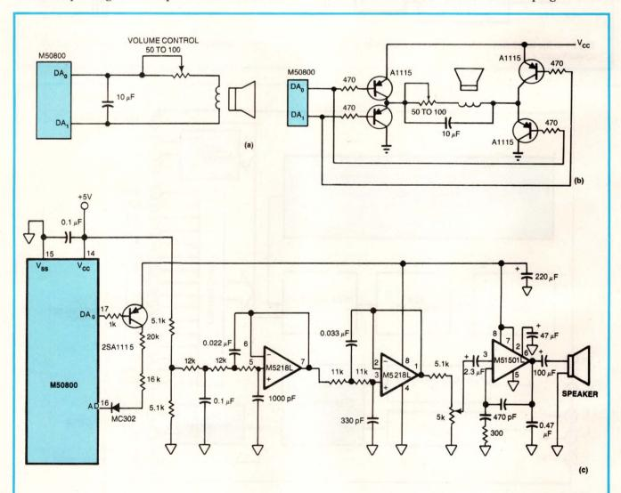
Fig 3—Although it can directly drive a speaker (a), you can also connect the M50800 to an external amplifier (b). To minimize output noise, you can use an active-filter configuration (c).
