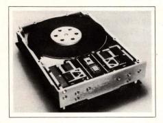
DISK DRIVES. Model 96202 5¼-in. half-height Winchester disk drive has a 103M-byte capacity, while Model 96204 has a 61.8M-byte capacity. The drives use a plated medium to achieve 960 tpi and 20,880 bytes per track. Each model is available in two formats: an entire disk drive or just the head-disk assembly. The units operate from
