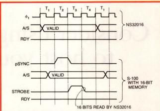
Fig 2—In 16-bit transfers with no wait states, an S-100 bus board's 16-bit  $\mu P$  asserts address and status strobes (A/S) during  $T_1$ . Assertion of pSYNC indicates a new bus cycle. The memory strobe occurs during  $T_3$ , and the  $\mu P$  reads the stored word on that strobe's falling edge.
