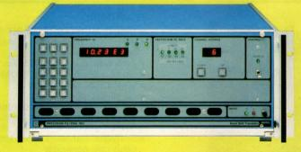
16-channels and programmable, the Precision 1776 frequency-band translator zooms in to make old equipment do more work. Ahead of an FFT
