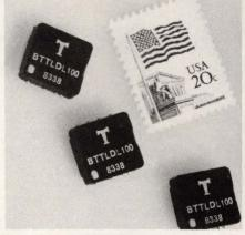
Satisfying many timing applications with minimum interfacing, these active delay lines from Technitrol suit use with TTL, Schottky TTL and low-power Schottky TTL.
