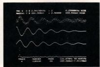
For system test applications the fully programmable Data 6000 can acquire waveforms, measure time domain waveforms with over 40 pre-programmed scalar measurements, compute and measure spectra, and transfer the resultant measurements or data points to your computer. In the above figure the Data 6000 performs summation averaging on a noisy signal, convolves the result with a user defined filter, and displays the FFT of the processed wave-form on trace four.
