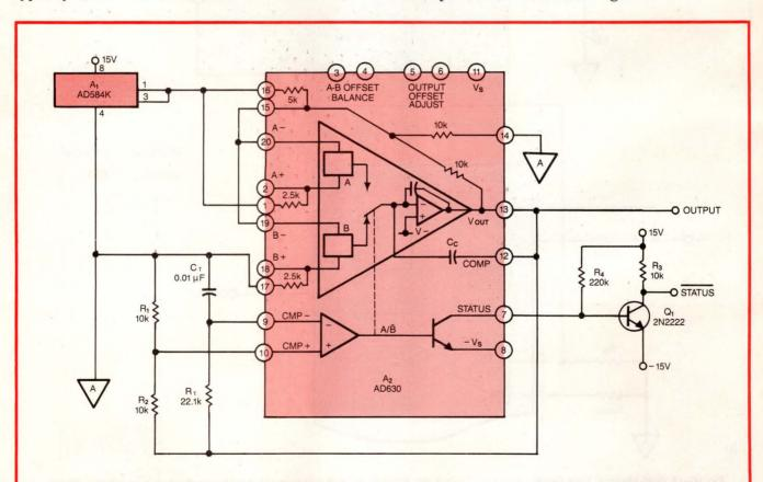
Fig 11—To produce a square wave with a precise, 10V p-p amplitude, the AD630 switches the polarity of the AD584K's precision 2.5V dc output and multiplies it by a gain of 2. The square wave's frequency is set by  $C_{T}$  and  $R_{T}$ ; in this case, it's about 2 kHz.
