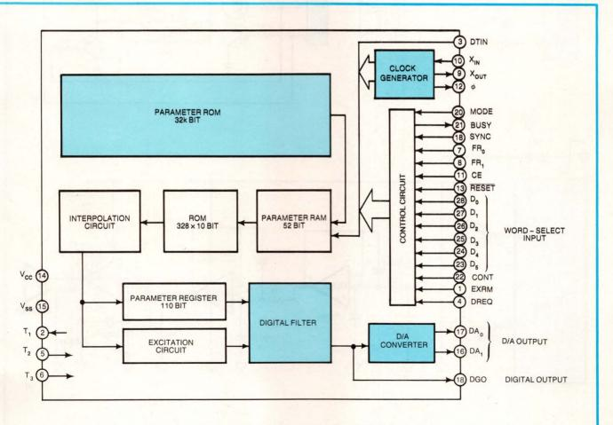
With on-board ROM as well as a digital filter, D/A converter and clock generator, the single-chip M50800 can function as a stand-alone speech-output circuit, or it can interface with external memory and a  $\mu P$ .
