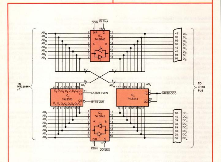
Fig 1—Four ICs provide the circuitry required to interface a 16-bit μP such as the NS32016 with the S-100 (IEEE-696) bus.
