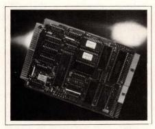
SINGLE - BOARD COMPUTER. STD Bus-compatible, Z80A-based Model MP6102 provides byte-wide memory in EPROM with 8k-bytes capacity. It provides three channels of user-definable counter/timer functions using one channel as a software-programmable time base
