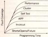
Take test patterns from a variety of sources to optimize fault coverage in the shortest programming time possible.
