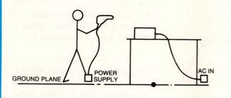
Fig 3—A ground plane on the test site's floor supplies a local earth ground. The plane has a free-space capacitance of 30 pF/ft². If large enough, a direct discharge to the ground plane will raise its potential only slightly.
