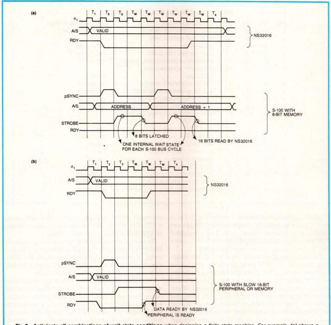
Fig 8—Anticipate all combinations of wait-state conditions when designing a finite-state machine. For example, (a) shows a byte-serialized, 16-bit transfer with one external wait per byte, and (b) shows a 16-bit transfer with S-100 wait states.
