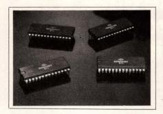
built-in delay timers and external delay timers, an on-chip crystal-controlled oscillator, a TTL-compatible interface, and low power dissipation; they operate at rates to 300 baud, full duplex. The -6927 and -6947 operate at rates to 1200 baud, half duplex. The company claims a bit-error rate of  $10^{-6}$  at a 7-dB S/N
