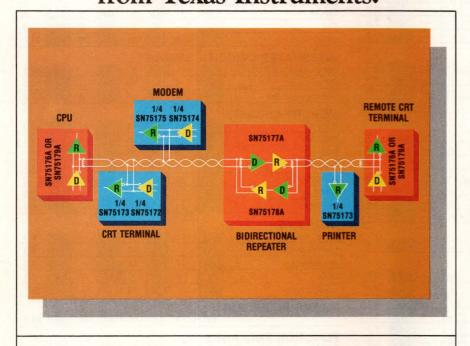
**Hooking 32 driver-receiver pairs** on a single bus to achieve party-line communication is possible with Tl's full family of line circuits.
