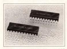
UPGRADED RAMs. Faster "A" versions replace the MCM93422 and -93L422 1024-bit (organized as 256×4 bit) RAMs. Dubbed the MCM93422A and MCM93L422A, these RAMs have maximum address access times of 35 and 45 nsec compared with their predecessors'
