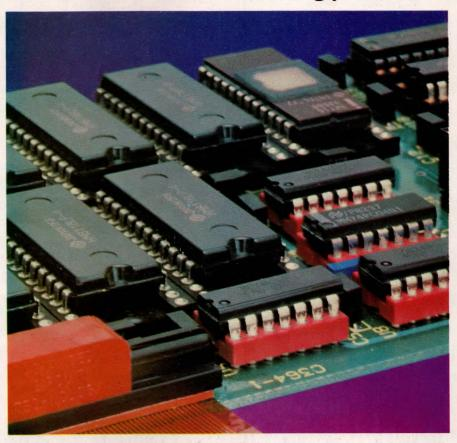
Offering twice the contact density of conventional insulation-displacement connectors, Advanced Circuit Technology's SNAP connectors mate flat flexible circuitry to pc boards.
