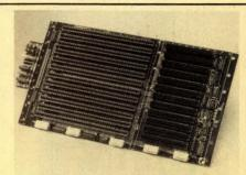
Combination backplane/monitor/power harness provides quality design. Grounded, terminated, 24-bit addressing, bussed p2. Unique 4-layer backplane is integrated unit with 32 system-monitor LEDs, ten voltage monitor LEDs providing system diagnostics, visual warning of improper performance. Signals, CPU readable, display bus master, pending interrupts, control strobes, incorrect voltage/ temperature, more. **PACIFIC MICROCOM-PUTERS, INC.**, 160 Chesterfield Drive, Car-diff, CA 92007, 619/436-8649.
