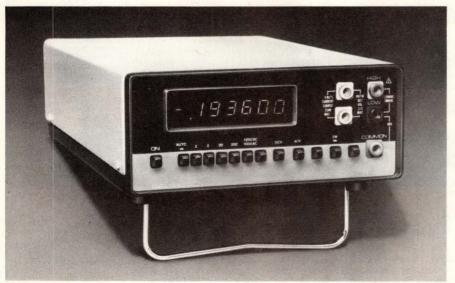
Optional modular plug-ins providing dc/dc and ac/dc ratios and ac conversion allow users of Data Precision's Model 3600 to start with a \$795 base price and add capabilities as required.
