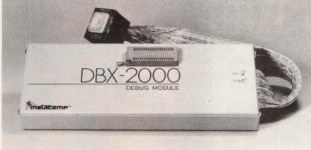
**Emulating an 80186 with an 8086** is possible with Metacomp's DBX-2000 emulator and debug module. The module includes PALs for emulating 80186 chip-select logic; memory-chip and peripheral-I/O-chip select/decode logic for independent wait-state generation; an i8254 programmable interval timer; an i8259A programmable interrupt controller; and space for 8k bytes of emulation memory.
