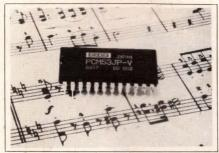
monotonicity. THD is 0.002% typ at full-scale (16 bits) input and 0.02% typ THD at -20-dB input. Differential-linearity error is typically 0.001% FS reading at the bipolar zero point. Dynamic range is 96 dB, and typical settling time is 3  $\mu$ sec. Housed in a 24-pin plastic package, the IC is spec, performance and pin
