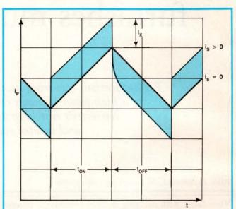
Fig 2—Secondary loading results in a step change in primary-inductor current  $i_P$  when Fig 1's  $Q_1$  switches. Here,  $i_P$  is shown for secondary current  $i_S$  both equal to zero and greater than zero; the deviation in  $i_P$  when  $i_S$  is greater than zero is labeled  $I_X$ .
