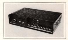
with airflow and 250W under normal convection cooling. It has 5V dc at 40A, 24V dc at 6A, 5V dc to 15V dc at 3A and two 12 to 15V dc at 6A outputs. Housed in a 2.56 × 7.5 × 11.81 -in. package, all outputs are regulated, switching, user-adjustable and floating. The supply meets UL 478, CSA 22.2, VDE 0804 and 0806, IEC 380 with SELV circuitry and has British Telecom approval to GT2 and GT26. \$410. Qualidyne Systems Inc, 2256 Main St, Chula Vista, CA 92011. Phone (619) 429-7440.
