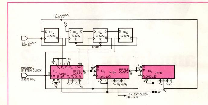
This digital-PLL circuitry provides a clock, in synchronization with an external clock, and a frequency 16 times that of the external clock. Synchronization of the counter—three 74169 ICs—is accomplished by holding or advancing the state of IC<sub>3</sub>.
