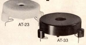
AT-23 and AT-33 piezo ceramic audio transducers... more sound proof of Projects Unlimited quality. These new transducers provide you with frequencies up to 3.3 KHz, low current drain, wave solderability, P.C. board mounting, plus high sound output... up to 94 dBA at 1 meter. ABS plastic cases. No electronics. Operating temperature from — 20°C to 70°C. Write for complete specs and full-line catalog: Projects Unlimited, Inc., 3680 Wyse Road, Dayton, Ohio 45414. Phone: (513) 890-1918.
