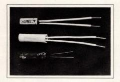
(33×5×7 mm) and resin case (21×3.6×7.6 mm). Models are available with trip temperatures ranging from 70 to 160°C for glass-cased units and 80 to 140°C for metal- and resin-cased models. Trip temperatures vary in 5°C increments. The switches open an electrical circuit as soon as their environment reaches
