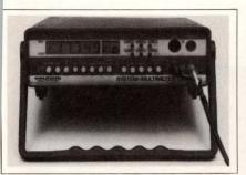
SYSTEMS DMM. The DM50 benchtop multimeter has a count of +54.000 digits. Basic dc-voltage accuracy is 0.02%, and the unit can measure true rms ac voltage (0.1% accuracy), resistance and current. It comes with built-in computing power for such tasks as calculating and displaying decibels, limit-testing results and percent deviation. 2450 DM. Optional IEEE-488 interface, 500 DM. Grundig Electronic AG, Wuerzburger Str 150, Fuerth/ Bay, West Germany. Phone (0911) 73301. TLX 623435.
