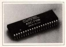
12-BIT A/D CONVERTER. The ADC7109 integrating A/D converter interfaces with 8- and 16-bit  $\mu$ Ps. It includes a buffer amplifier, integrator, comparator, 12-bit binary counter and 3-state outputs for data-bus interfacing. In the byteorganized parallel mode, the converter interfaces with such  $\mu$ Ps as the 6800, 8080 and 8048. Fourteen data outputs provide 12 magnitude
