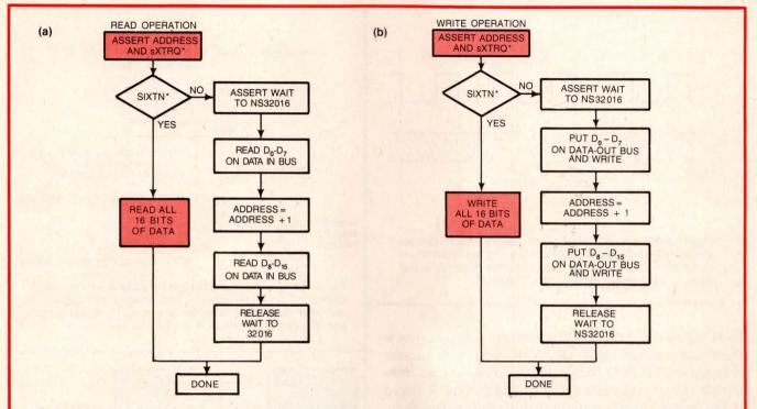
Fig 3—Read (a) and write (b) operations for a 16-bit processor on the S-100 bus begin with the presentation of an address and assertion of the sXTRQ\* line. A 16-bit-wide memory board would respond by asserting SIXTN\*, allowing a single 16-bit transfer. An 8-bit memory board wouldn't assert SIXTN\*, signaling its requirement for two single-byte data transfers.
