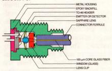
This cross section of an HP fiber optic transmitter shows HP's advanced lensing scheme for optimal coupling of light into the fiber.
