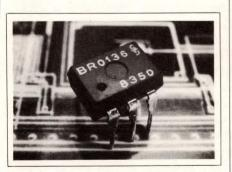
OPTO AC SWITCH. The BRT12 6-pin IC contains a light-triggered ac switch capable of linking logic to 220V mains. Input sensitivity is lower than 2 mA, and reverse volt-
