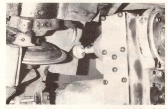
**Typical of the rough environments** now being invaded by digital motion-control equipment is this special grinding machine by Atrax Research and Development. Here, a Compumotor electronically controlled microstepping motor replaces the hydraulic drive of earlier designs.
