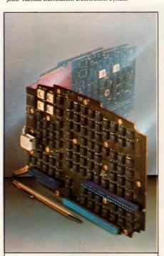
Successful application of high-density packaging was achieved in the PC boards of the F-15's new communications equipment. Tl's clad metal system solved thermal expansion mismatch. This mirror-reflection photo shows how ICs were mounted on both sides of the PC boards.
