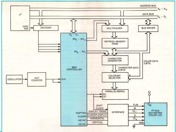
Fig 2—Similar to CRT-drive systems, FT1616 displays use the familiar refresh memory, a 6845 CRT-controller IC and a character ROM to generate characters or graphics.
