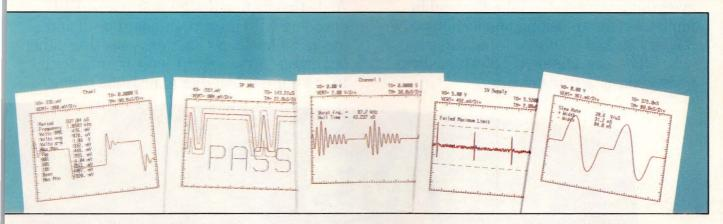
you get consistently accurate results. Comparison measurements with the HP 1980 are orders of magnitude faster than manual testing. For example, parametric tolerance tests, such as comparing peak amplitude to preset limits, can be performed within several hundred milliseconds.
