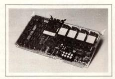
4M-BIT MEMORY CARDS. Four Multibus-compatible memory cards feature capacities of 128k, 256k, 384k and 512k bytes. Using expansion ports, you can raise memory
