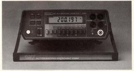
The \$595 base price for the 5½-digit Model 197 from Keithley includes 5-function measurement capabilities and a 100-measurement storage buffer.
