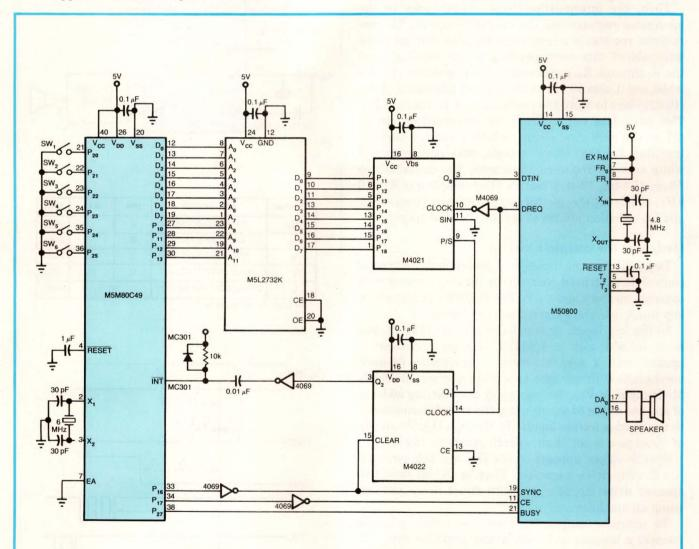
Fig 5—For applications that require more storage than the M50800's on-chip ROM provides, you can add external memory. The circuit shown here provides 20 sec of speech output. The amount of memory such a circuit can accommodate is limited only by the addressing range of the accompanying  $\mu P$ .
