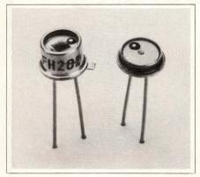
multimode stepped-index fiber with core diameters between 50 and 200  $\mu m$ . It produces 4.7-mW max radiant power; switching time is 40 to 50 nsec at 100 mA. The Si SFH202 receives these signals with a 0.55-mA/mW response. SFH407, \$6.80; SFH202, \$3.95 (10,000). Siemens Components Corp, Optoelectronics Div, 19000 Homestead Rd, Cupertino, CA 95014. Phone (201) 321-4842.
