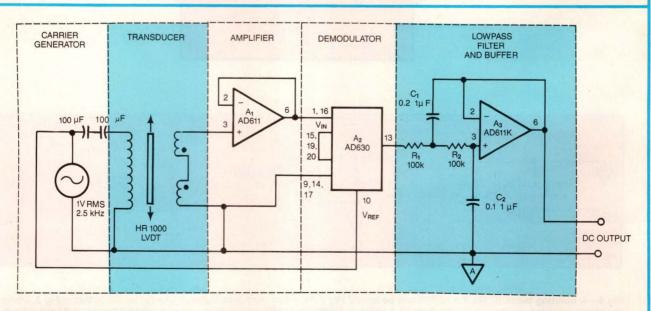
**Fig 6—A linear variable differential transformer** whose measurement signal rides on a 1V rms, 2.5-kHz carrier can work with a commutating modulation/demodulation circuit such as the one shown in **Fig 4**. The lowpass filter at right, with a 10-Hz corner frequency, removes any high-frequency noise.
