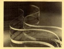
Miniature, axial lead ceramic capacitors for automatic insertion into pc boards. Replace monolithics and ceramic discs in some applications. More reliable than ceramic discs. Values from .47 pF to 100,000 pF. Voltages of 16, 25 and 50 WVdc. Temperature coefficients from NPO (COG) to Y5T. Measures .276" long × .110" dia., max. Packaged on tape and reel.
