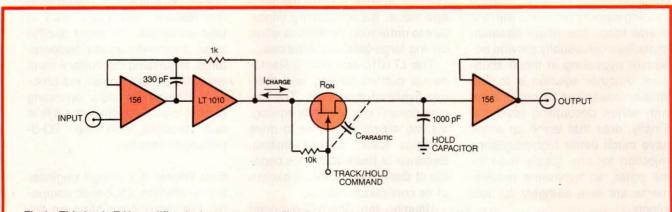
Fig 4—This basic T/H-amplifier design presents conflicts between low pedestal (hold step) and fast acquisition time. A large hold capacitor reduces the former problem but increases the latter. The circuit also needs a fast level shifter to drive the FET's gate from TTL signals.
