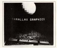
Users of the 4-bits/pixel model can choose 16 colors from a palette of 4096; the 8-bits/pixel version lets users choose 256 colors from 16M. The instruction set contains single-instruction polygon, box, circle and vector drawing commands as well as solid fill, outline, stipple, cut and paste and opaque/transparent modes. The double-buffered controllers feature dual-ported video memory, RS170 video compatibility with gen-lock, two frame buffers, zoom, smooth pan and scroll. They
