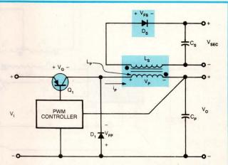
Fig 1—A secondary inductor magnetically coupled to a buck-type converter's primary circuit can derive isolated auxiliary output voltages. The secondary rectifier  $D_{\rm S}$  is oriented so that it conducts only when switch  $Q_{\rm 1}$  is Off.
