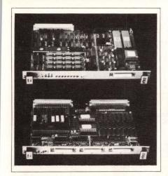
SINGLE-BOARD \( \mu C.\) Based on the 68000 µP and the VME Bus, the CPU-1B and CPU-2 are available with an 8- or 10-MHz processor unit and options of 128k or 512k bytes of local dynamic RAM. The -1B board provides three RS-232C I/O ports (110 to 38.4k baud) and one parallel, 68320-based I/O port. It features a 24-bit programmable timer, an onboard, real-time clock with battery,
