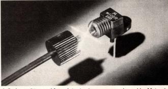
A GaAs emitter and four detector types are packaged by Motorola in a standardized plastic receptacle that has a mounting flange and the male portion of a fiber-optic connector. A plastic fiber-optic cable mates with the receptacle.
