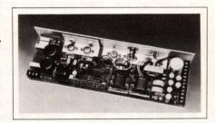
400W SWITCHERS. DP-400 Series open-frame power supplies deliver 400W at 80% efficiency with as many as five regulated voltage/current output combinations. Five supplies have a fixed 5V dc at 50A output with four other V/I combinations, and the sixth has custom-configured outputs. Conforming to VDE 0806 and IEC 380, the power supplies provide separate primary
