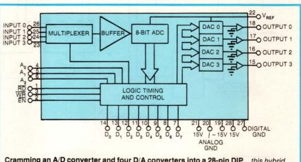
Cramming an A/D converter and four D/A converters into a 28-pin DIP, this hybrid accepts four analog-input channels and yields four D/A-converter-controlled analogoutput voltages.
