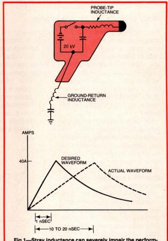
Fig 1—Stray inductance can severely impair the performance of an ESD simulator, slowing rise time as a consequence. This inductance results from ground-return length or the length of the probe.
