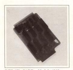
RELAY CARD. Model 4303 provides eight to 16 solid-state relay outputs for the STD Bus system. With strappable addressing and internal data latches, it provides the STD system with power output switching capabilities and optocoupled isolation through the relay module. Standard units have eight dc relays with load capacities of 4 to 60V dc and 3A max. On-board mounted suppression diodes for in-
