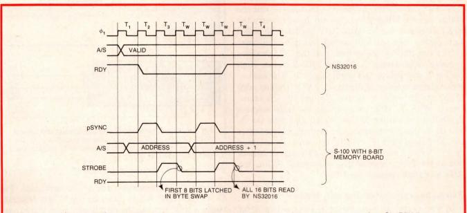
Fig 4—To perform the byte swapping necessary for reading 16-bit data in two byte-wide segments, the  $\mu$ P's RDY line goes Low to halt the  $\mu$ P. On the first falling edge of the strobe, the low byte is latched, after which the address is incremented. Finally, on the second falling edge of the strobe, the  $\mu$ P reads the 16-bit data.
