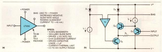
**Featuring a bias pin to optimize negative slewing**, the LT1010 offers high speed and the capability to drive highly reactive loads. The device is available in a TO-39 package or the heftier TO-3 package.
