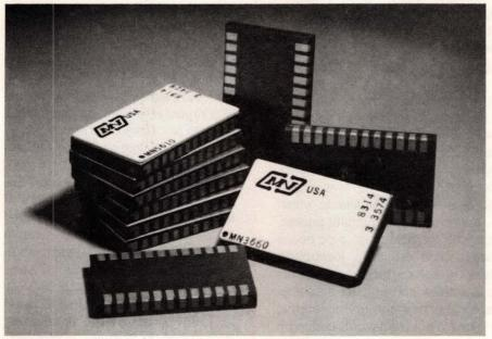
**Surface-mountable A/D and D/A converters** from Micro Networks come in leadless packages with a maximum height of 0.183 in. Outside dimensions measure 0.81×1.315 in. max, and each unit's 24 bonding pads are located on 100-mil centers.
