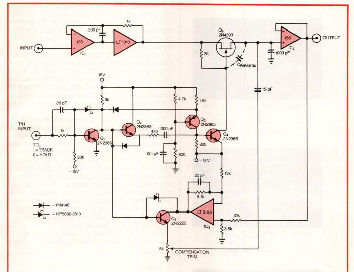
Fig 5—This fast, accurate T/H amplifier uses discrete transistor circuitry to provide both low pedestal and fast acquisition time. It also features a very fast TTL-to-FET level shifter. The scheme uses a compensation technique to reduce parasitic-induced pedestal.
