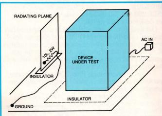
Fig 4—For floor-standing units, run tests with the device under test both in contact with the metal plane and standing on a 0.5-in.-thick plastic insulator.
