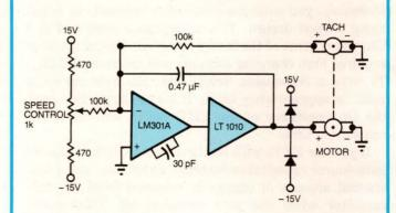
Fig 7—This simple motor-tachometer circuit takes advantage of the LT1010's ability to drive heavy reactive loads. The circuit allows speed control in both directions, thanks to the tachometer's bipolar output.
