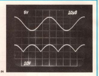
Fig 5—In an absolute-value circuit with a gain of 2, the AD630 produces positive rectified outputs. In (a), the 2-kHz, 25-mV pk signal at the top produces the 50-mV pk rectified output below it. In (b), a high-amplitude (5V pk), high-frequency (20-kHz) signal at top produces the 10V pk output below it. In either case, the sign of the input is available from the device's status output.
