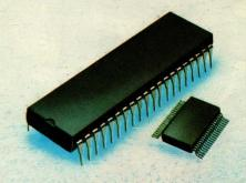
Philips also put the PCD3343 and other ICs in space-saving SO mini packages. Comparison shown here is between 40-pin DIL and 40-pin SO.
