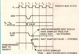
Fig 6—Early wait requests to the NS32016 μP can inhibit generation of strobe signals, thus freezing the system. A wait-state-generation scheme employing a timing-control unit (Fig 7) is one method of solving this problem.
