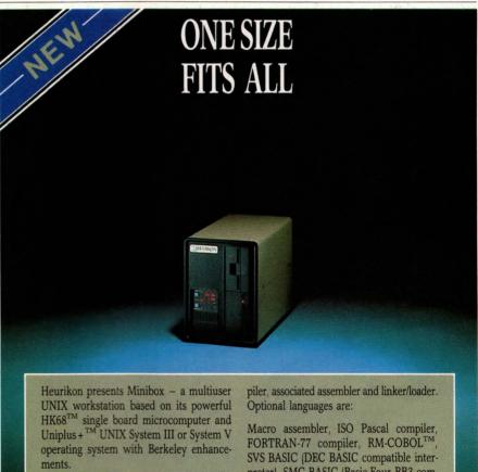
Designed with the OEM in mind, one size fits all. Both compact and flexible, the Minibox includes within its 10.5"w x 13.9"h x 20.5"l frame a 200 or 400 watt power supply, six slot Multibus<sup>TM</sup> card cage, (4-5 available for user use!), single double density floppy disk drive, streamer tape drive, and 31 or 65 Mbyte Winchester drive (expandable to 280 Mbytes). All this within the same cabinet! System status LEDS on the front panel inform the user of CPU and disk drive activity.
