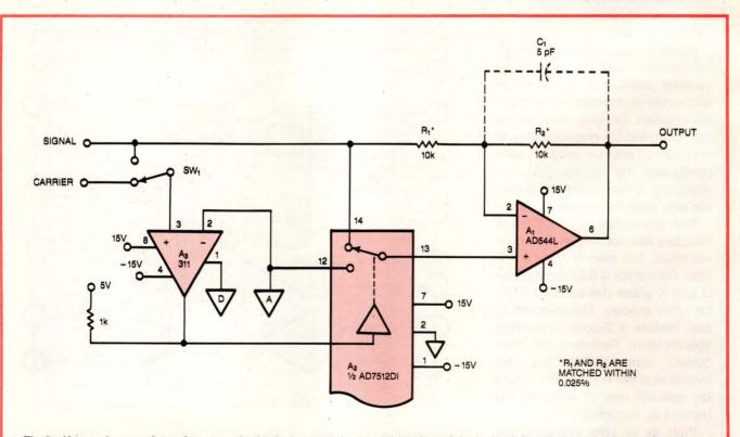
Fig 3—Known by a variety of names, the basic commutating modulator/demodulator circuit is called a sign-bit amplifier when comparator  $A_3$ 's carrier input, selected with switch  $SW_1$  in the position shown, is a sign-bit signal. When the signal serves as  $A_3$ 's input, the circuit is called an absolute-value or precision-rectifier circuit.
