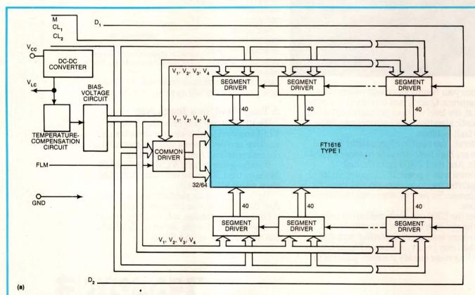
Fig 1—Requiring different drive circuitry, Types I and II are constructed with upper and lower sections and with a single section, respectively. Type I needs two data-drive lines (a); Type II has lower contrast but requires only one data line (b).
