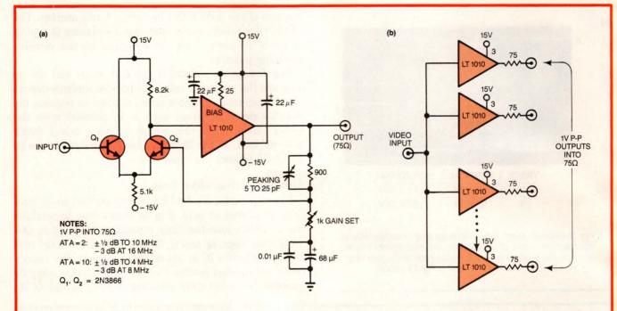
Fig 3—Suitable for video applications, these circuits provide standard 1V p-p composite-video signals into 75 $\Omega$  lines. The circuit in (a) provides variable gain. The one in (b) allows you to drive multiple video lines.
