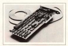
LAN. AST-PCnet is a shared resource system that incorporates twisted-pair technology and print spooling. Its total network capacity is 160 workstations and 2500 ft of
