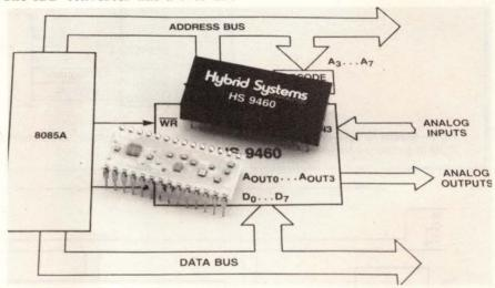
Offering both data acquisition and distribution, Model HS9460 hybrid I/O subsystem allows easy interface to most 8-bit microprocessor buses.
