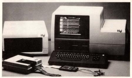
In a dedicated μP development system, in-circuit emulation, logic-timing analysis and high-level-language software debugging occur via a common user interface. This system is Intel's Series IV with its integrated instrumentation and in-circuit emulator (I²ICE).
