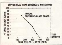
After 540 thermal cycles from -55° to 125°C failed to break chip carrier solder joints, Collins Avionics halted tests of PC board used in F-15 communications system. Reliability goals had been surpassed by a wide margin.
