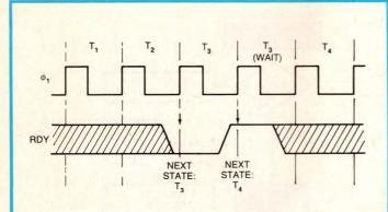
Fig 5—Adding wait states allows 16-bit  $\mu$ Ps to operate with slow 8-bit memories or peripherals. If at the beginning of  $T_3$  the  $\mu$ P's RDY line is Low, the next state becomes a wait state, or essentially a repeat of the  $T_3$  cycle.
