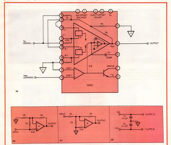
Fig 4—A building block IC like the AD630 can be turned into a balanced modulator/demodulator (a) similar to that in Fig 3. Using the chip's precision resistors to set the gain (to a value of 2 with the configuration shown here) eliminates the need for trimming in most applications. The equivalent circuits seen when looking into the AD630's input when channel A or B is active are shown in (b) and (c), respectively, and the supply-conditioning circuitry for the chip appears in (d).
