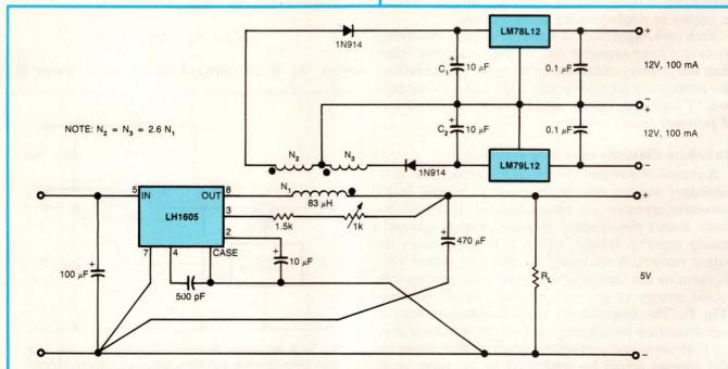
Fig 3—At the heart of this buck-type converter, an LH1605 switching regulator controls a 5V, 5A main output channel. Linear post regulators hold the derived secondary outputs to  $\pm$ 12V at 100 mA.
