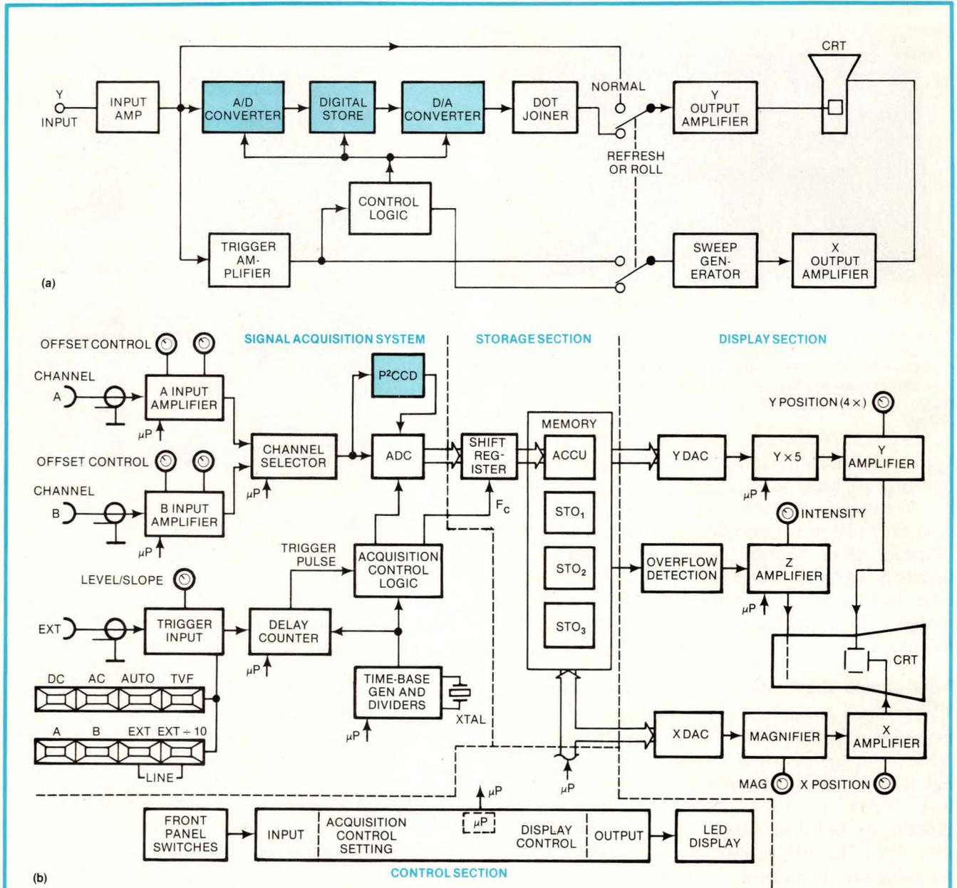
**Fig 2—The simplified block diagram of one channel of Gould's Model DSO4000 (a) illustrates that the scope provides a choice of analog nonstorage operation or digital-storage capability. The diagram of Philips's Model PM 3310 (b), however, illustrates that this scope furnishes only digital-storage operation. Note that the P<sup>2</sup>CCD (profiled peristaltic charge-coupled device) can sample**
