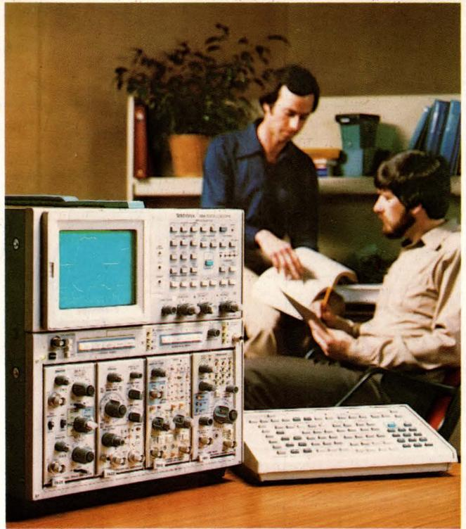
Aimed at both production and laboratory applications, Tektronix's Model 7854 can capture waveforms and then determine such parameters as rise time and rms levels. The programmable instrument's calculator-type keyboard lets you tailor it to your measurement applications.
