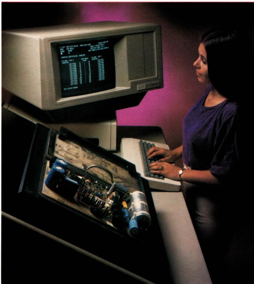
A large 14-in. CRT screen displays prompts to users of Fluke's Model 3200A, simplifying the in-circuit tester's operation. The ability to handle as many as four stations per controller holds down costs.
