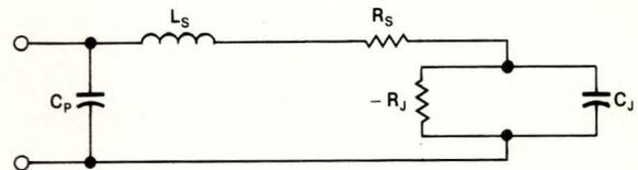
The equivalent circuit of a tunnel diode consists of five basic elements:  $R_j$  is dynamic junction resistance;  $C_j$ , junction capacitance;  $R_s$ , dc resistance;  $C_p$ , total package capacitance;  $L_s$ , package inductance.
