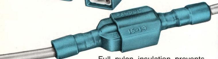
Full nylon insulation prevents shocks or shorting if energized circuit is disconnected. Wire sizes #22 through #14. Female can be used alone as a fully pre-insulated disconnect.
