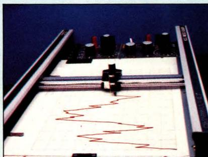
The Series 100 records on 8½" x 11" (DIN A4) paper and displays  $Y=f(X)$  or  $Y=f(T)$ . The linear bearing supported pen bar assures alignment for the lifetime of the recorder. All electrical and mechanical components are easily accessible by simply removing four screws on the bottom panel.
