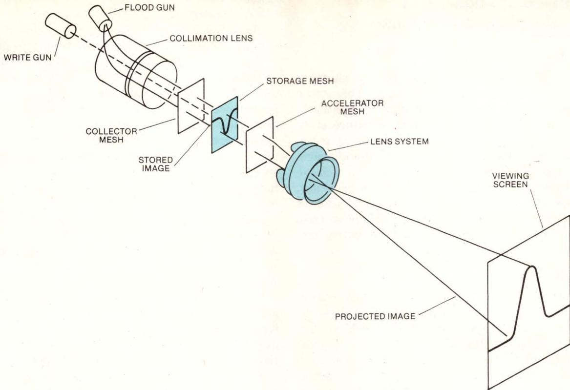
**Fig 6—An expansion-type storage CRT** combines a small precision storage mesh with a static-electric-field lens system to achieve high writing speeds in both Variable Persistence and Single Shot modes.
