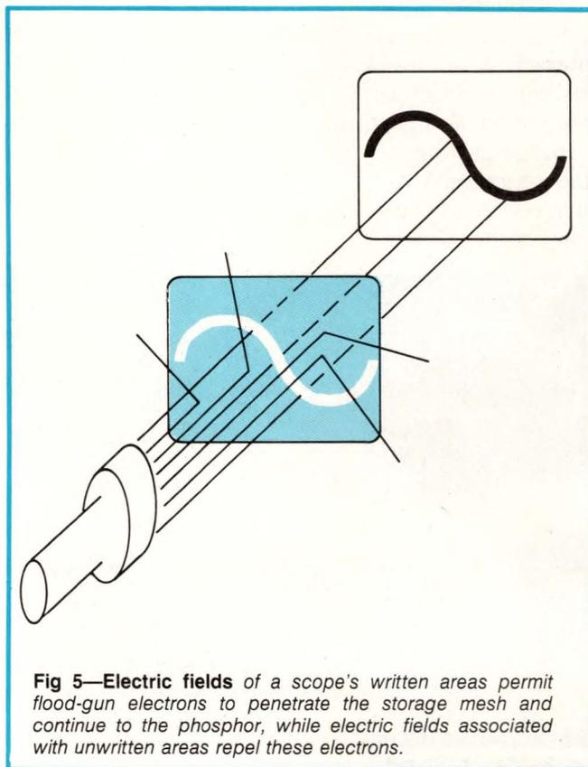
Fig 5—Electric fields of a scope's written areas permit flood-gun electrons to penetrate the storage mesh and continue to the phosphor, while electric fields associated with unwritten areas repel these electrons.
