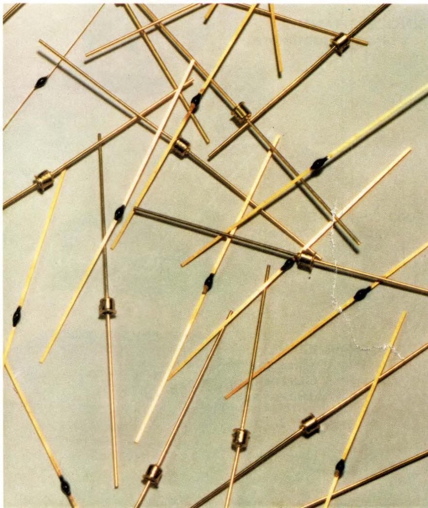
Compare the relatively large package of General Electric's standard 3700 Series tunnel diodes with the tiny Series TD-260 packages. The ultralow capacitance of the latter devices contributes to their very-high-speed switching characteristics.
