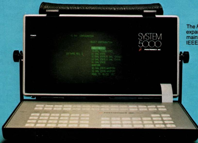
The *PI-540* resides in the expandable System 5000 mainframe. RS-232 and IEEE-488 interfaces are available.
