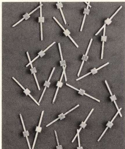
**Developed to integrate tunnel diodes** directly onto microstrip and microline circuit boards, these microwave packages from Custom Components provide good continuity of the transmission-line impedance into the semiconductor chip.
