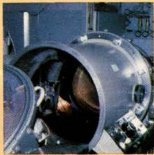
Ion beam system etches Resistor Research resistors in production quantities.
