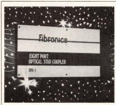
**STAR COUPLER.** Furnishing 16 connection points (eight input fibers optically coupled to all eight output fibers), the 8-port Model EPS-1 permits a remote computer or central processor to link with as many as seven terminals or peripherals using graded-index optical fibers. A totally passive device, it provides typical excess loss of 5 dB and
