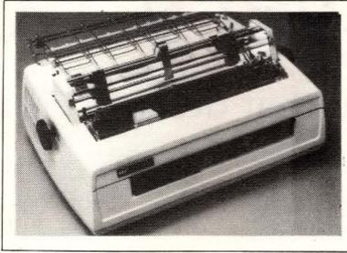
user-installable forms-handling options, 115/230V ac universal power supplies and enhanced diagnostic self test. Terminal models furnish an optional word-processing feature that permits creation of graphs, plots and bold-face printing. OEM units, from \$1254; terminal models, from \$2170 (100). Delivery, 30 to 60 days ARO. **NEC Information Systems Inc**, 5 Militia Dr, Lexington, MA 02173. Phone (617) 862-3120.
