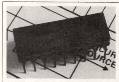
**DAC.** A 10-bit IC with sign-magnitude coding, DAC-210 provides 1.5- $\mu$ sec settling time and nonlinearity over full temperature range as low as  $\pm 0.075\%$  FS. Containing an output amplifier, reference, logic-controlled polarity switch and ladder-network switches, it's directly
