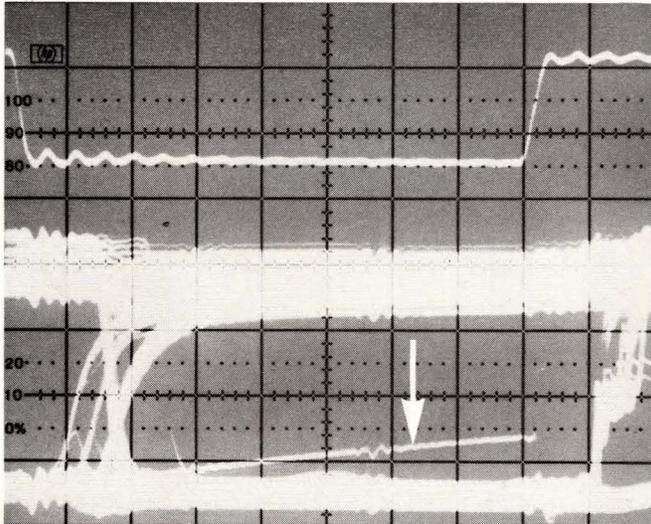
Fig 2—Very high persistence settings extract a floating-bus condition (arrow) that could go unnoticed with conventional oscilloscopes.
