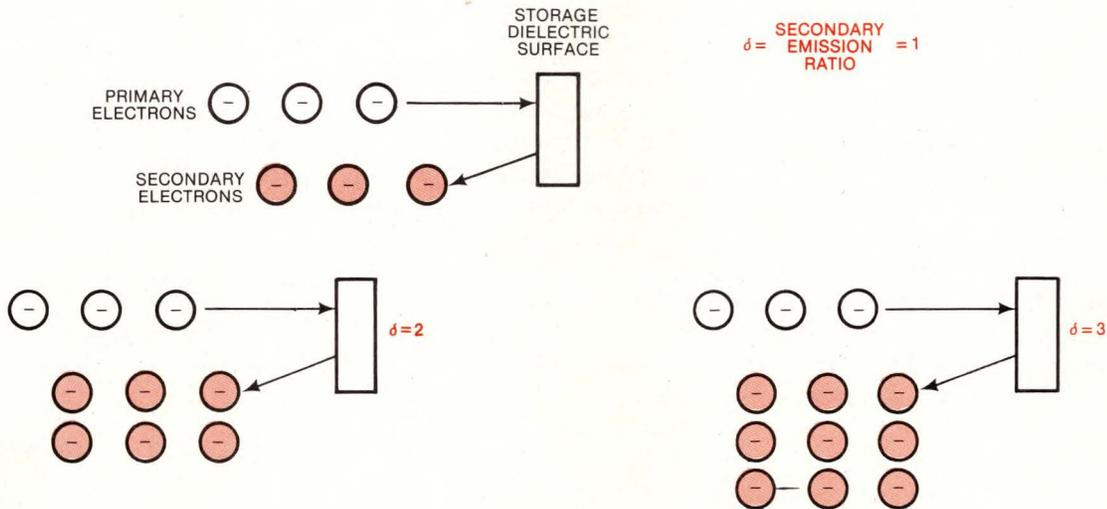
Fig 4—The secondary-emission ratio ( $\delta$ ) is defined as the average number of secondary electrons emitted from a bombarded material as a function of primary-electron energy.
