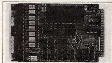
**μC BOARD.** Providing sockets for 8k to 32k bytes of ROM and EPROM and 64k bytes of dynamic RAM, the 4-MHz Z80 MCP80-800 STD Bus card requires no Wait states when used with the on-board RAM and 350-nsec-access-time ROMs. 16k blocks of RAM and ROM can be selectively enabled or disabled by software via a memory-map port and its associated bipolar PROM. A com-
