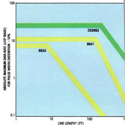
\*Twisted pair cable (22 AWG stranded), terminated 180 // 390 Ω, 50% duty cycle.
