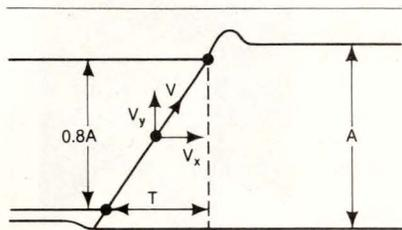
**When calculating maximum spot velocity for single-shot pulse measurements, assume that the quantity equals the average velocity between a waveform's 10% and 90% points.**
