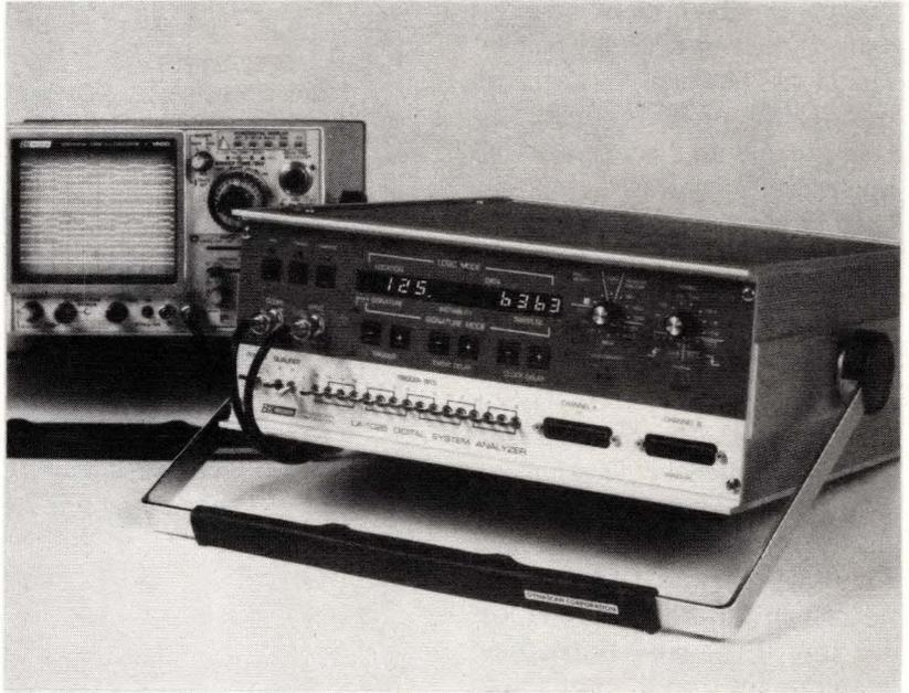
Featuring signature-analysis capability, Model LA-1025 logic analyzer displays state data on its 12-digit LED readout or timing diagrams on a conventional oscilloscope. It contains a 16-channel $\times$ 250-word memory and 18 trigger qualifiers and operates at rates as high as 20 MHz. The companion LA-1020 has the same features except for signature-analysis capability.
