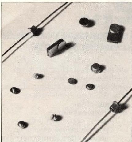
**Ge and GaAs back diodes**, such as these from Microwave Associates, suit mixers and detectors through the Ku Band. Packages are available for waveguide, coaxial, stripline and microstrip applications.
