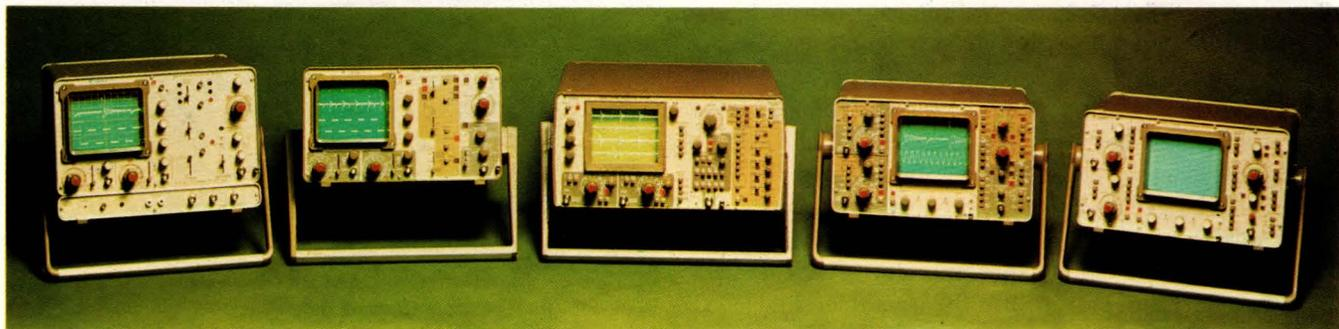
A line of five digital-storage scopes from Gould includes models that provide sampling rates to 10 MHz, vertical resolutions to 10 bits and real-time bandwidths to 25 MHz. For example, Model DSO4020 features a 2-MHz sampling rate, 8-bit vertical resolution, 4k bytes of RAM and an IEEE-488 interface, and Model DSO440 offers 4-trace capability.
