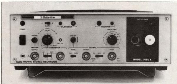
Add pre-trigger and storage capabilities to a nonstorage scope with Ballantine's Model 7050 A electronic signal recorder. This 100-kHz instrument can store a transient signal lasting 20 msec or less on a continuous magnetic-tape loop for subsequent display on a standard real-time scope's CRT.
