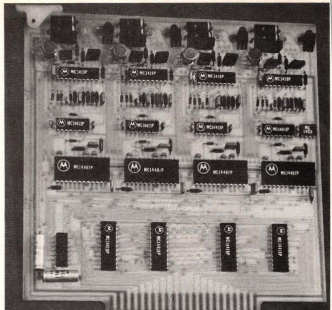
**Fig 3**—One  $\mu\text{P}$  controls four channel banks of 32 channels each for a total of 128 subscriber lines. Because the  $\mu\text{P}$ /ITSAC interface requires two frames (250  $\mu\text{sec}$ ) to transfer to each channel, the entire 128 channels can be updated every 32 msec. You can mount eight of these cards in a 343-in.<sup>3</sup> space to service 32 customers.
