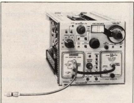
**Pulses with 25-psec rise times** are generated by high-speed tunnel switching diodes in the Type S-6 sampling head of this Tektronix Model 7S12 time-domain-reflectometry plug-in. Sampling scopes use similar front ends.
