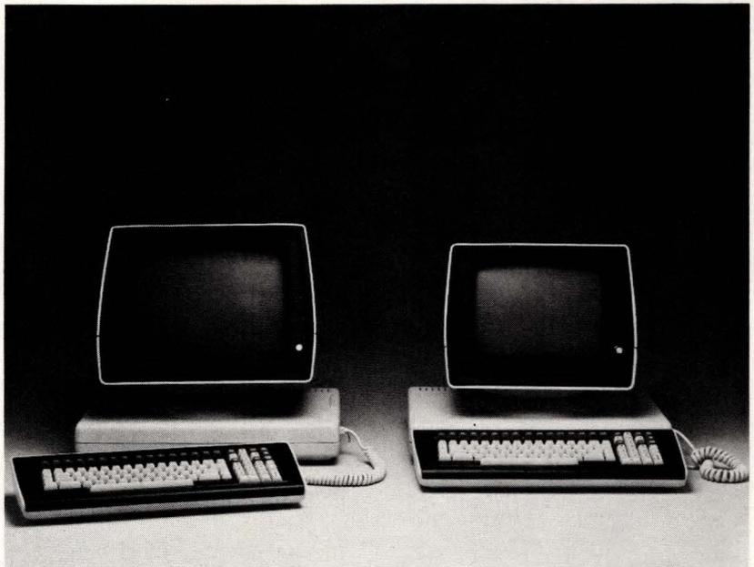
**For OEMs that need flexibility in custom applications, Zentec's Series 8000 modular intelligent terminals include a video module (12- or 15-in. monitors), a logic module and a detachable keyboard module.**
