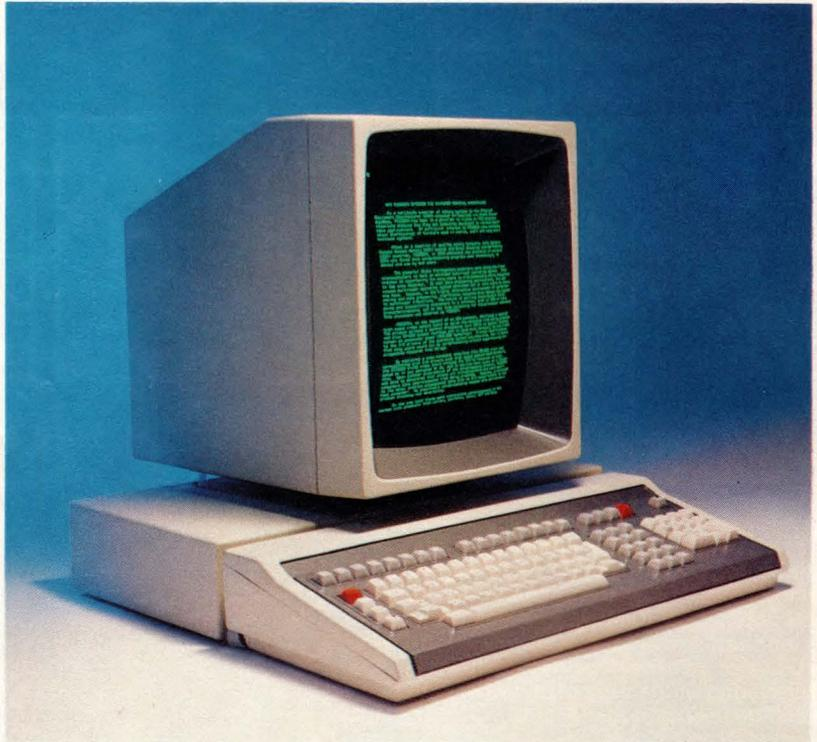
Displaying 66 80-character lines in a full-page format, Model 2010 intelligent terminal employs an Intel 8086  $\mu$ P and provides two RS-232C serial ports and a detachable 107-key sculptured keyboard.
