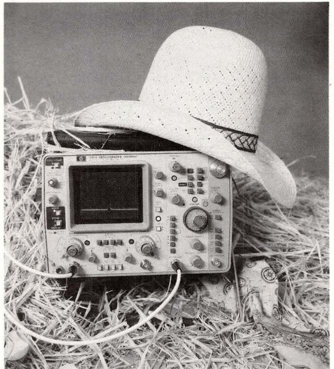
**Variable-persistence oscilloscopes** such as Hewlett-Packard's Model 1741A perform the electronic equivalent of finding a needle in a haystack—they can sort out one wayward signal from several thousand sweeps.
