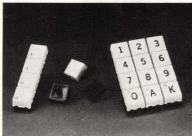
**Compatible with wave-soldering and immersion-cleaning assembly operations, 0.25-in.-square 225 Series pushbutton switches utilize an internal sealing system that reduces parts count to increase reliability—lifetime specs at  $10^6$  operations.**
