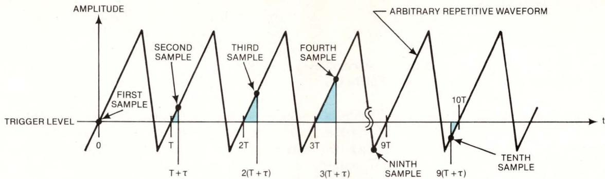
**Fig 3—This sampling technique** can digitize repetitive waveforms with frequencies higher than the sampling rate. In this example, the first sample of a waveform of period  $T$  is taken at the initial trigger point at  $t=0$ . The second trigger point occurs one period later at  $t=T$ , but the second sampling is delayed until a time  $\tau$  after this trigger point; thus, the second sampling occurs at  $t=T+\tau$ . The sampling time is then delayed  $2\tau$  after the third
