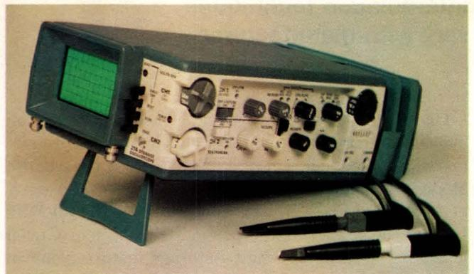
Weighing 3.5 lbs and measuring 3×25×29.5 in., the 500-kHz dual-trace Model 214 from Tektronix is the smallest available storage scope. Its bistable CRT achieves a 0.5-div/μsec (0.52 cm/div) stored writing speed and storage times to 1 hr.
