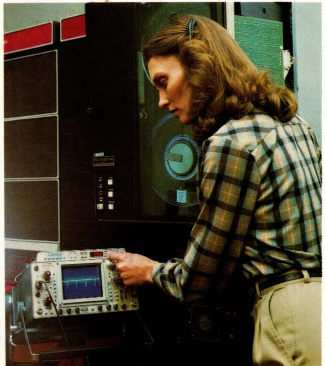
**Suited to portable operation,** Tektronix's Model 468 digital-storage scope furnishes 100-MHz nonstorage capability and achieves a 25-MHz sampling rate. Combined with the unit's sinusoidal-interpolation function, this rate yields a 10-MHz useful storage bandwidth.
