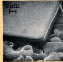
Massive SEM enlargement shows clean wall of ion beam etched conductor pattern.
