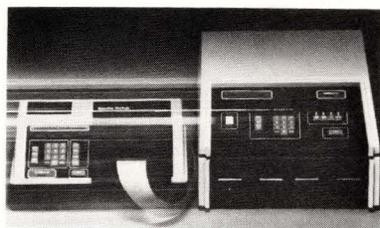
**Meeting manufacturing requirements, Model 100A production PROM programmer and Model 200A data-control unit team up to handle programming, testing and recordkeeping chores.**
