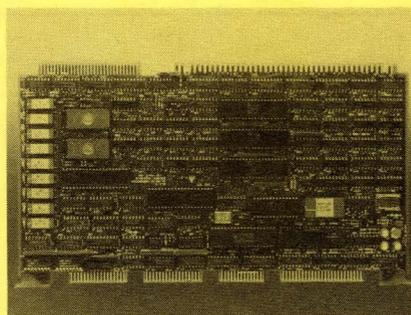
Heurikon presents the MLZ-91A with Z80A CPU, floppy controller, winchester and streamer I/F, DMA, AM9511 math chip, GPIB I/F, 32K/64K RAM with parity, 2 ROM sockets, 2 RS232 ports (RS422/423 option), 4 counter/timers, 20 bit Intel Multibus, Bi-directional bus I/F, memory mapping RAM, I/O map, user defined LEDS and dip switch positions, CP/M and MP/M operating systems. **Heurikon Corporation**, 3001 Latham Drive, Madison, Wisconsin 53713. (608) 271-8700.
