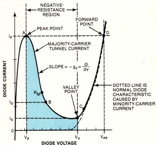
The reverse slope on a tunnel diode's static V-I curve defines its negative-resistance region. Note the normal operating point ( $R_N$ ) in the region of minimum noise and the point of minimum negative resistance ( $R_M$ ).
