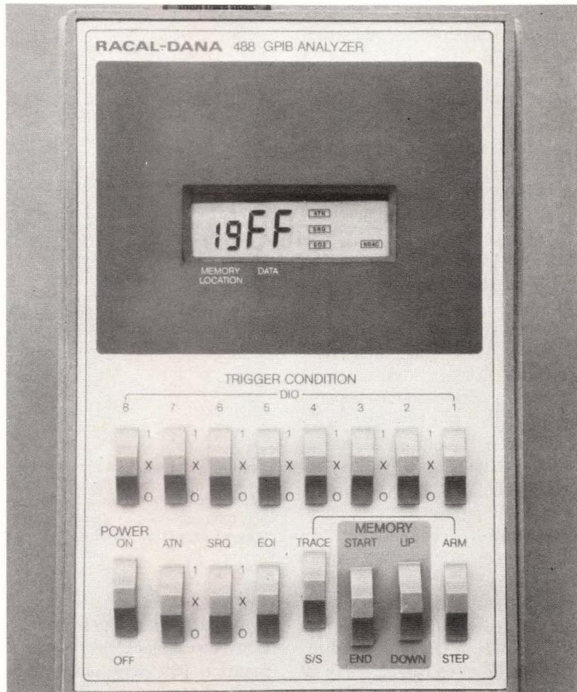
**Battery operation, 40 words of memory and three operating modes allow Model 488 bus analyzer to help you debug IEEE-488 systems. The LCD reads out data in 2-digit hexadecimal format and memory locations in 2-digit decimal format. And it provides direct readout of handshake- and housekeeping-line status.**
