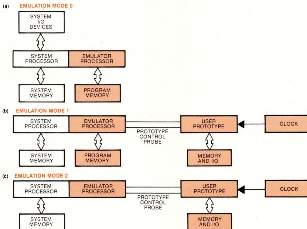
**Emulation modes** define the functions performed by an emulator and those executed by its associated development system. In Mode 0 (a), the development system and the emulator can simulate prototype software operation without the need for the prototype's hardware. In partial emulation, Mode 1 (b) allows the emulator's program memory to access both the development system's and prototype's memories. Mode 2 (c)—the Full Emulation mode—employs the prototype's memory, clock and I/O facilities.
