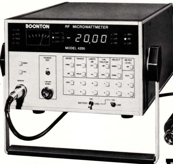
non-volatile memory with interpolated cal factors automatically applied after frequency entry.
