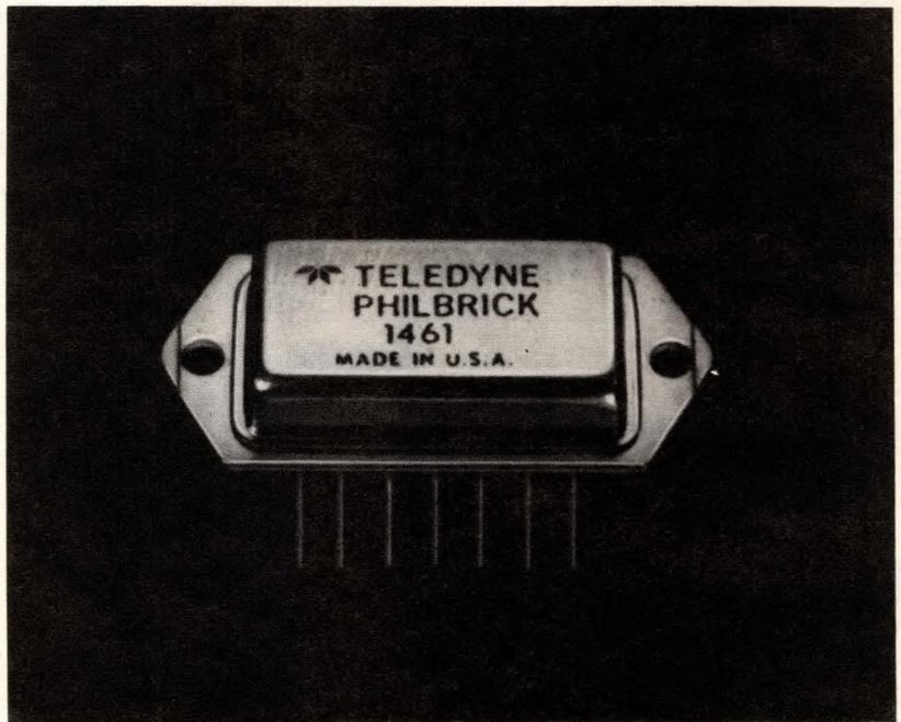
Combining  $\pm 30V$ ,  $\pm 600\text{-mA}$  output capability and 1-GHz gain-bandwidth product, Model 1461 op amp furnishes a typical input noise of  $1.5\text{ }\mu\text{V rms}$  from 100 Hz to 10 kHz.
