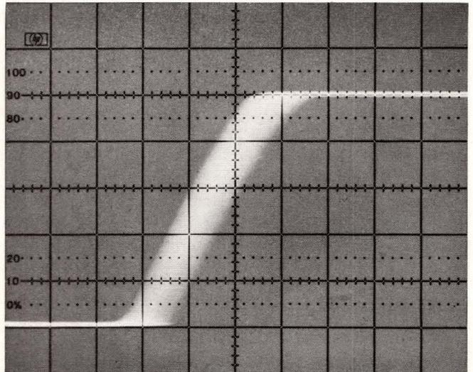
Fig 3—Jitter is clearly defined and easily measured using variable-persistence measurement techniques.
