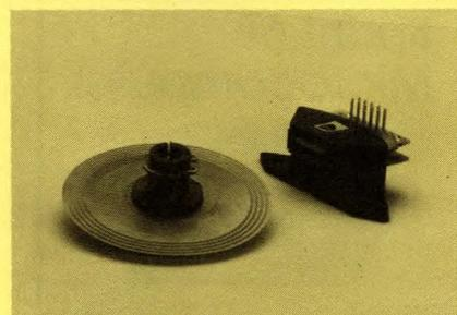
A DRC breakthrough in encoder technology, incorporated into our new Series 560 Modular Optical Incremental Encoders, allows operation at gaps of  $.03" \pm .02"$ . This insensitivity to gap variations means fast, easy integration for volume production applications. These low-cost encoders are available in resolutions to 500 cycles/revolution with sinusoidal or TTL output. Get more information today.
