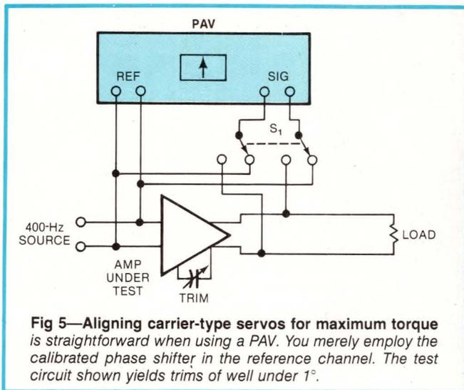
**Fig 5—Aligning carrier-type servos for maximum torque is straightforward when using a PAV. You merely employ the calibrated phase shifter in the reference channel. The test circuit shown yields trims of well under 1°.**
