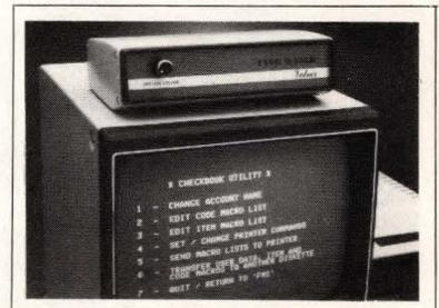
**SPEECH SYNTHESIZER.** Type-'N-Talk text-to-speech synthesizer permits an RS-232C-interfaced personal computer to reproduce words typed on the keyboard in English words and phrases. Without using the host memory, words can be spoken simultaneously as soon as they are typed, and the 750-character buffer can hold them until the user prompts the computer to speak in phrases or sentences. The phonetic speech is heard
