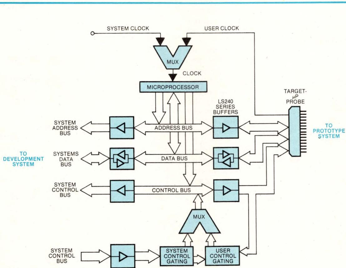
**Fig 1—With help from a development system, an emulator can monitor, control and modify the interaction between a  $\mu P$ -based prototype's hardware and software. To carry out these tasks, it contains interface, control and gating logic, buffers and multiplexers and a  $\mu P$  that closely resembles that of the prototype.**
