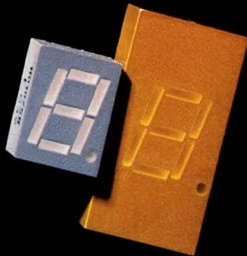
Shown above is the new .28" LED display VS the standard .3" display.
