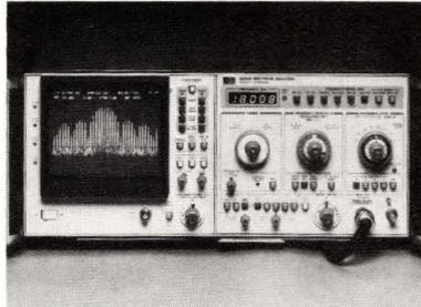
**Featuring 10-MHz to 22-GHz operation, Model 8569A provides  $\mu$ P control that suits it to production test.**
