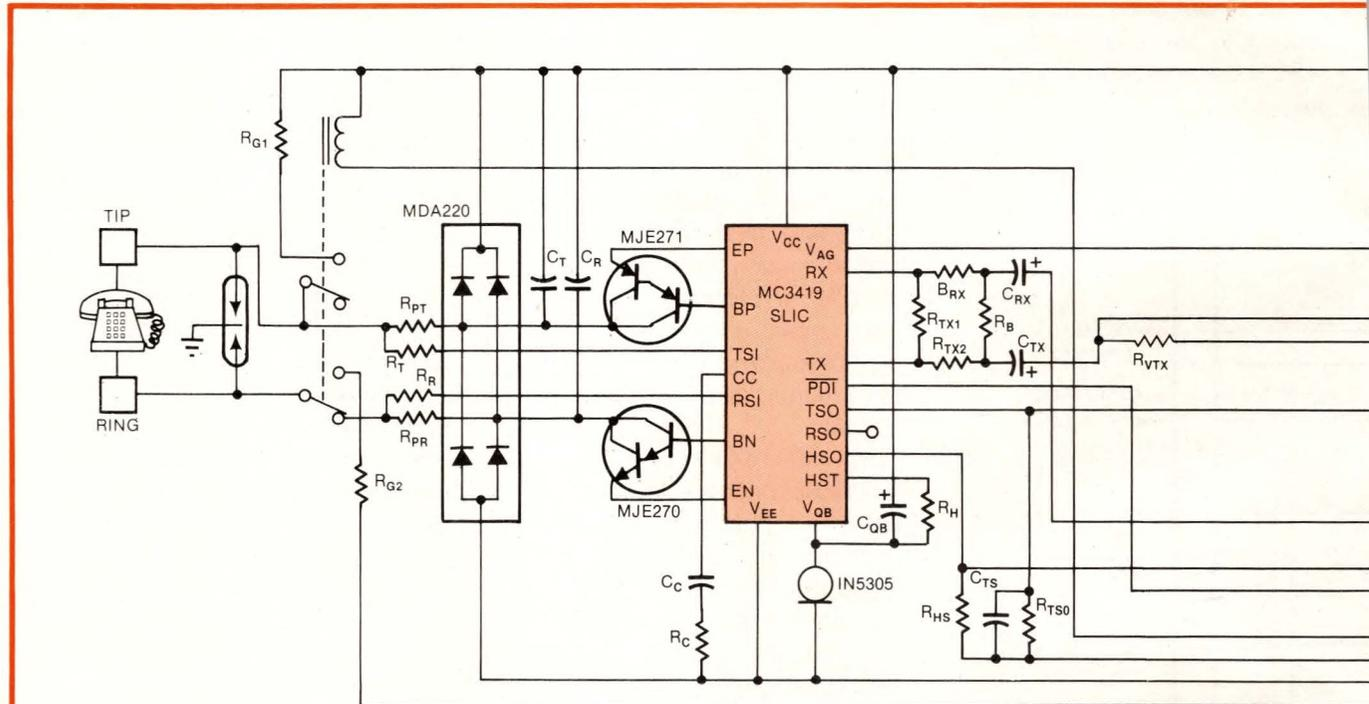
**Fig 2**—Each subscriber-channel unit (SCU) employs several dedicated digital ICs to perform critical voice- and status-data handling. In addition to the codec, filter, SLIC and TSAC ICs, the circuit contains several logic-controlled transmission gates, a voltage-regulator IC and a diode-bridge transient arrester.
