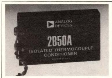
**THERMOCOUPLE CONDITIONER.** Featuring pin-programmable cold-junction compensation, Model 2B50 also provides input protection, filtering, isolation and screw terminals for direct connection of Type J, K, R, S, T, E and B thermocouples. Key specs in-
