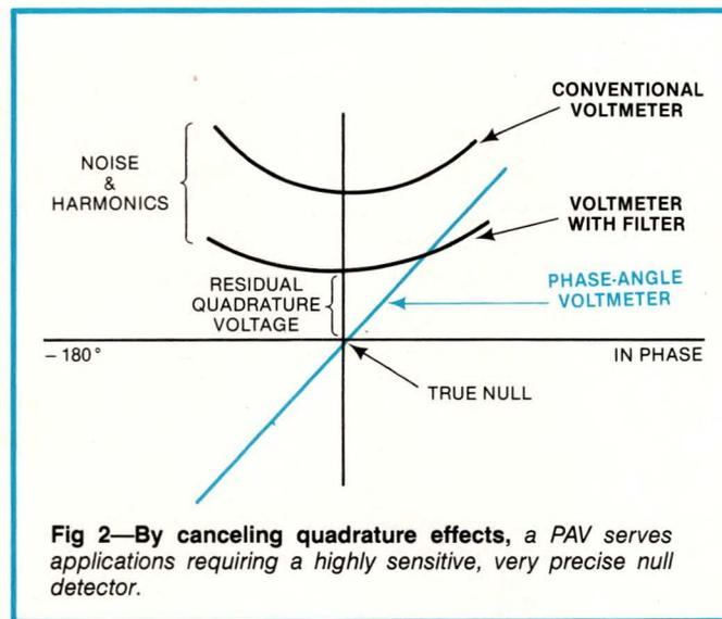
voltage—proportional to the signal's fundamental component—whose value is multiplied by the cosine of its phase angle with respect to a reference voltage. The demodulator also eliminates harmonic effects to any desired degree.
