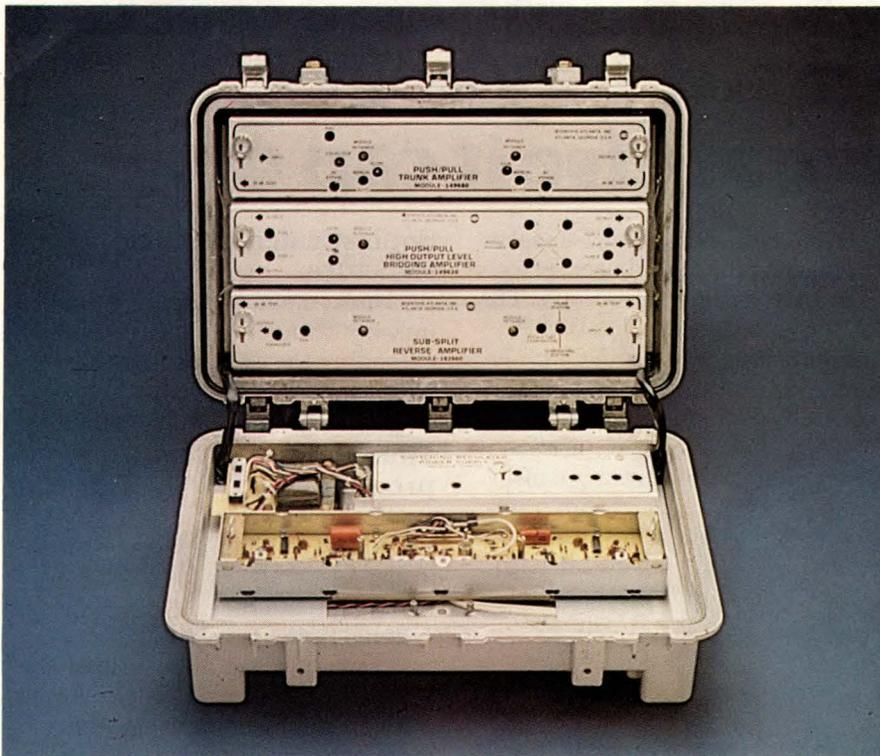
Tunnel diodes detect pilot-signal levels to compensate for changes in cable attenuation with temperature in this Model 6540 ABR cable-TV trunk repeater/amplifier from Scientific Atlanta. Control signals generated by the back diodes correct for attenuation as a function of both cable length and frequency.
