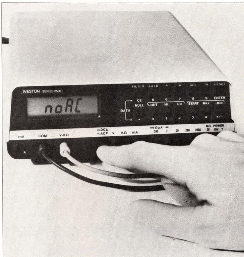
**Operator-prompting functions and computational capabilities useful in DMM applications highlight Weston's Series 6500 DMMs. Here, an instrument warns that the ac mode is incompatible with resistance measurements.**
