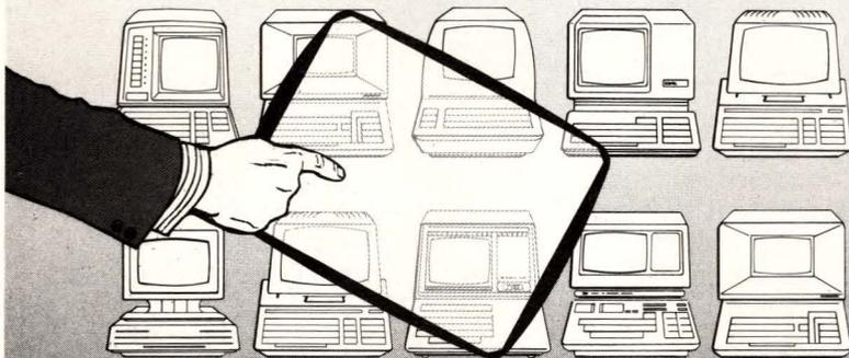
With the touch of a finger on the Elographics E270 Position Sensor, the coordinates of the touch point are transmitted to your terminal or computer for limitless menu and graphic applications. Replaces light pens and joy sticks. Opens new applications where finger touch simplicity is a must.
