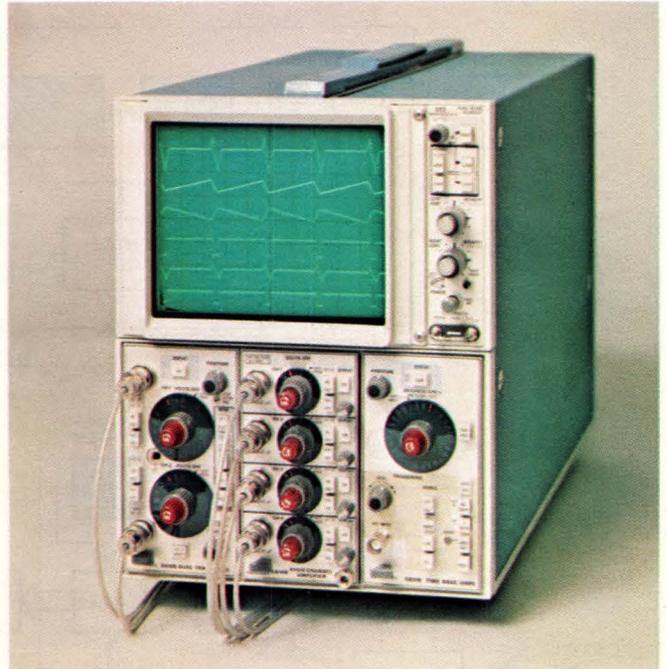
Dual-beam performance highlights Tektronix's Model 5113, which features split-screen bistable operation and writing speeds to 0.25 cm/μsec with an optional fast-writing-speed CRT. Standard writing speed equals 25 cm/msec.
