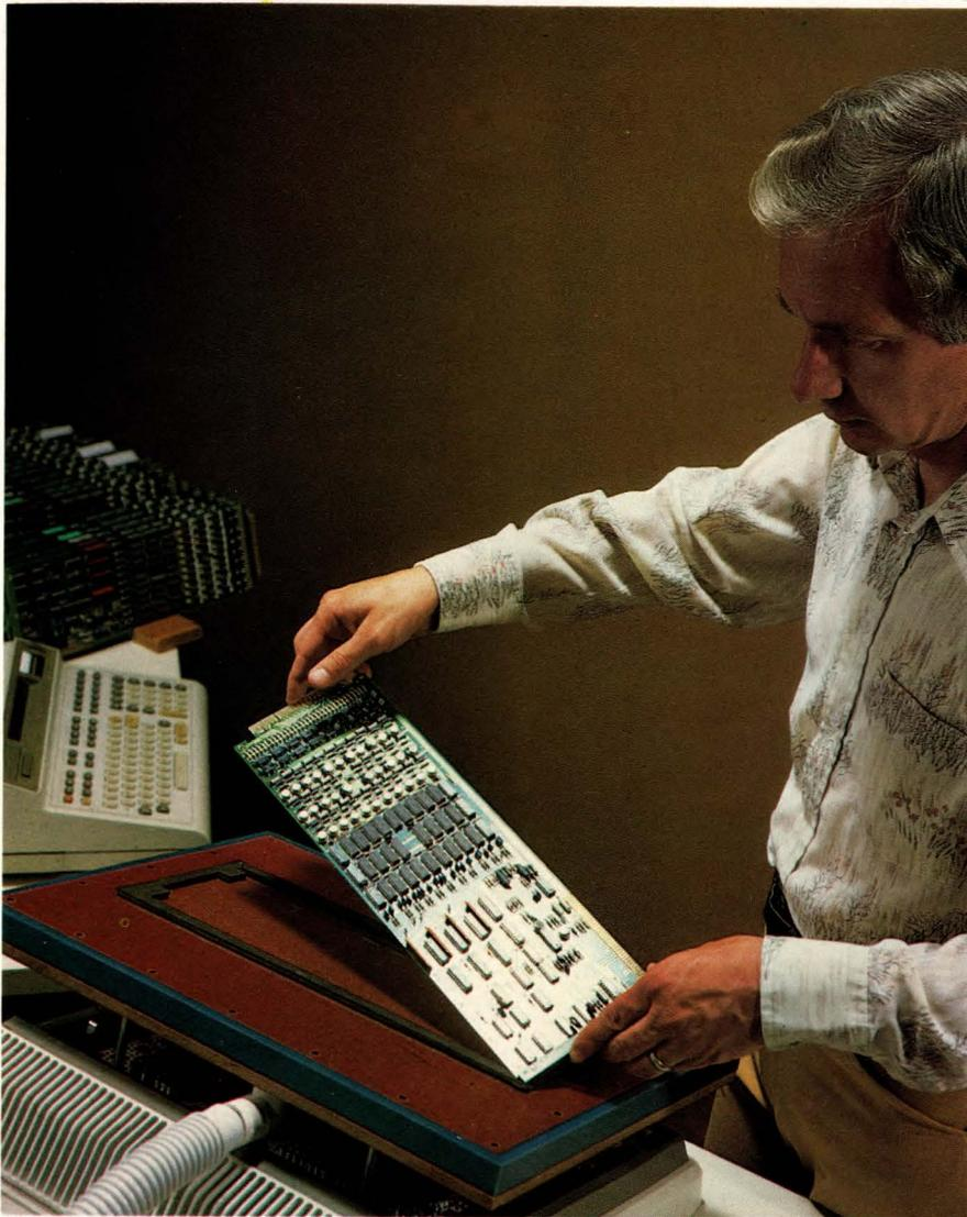
Bed-of-nails fixtures aren't limited only to in-circuit board testers. The Hewlett-Packard Model 3060A can also perform functional board tests.
