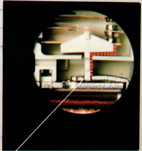
The path between coil and contacts is greater than 8mm.
