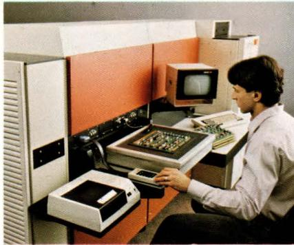
Parallel stimulus/response facilities help test digital boards in GenRad's Model 2270 in-circuit test system.
