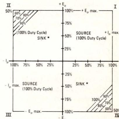
\* derating as a function of duty cycle or temperature
