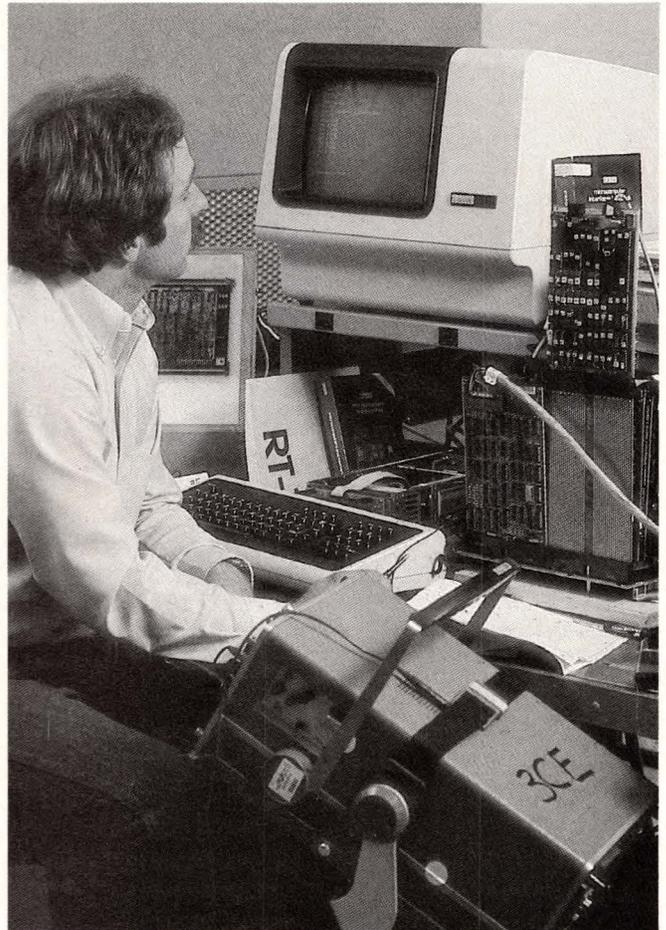
*Writing software on a target product often proves difficult. Most lack the built-in development tools found in this system from Digital Equipment Corp.*
