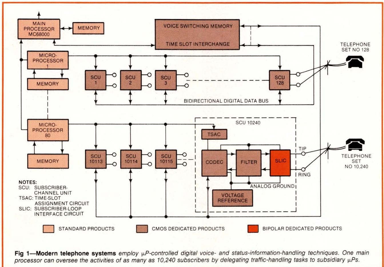
Fig 1—Modern telephone systems employ  $\mu$ P-controlled digital voice- and status-information-handling techniques. One main processor can oversee the activities of as many as 10,240 subscribers by delegating traffic-handling tasks to subsidiary  $\mu$ Ps.
