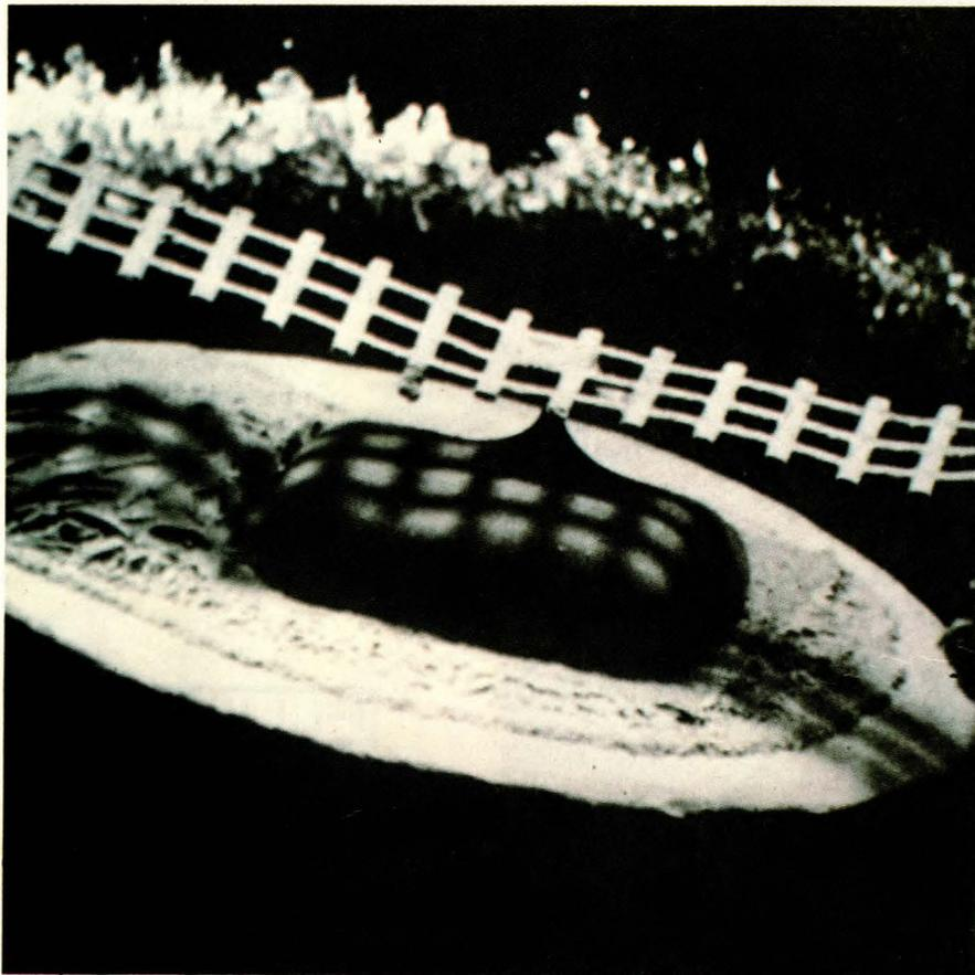
Basic construction of a mesa-type tunnel diode consists of a junction alloyed to a mesh contact that minimizes device capacitance. (Courtesy Aertech Industries)
