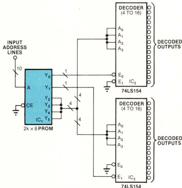
Decode nonconsecutive addresses by using a PROM to translate the inputs to a format that can then be sorted out by an m-in/n-out decoder. Here, the PROM's most significant output allows the decoders to yield a 32-of-1024 sort.
