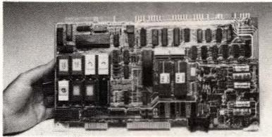
Featuring large vocabulary capacity, high-fidelity speech and 3-way interfacing, the Speech 1000 synthesizer board allows computers to generate recorded voice responses.
