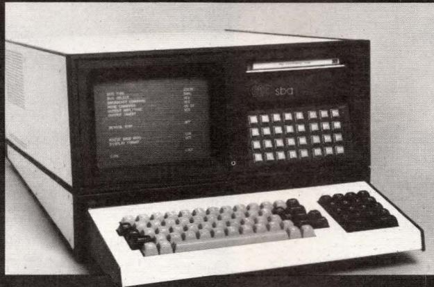
simulation device. The Serial Bus Analyzer will verify subsystem design and integration, confirm system integrity, and provide implementation of system standardization. It will also actively stimulate the bus with messages and programmed errors.
