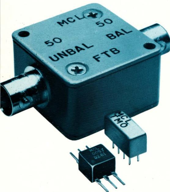
Select from the economical, microminiature T-series (plastic case) or TMO series (hermetically-sealed metal case) covering 10 KHz to 800 MHz. These models operate from 12.5 to 800 ohms with insertion loss typically less than 0.5 dB. For large dynamic range applications, specify the T-H series which can handle up to 100 mA primary current without saturation or distortion.
