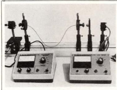
Fiber Parameter Measurement System comes in modular form on an optical bench. Measurements are possible at as many as five user-selectable wavelengths. \$2750. Delivery, 4 to 6 wks ARO. **Math Associates Inc.**, 6 Manhasset Ave, Port Washington, NY 11050. Phone (516) 944-7050. **Circle No 238**
