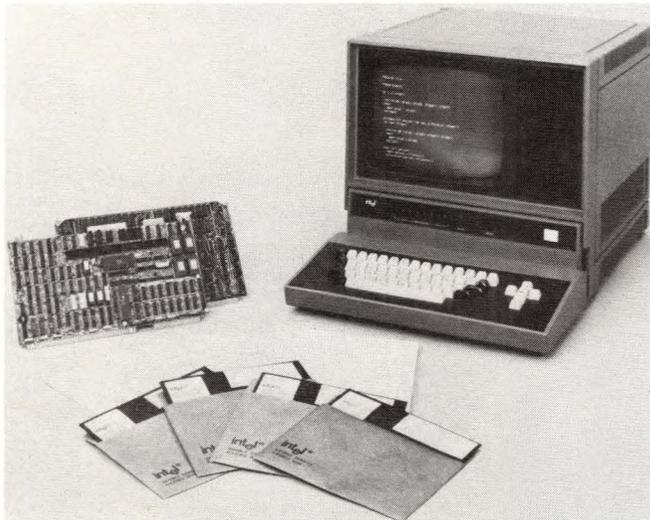
**A single-user development system, such as this Intel Intellec unit, has its own computer and is optimized for a particular processor or processor family.**
