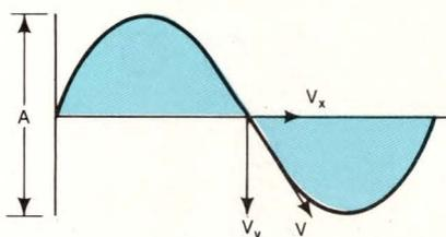
When a CRT beam writes a sine wave, the vector spot velocity ( $V$ ) is composed of a vertical ( $V_y$ ) and horizontal ( $V_x$ ) component.
