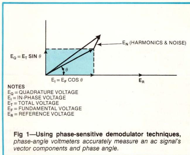
Complex ac-signal measurements thus demand an instrument capable of monitoring a signal while ignoring the noise and distortion in typical ac-control- and servo-system applications. The phase-angle voltmeter meets these requirements.
