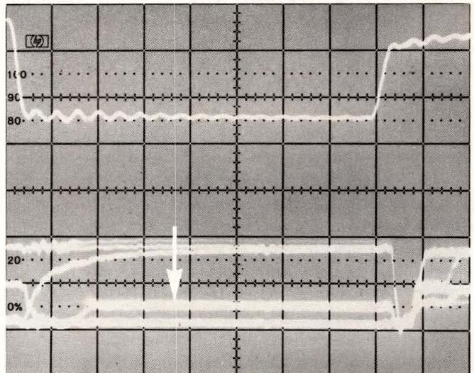
Fig 1—Monitoring a  $\mu$ P data bus (lower trace) during a read strobe (upper trace) shows that a high-persistence setting easily captures the data-bus-conflict condition between the logic levels (arrow).
