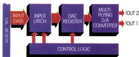
And since they're all monotonic with differential non-linearity specified over temperature, they fit particularly well in either fixed or multiplying reference applications such as servo control or synchro-to-digital converters. Thanks to their low cost, these new 8-, 10- and 12-bit D/As can also be used as programmable gain amps, digital attenuators, band-pass filters and more.
