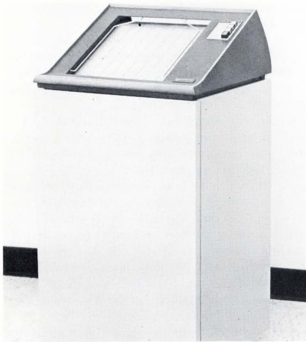
Non-impact dot-matrix line printer uses an electrostatic writing technique. It prints at 500 lines/min. (132 char/line). (Versatec)
