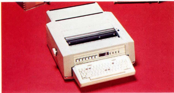
Full-character serial-impact chain printer in foreground prints up to 120 characters/sec. (General Electric)
