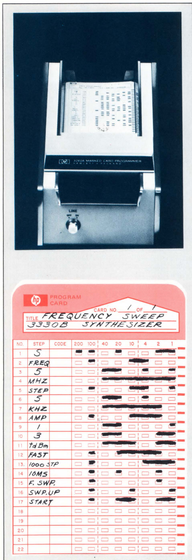
Fig. 10—Playing cards with a bus. Byte serial data programs the automatic synthesizer for a complete frequency sweep in a half a second.
