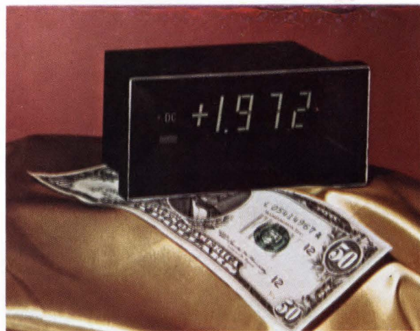
Low-power consumption, especially for the reflective-types, is one of the major advantages of liquid-crystal displays.
