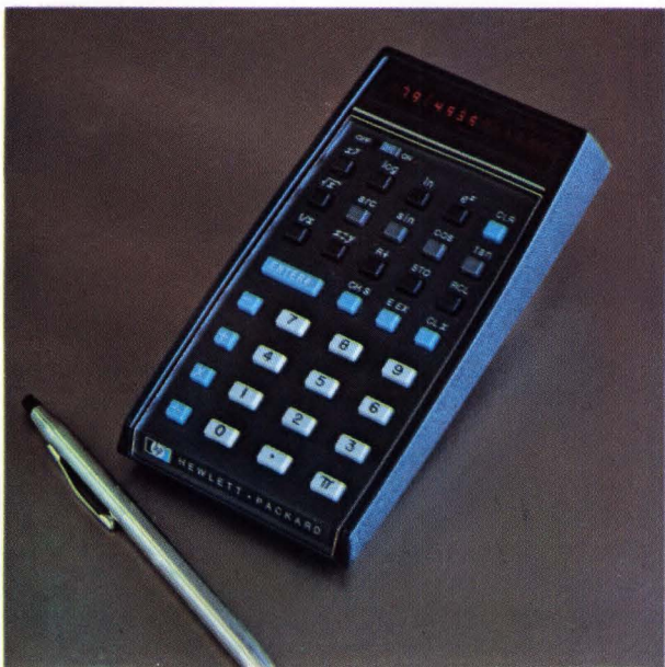
LED displays can be made to look larger than their actual physical size by the use of magnifying lenses. This technique is used in the readout of the Hewlett-Packard Model 35 hand-held calculator.
