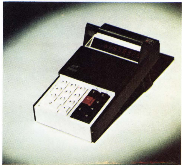
In the flat-plane, gas-discharge displays of Sperry-Rand, the digits appear to be continuous, even though each is actually made up of 7 discrete segments.
