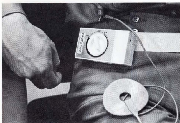
Fig. 2—The stimulator package is held by a belt worn by the patient (top). Connection from the antenna to the stimulator can be made with one hand (bottom).
