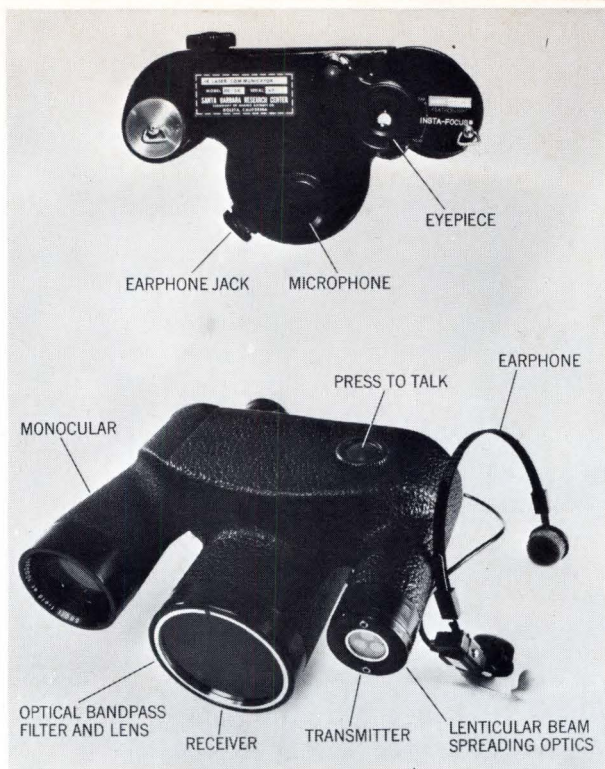
IR laser communicator provides secure point-to-point communications to a range of four miles.
