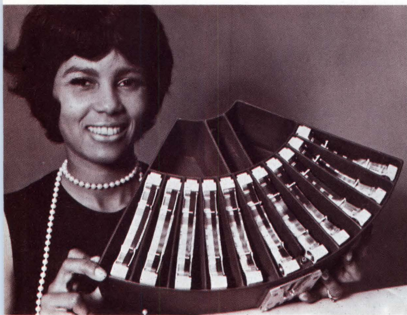
Cartridges fit into MASSTAPE Pacs, providing a half-billion bytes of removable storage.
