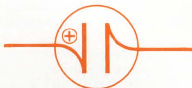
Fig. 1—Symbol and equivalent low frequency circuit of the energy storage device (ESD).
