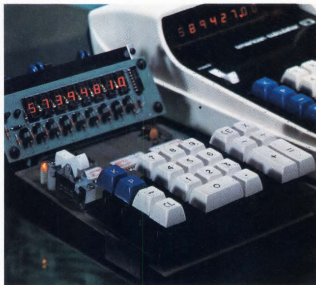
Close look at keyboard shows the K (multiply or divide by a constant select key), the P (select decimal 0-7 position key), the shift key (shift to 8 most or 8 least significant readouts key) and the clear, numeral and function select keys.
