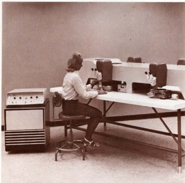
Fig. 16—Multiple laser-trim station uses the high-power output of a single YAG laser. The laser beam is split and fed to the various stations. Each operator can monitor and adjust the laser power to his workpiece. (HUGHES AIRCRAFT).
