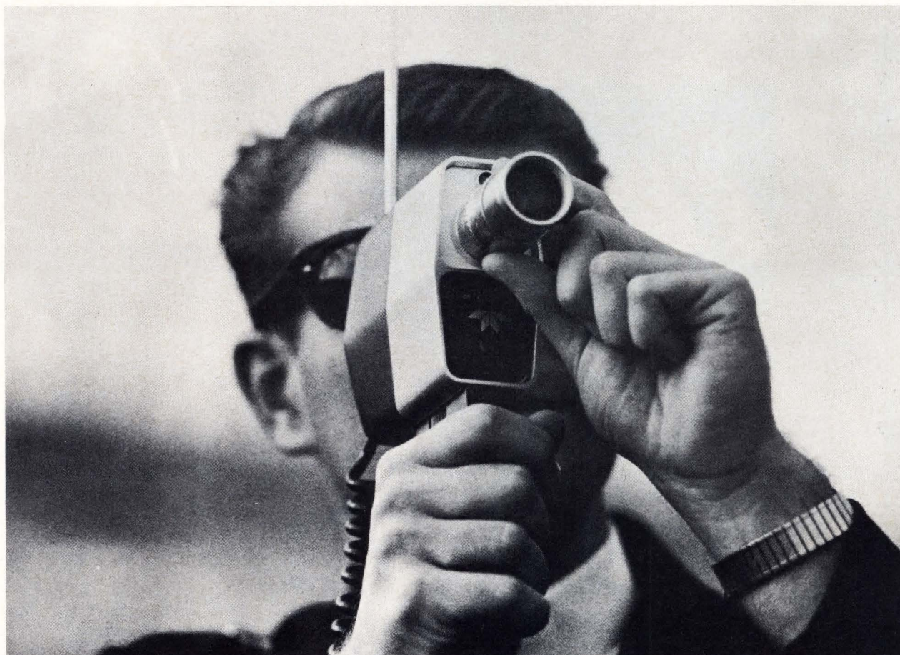
Fig. 1—Ultraminiature TV system is 3 by 4-1/2 by 1-1/2 inches and weighs about 1-1/2 lb without optics.
