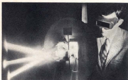
Multiple exposure shows the new laser. Beams were separated by rotating a prism in front of the laser.
