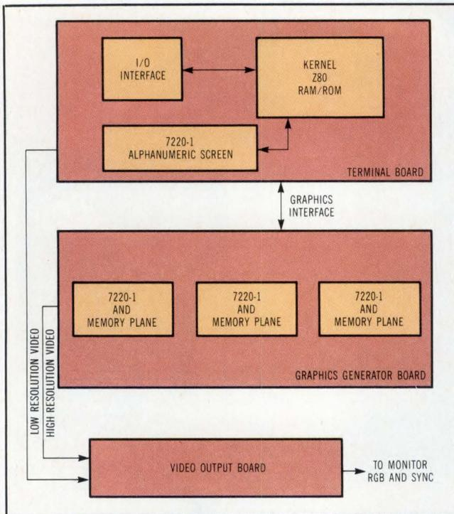
**Fig 3** A block diagram of the system shows the principal components—terminal board, graphics generator board, and video output board. The terminal board controls the system sending display commands to the graphics generator, and color map commands to the video output board.
