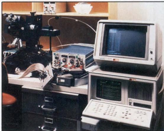
Engineers presently using VLSI design automation tools available on VAX computers can now test chip designs on the Tektronix DAS 9100 logic analysis system. The 91DVV VLSI verification software package from Tektronix creates a close relationship between the VAX host and logic analyzer. This combination imple-
