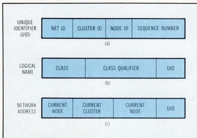
**Fig 3 Network operating system processes have specific name and address formats. The unique identifier (UID) in (a) is included in both the logical name (b), and the network address (c). It is 48-bits long, guaranteed to be unique, and is assigned at process creation time.**
