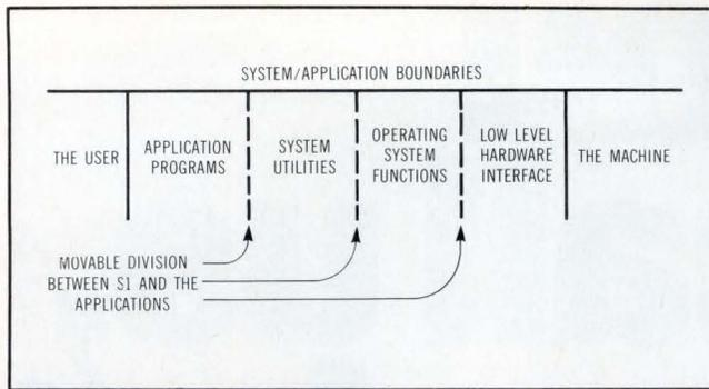
**Fig 1** With the S1 operating system, the division between the operating system and application programs is arbitrary. Modules implementing system functions can be linked into applications, and both utilities and applications can be included in the developer-tailored system.
