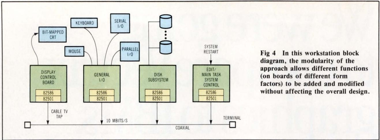
**Fig 4** In this workstation block diagram, the modularity of the approach allows different functions (on boards of different form factors) to be added and modified without affecting the overall design.
