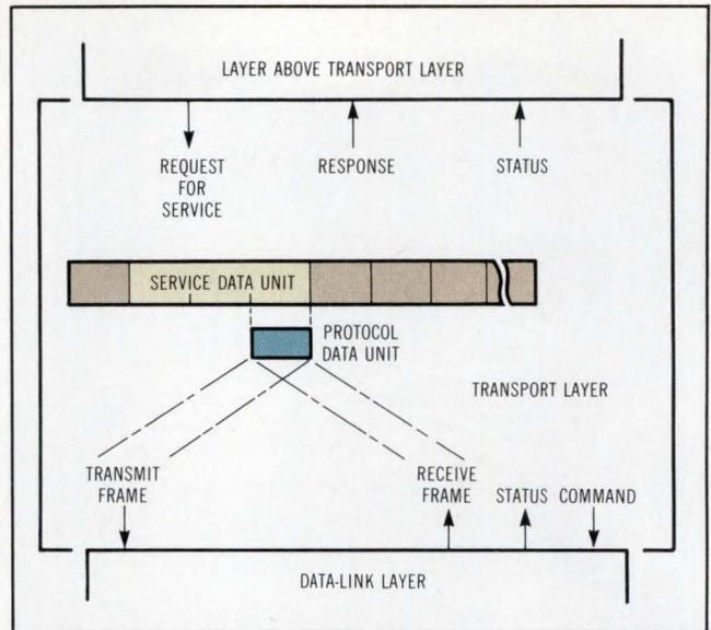
**Fig 3** Since the short-topology LAN does not use internetwork addressing, the data-link layer interfaces to the transport layer, with no network (layer 3) layer in between. The transport layer exchanges records or files with transport layers at other stations in the network.
