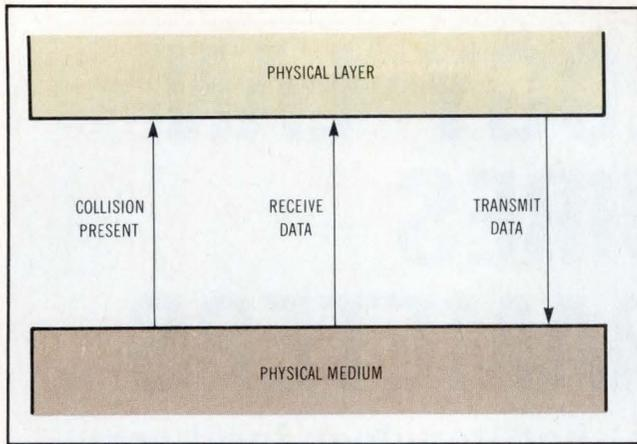
**Fig 1** At the lowest level of the Open System Interconnection (OSI) model—layer 1—the physical medium, usually a bus, interfaces to the physical layer. This interface is configured to accommodate the access method.
