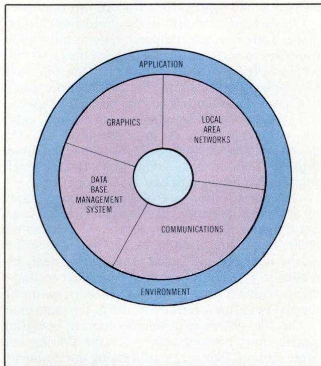
Fig 1 Digital Research's model of an operating system provides the services for state-of-the-art 16- and 32-bit microcomputer systems. It includes support for graphics, local networks, communications, and database management systems—all within an application environment.
