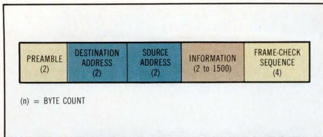
**Fig 5** The frame structure shown here represents the protocol by which data is passed between stations on the short-topology LAN. This structure is set by the transport layer when a station is first powered up.
