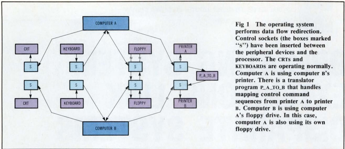
**Fig 1** The operating system performs data flow redirection. Control sockets (the boxes marked "s") have been inserted between the peripheral devices and the processor. The CRTs and KEYBOARDS are operating normally. Computer A is using computer B's printer. There is a translator program P.A.TO.B that handles mapping control command sequences from printer A to printer B. Computer B is using computer A's floppy drive. In this case, computer A is also using its own floppy drive.
