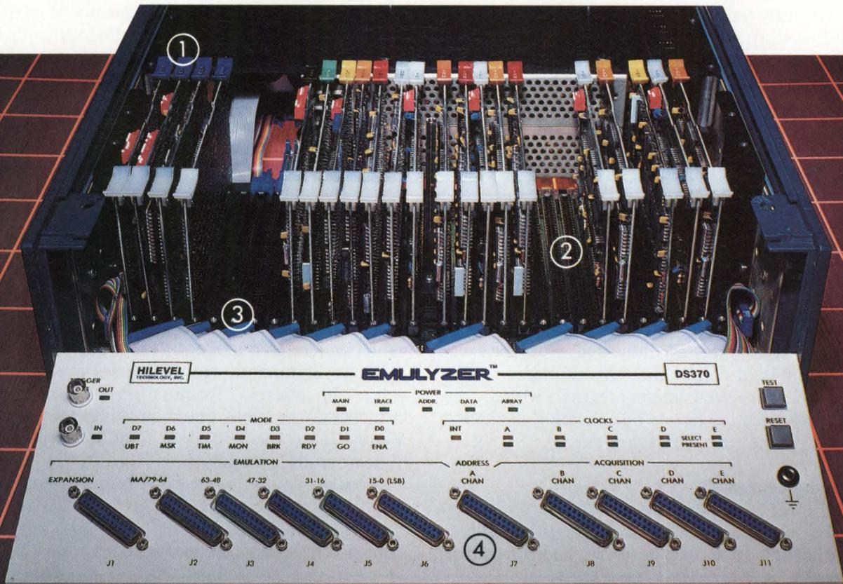
The raw power and flexibility required to tackle your bit-slice, microprogrammed, or other high performance processor-based designs head-on is in the DS370. No other system uses bit-slice architecture. This built-in power emerges in the versatile logic analyzer and integrated writable control store, graphic performance analysis, selective trace, symbolic debug, and 16 triggering levels.
