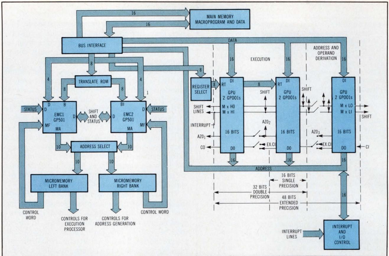
Fig 3 The control section of a 1750A computer uses two GP501 controllers in a synchronized fashion to address micromemory. Concatenated 8-bit ALU slices form the general processing section which comprises an execution part, and an address and operation generation part. Operations can be performed on 16-, 32-, and 48-bit wide data. A few LSI parts tie the whole system together.
