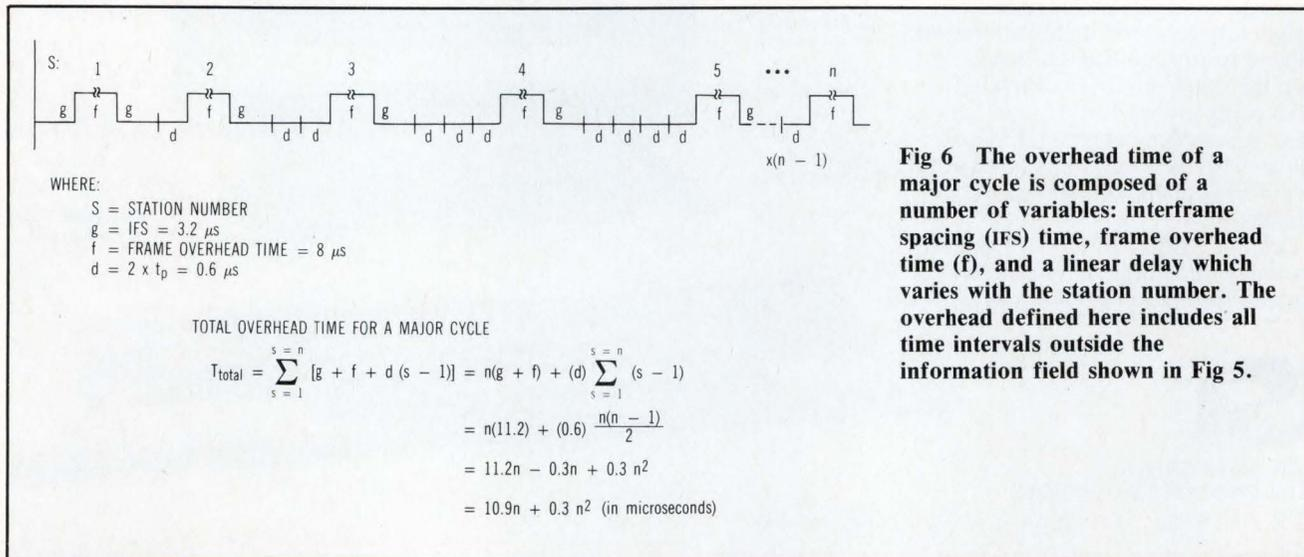
**Fig 6** The overhead time of a major cycle is composed of a number of variables: interframe spacing (IFS) time, frame overhead time (f), and a linear delay which varies with the station number. The overhead defined here includes all time intervals outside the information field shown in Fig 5.
