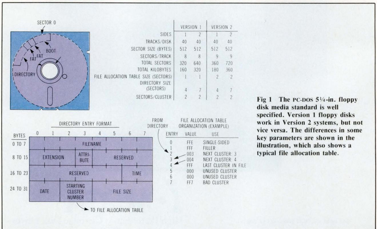
**Fig 1** The PC-DOS 5 1/4-in. floppy disk media standard is well specified. Version 1 floppy disks work in Version 2 systems, but not vice versa. The differences in some key parameters are shown in the illustration, which also shows a typical file allocation table.
