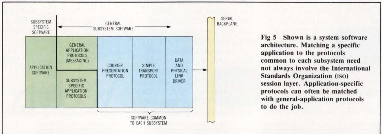
**Fig 5** Shown is a system software architecture. Matching a specific application to the protocols common to each subsystem need not always involve the International Standards Organization (ISO) session layer. Application-specific protocols can often be matched with general-application protocols to do the job.
