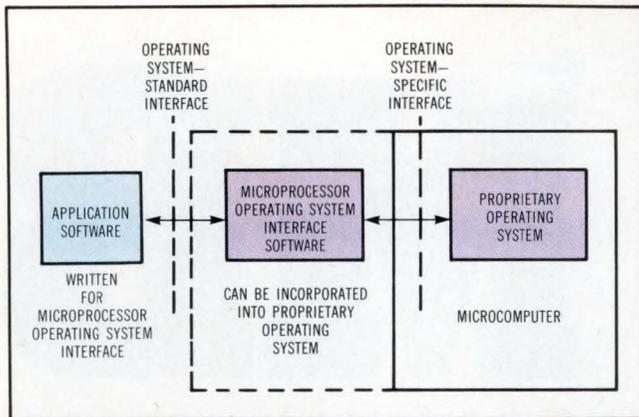
**The IEEE's Microprocessor Operating System Interface (MOSI) Task Group 855 is charged with devising a standard interface so that application programs can communicate with diverse operating systems. The interface will translate system calls and functions as shown.**
