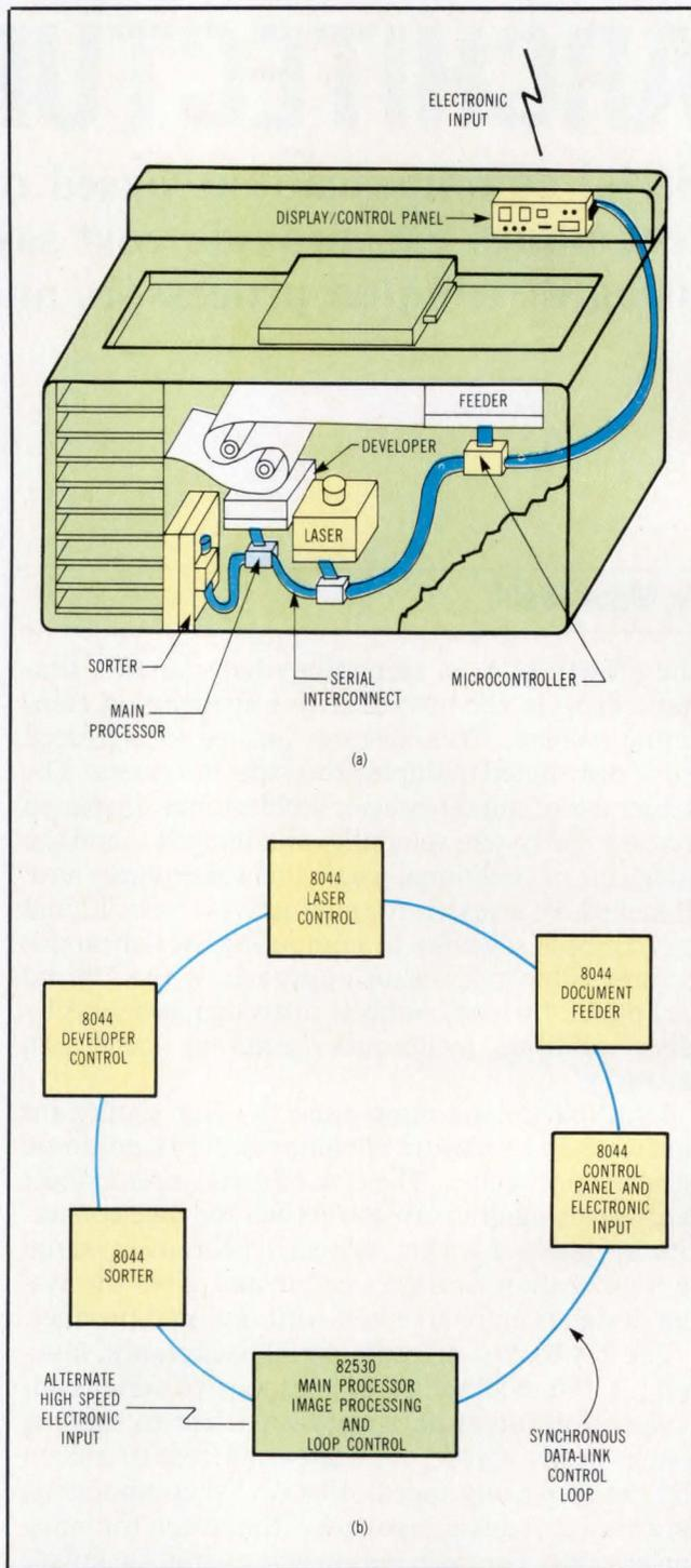
**Fig 1** Pictured is a copier architecture using the master/slave approach (a). The 82530 serial communication controller (SCC) controls use of the data channel (b). Traffic is generally low in volume, consisting mainly of commands and status exchanges.
