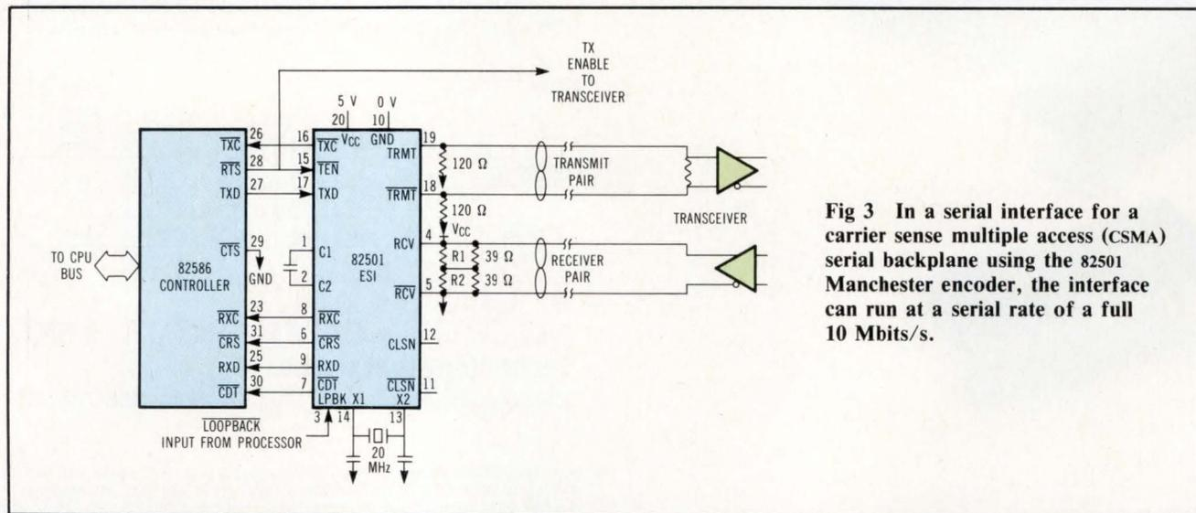
**Fig 3** In a serial interface for a carrier sense multiple access (CSMA) serial backplane using the 82501 Manchester encoder, the interface can run at a serial rate of a full 10 Mbits/s.
