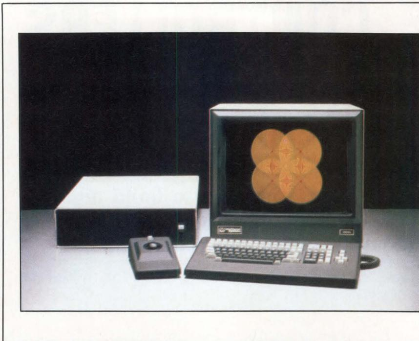
**Fig 1** The color graphics terminal incorporates four 7220-1 graphics chips for high speed processing. Design objectives include 1024 x 1024 dot-addressable resolution, smooth pan, and zoom.
