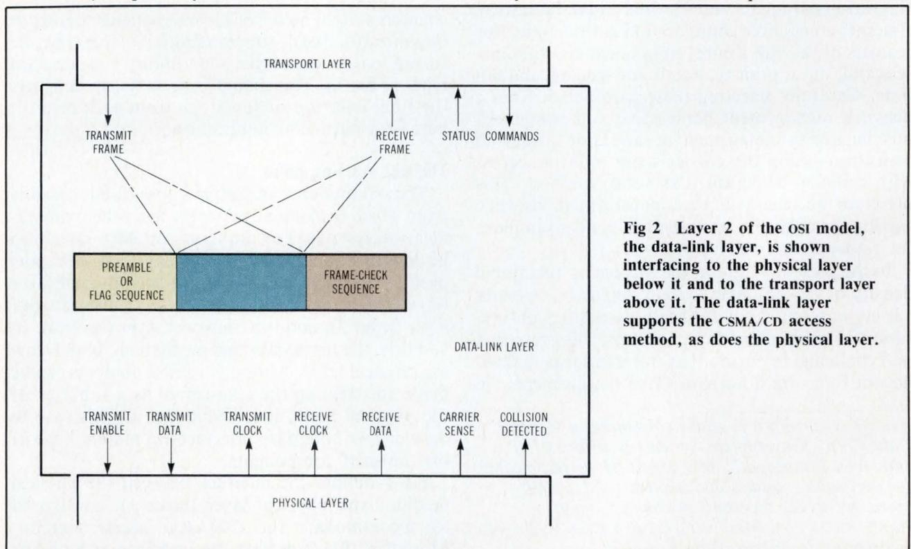
**Fig 2** Layer 2 of the OSI model, the data-link layer, is shown interfacing to the physical layer below it and to the transport layer above it. The data-link layer supports the CSMA/CD access method, as does the physical layer.
