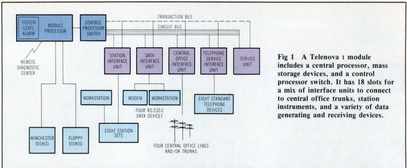
**Fig 1** A Telenova 1 module includes a central processor, mass storage devices, and a control processor switch. It has 18 slots for a mix of interface units to connect to central office trunks, station instruments, and a variety of data generating and receiving devices.
