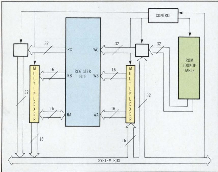
The register file has three read and three write ports. In each case, two of the three ports are 16-bit, and the third is 32-bit. Using these ports, the package can accommodate 16-, 32-, and 64-bit data from a number of host computer buses.
