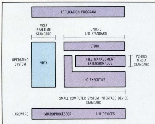
**Fig 2** A typical VRTX-based realtime operating system can have four modules that take care of a realtime tasking services interface, the STDIO I/O services interface, the PC-DOS media interface, and the Small Computer System Interface (SCSI) device interface. Other modules are under development.
