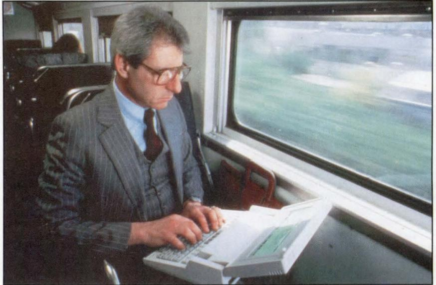
Weighing only 9 lb (4.08 kg) and measuring 13 x 10 x 3 in. (33 x 25 x 8 cm), the portable HP 110 is an ideal battery-powered personal computer for travelers. All-CMOS technology has made this possible.
