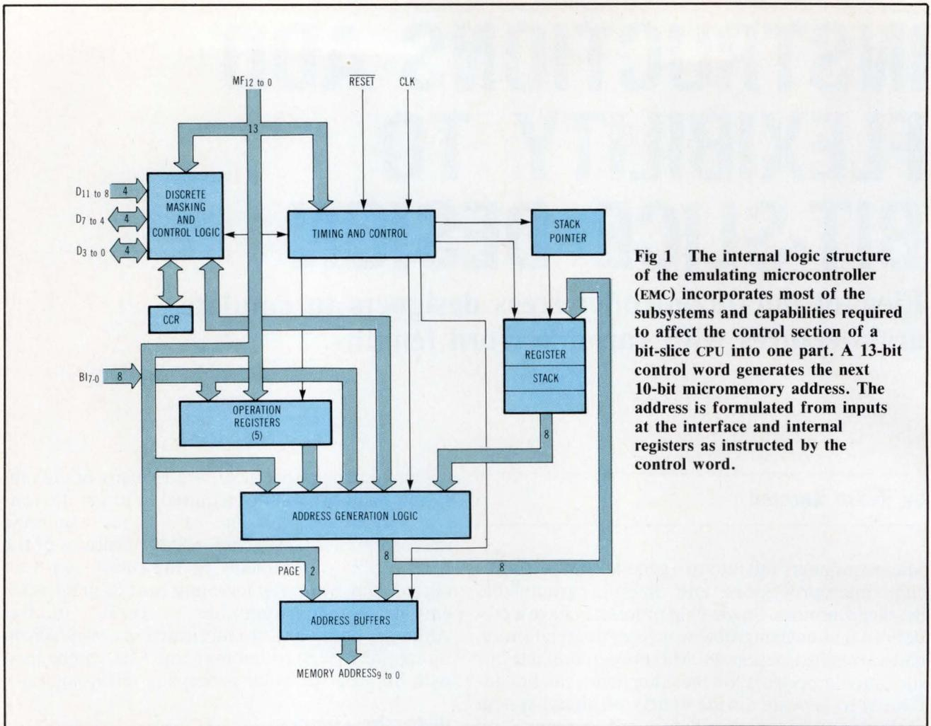
**Fig 1** The internal logic structure of the emulating microcontroller (EMC) incorporates most of the subsystems and capabilities required to affect the control section of a bit-slice CPU into one part. A 13-bit control word generates the next 10-bit micromemory address. The address is formulated from inputs at the interface and internal registers as instructed by the control word.
