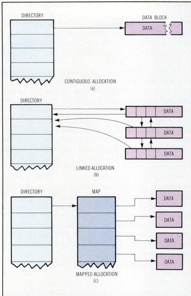
**Fig 3** The computer system designer may choose from three disk allocation methods with the operating system. Contiguous allocation (a), linked allocation (b), and mapped allocation (c) all have advantages and disadvantages that must be taken into account.
