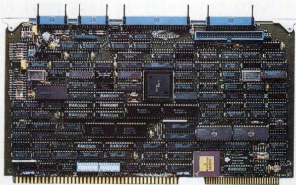
for the very first time on a controller, Storerger has an *on-board* 68000 CPU.
