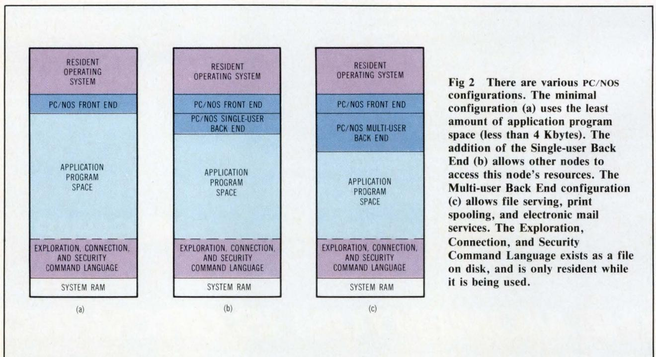
**Fig 2** There are various PC/NOS configurations. The minimal configuration (a) uses the least amount of application program space (less than 4 Kbytes). The addition of the Single-user Back End (b) allows other nodes to access this node's resources. The Multi-user Back End configuration (c) allows file serving, print spooling, and electronic mail services. The Exploration, Connection, and Security Command Language exists as a file on disk, and is only resident while it is being used.
