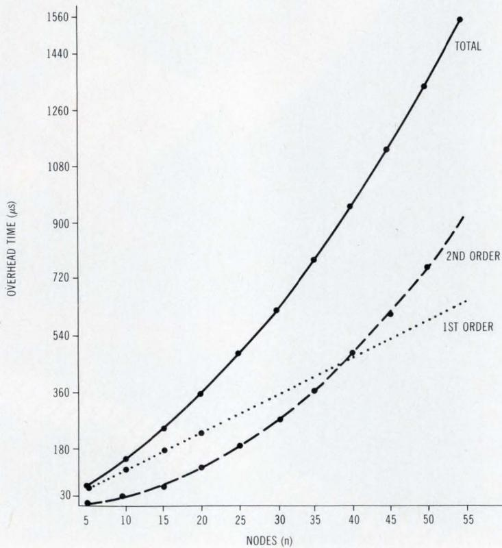
**Fig 7 Total overhead ( $T_{total}$ ) consists of a first- and second-order term. In a LAN with up to 40 nodes or stations, the first-order term is the larger contributor to overhead, but as more stations are added, the second-order term makes a greater contribution to the total overhead.**
