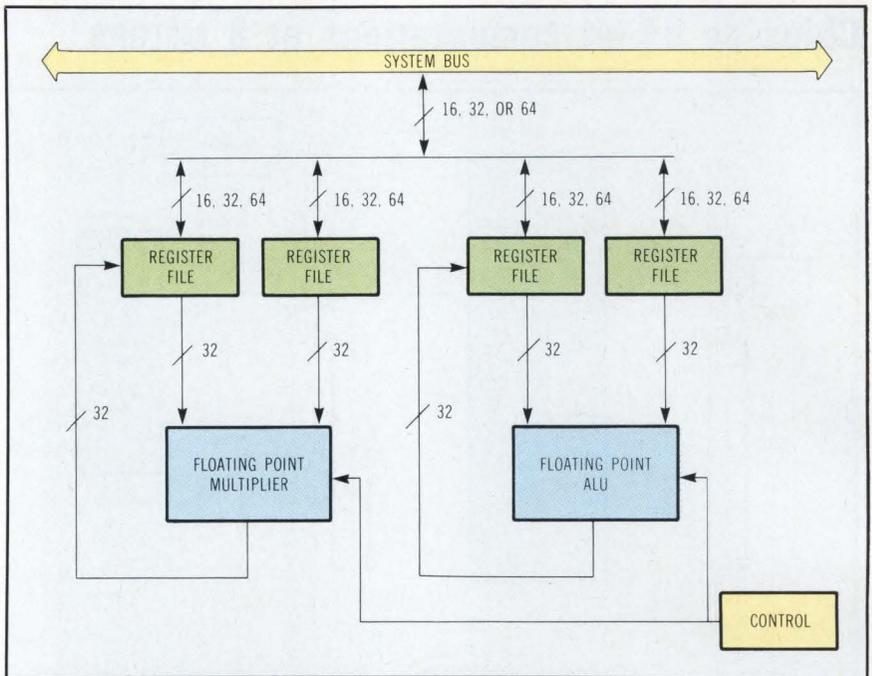
By using two register files in parallel with each floating point unit, the full speed of the 64-bit multiplier and the ALU can be used. Data can be down-loaded to the unit via DMA over the host bus, then used as needed by the math coprocessors.
