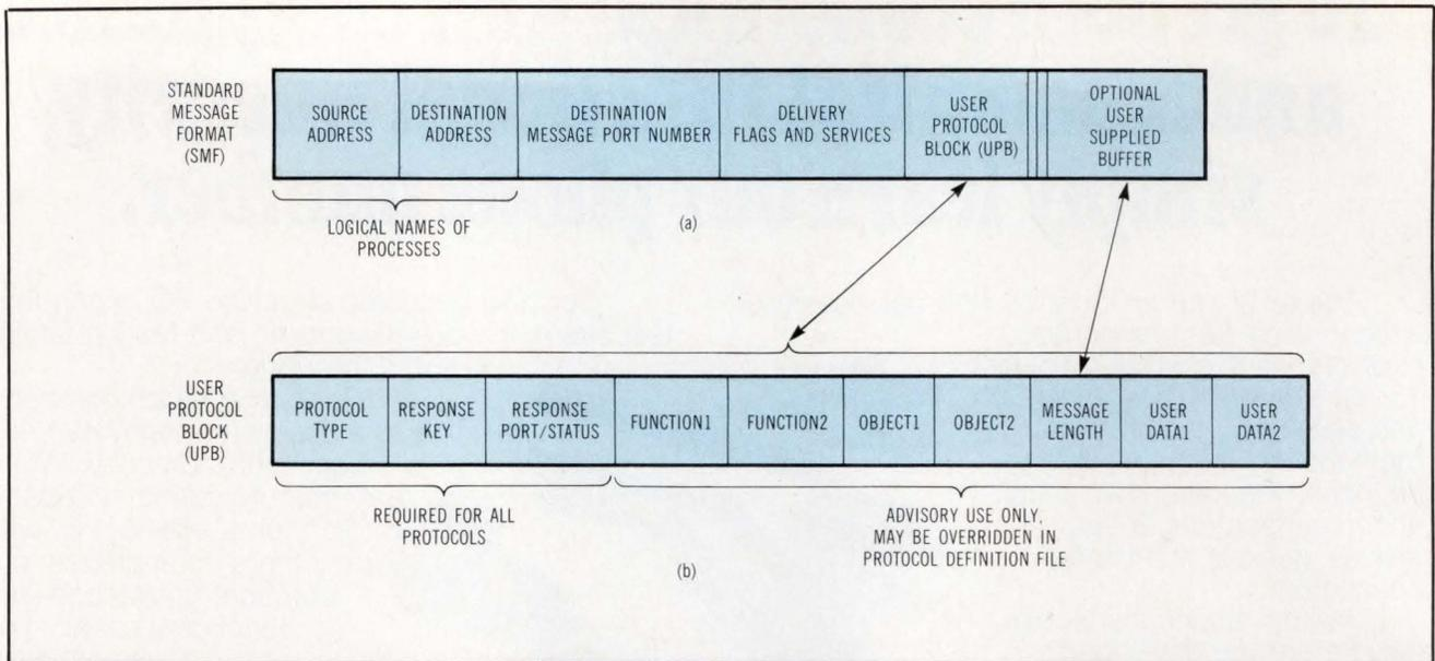
**Fig 4** The TNOS standard message format (SMF) in (a) includes the user protocol block (UPB) in (b). Part of the UPB is optional and may be suppressed by the particular protocol in use. Similarly, there is an optional user-supplied buffer in the standard message format.
