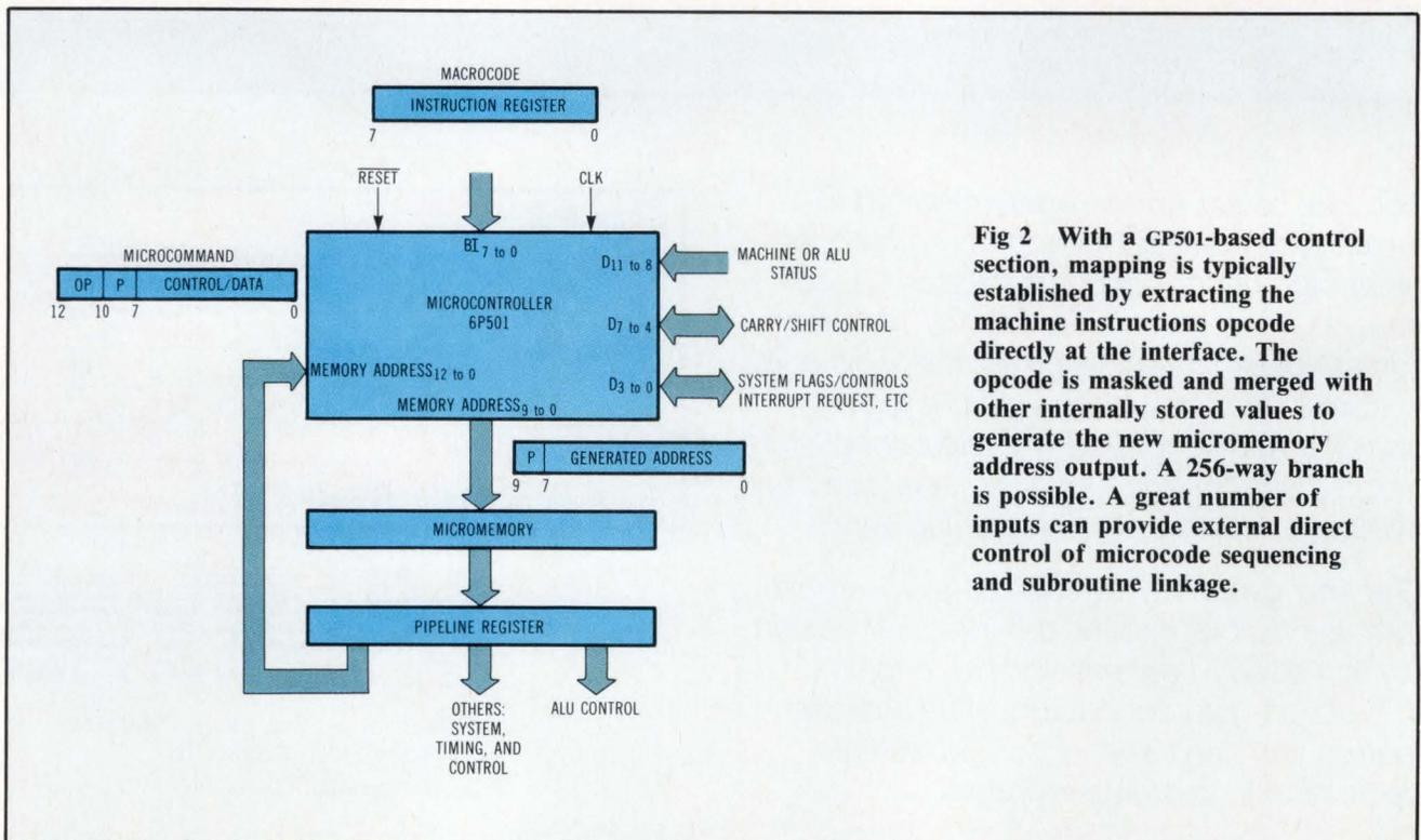
**Fig 2** With a GP501-based control section, mapping is typically established by extracting the machine instructions opcode directly at the interface. The opcode is masked and merged with other internally stored values to generate the new micromemory address output. A 256-way branch is possible. A great number of inputs can provide external direct control of microcode sequencing and subroutine linkage.
