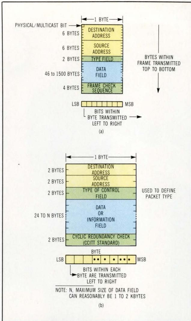
**Fig 2** In the realm of the serial backplane, certain changes in the Ethernet frame format (a) can be modified to improve performance. The backplane frame format (b) has been reduced by at least 10 bytes.
