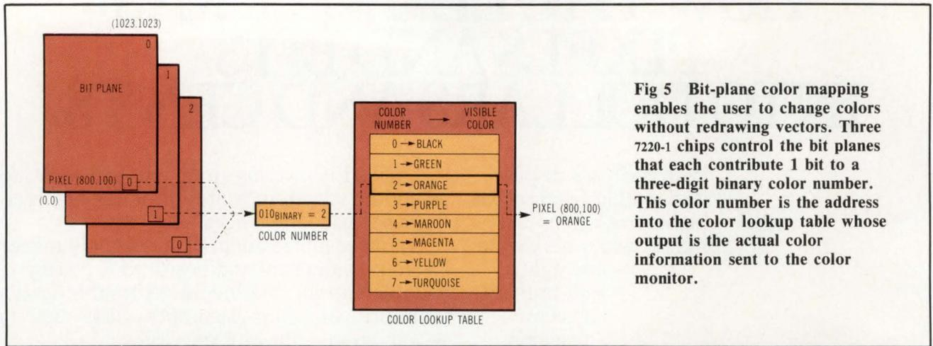
**Fig 5 Bit-plane color mapping enables the user to change colors without redrawing vectors. Three 7220-1 chips control the bit planes that each contribute 1 bit to a three-digit binary color number. This color number is the address into the color lookup table whose output is the actual color information sent to the color monitor.**
