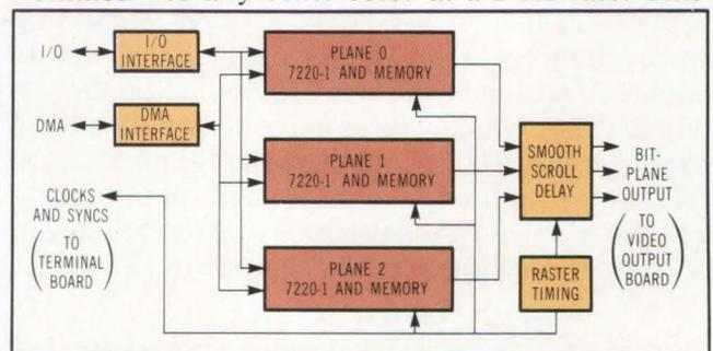
**Fig 2** The graphics generator board has three 7220-1 chips, each controlling a separate bit plane. Parallel outputs feed into the smooth scroll taped delay line and then to the video output board.
