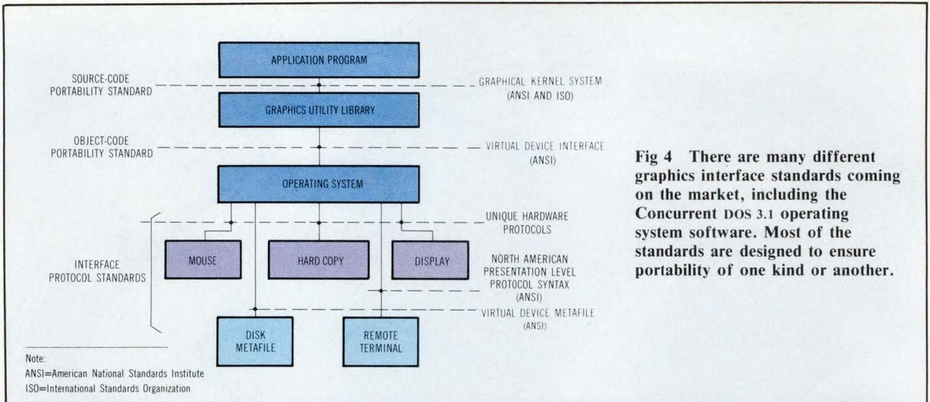
**Fig 4** There are many different graphics interface standards coming on the market, including the Concurrent DOS 3.1 operating system software. Most of the standards are designed to ensure portability of one kind or another.
