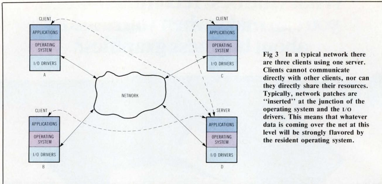
**Fig 3** In a typical network there are three clients using one server. Clients cannot communicate directly with other clients, nor can they directly share their resources. Typically, network patches are "inserted" at the junction of the operating system and the I/O drivers. This means that whatever data is coming over the net at this level will be strongly flavored by the resident operating system.
