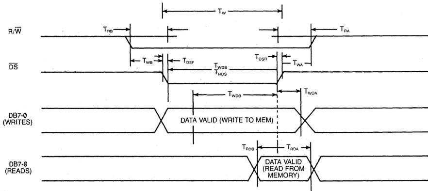
FIGURE 4: UDC TO MEMORY TIMING (BUS MASTER)
