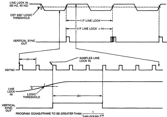
Note: To ensure a stable display when using the line lock mode, the CRT 5057 should be used with DC coupled monitors only.
