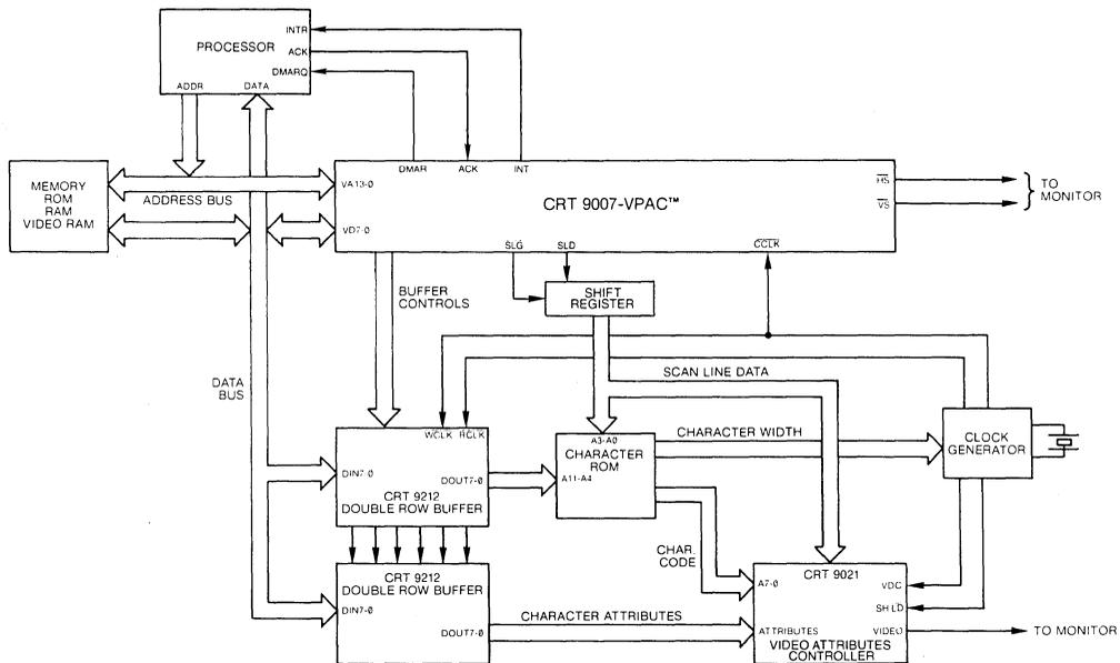
FIGURE 10: CRT 9007 CONFIGURATION FOR PROPORTIONAL CHARACTER DISPLAY
