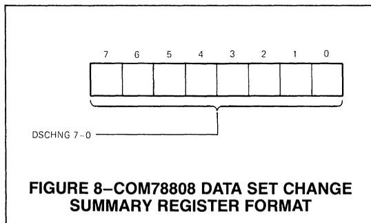
then be obtained from that line's status register. If the state of a line changes twice within one microsecond, the change in state may not be detected. Figure 8 shows the format of the data set change summary register.
