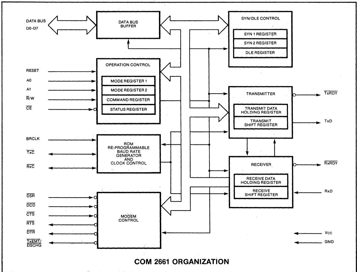
The COM 2661 is organized into 6 major sections. Communication between each section is achieved via an internal data and control bus. The data bus buffer allows a processor access to all internal registers on the COM 2661. The differences between the COM 2661 and COM 2651 are outlined in table 1.
