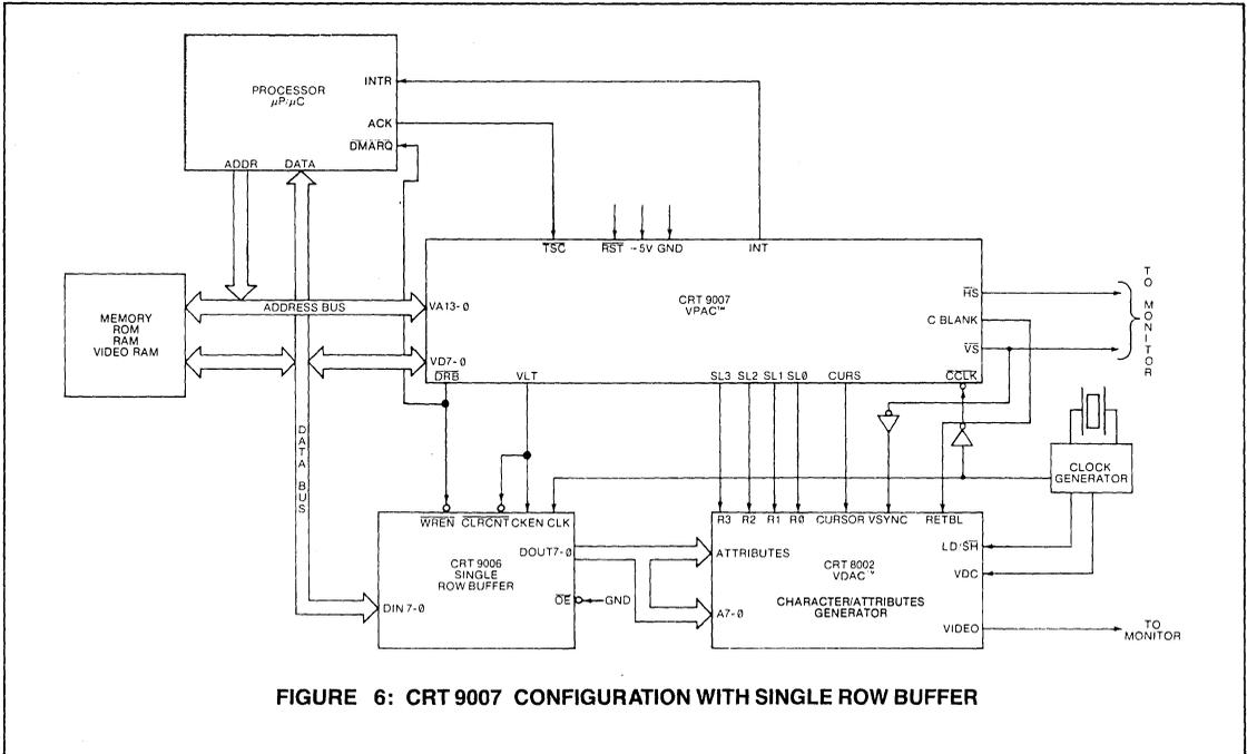
**FIGURE 6: CRT 9007 CONFIGURATION WITH SINGLE ROW BUFFER**
