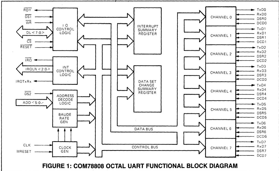
**FIGURE 1: COM78808 OCTAL UART FUNCTIONAL BLOCK DIAGRAM**
