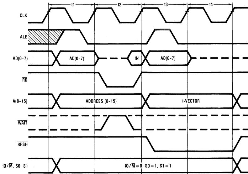
FIGURE 2a. Opcode Fetch Cycles without  $\overline{\text{WAIT}}$  States
