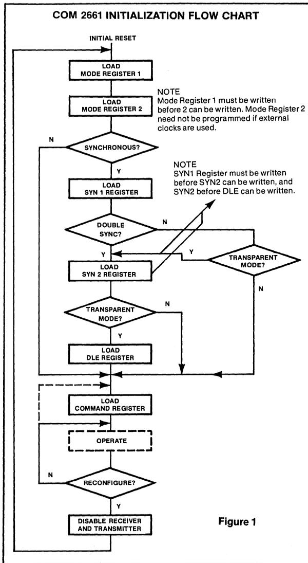
than the required number of accesses are made, the internal sequencer recycles to point at the first register. The pointers are reset to SYN1 Register and Mode Register 1 by a RESET input or by performing a "Read Command Register" operation, but are unaffected by any other read or write operation.
