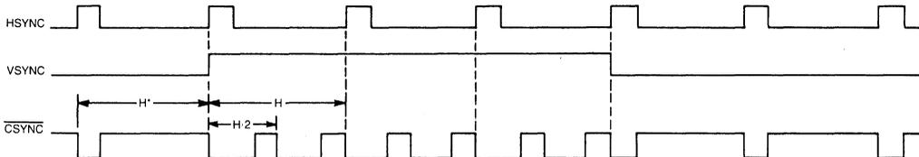
NOTE: Delays between pulse edges and pulse width values may vary due to mask programmable features.
