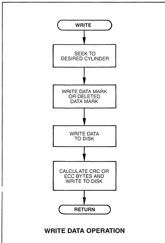
Before writing data to the selected disk drive, the UDC will read the current ID field, step to the desired cylinder and verify that it has located the correct cylinder and sector. (These steps were described previously under "UDC Command Overview").
