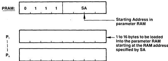
From the starting address, SA, any number of bytes may be loaded into the parameter RAM at incrementing addresses, up to location 15. The sequence of parameter bytes is terminated by the next command byte entered into the FIFO. The parameter RAM stores 16 bytes of information in predefined locations which differ for graphics and character modes. See the parameter RAM discussion for bit assignments.
