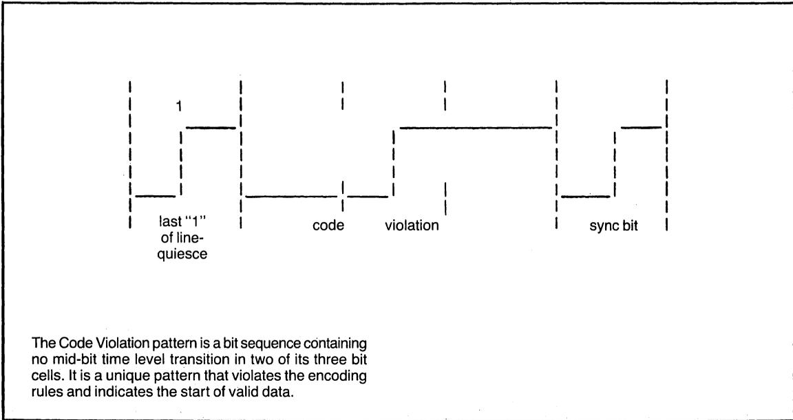
The Code Violation pattern is a bit sequence containing no mid-bit time level transition in two of its three bit cells. It is a unique pattern that violates the encoding rules and indicates the start of valid data.
