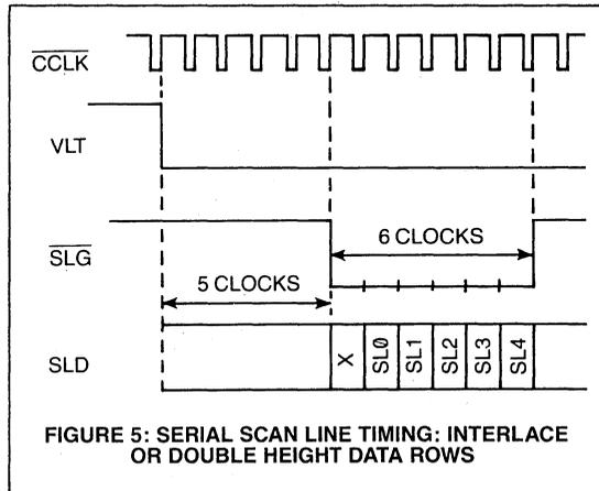
**FIGURE 5: SERIAL SCAN LINE TIMING: INTERLACE OR DOUBLE HEIGHT DATA ROWS**
