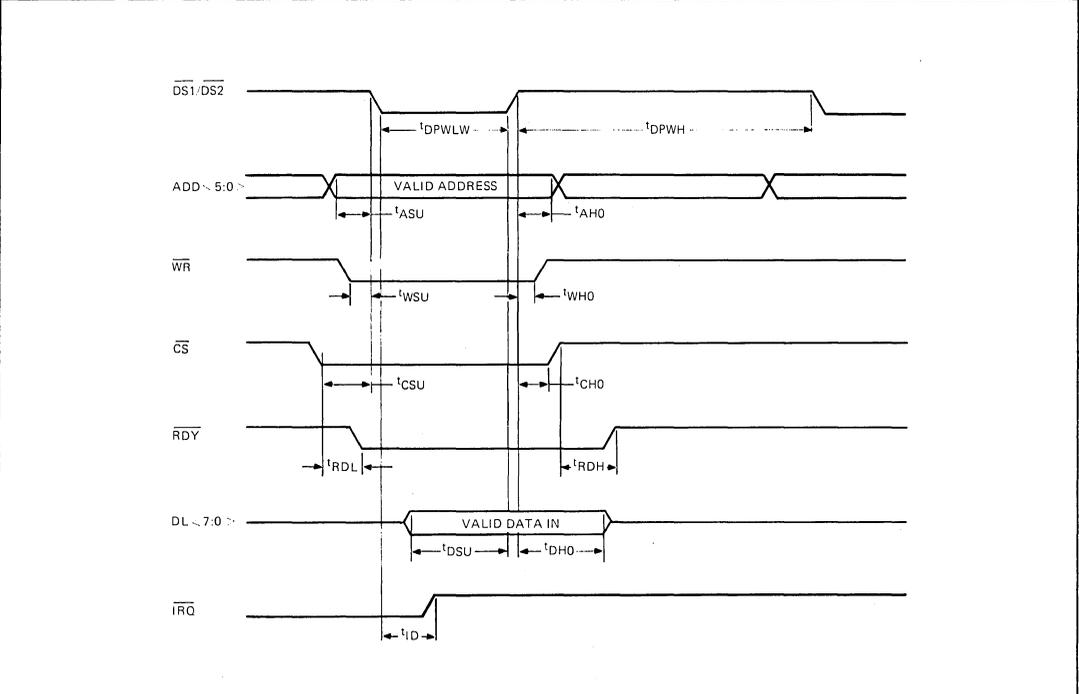
FIGURE 11—COM78808 BUS WRITE CYCLE TIMING
