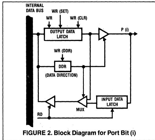
**FIGURE 2. Block Diagram for Port Bit (i)**
