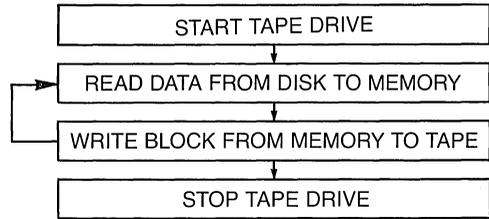
Control of a streaming tape drive is similar to that of a start/stop drive. The tape is started at the beginning of the data transfer and stopped after the last block is written to the tape. The tape is not stopped in between blocks. The UDC will however turn the Write Gate signal on when it is writing data and off when it is not so that gaps will be written (with external hardware) on the tape between the data blocks.
