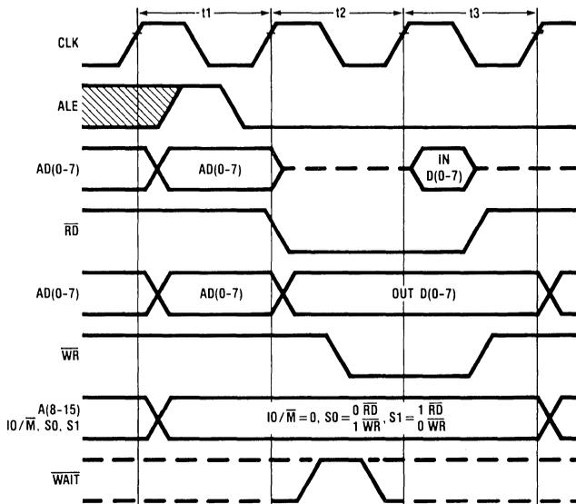
FIGURE 3a. Memory Read/Write Cycles without WAIT States
