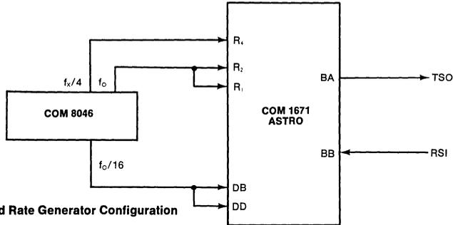
Typical ASTRO-Baud Rate Generator Configuration
