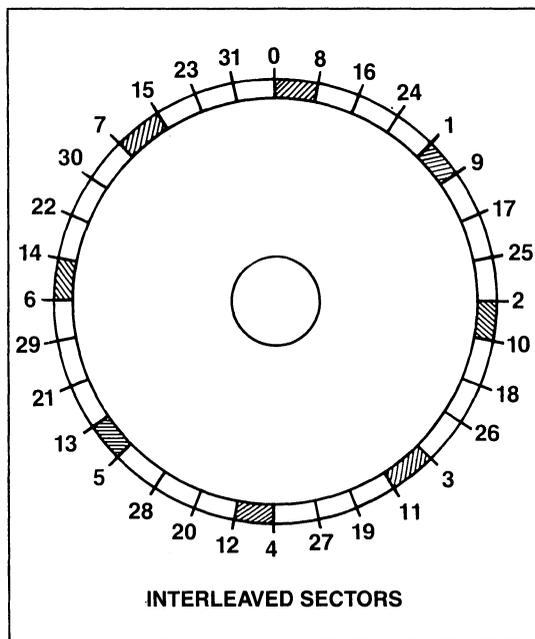
The UDC can format a track with interleaved sectors by staggering the sector numbers. For example, to format a 32 sector track, with a sector interleave factor of 4, the system processor would set up the ID Field table sector numbers as follows:
