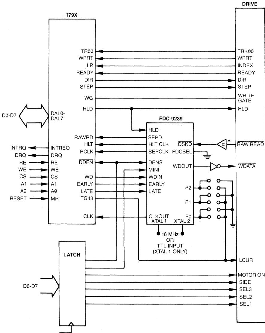
\*The FDC9239/B, as all other CMOS integrated circuits, presents a high impedance on all inputs.
