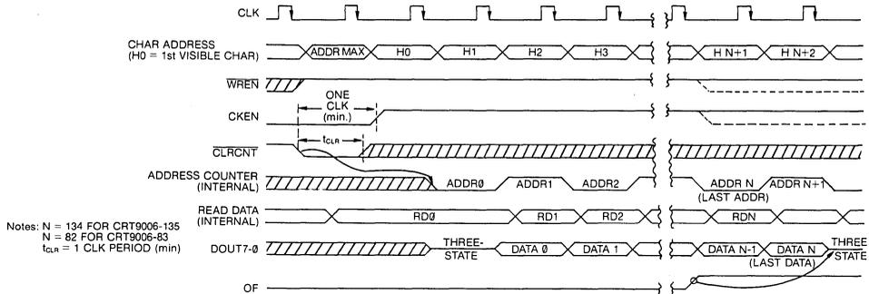
**FIGURE 3: SINGLE ROW BUFFER WRITE TIMING**
