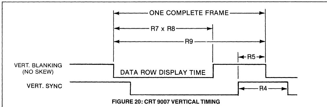
FIGURE 20: CRT 9007 VERTICAL TIMING
