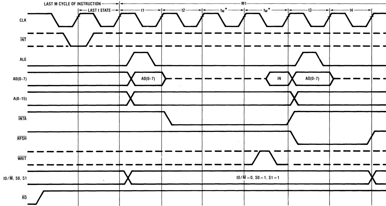
\* $t_w$  is the CPU generated WAIT state in response to an interrupt request.
