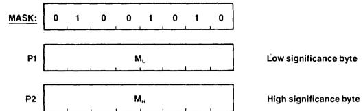
This command sets the value of the 16-bit Mask register of the figure drawing processor. The Mask register controls which bits can be modified in the display memory during a read-modify-write cycle.
