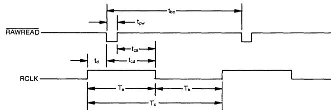
Note: Pulse width on RAW READ (Pin 27) is normally 10-300 ns. However, pulse may be any width if pulse is entirely within window. If pulse occurs in both windows, then pulse width must be less than 300 ns for MFM at CLK = 2 MHz and 600 ns for FM at 2 MHz. Times double for 1 MHz.
