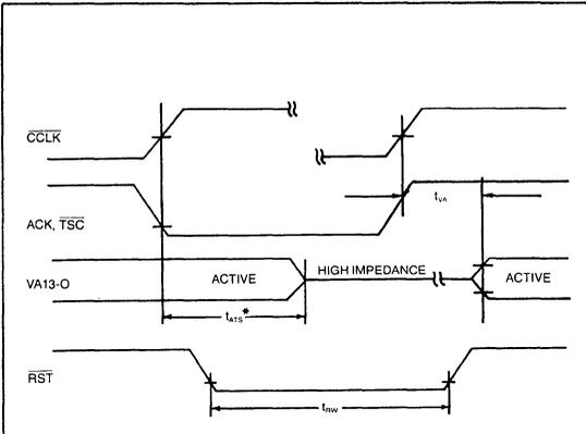
\* t\_A13 is controlled directly from ACK or TSC or from the particular CCLK that ends a DMA burst cycle.
