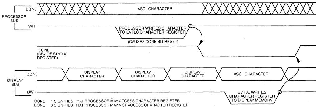
**FIGURE 6. TYPICAL PROCESSOR TO DISPLAY MEMORY TRANSFER**
