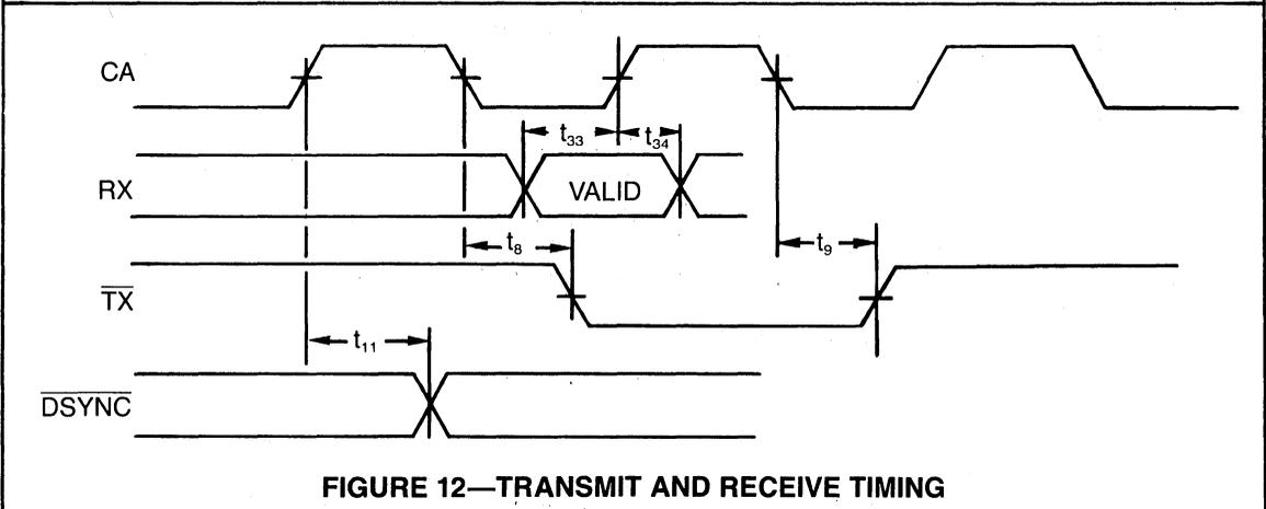
**FIGURE 12—TRANSMIT AND RECEIVE TIMING**
