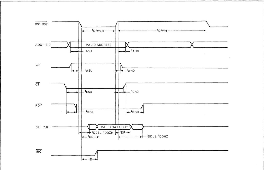
FIGURE 10—COM78808 BUS READ CYCLE TIMING
