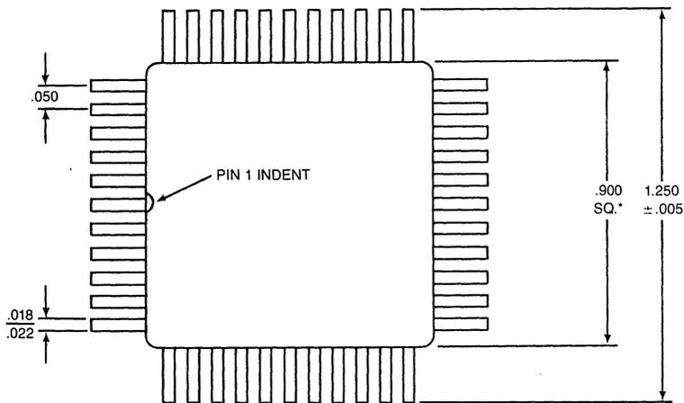
\*DEFINES MINIMUM CLEAR LEADFRAME ZONE -zone consists of package body, including ceramic and glass.
