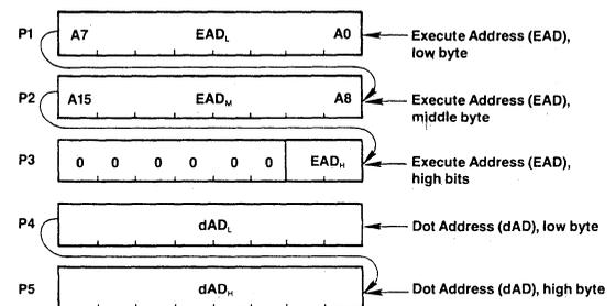
The Execute Address, EAD, points to the display memory word containing the pixel to be addressed.
