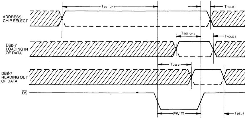
FIGURE 3 SCAN AND DATA ROW COUNTER TIMING
