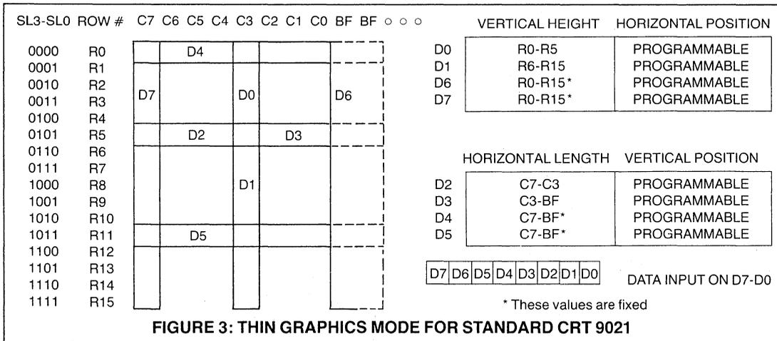
**FIGURE 3: THIN GRAPHICS MODE FOR STANDARD CRT 9021**
