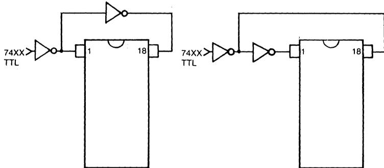
74XX—totem pole or open collector output (external pull-up resistor required)
