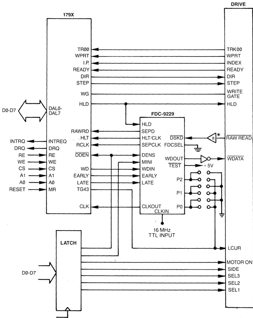
\*The FDC9229/B, as all other NMOS integrated circuits, presents a high impedance on all inputs.
