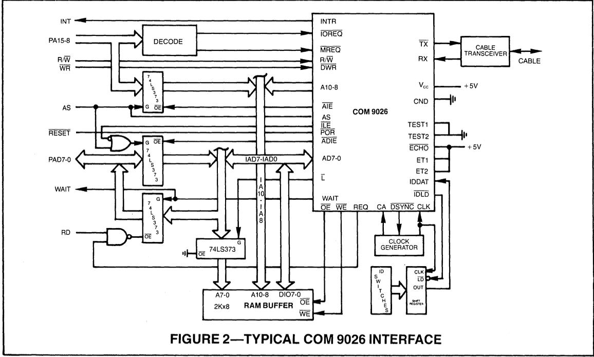
**FIGURE 2—TYPICAL COM 9026 INTERFACE**
