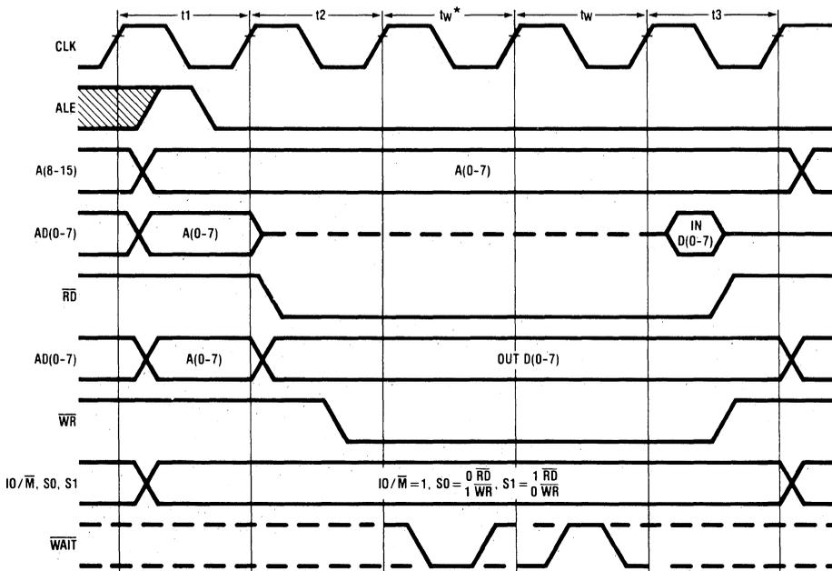
\*  $\overline{\text{WAIT}}$  state automatically inserted during IO operation.
