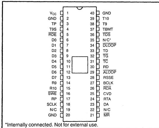
\*Internally connected. Not for external use.
