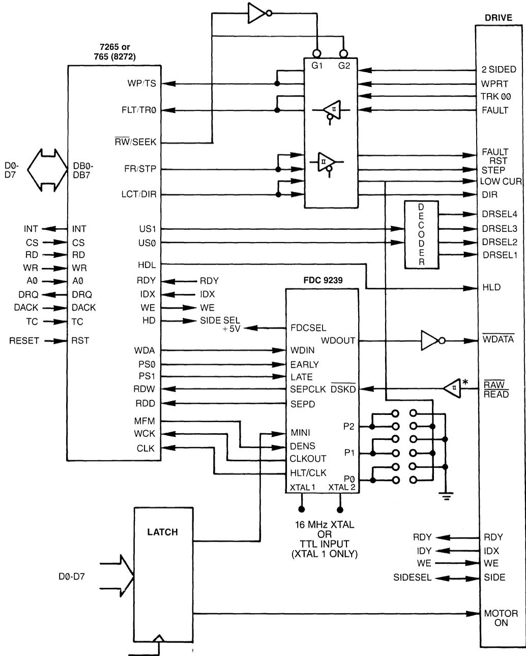
\*The FDC9239/B, as all other NMOS integrated circuits, presents a high impedance on all inputs.
