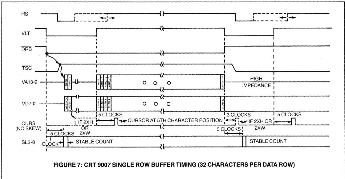
**FIGURE 7: CRT 9007 SINGLE ROW BUFFER TIMING (32 CHARACTERS PER DATA ROW)**
