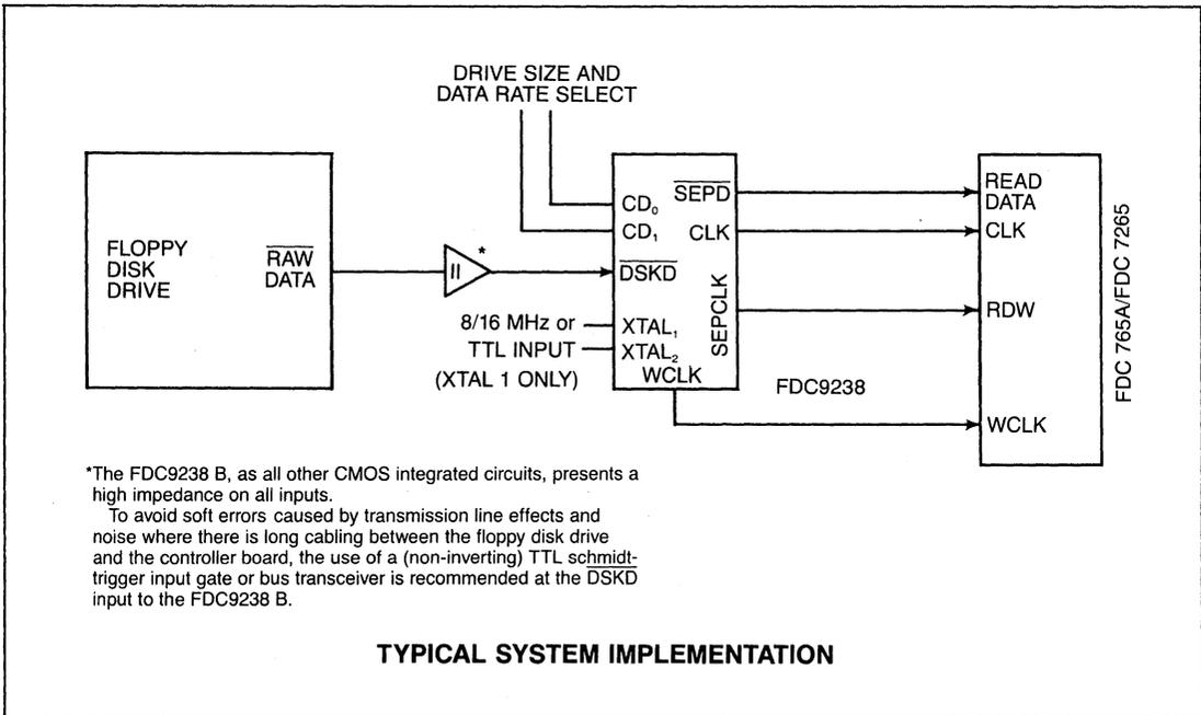
\*The FDC9238 B, as all other CMOS integrated circuits, presents a high impedance on all inputs.
