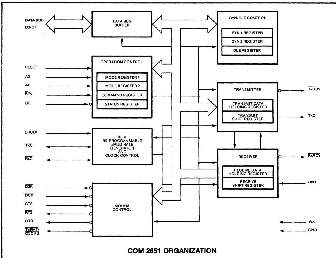
The COM 2651 is organized into 6 major sections. Communication between each section is achieved via an internal data and control bus. The data bus buffer allows a processor access to all internal registers on the COM 2651.
