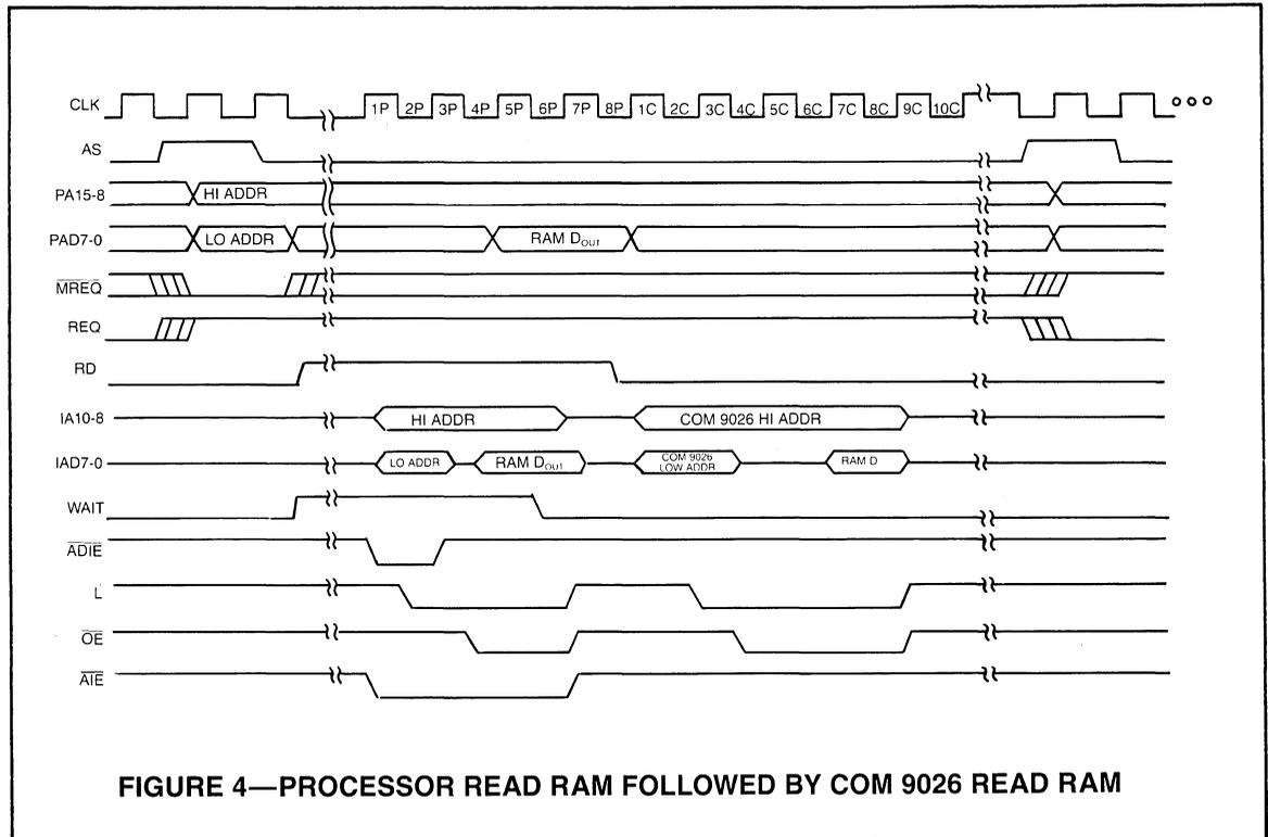
FIGURE 4—PROCESSOR READ RAM FOLLOWED BY COM 9026 READ RAM
