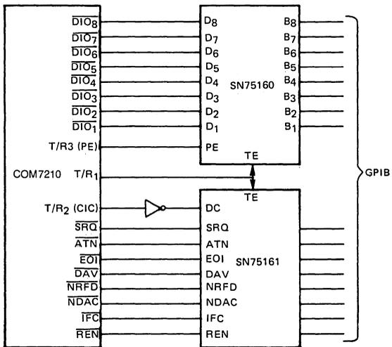
**Note:** In the case of low-speed data transfer (B<sub>2</sub> = 0), the T/R<sub>3</sub> pin can be used as a TRIG output. The PE input of SN75160 should be cleared to "0."
