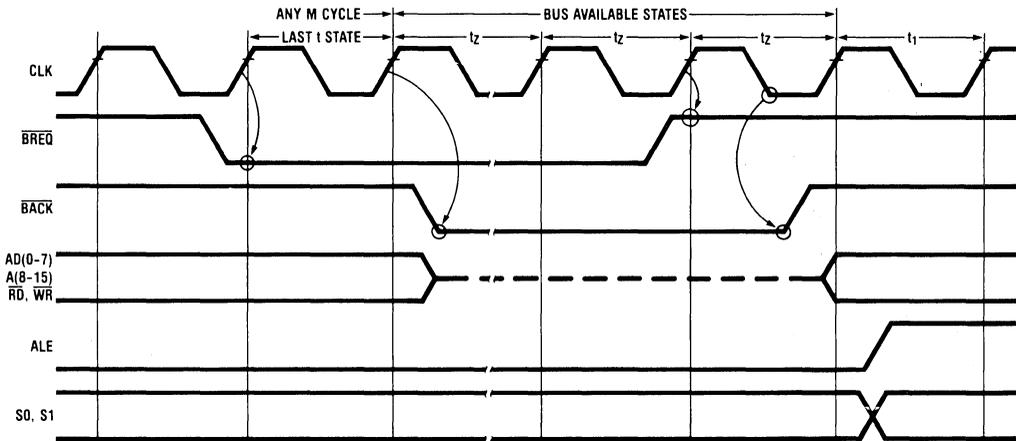
\* S0, S1 during **BREQ** will indicate same machine cycle as during cycle when **BREQ** was accepted.
