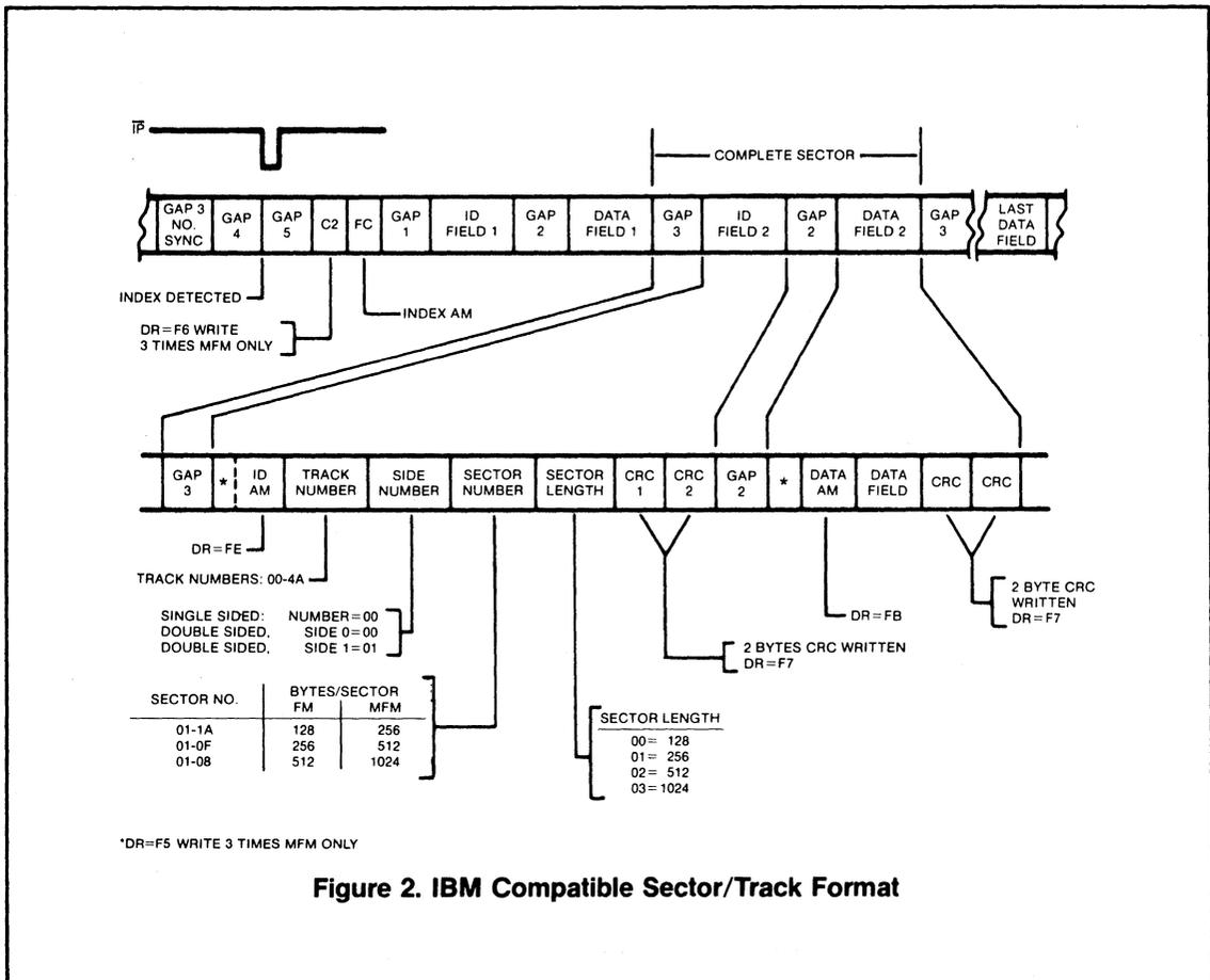
Figure 2. IBM Compatible Sector/Track Format
