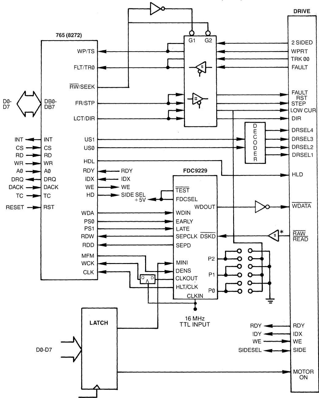
\*The FDC9229/B, as all other NMOS integrated circuits, presents a high impedance on all inputs.
