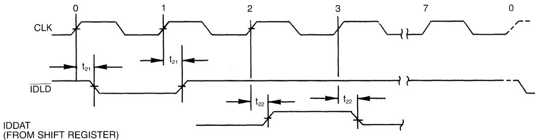
**FIGURE 19—ID INPUT AC TIMING**
