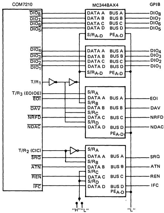
**Note:** In this example, high-speed data transfer cannot be made since the bus transceiver is of the open collector type (Set B<sub>2</sub> = 0).
