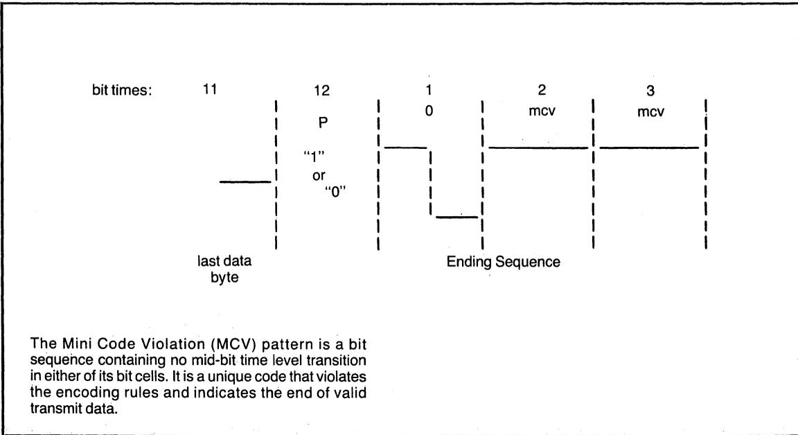
The Mini Code Violation (MCV) pattern is a bit sequence containing no mid-bit time level transition in either of its bit cells. It is a unique code that violates the encoding rules and indicates the end of valid transmit data.
