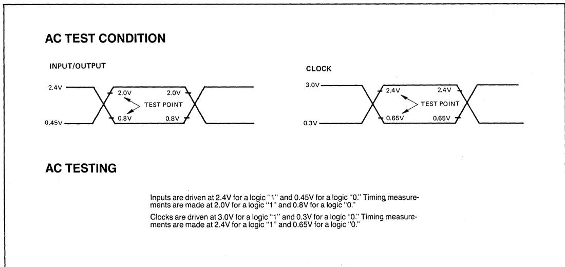
AC CHARACTERISTICS  $T_a = -10^{\circ}\text{C}$  to  $+70^{\circ}\text{C}$ ;  $V_{CC} = +5\text{V} \pm 5\%$  unless otherwise specified.
