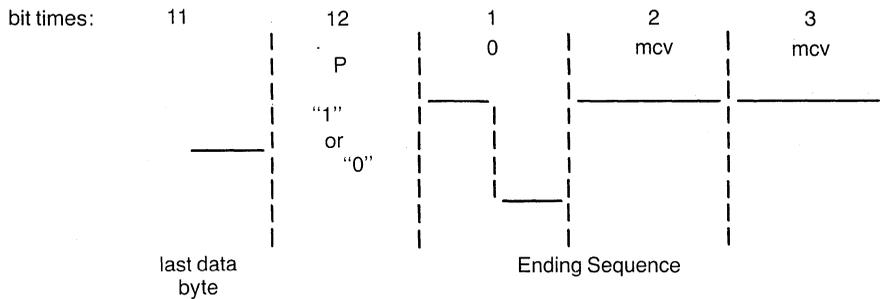
The Mini Code Violation (MCV) pattern is a bit sequence containing no mid-bit time level transition in either of its bit cells. It is a unique code that violates the encoding rules and indicates the end of valid transmit data.
