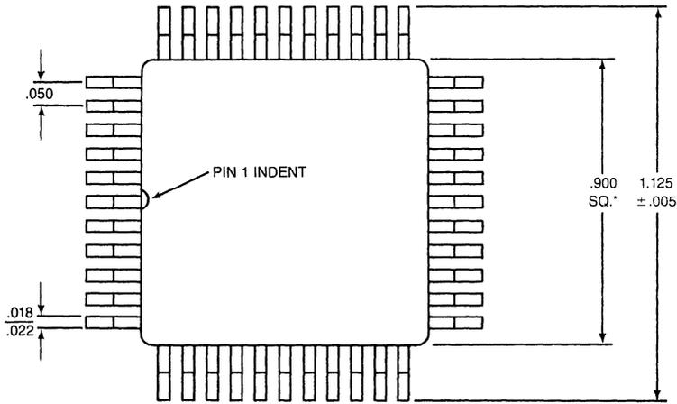
\*DEFINES MINIMUM CLEAR LEADFRAME ZONE -zone consists of package body, including ceramic and glass.
