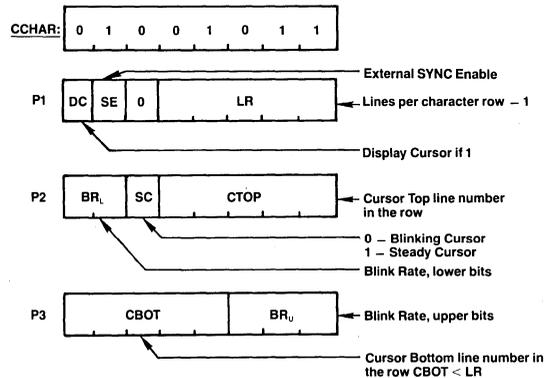
In graphics mode, LR should be set to 0. The blink rate parameter controls both the cursor and attribute blink rates. The cursor blink-on time = blink-off time = 2 x BR (video frames). The attribute blink rate is always 1/2 the cursor rate but with a 3/4 on -1/4 off duty cycle. All three parameter bytes must be output for interlace displays, regardless of mode. For interlace displays in graphics mode, the parameter BR<sub>L</sub> = 3.
