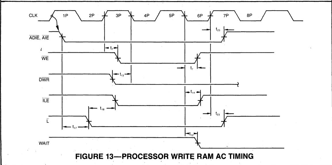
**FIGURE 13—PROCESSOR WRITE RAM AC TIMING**
