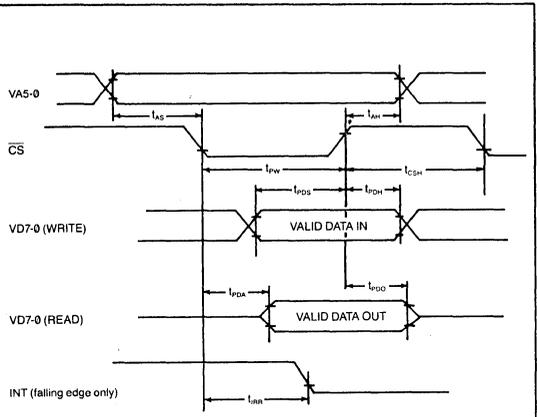
FIGURE 2: CRT 9007 PROCESSOR READ AND WRITE TIMING PARAMETERS
