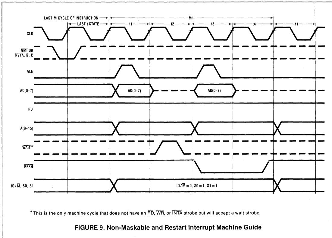
FIGURE 9. Non-Maskable and Restart Interrupt Machine Guide
