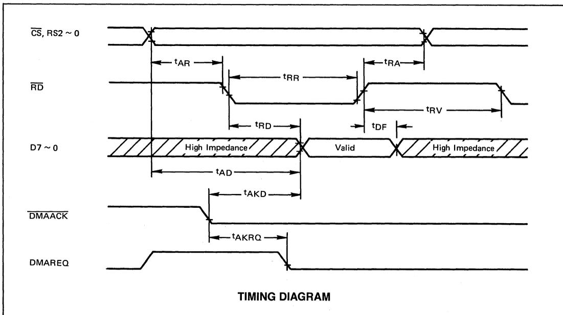
**AC CHARACTERISTICS, ( $T_a = 0$  to  $70^\circ\text{C}$ ,  $V_{CC} = 5V \pm 10\%$ )**
