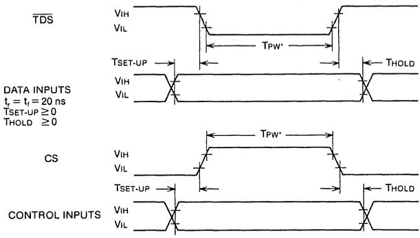
\*Input information (Data/Control) need only be valid during the last  $T_{pw}$ , min time of the input strobes (TDS, CS).
