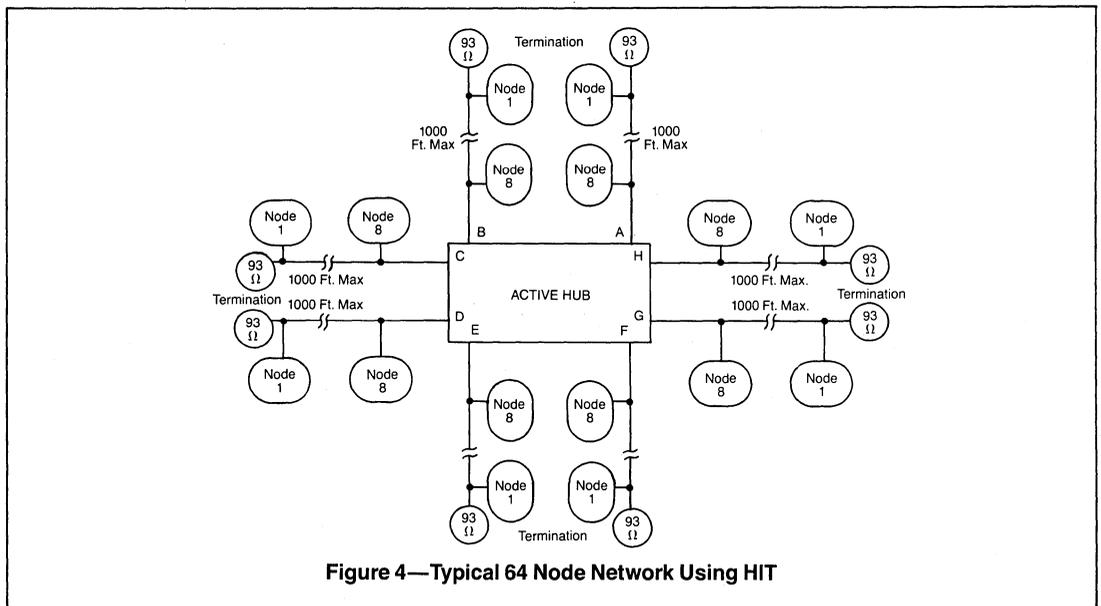
Figure 4—Typical 64 Node Network Using HIT
