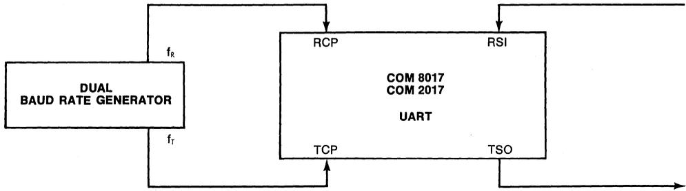
Typical UART-Dual Baud Rate Generator Configuration
