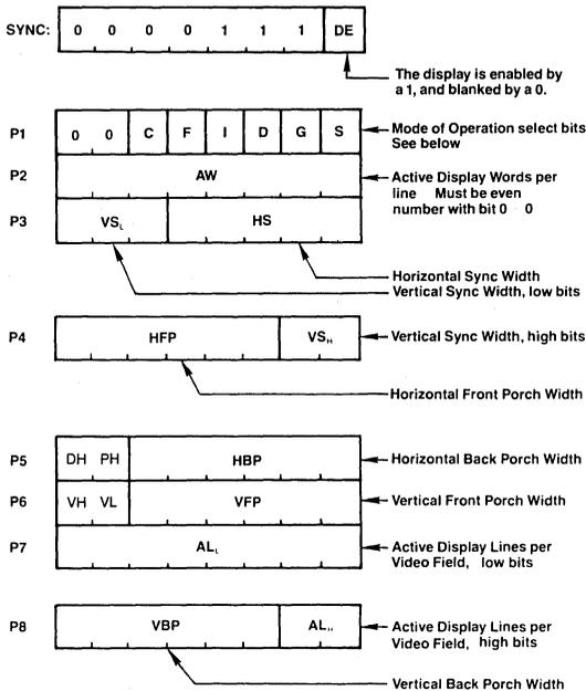
This command also loads parameters into the sync generator. The various parameter fields and bits are identical to those at the RESET command. The HGDC is not reset nor does it enter idle mode.
