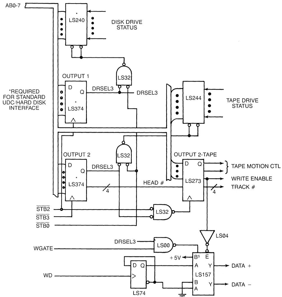
**SCHEMATIC 2: UDC/TAPE DRIVE INTERFACE CIRCUIT**
