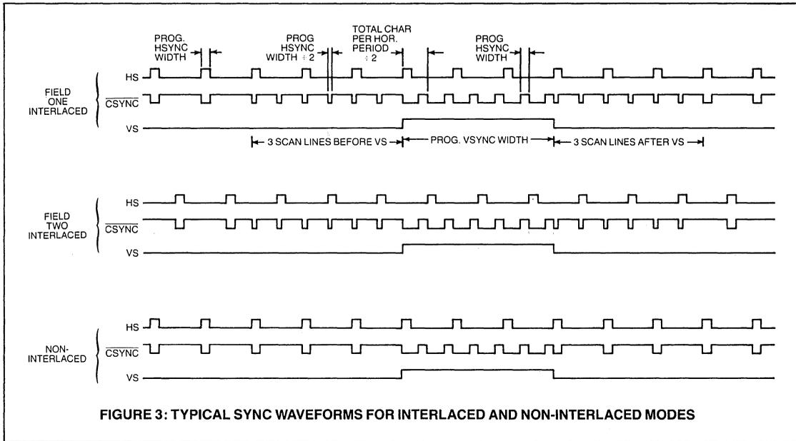
**FIGURE 3: TYPICAL SYNC WAVEFORMS FOR INTERLACED AND NON-INTERLACED MODES**
