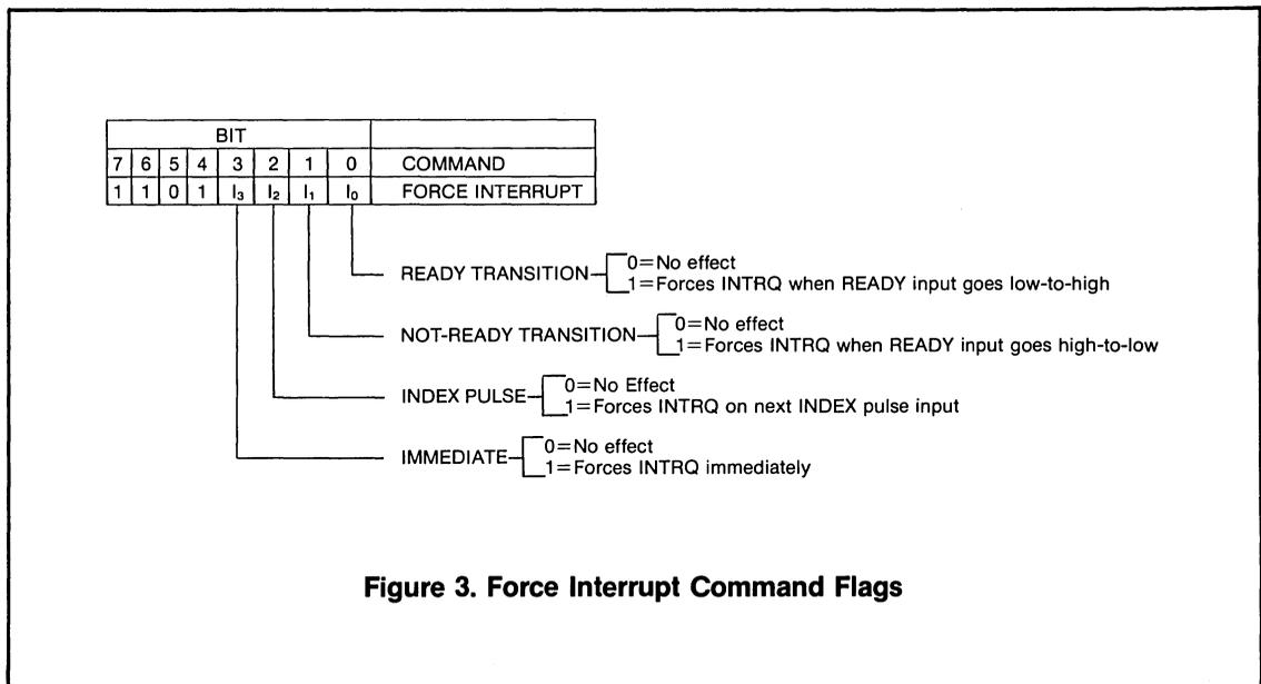
Figure 3. Force Interrupt Command Flags
