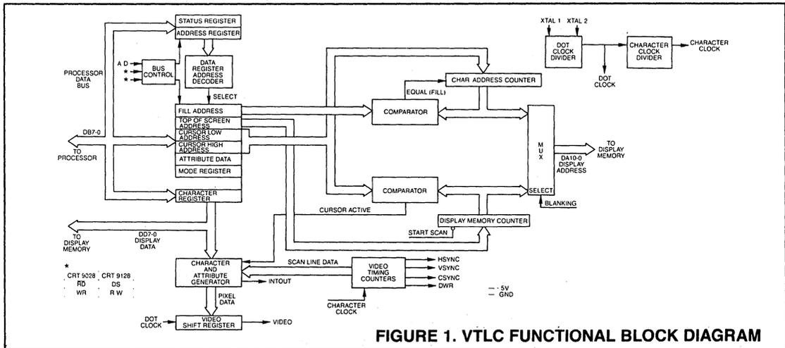
**FIGURE 1. VTLC FUNCTIONAL BLOCK DIAGRAM**
