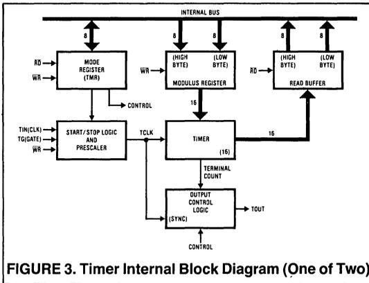
FIGURE 3. Timer Internal Block Diagram (One of Two)
