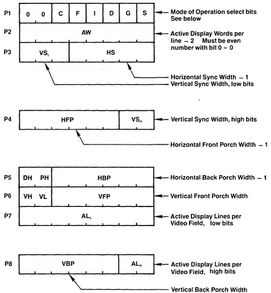
In graphics mode, a word is a group of 16 pixels. In character mode, a word is one character code and its attributes, if any. The number of active words per line must be an even number from 2 to 256. An all-zero parameter value selects a count equal to  $2^n$  where  $n$  = number of bits in the parameter field for vertical parameters. All horizontal widths are counted in display words. All vertical intervals are counted in lines.
