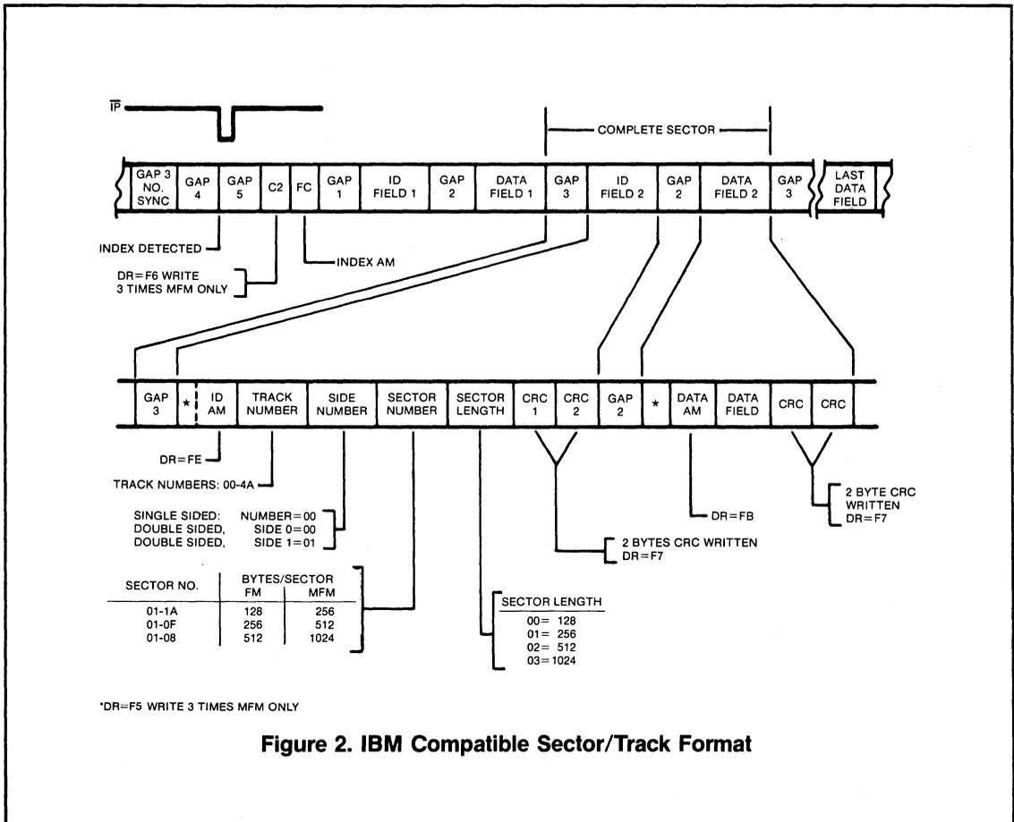
Figure 2. IBM Compatible Sector/Track Format
