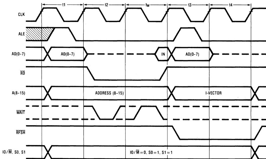
FIGURE 2b. Opcode Fetch Cycles with  $\overline{\text{WAIT}}$  States
