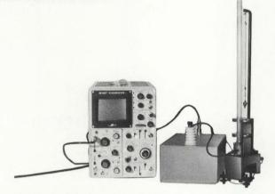
\*Output voltage measurement by using synchroscope
