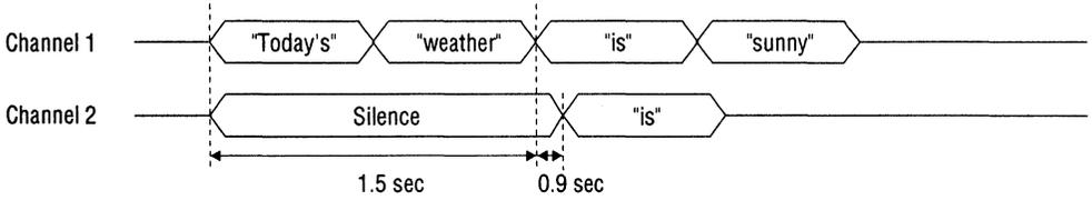
Figure 13.6 Vocalization Timing Using Edit Data of Table 13.14
