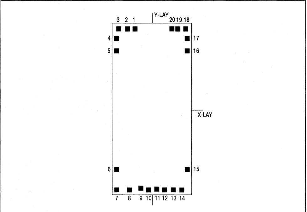
Pad Position (the die center is located at X=0, Y=0)
