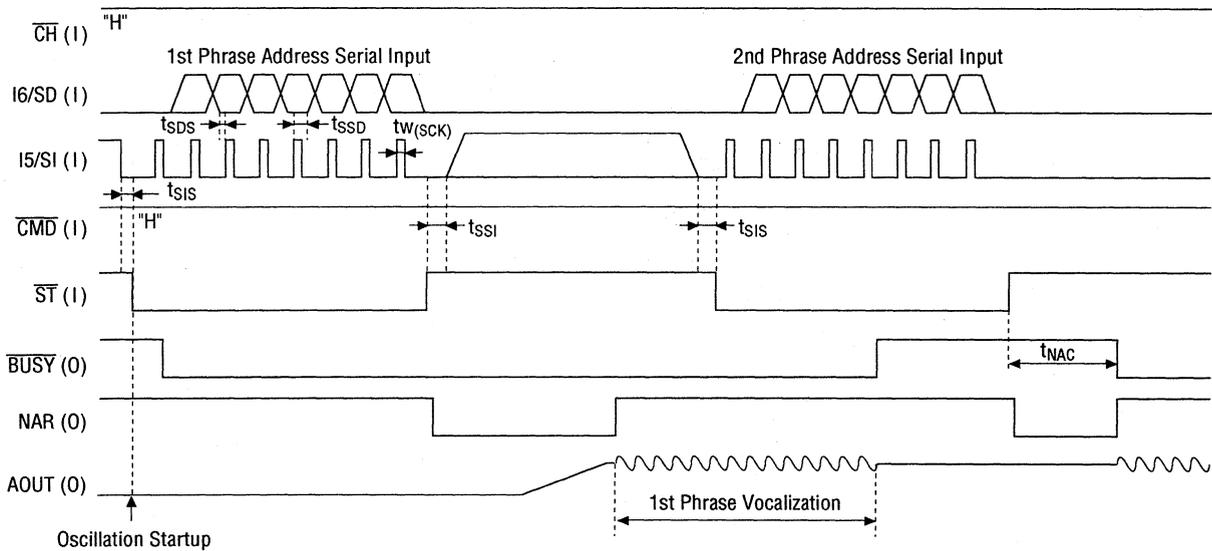
In serial input, data is transferred to the LSI when the  $\overline{ST}$  signal rises after serial data is input. SD is captured at the former edge of SI.
