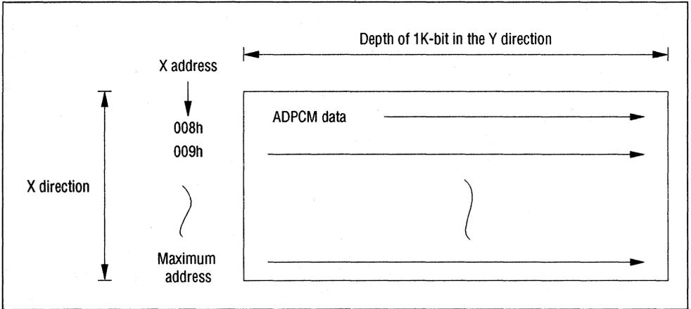
The storage method of ADPCM data per 1 address in the X-direction (1K-bit) is different for 3-bit and 4-bit ADPCM. It is summarized as follows:
