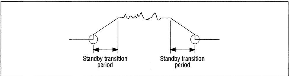
Figure 9 Pop Noise of Low-pass Filter Output
