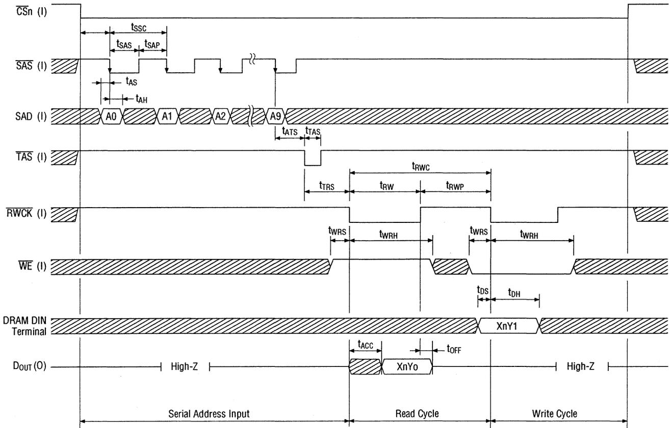
DRAM Drive Timing (Write Cycle, Write Time)
