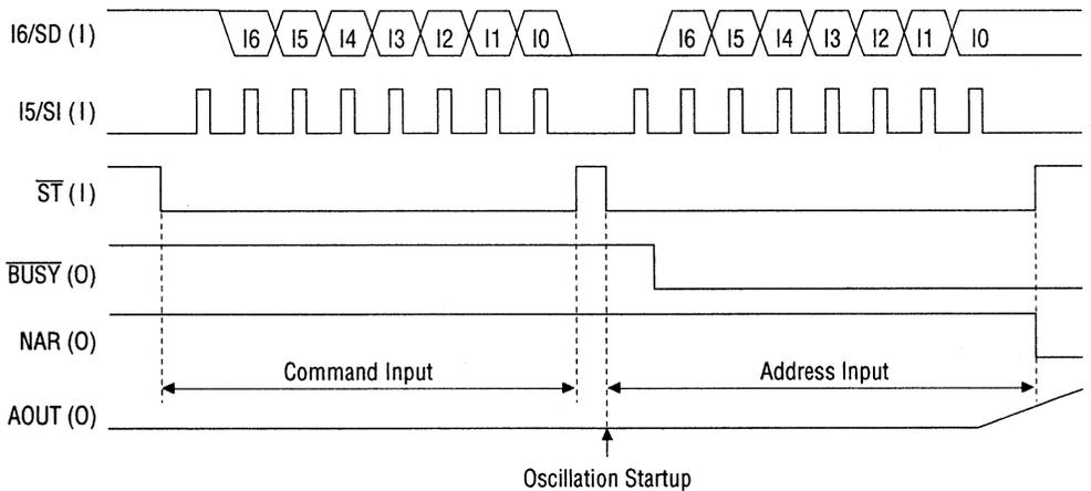
**Figure 4.2 Command, Address Input Timing (Serial Input)**
