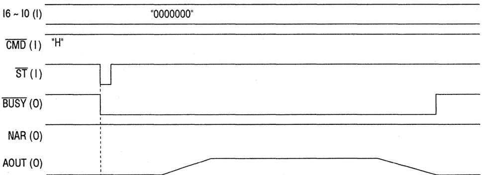
Figure 8.2 Timing when Stop Code is Input in Standby Status
