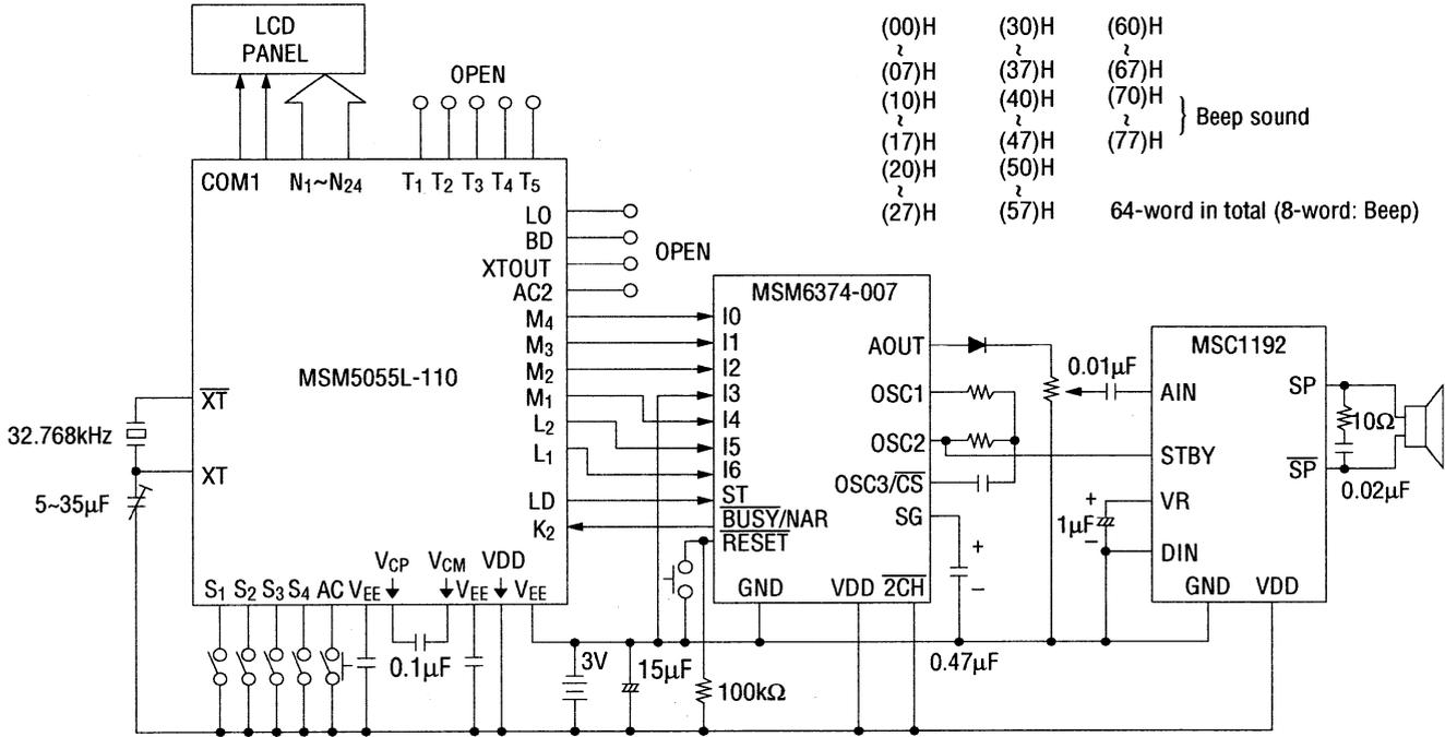
Note: When the LSIs are connected as shown below, usable addresses of the MSM6374 are as follows:
