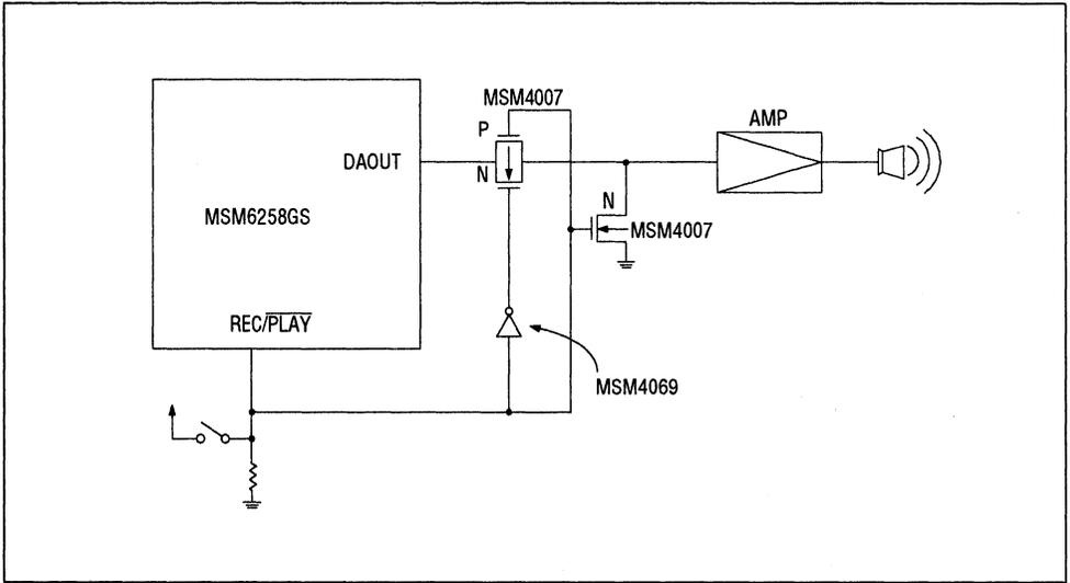
Figure 33 Example of Mute Circuit for Recording
