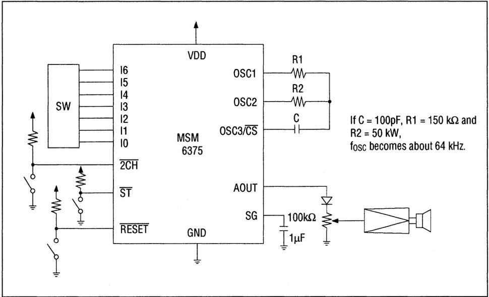
Figure 15 Application Circuit Example in the Case of Selecting RC, LPF and SW in Option
