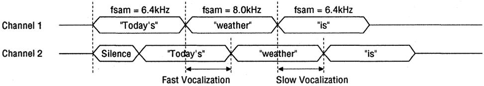
**Figure 12.5 Vocalization Timing of Echo Regenerations with Different Sampling Frequencies**
