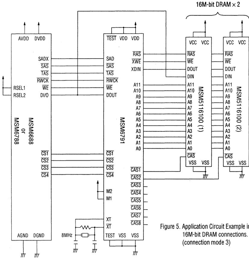
Figure 5. Application Circuit Example in two 16M-bit DRAM connections. (connection mode 3)
