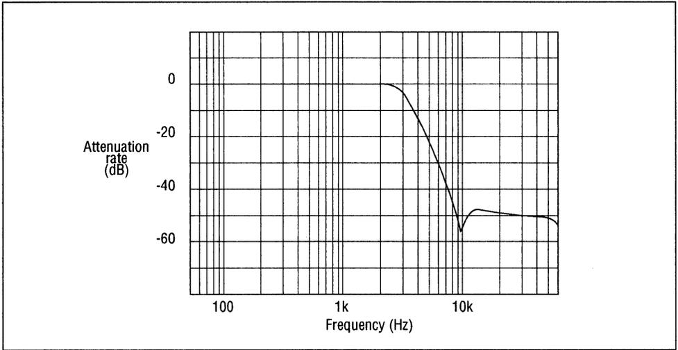
**Figure 8 Low-pass Filter Characteristics (fsam=8kHz)**
