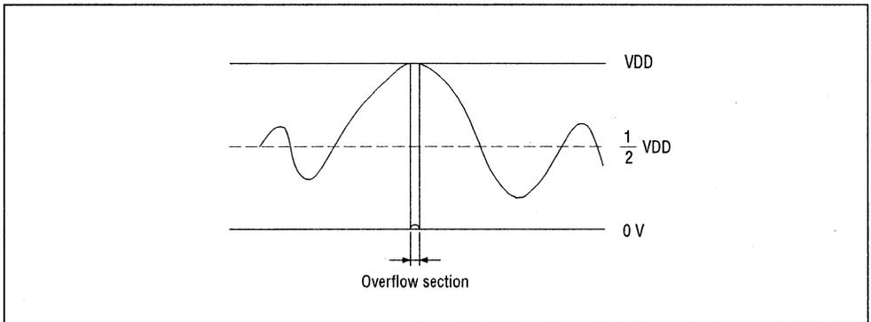
**Figure 9 Output Waveform When an Overflow Occurs**
