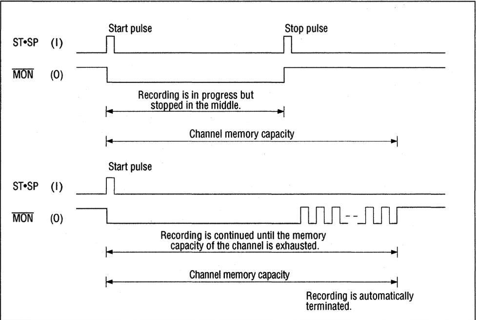
**Note:** As mentioned above, the memory capacity of the external serial registers is divided by the number of phrases and is assigned as the channel memory capacity. During recording, ADPCM data is written, starting from the first address of the memory of the specified channel. When recording is terminated in the middle of the channel memory capacity by a stop pulse, the subsequent memory area remains unused.
