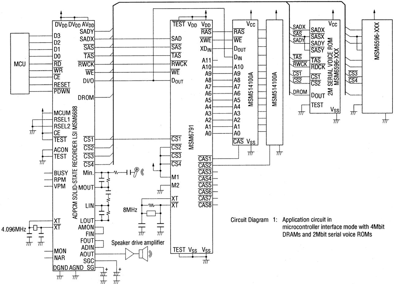
Circuit Diagram 1: Application circuit in microcontroller interface mode with 4Mbit DRAMs and 2Mbit serial voice ROMs
