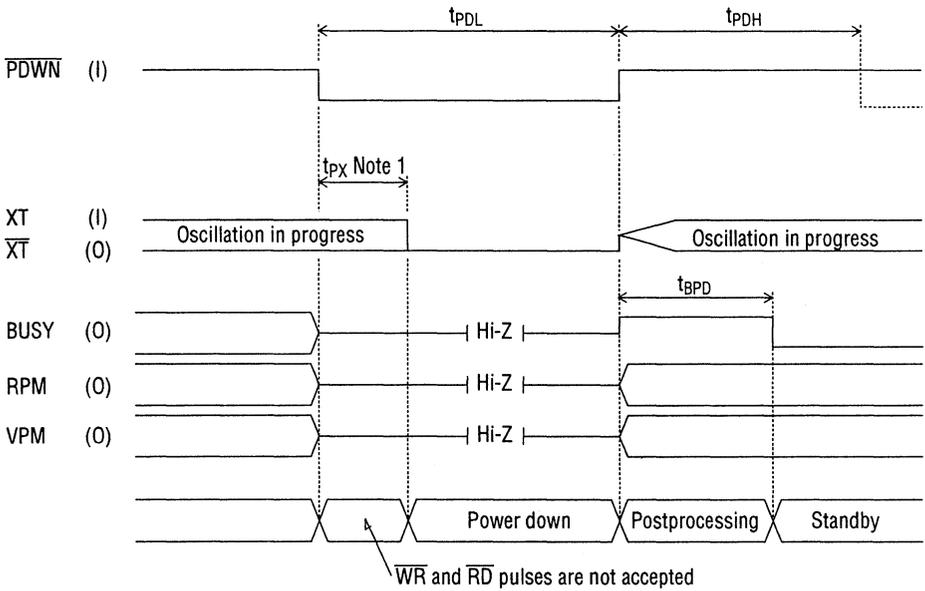
**Note 1:** When an external clock is used, apply a low level to the  $\overline{\text{PDWN}}$  pin and then continue to apply the external clock to the XT pin for  $t_{\text{PX}}$ .
