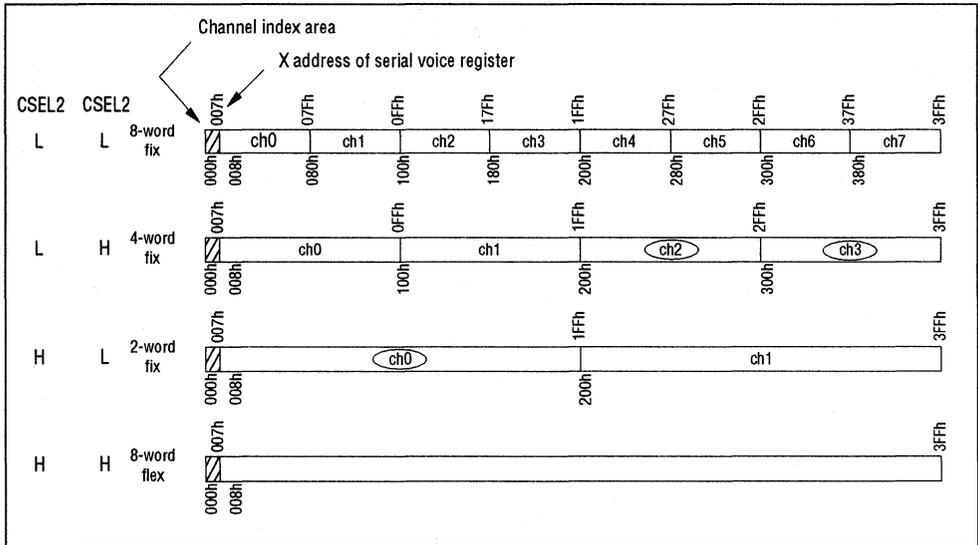
By combining CSEL1, CSEL2, CA1, CA2 and CA3, it is possible to assign (the circled channels) ch0=16 seconds, ch2=8 sec-
