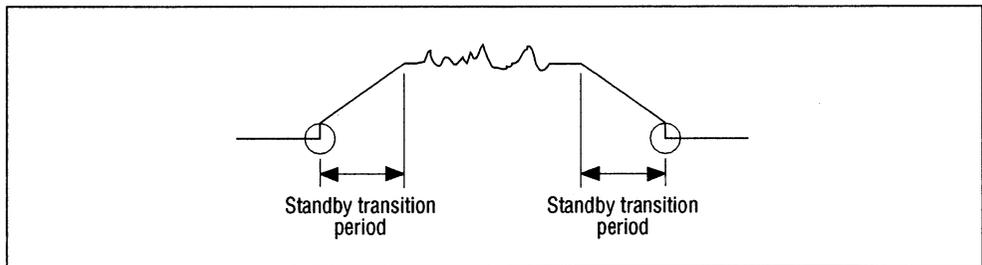
Figure 9 Pop Noise of Low-pass Filter Output
