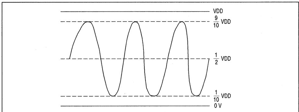
**Figure 10 Waveform When the Maximum Amplitude Level of the Input Waveform is about 80% of the Dynamic Range**
