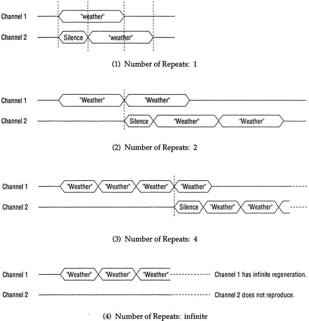
**Figure 12.3 Vocalization Timing of Echo Reproduction According to Number of Repeats**
