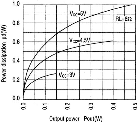
Power dissipation vs output power (example)
