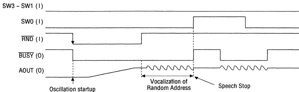
**Figure 5.9 Timing when a Pulse is Input to SW0 pin during Random vocalization**
