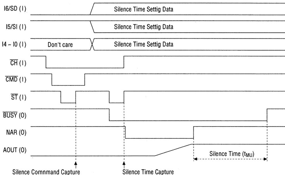
**Figure 6.2 Channel 2 Silence Setting Timing (Parallel Input)**
