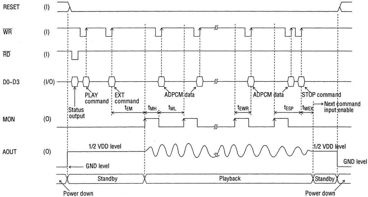
● Timing for DC Level Transition by LEV Command
