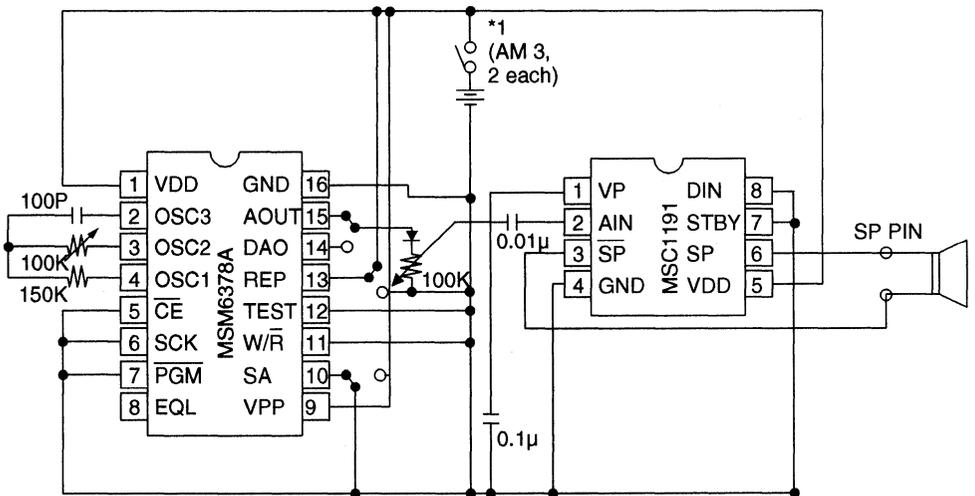
\* Note: The guaranteed voltage of LPF output of MSM6378 ranges from 2.7 V ~ 5.5 V.
