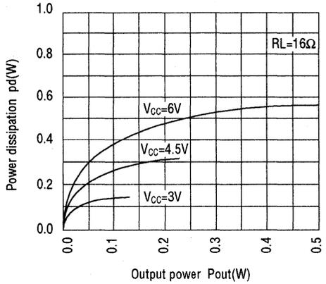
Power dissipation vs output power (example)
