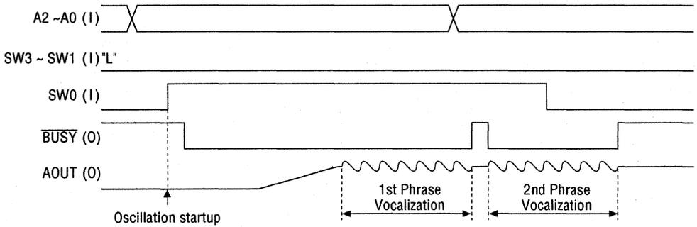
**Figure 5.3 Complete SW Input Interface Vocalization Timing**
