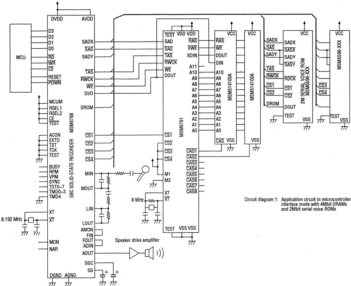
Circuit diagram 1: Application circuit in microcontroller interface mode with 4Mbit DRAMs and 2Mbit serial voice ROMs
