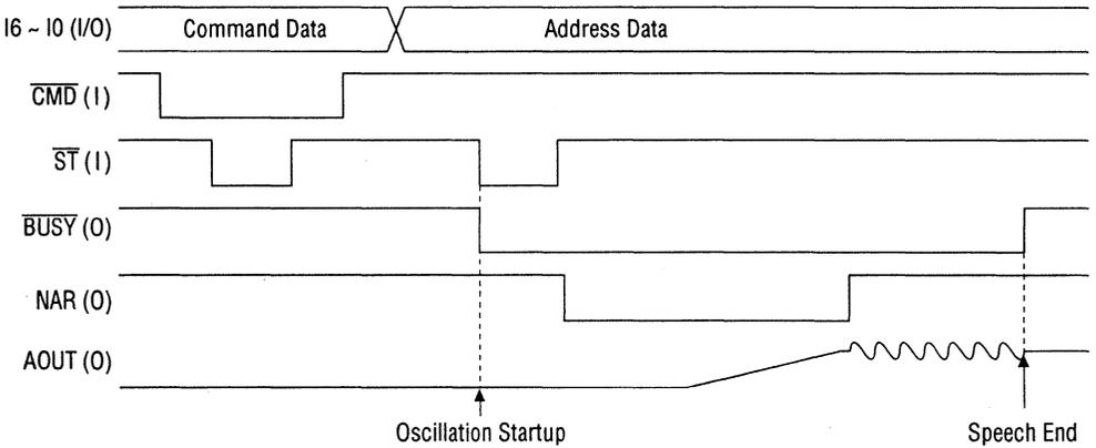
Figure 5.1 Command, Address Input Timing (Parallel Input)
