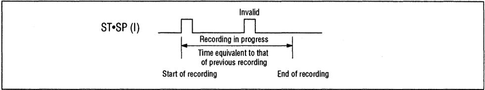
**Figure 7 Recording in Status B (Preservation of Data in Channel)**
