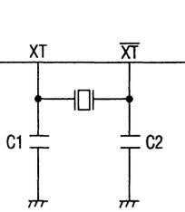
Figure 16.1 External circuit diagram
