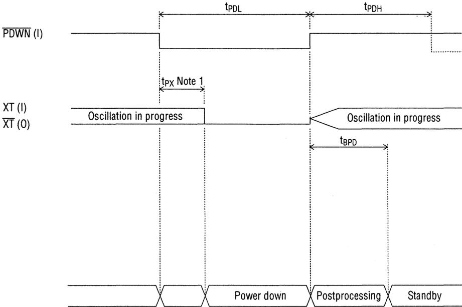
**Note 1:** When an external clock is used, continue to apply the clock input to the XT terminal during  $t_{px}$  after the  $\overline{\text{PDWN}}$  pin is set to a low level.
