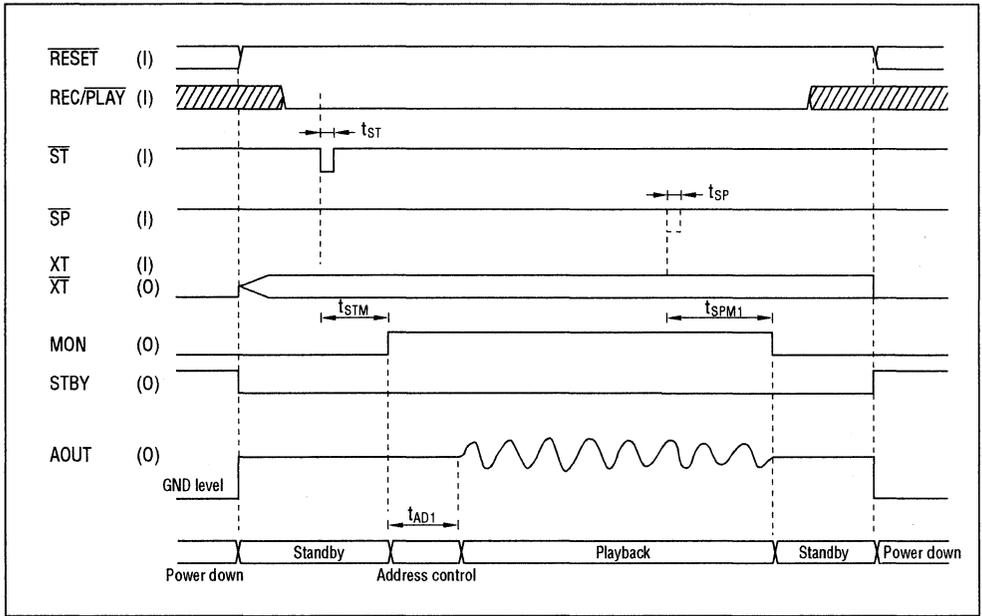
8. Timing during repeated playback (PDMD pin = "H")
