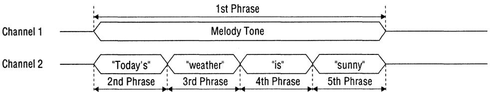
Figure 13.7 Example of Four Phrase Channel Synthesis Timing with Melody Tone as GBM
