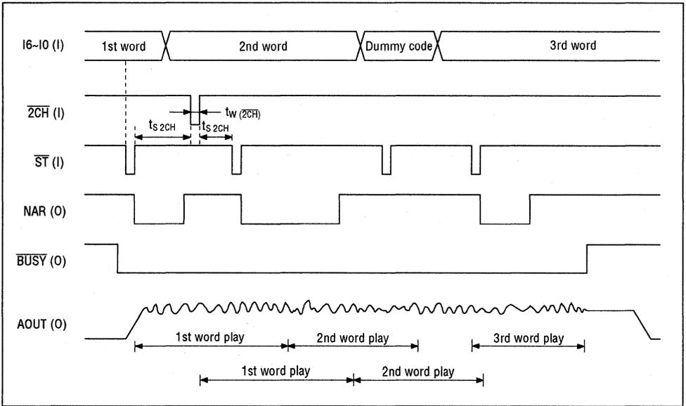
1. Input of the  $\overline{2CH}$  pulse without lowering  $\overline{ST}$  starts echo playback. Echo playback is canceled unless play is continuous.
