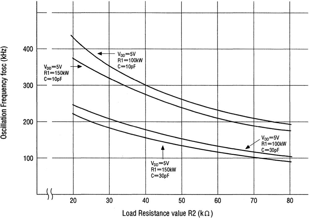
Figure 12.1 RC oscillation Frequency eharacteristics
