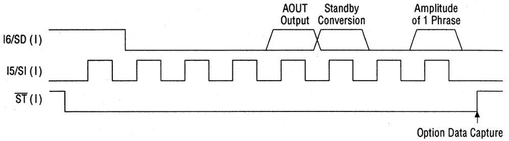
Figure 4.2 Option Setting Timing (during Serial Input)
