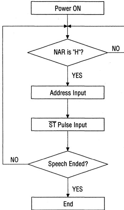
Figure 4.3 Input Flow Chart when Command Is Not Set
