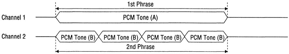
**Figure 10.9 Example of Channel Synthesis between PCM Main Melody Tone (A) and PCM Rhythm Tone (B) with 4 Repeats**
