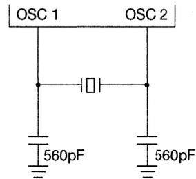
**Figure 3-1 Ceramic Oscillator (CSB256D) Connection Circuit**
