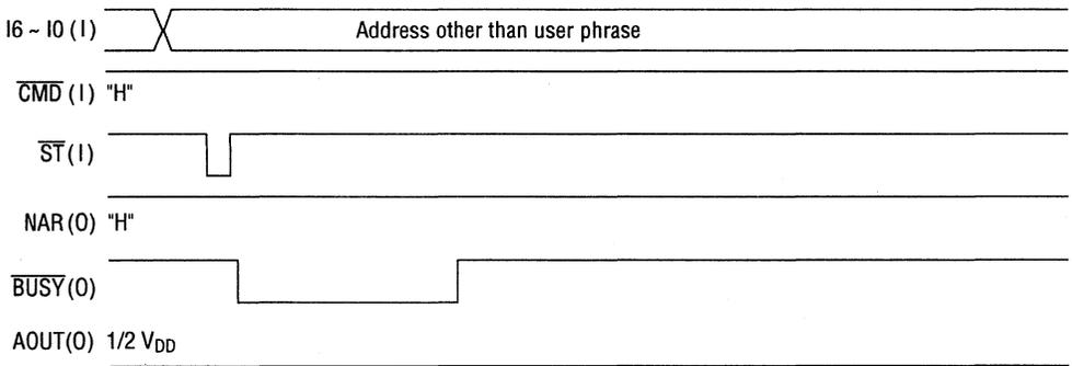
**Figure 6.3 Timing when Address, other than User Phrase, Is Input in Status that AOUT is 1/2 V<sub>DD</sub>**
