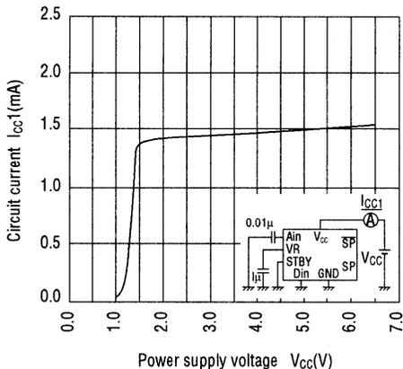
Circuit current vs power supply voltage (example)
