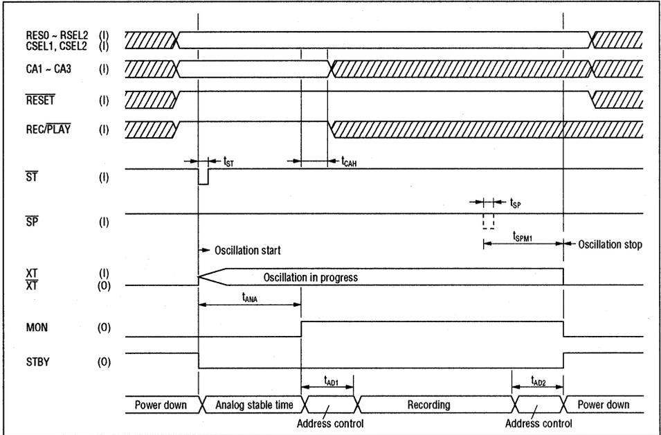
2. Timing during voice triggered starting function on record (PDMD pin="L", VDS pin="H")
