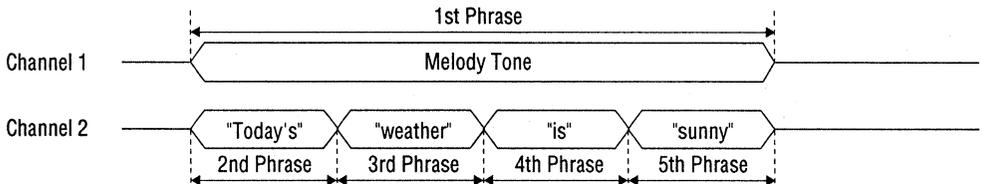
**Figure 10.7 Example of Four Phrase Channel Synthesis Timing with Melody Tone as BGM**
