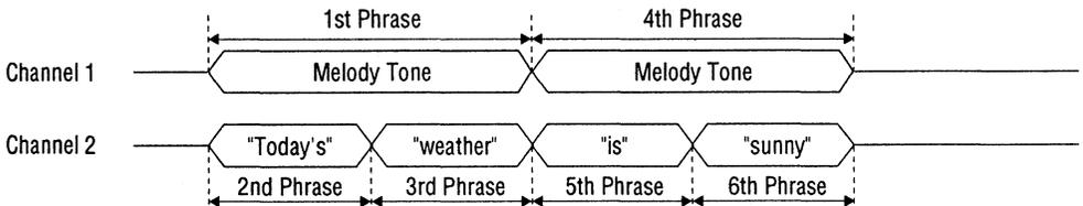
Figure 13.8 Example of Four Phrase Channel Syntehsis Timing with Melody Tone and 1st and 4th Phrases as BGM
