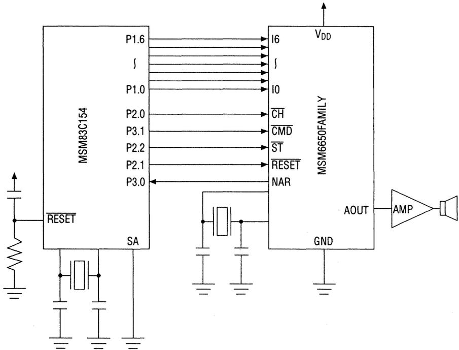
Example of Application Circuit at Parallel Input Interface
