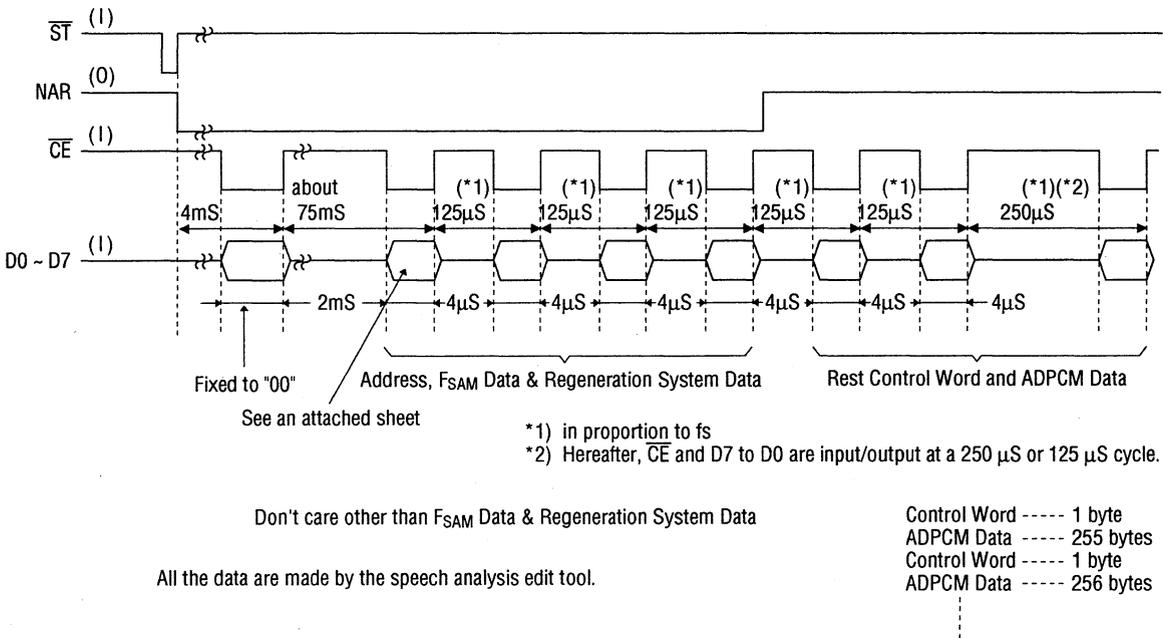
Figure 15.1 External ROM Driving Timing
