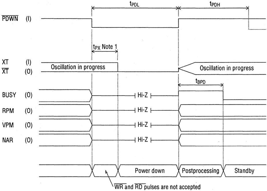
**Note 1:** When an external clock is used, apply a low level to the  $\overline{\text{PDWN}}$  pin and then continue to apply the external clock to the XT pin for  $t_{\text{PX}}$ .
