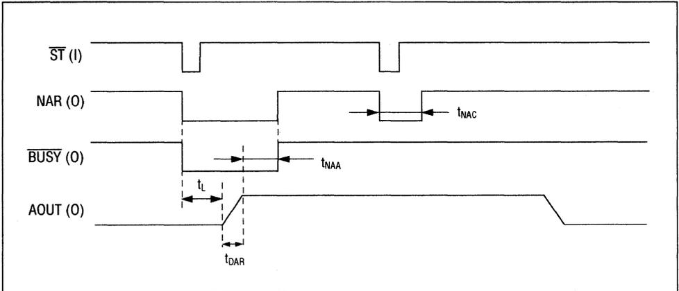
6. Timing Diagram of Echo Playback in Channel 1
