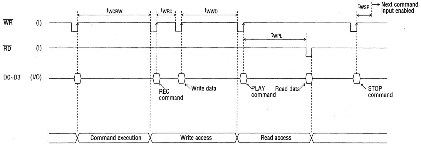
● Timing for Data Transfer by DTRW Command
