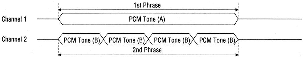
**Figure 13.9 Example of Channel Synthesis between PCM Main Melody Tone (A) and PCM Rhythm Tone (B) with 4 Repeats**
