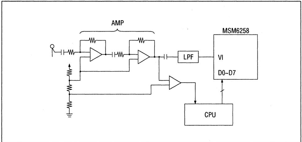
Figure 34 Voice-Triggered Starting Circuit for CPU Interface
