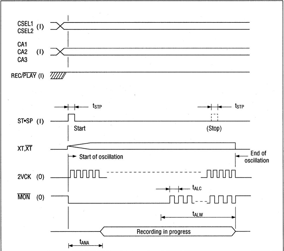
**Note:** When the remaining capacity of available memory of the selected channels falls to 128K-bit (last four seconds) during recording, a 4Hz clock is output from the  $\overline{MON}$  pin. ( $f_{sam}=8kHz$ )
