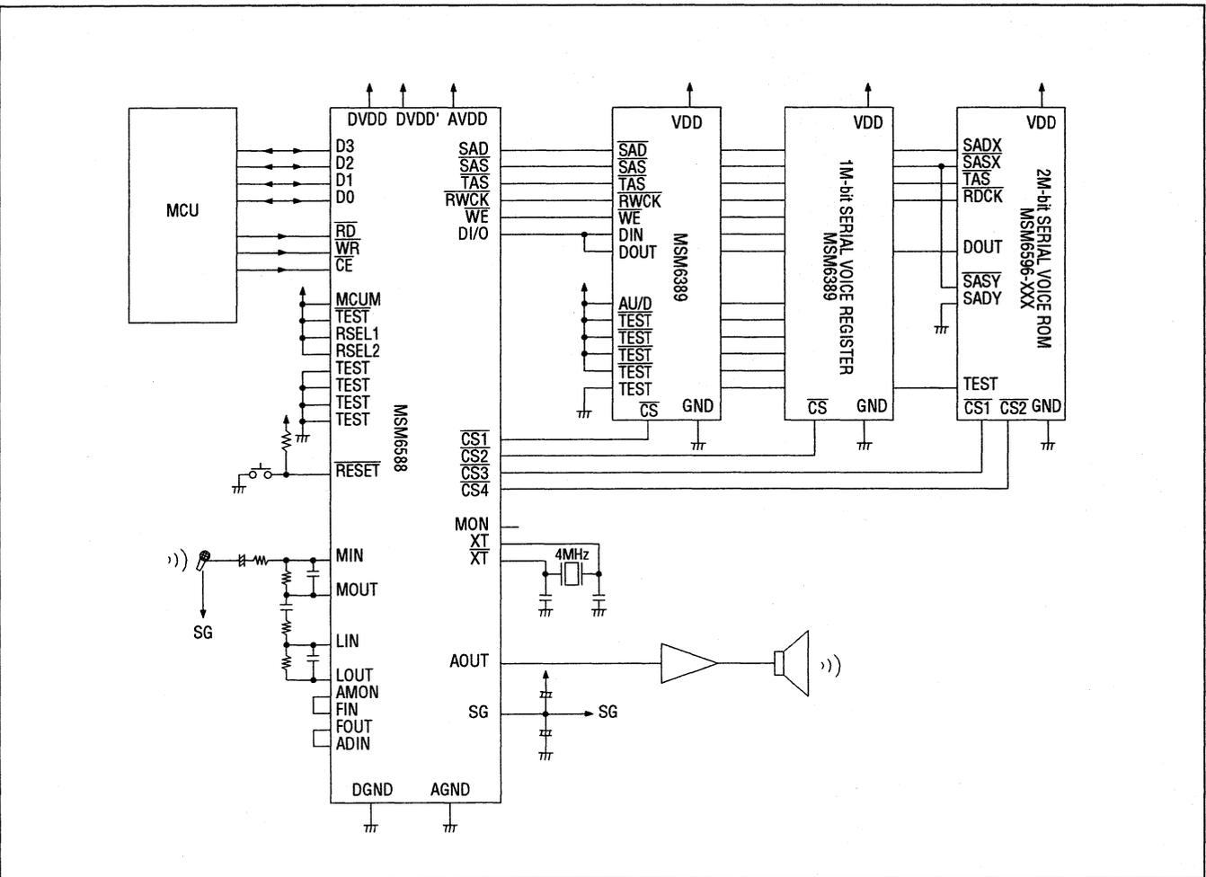
Note: MSM6588 cannot control the MSM6596-XXX without a Serial Voice Register.
