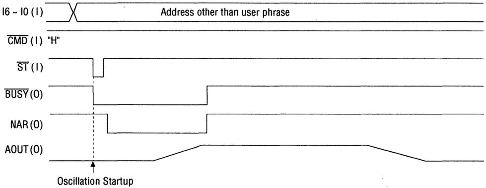
**Figure 6.2 Timing when Address, other than User Phrase, Is Input in Standby Status**
