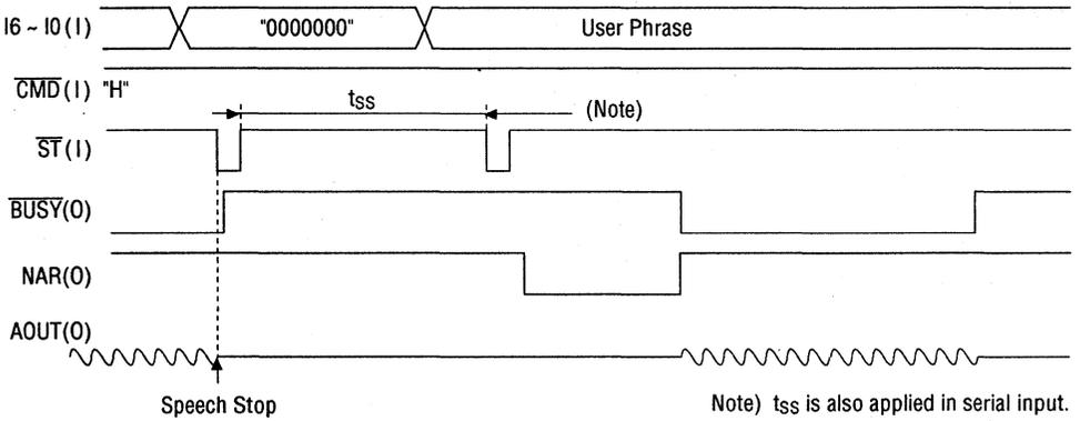
Figure 7.1 Stop Code Input Timing
