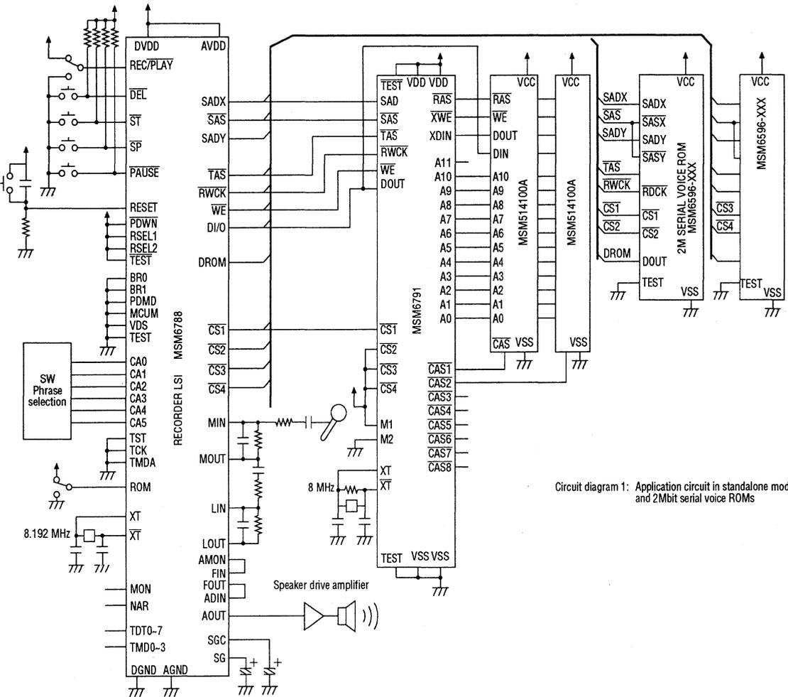
Circuit diagram 1: Application circuit in standalone mode with 4Mbit DRAMs and 2Mbit serial voice ROMs
