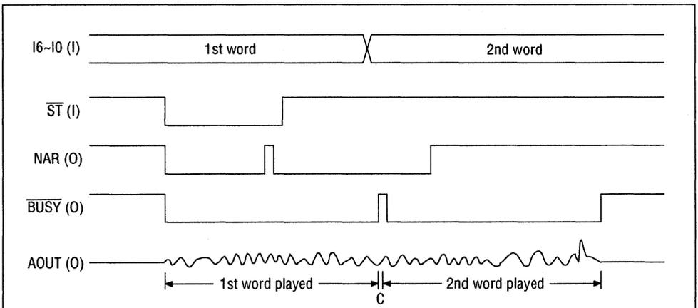
Figure 2 Timing of CPU Interface ( $800\mu s < \overline{ST}$ )
