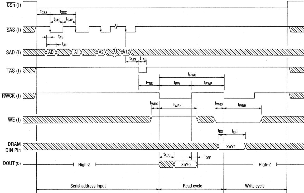
DRAM Drive Timing (Write cycle at recording)
