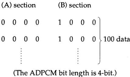
Since an offset of about 5 mV can be obtained for each 2 samples of data, it is recommended that about 100 samples of data be entered to shift the waveform center about 250 mV.
