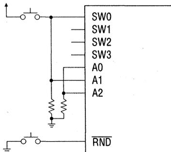
Figure 4.10 Circuit Example to Stop Random Vocalization
