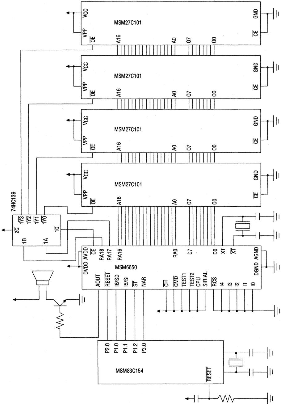
Application circuit example when four 1-Mbit EPROMs are used (serial input interface).
