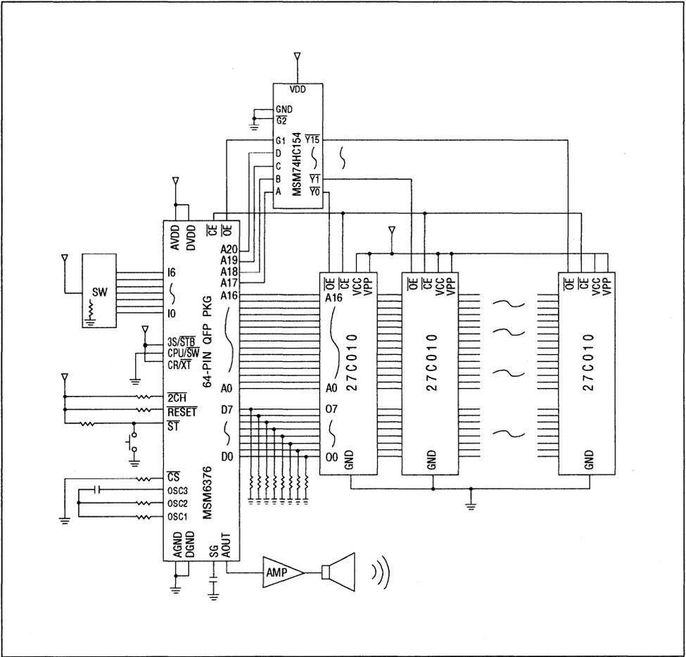
**Note:** Use a CMOS type 27C010 as an EPROM if possible. If an NMOS type EPPROM is used the power voltage variation of the EPROM becomes a source to generate noise.
