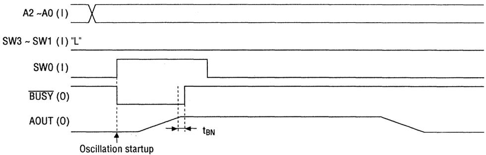
**Figure 5.5 Timing when Speech is Started up at an Address except the User-Specified Phrase**
