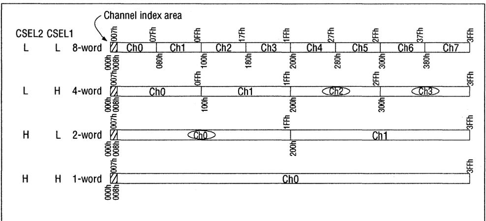
**Note:** By the combination of CSEL1, CSEL2, CA1, CA2 and CA3, the circled channel memory capacities can be allocated as Ch0=16sec., Ch2=8 sec. and Ch3=8 sec. (@ $f_{sam}=8kHz$ ).
