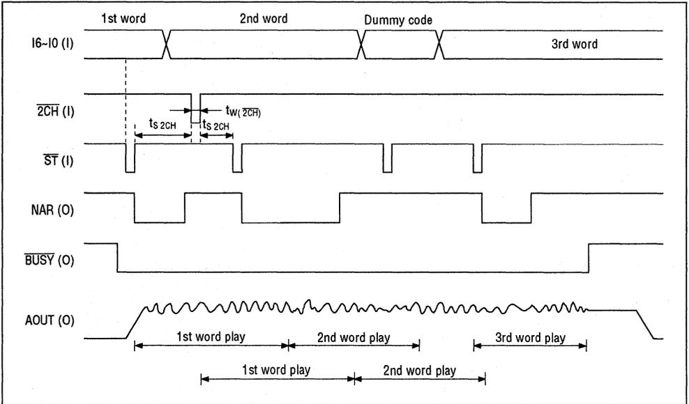
1. Input of the  $\overline{2CH}$  pulse without lowering  $\overline{ST}$  starts echo playback. Echo playback is canceled unless play is continuous.
