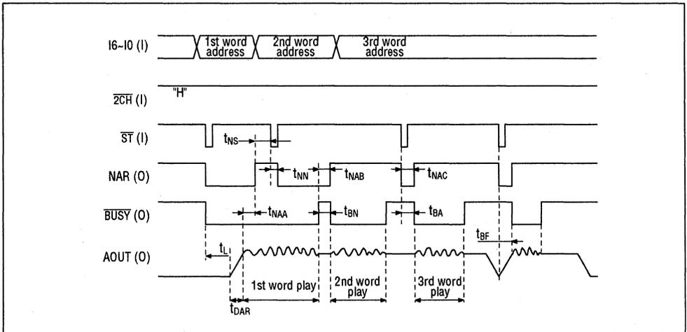
4. Operation in Channel 2 Only (CPU input interface)
