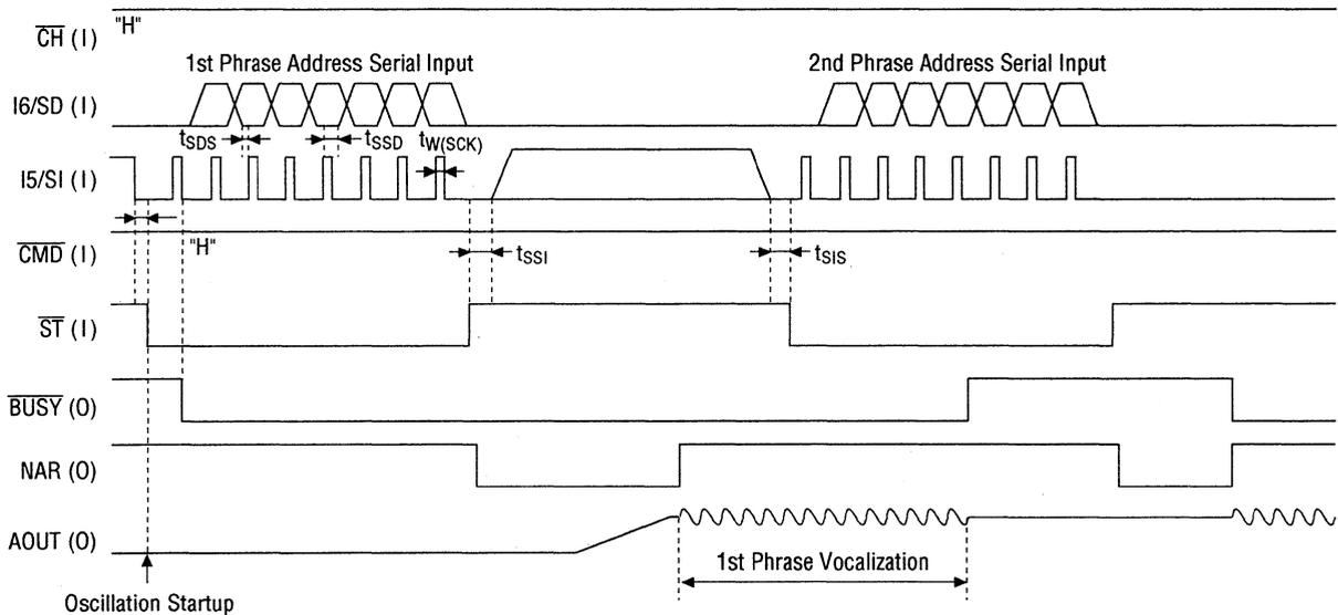
In serial input, data is transferred to the LSI when the ST signal rises after serial data is input. SD is captured at the former edge of SI.
