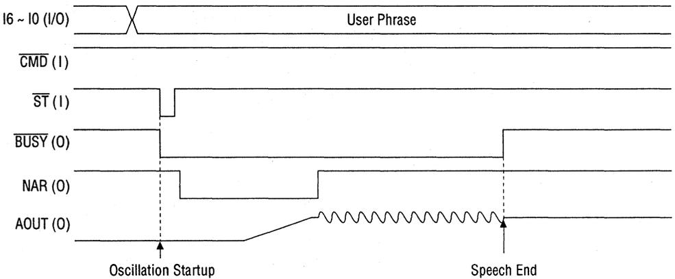
Figure 7.1 Speech Startup Timing
