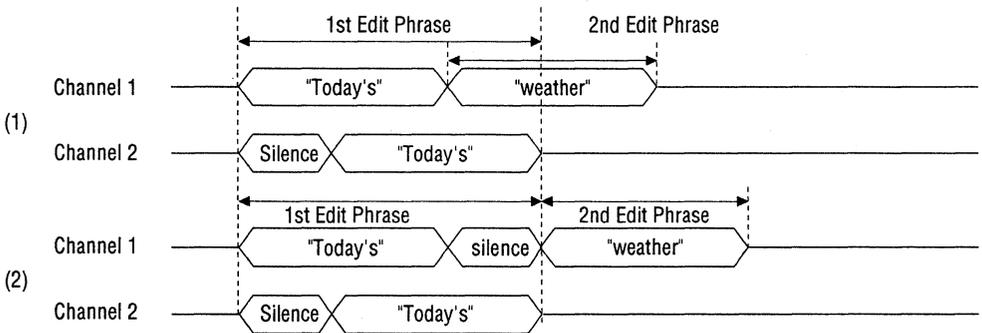
Figure 12.2 Example of Continuous Regeneration Timing
