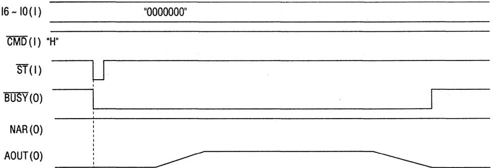
Figure 7.2 Timing when Stop Code Is Input in Standby Status
