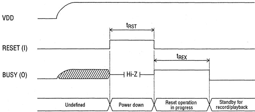
● Power Down by the  $\overline{\text{PDWN}}$  pin
