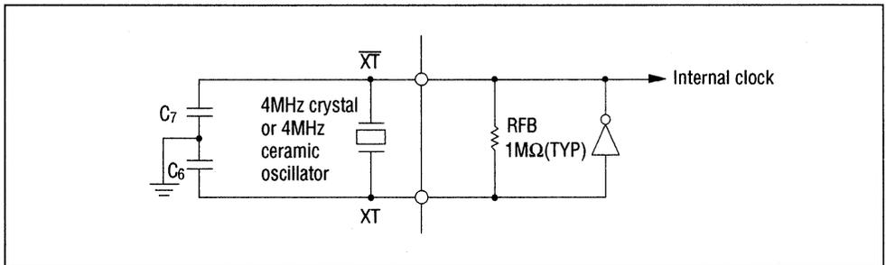
Figure 5 Oscillation Circuit
