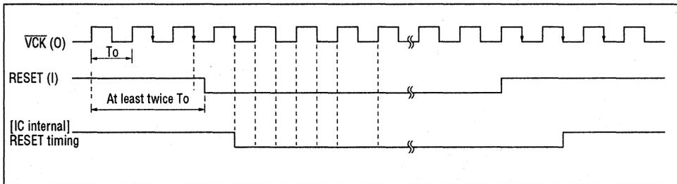
**Figure 8 MSM5205 Reset Timing**
