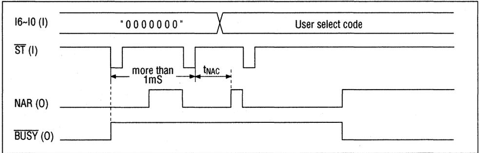
Figure 6 Example of STOP Code Input Timing
