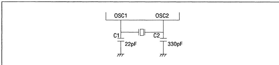
Figure 13 Circuit Diagram of Crystal Oscillator Connection
