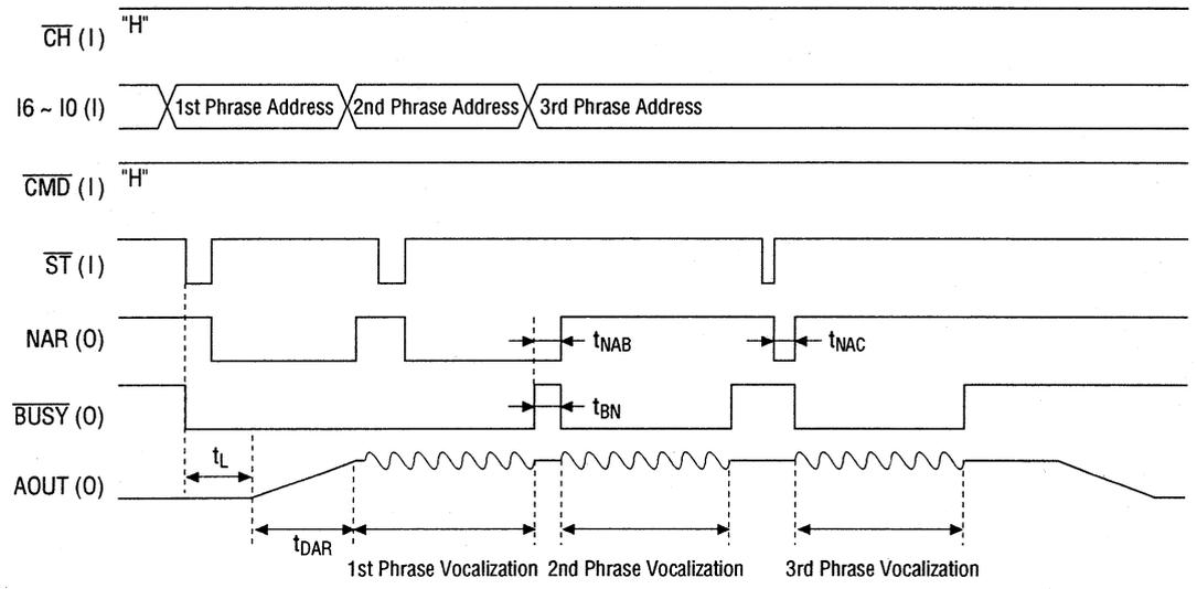
4. Channel 1 Regeneration Timing Chart when External Command is used (Parallel Input)
