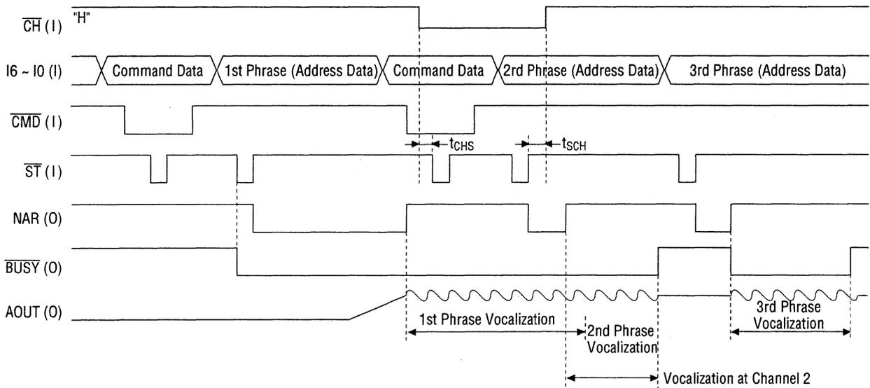
Since command data is maintained independently at channels 1 and 2, If speech is started up at channel 1 without a command setting, speech is vocalized by the same command set at the 1st phrase.
