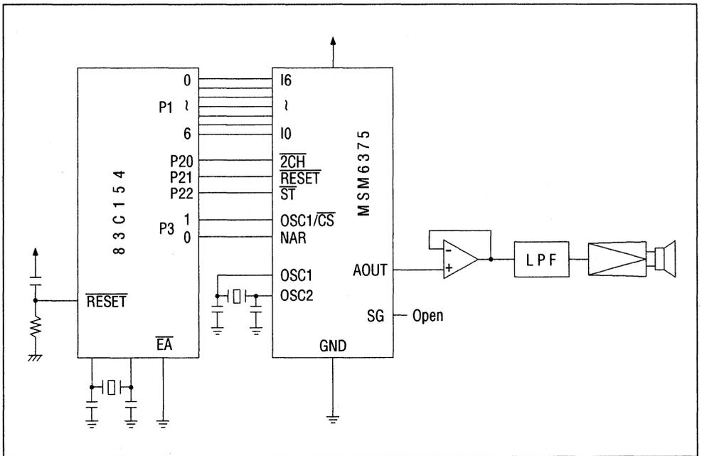
Figure 16 Application Circuit Example in the Case of Selecting XT, DAC and CPU in Option
