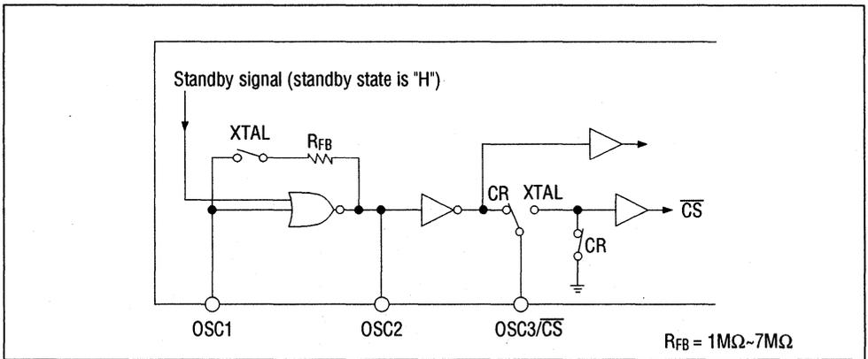
Figure 14 Internal Oscillation Circuit
