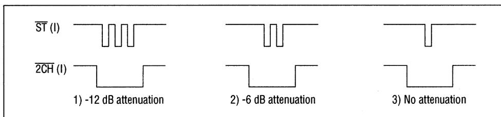
**Figure 7 Input Timing of 2 Channel Mixing**
