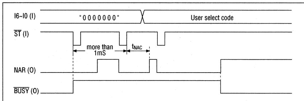
Figure 6 Example of STOP Code Input Timing
