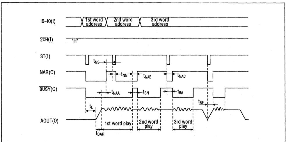
4. Operation in Channel 2 Only (CPU input interface)
