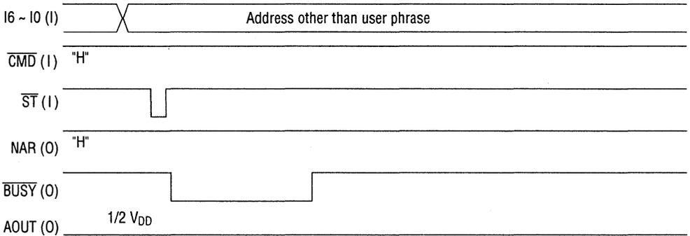
**Figure 7.3 Timing when Address, other than User Phrase, is Input in Status that AOUT is 1/2 V<sub>DD</sub>**
