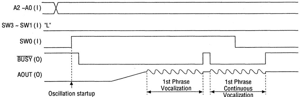
**Figure 4.2 Complete SW Input Interface Repeat Vocalization Timing**
