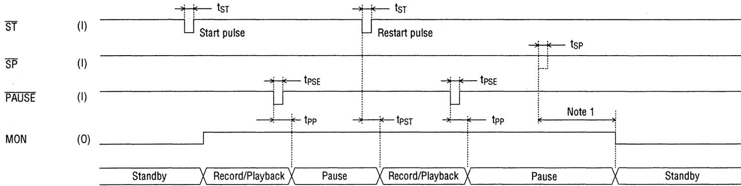
Note 1: This time interval varies depending on the state of PDMD pin and the record/playback mode and is one of  $t_{PMH1}$ ,  $t_{PMH2}$ ,  $t_{PMH3}$ ,  $t_{PML2}$  and  $t_{PML3}$ .
