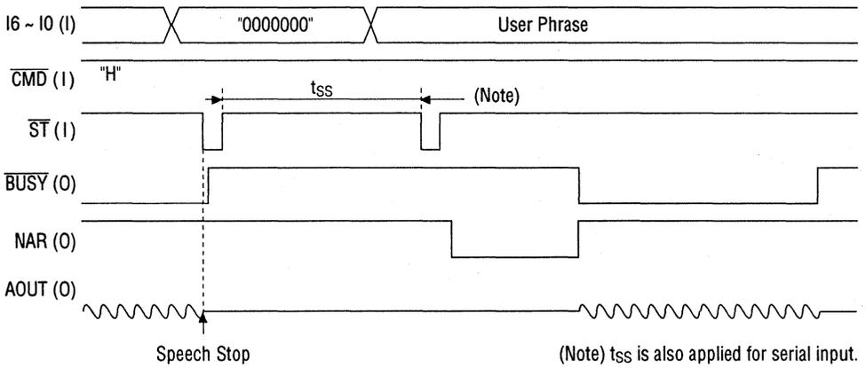
Figure 8.1 Stop Code Input Timing
