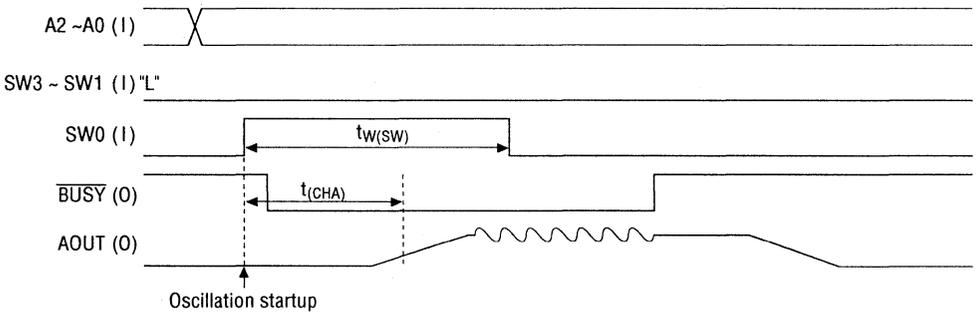
Figure 5.1 Complete SW Input Interface 1 Phrase Vocalization Timing
