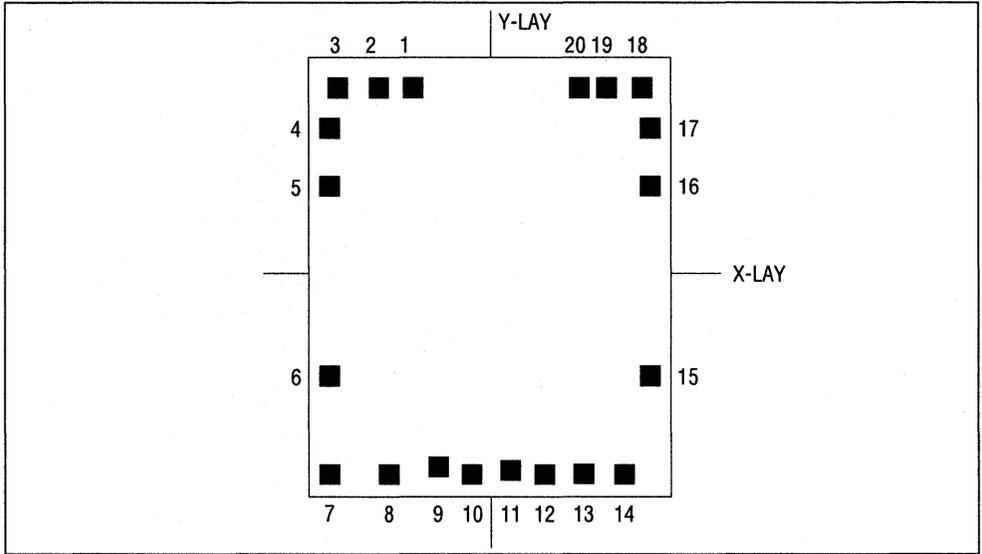
Pad Position (the die center is located at X=0, Y=0)
