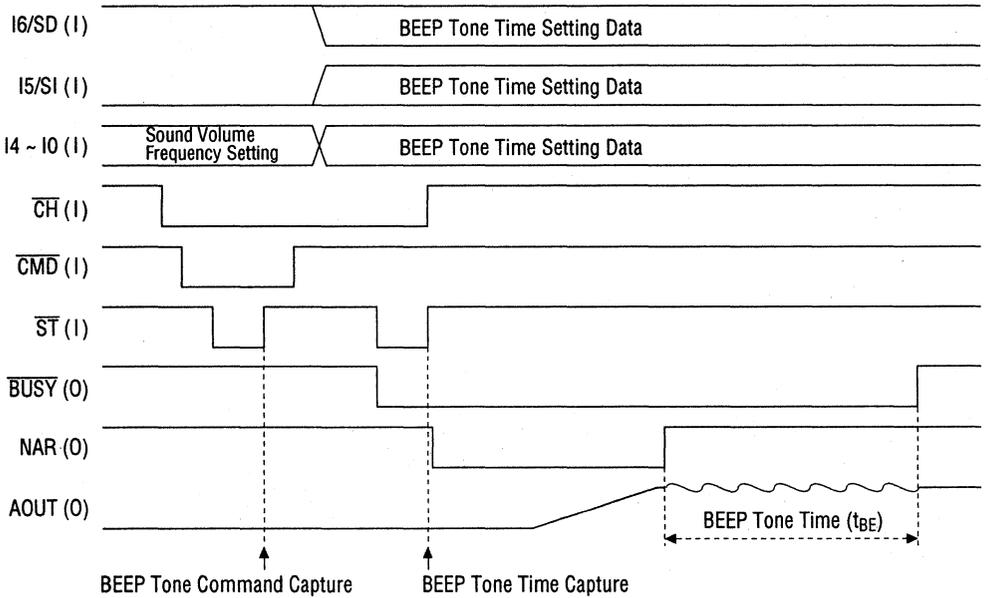
Figure 5.6 BEEP Tone Setting Timing (during Parallel Input)
