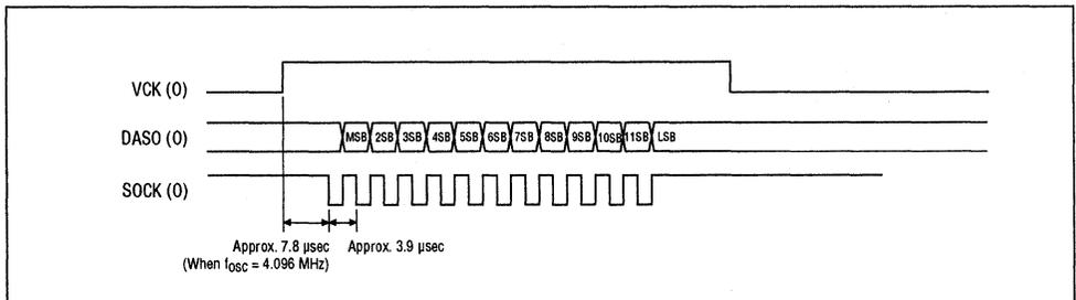
Figure 2-2 Use of External DA Converter and Timing
