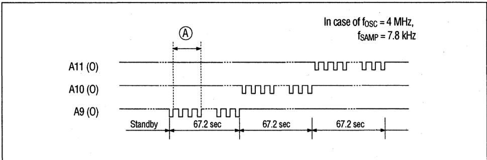
Figure 15 Address Timing for 256 × 4-Bit DRAM
