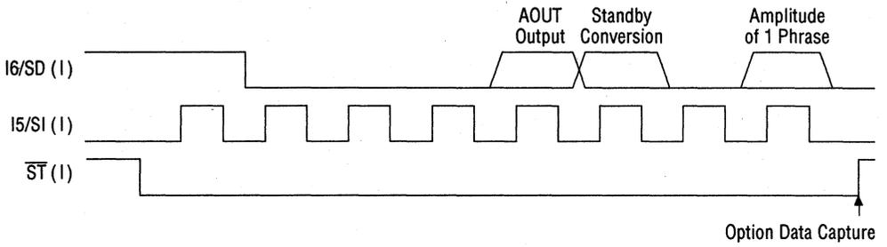
Figure 3.2 Command Option Setting Timing (during Serial Input)
