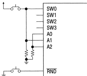
**Figure 5.10 Circuit Example to Stop Random Vocalization**
