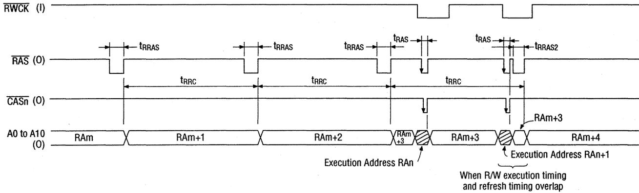
DRAM Drive Timing (When R/W timing and refresh timing overlap)
