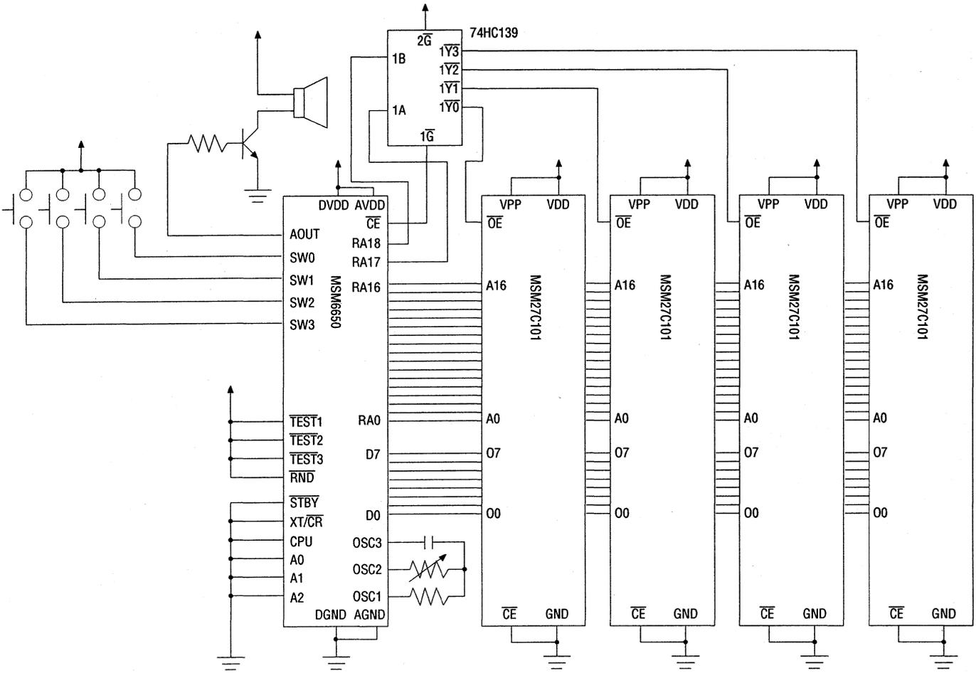
Application Circuit Example when Using Four 1 Mbit EPROMs
