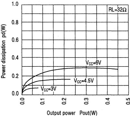
Power dissipation vs output power (example)
