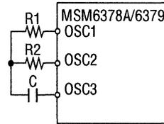
The values of C, R1, and R2 for the above table are for the MSM6378A 16-pin DIP. The oscillation frequency fluctuates with an external resistance and floating capacity. Therefore, since the oscillation frequency fluctuates when the board wiring and packages are different, determine the constant after check with monitoring fosc at OSC3 pin with reference to the above table.
