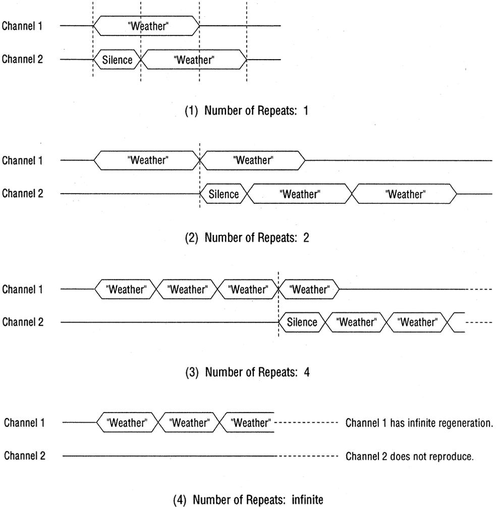
**Figure 10.3 Vocalization Timing of Echo Regeneration According to Number of Repeats**
