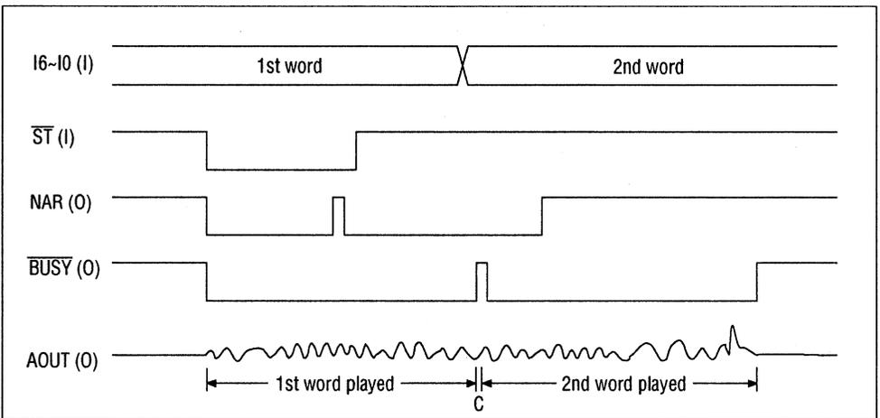
Figure 2 Timing of CPU Interface ( $800 \mu s < \overline{ST}$ )
