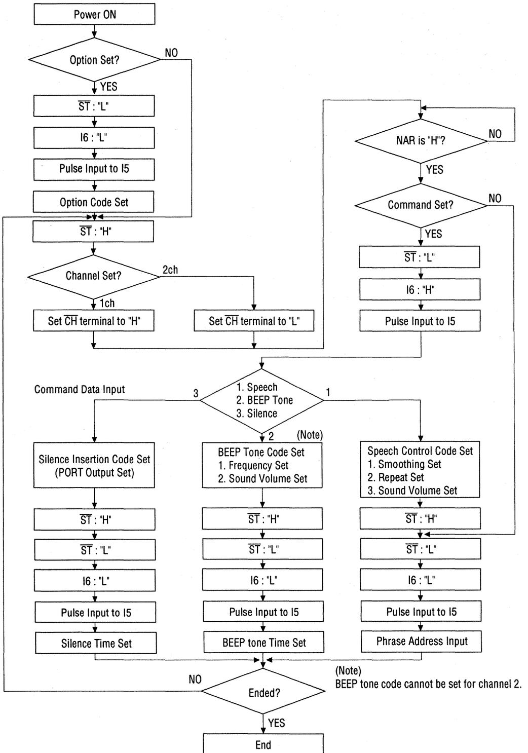
Figure 4.5 Serial Input Flow Chart when External Command is used
