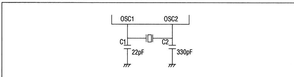
**Figure 13 Circuit Diagram of Crystal Oscillator Connection**
