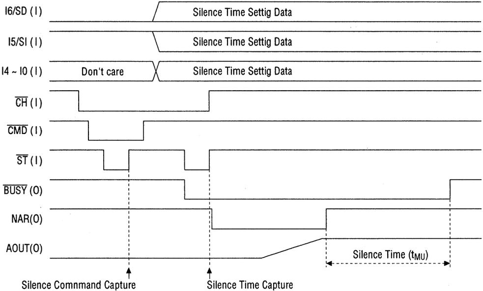
**Figure 5.4 Channel 2 Silence Setting Timing (Parallel Input)**
