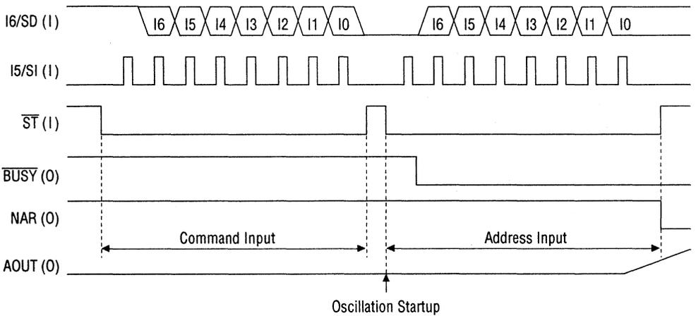
Figure 5.2 Command, Address Input Timing (Serial Input)
