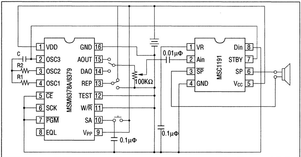
**Note:** \* MSC1191 is the most suitable amplifier to drive a speaker for the voice LSI. When MSM6378A terminates the reproduction of speech data, MSC1191 is also put into power save mode automatically.
