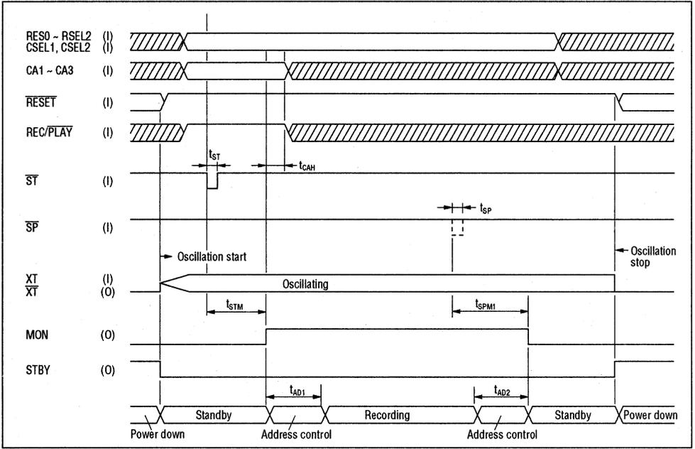
6. Timing during voice triggered starting function on record (PDMD pin="H", VDS pin="H")
