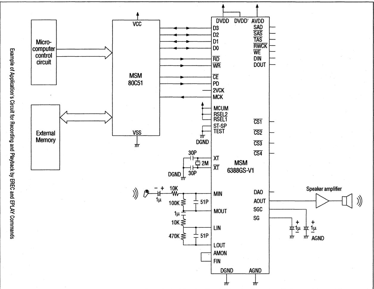
Example of Application's Circuit for Recording and Playback by EREC and EPLAV Commands
