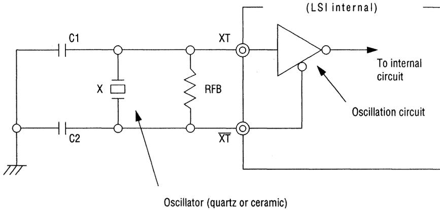
Figure 1. Quartz/Ceramic Oscillation Circuit
