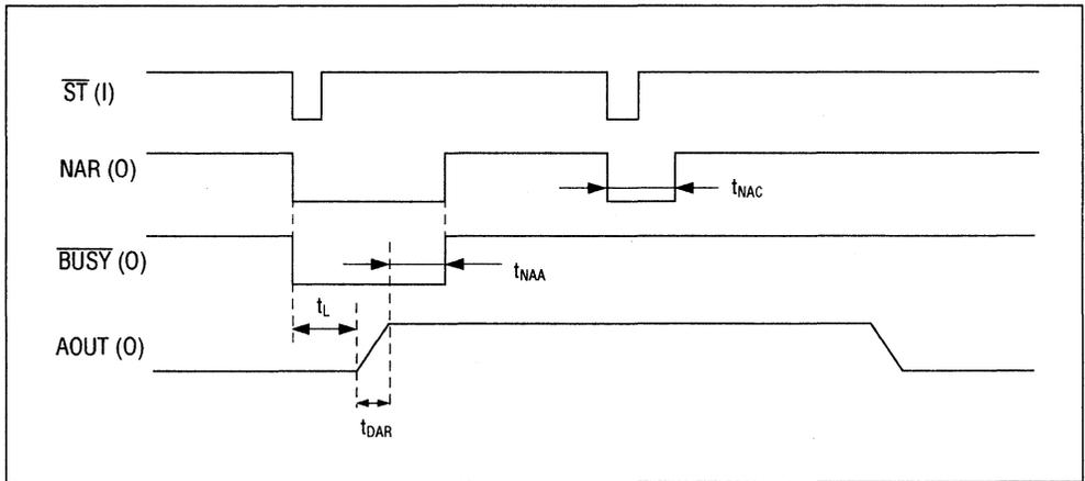
6. Timing Diagram of Echo Playback in Channel 1
