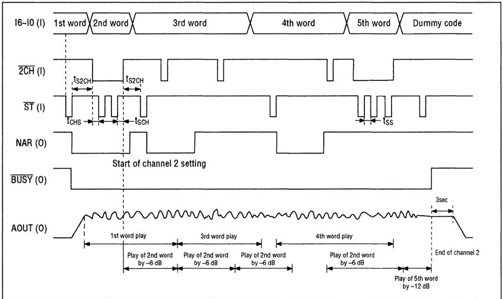
1. Channel 2 starts playing when the  $\overline{ST}$  pulse is input and  $\overline{2CH}="L"$ . The sounds volume can be changed by the number of the  $\overline{ST}$  pulses using the table below.
