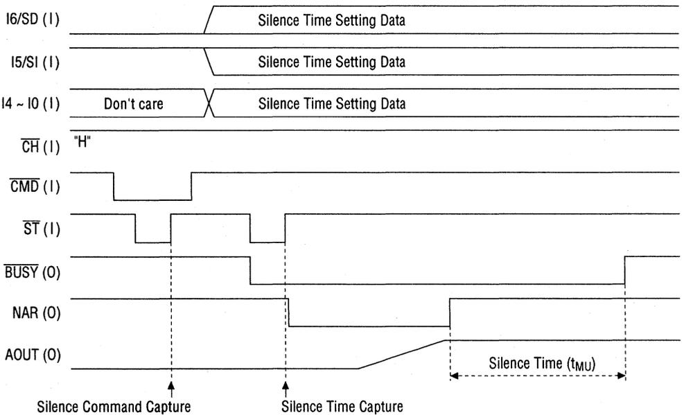
Figure 6.1 Channel 1 Silence Setting Timing (Parallel Input)
