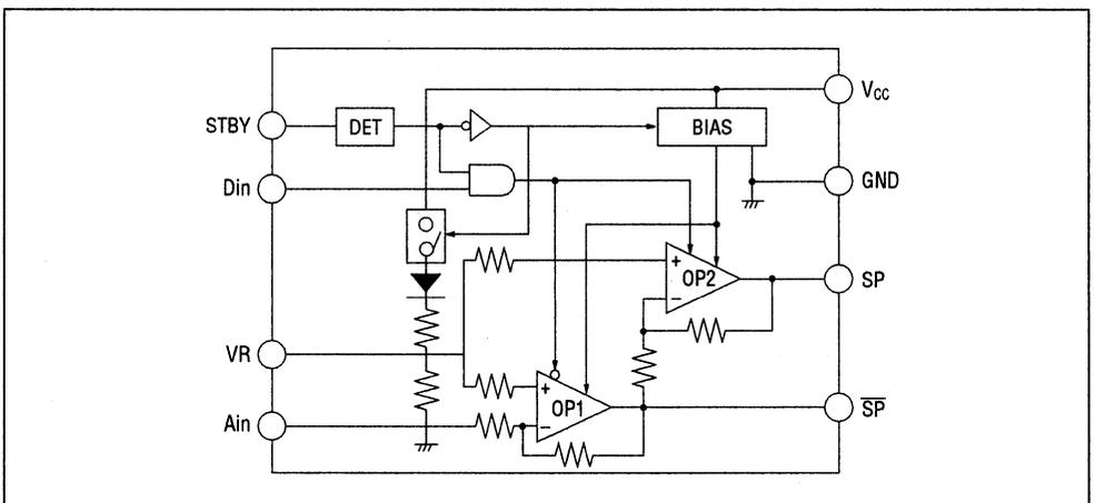
**Note:** MSC1191: Standby mode is activated by "H" level to the input STBY
