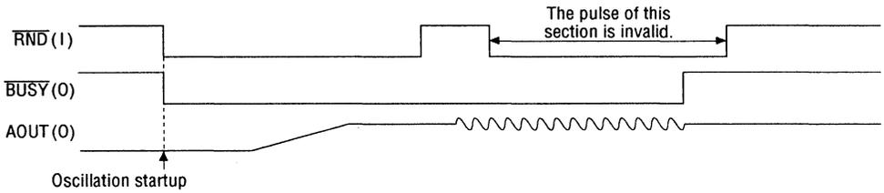
**Figure 4.7 Timing when a Pulse Is Input to the  $\overline{RND}$  Pin during Random Vocalization**
