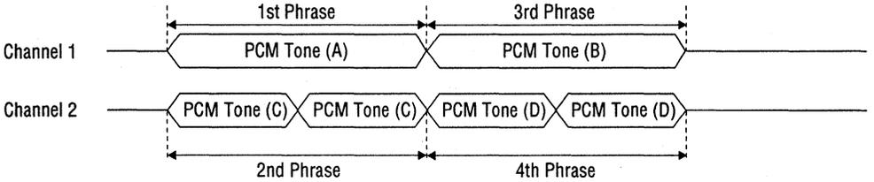
**Figure 9.10 Example of Channel Synthesis between PCM Main Melody Tone (A) (B) and PCM Rhythm Tone (C) (D) with 2 Repeats**
