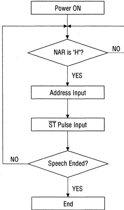
Figure 5.3 Input Flow Chart when Command is not set
