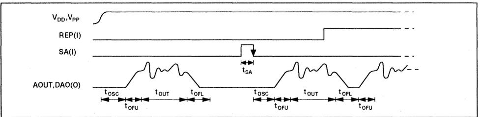
**Note:** When REP pin is merely set to "H" level, the speech is not output.
