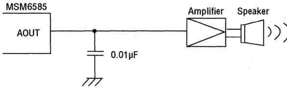
Even when the DAO pin is used, connect a 0.01µF capacitor to the AOUT pin. This capacitor is used for the improvement of a voice quality.
