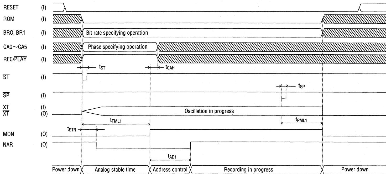
● Timing for Voice Activated Recording (PDMD Pin = Low)
