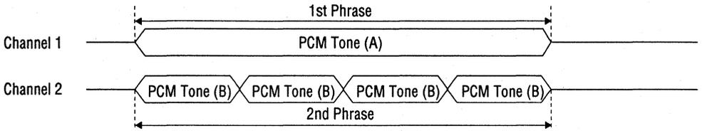
**Figure 12.9 Example of Channel Synthesis between PCM Main Melody Tone (A) and PCM Rhythm Tone (B) with 4 Repeats**
