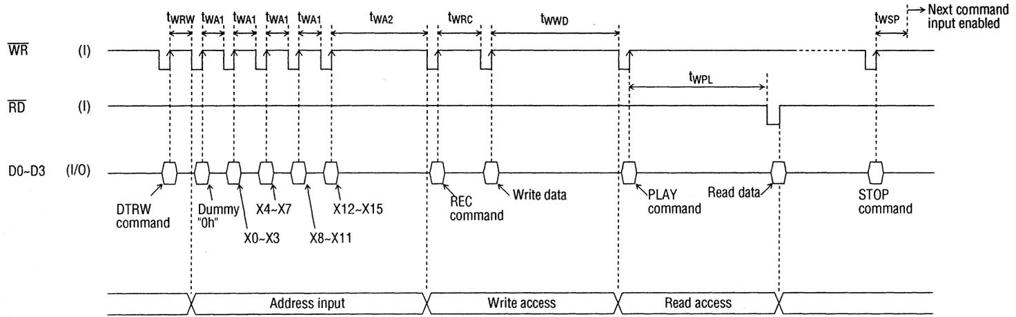
● Timing for Data Read by DTRD command
