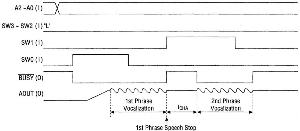
**Figure 5.4 Vocalization Timing when SW3~SW0 Are Changed during Vocalization**
