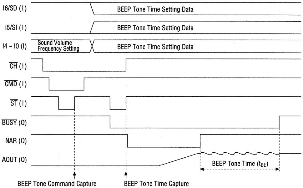
**Figure 6.4 BEEP Setting Timing (during Parallel Input)**
