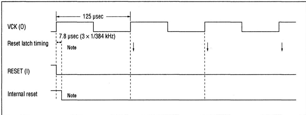
Figure 7 MSM5218 Reset Timing ( $f_{\text{sample}} = 8\text{kHz}$ )
