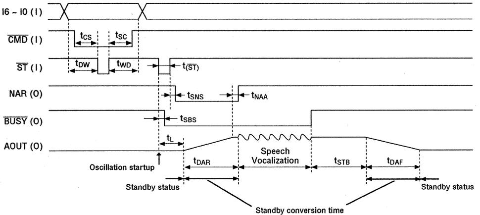
3. Channel 1 Regeneration Timing Chart when External Command Is Not Used (Parallel Input)
