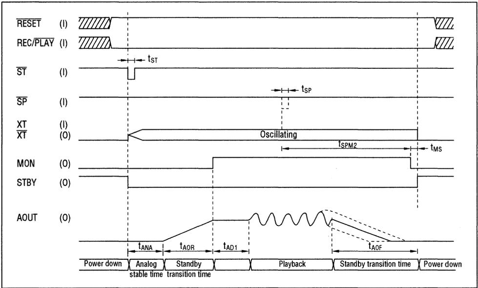
4. Timing during repeated playback (PDMD pin = "L")
