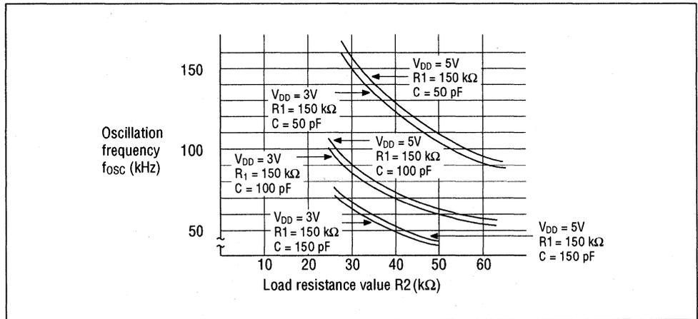
Figure 12 RC Oscillation Frequency Characteristics
