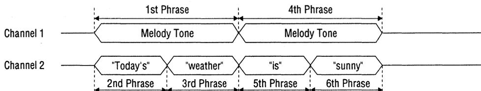
**Figure 12.8 Example of Four Phrase Channel Syntehsis Timing with Melody Tone and 1st and 4th Phrases as BGM**
