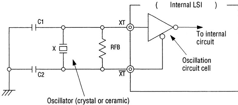
**Figure 1 Crystal/Ceramic Oscillation Circuit**
