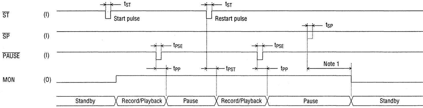
Note 1: This time interval varies depending on the state of PDMD pin and the record/playback mode and is one of  $t_{PMH1}$ ,  $t_{PMH2}$ ,  $t_{PMH3}$ ,  $t_{PML1}$ ,  $t_{PML2}$  and  $t_{PML3}$ .
