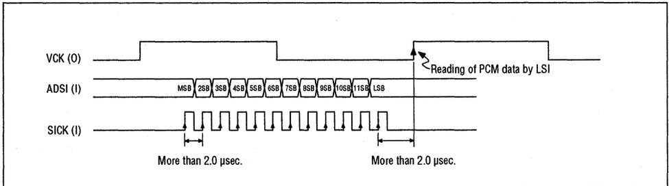
Figure 2-1 Use of External AD Converter and Timing
