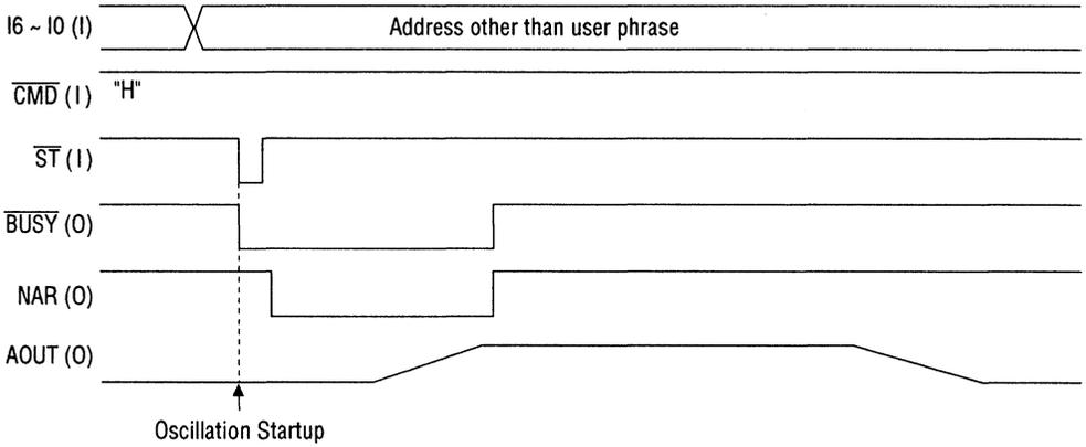
**Figure 7.2 Timing when Address, other than User Phrase, is Input in Standby Status**
