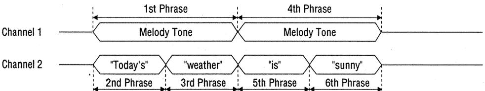
**Figure 10.8 Example of Four Phrase Channel Synthesis Timing with Melody Tone and 1st and 4th Phrases as BGM**
