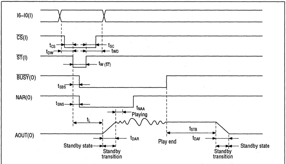
**3. Operation in channel 1 only (CPU input interface)**
