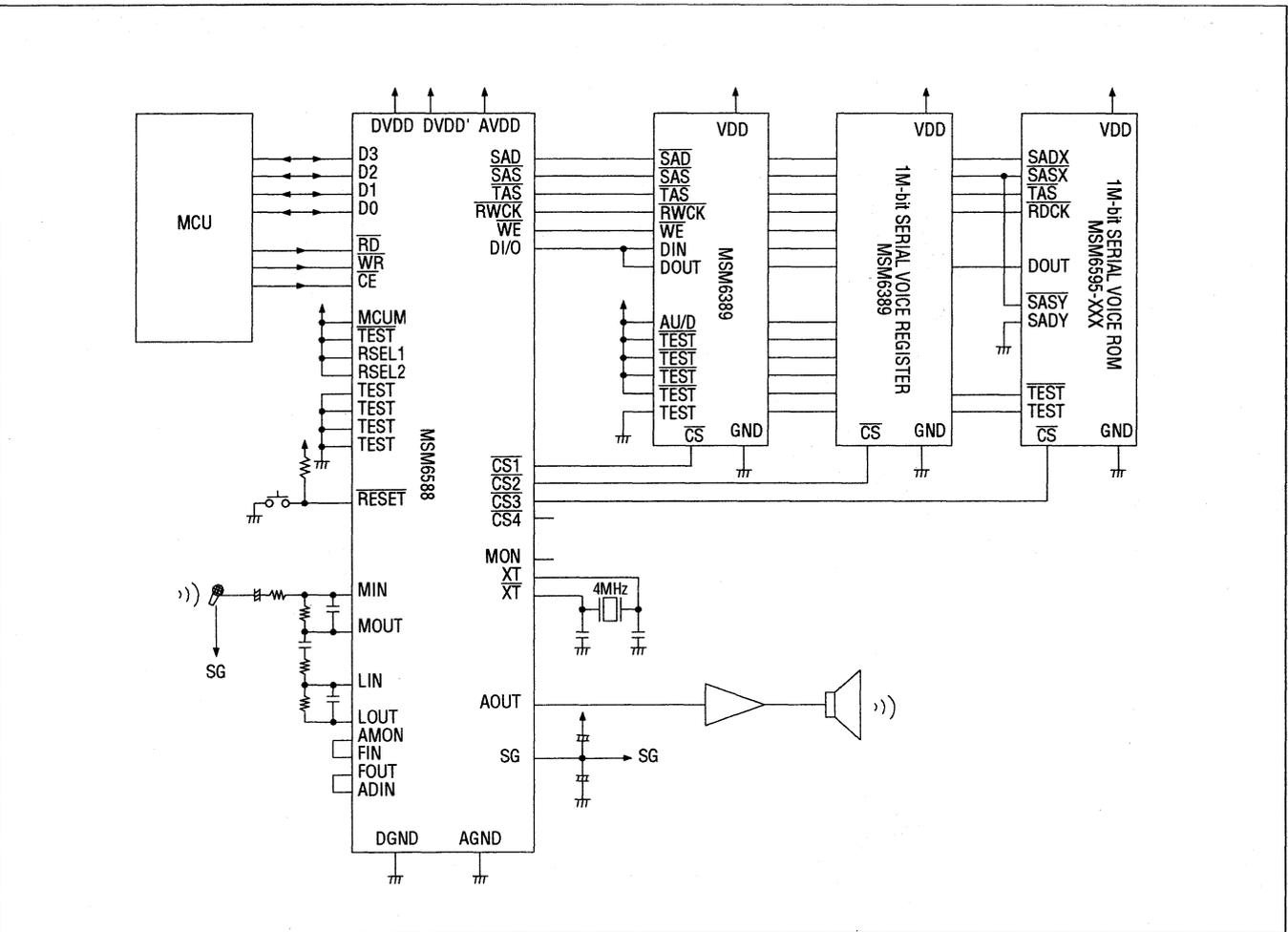
Note: MSM6588 cannot control only MSM6595-XXX without Serial Voice Register.
