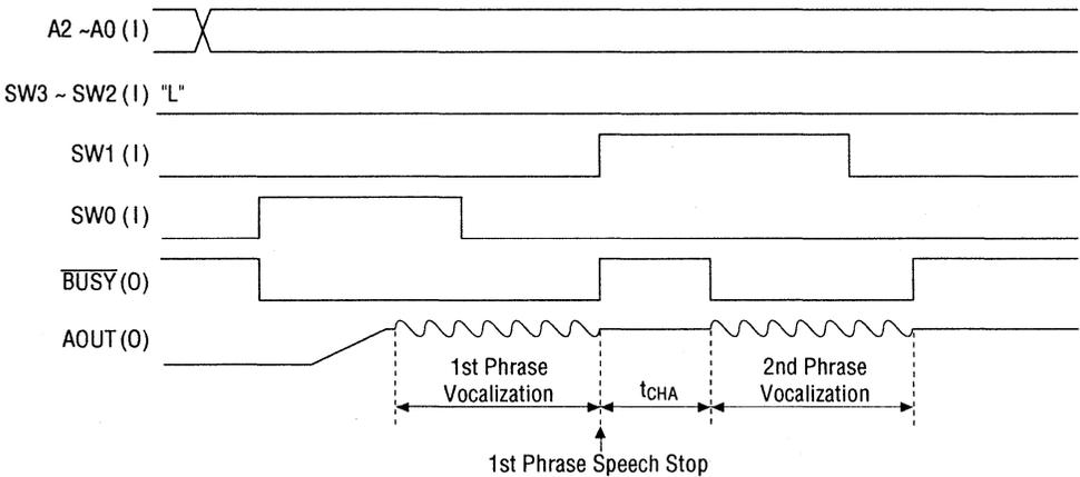
**Figure 4.4 Vocalization Timing when SW3~SW0 Are Changed during Vocalization**
