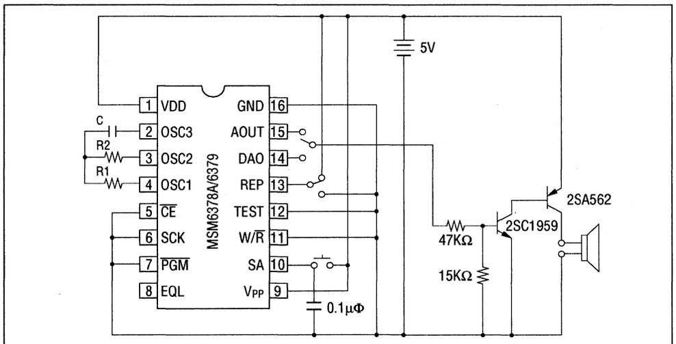
**Note:** If 5V or less is used, change the constant used to divide the resistor in the output stage.
