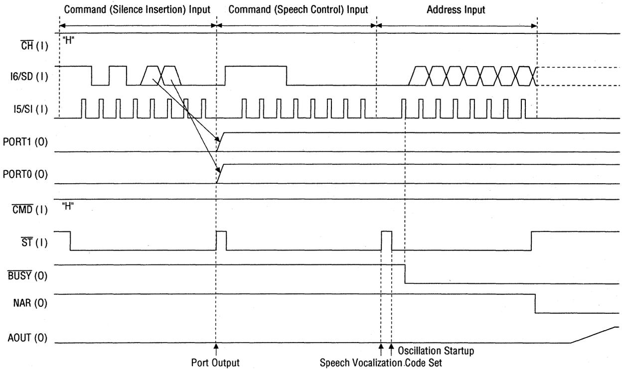
Figure 5.5 Port Output and Command, Address Setting Timing (during Serial Input)
