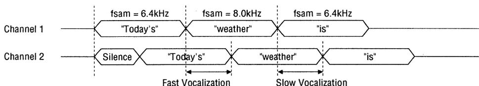
Figure 10.5 Vocalization Timing of Echo Regenerations with Different Sampling Frequencies
