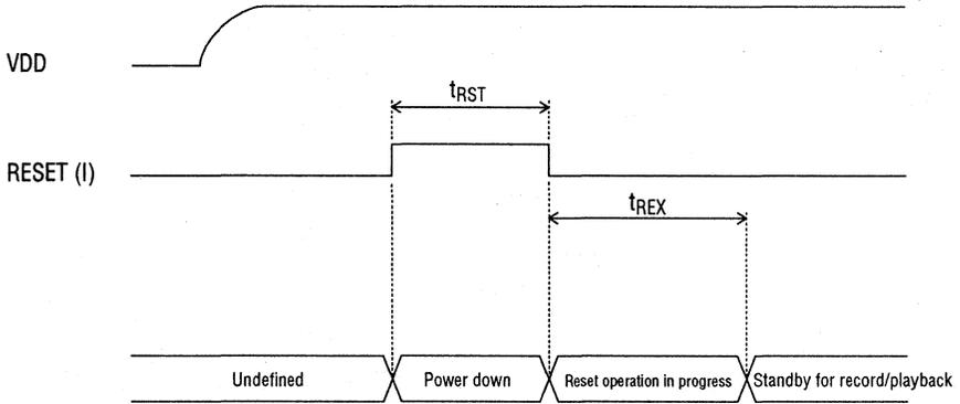
● Power Down by  $\overline{\text{PDWN}}$  Pin
