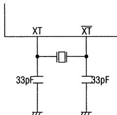
Figure 16.4 PBRC 4.00 MSA/MSK/MWS
