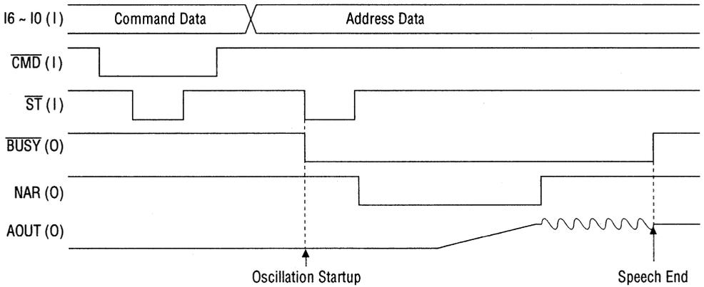
**Figure 4.1 Command, Address Input Timing (Parallel Input)**
