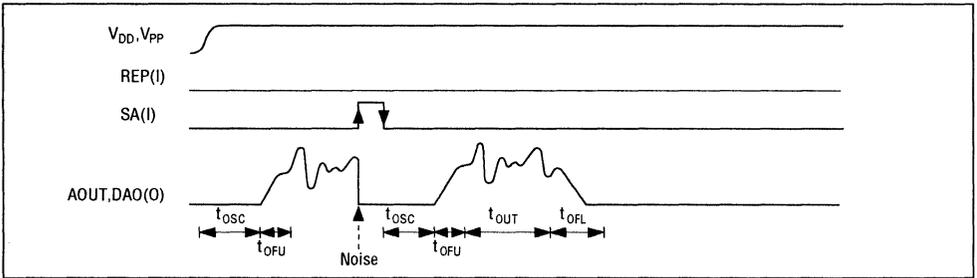
**Note:** When SA pin goes to "H" level during playback, speech is stopped and a noise is output.
