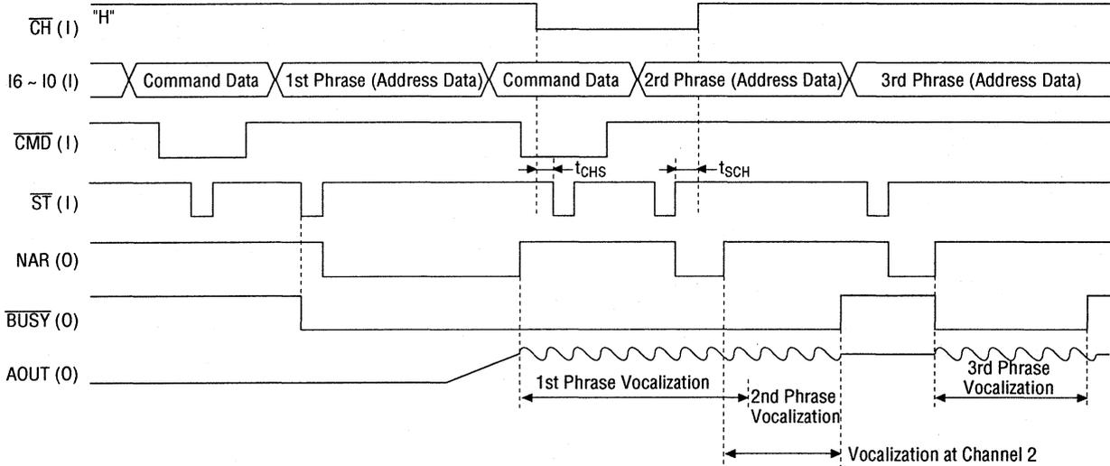
Since command data is maintained independently, If speech is started up at channel 1 without a command setting, speech is vocalized by the same command set at the 1st phrase.
