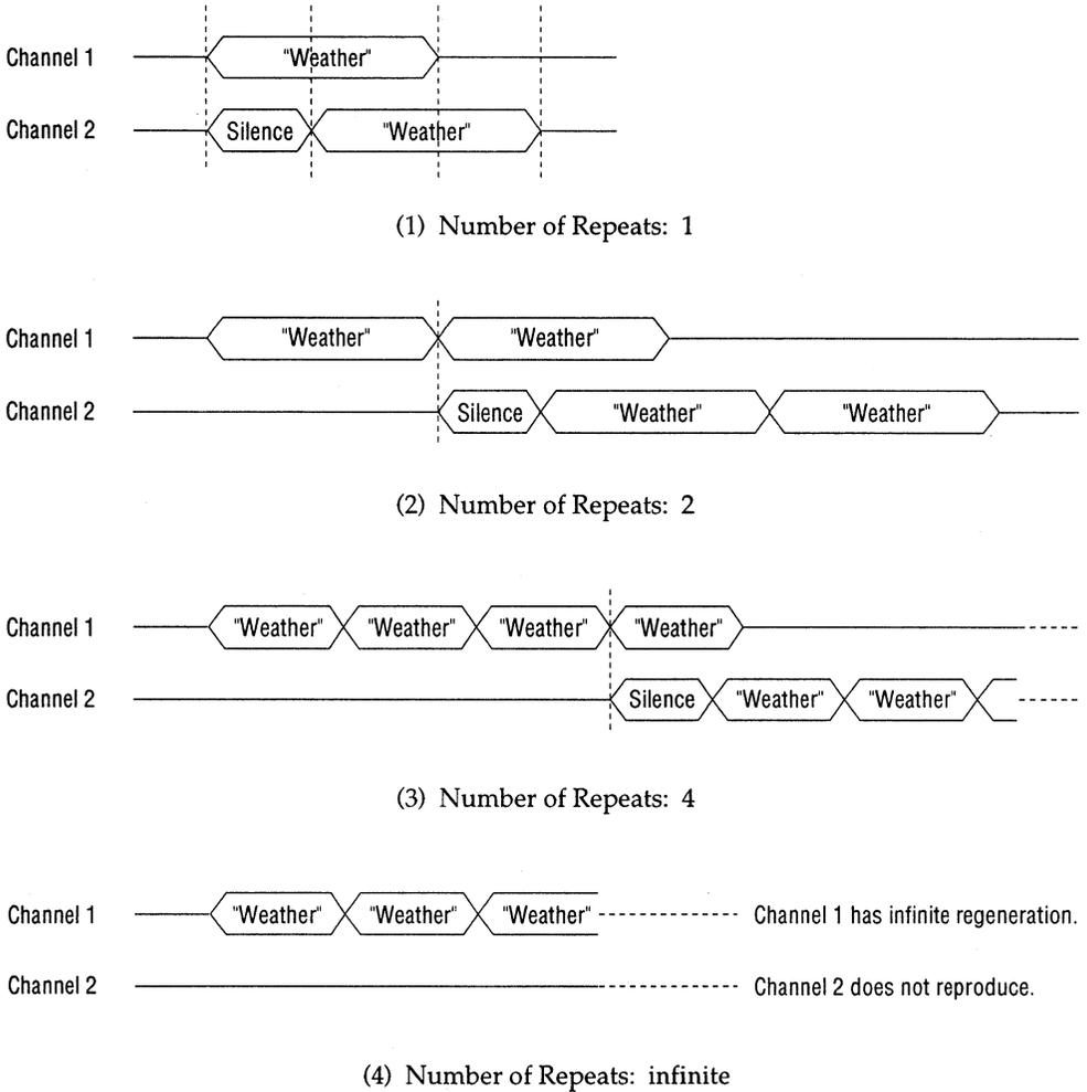
**Figure 9.3 Vocalization Timing of Echo Regeneration According to Number of Repeats**
