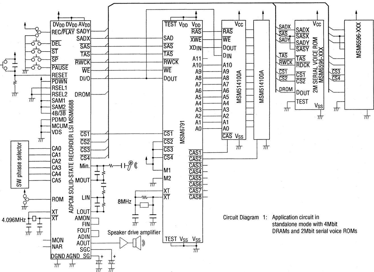
Circuit Diagram 1: Application circuit in standalone mode with 4Mbit DRAMs and 2Mbit serial voice ROMs
