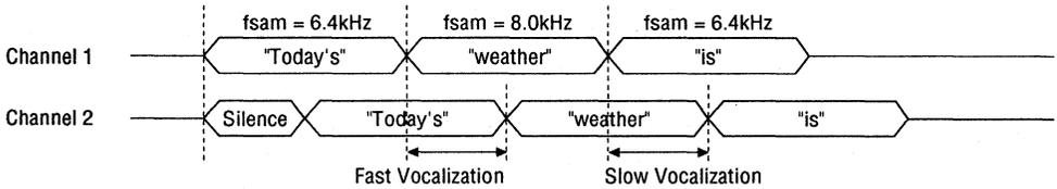
**Figure 13.5 Vocalization Timing of Echo Regenerations with Different Sampling Frequencies**
