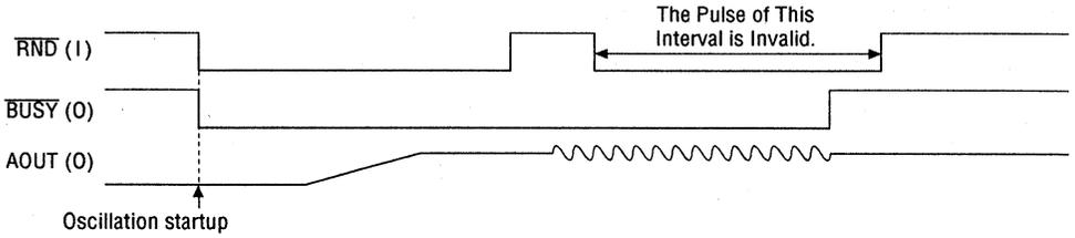
**Figure 5.7 Timing when a Pulse is Input to the  $\overline{\text{RND}}$  pin during Random Vocalization**
