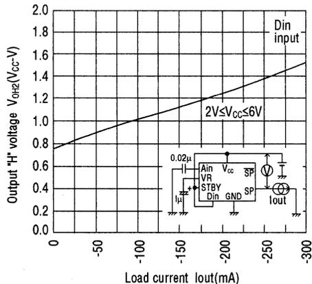
Output voltage vs load current (example)
