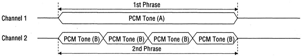
**Figure 9.9 Example of Channel Synthesis between PCM Main Melody Tone (A) and PCM Rhythm Tone (B) with 4 Repeats**
