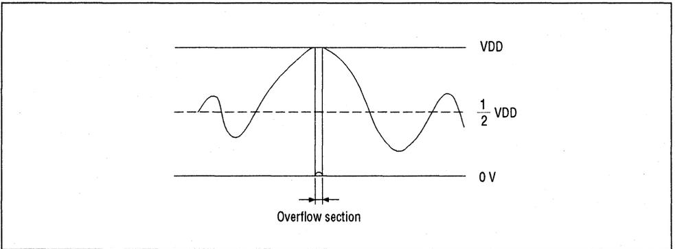
**Figure 5 Output Waveform When an Overflow Occurs**
