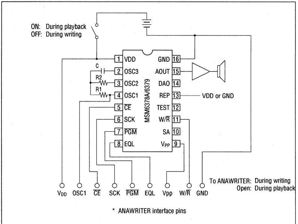
**Note:** \* Be careful about noise margin for input pins that are open during playback.
