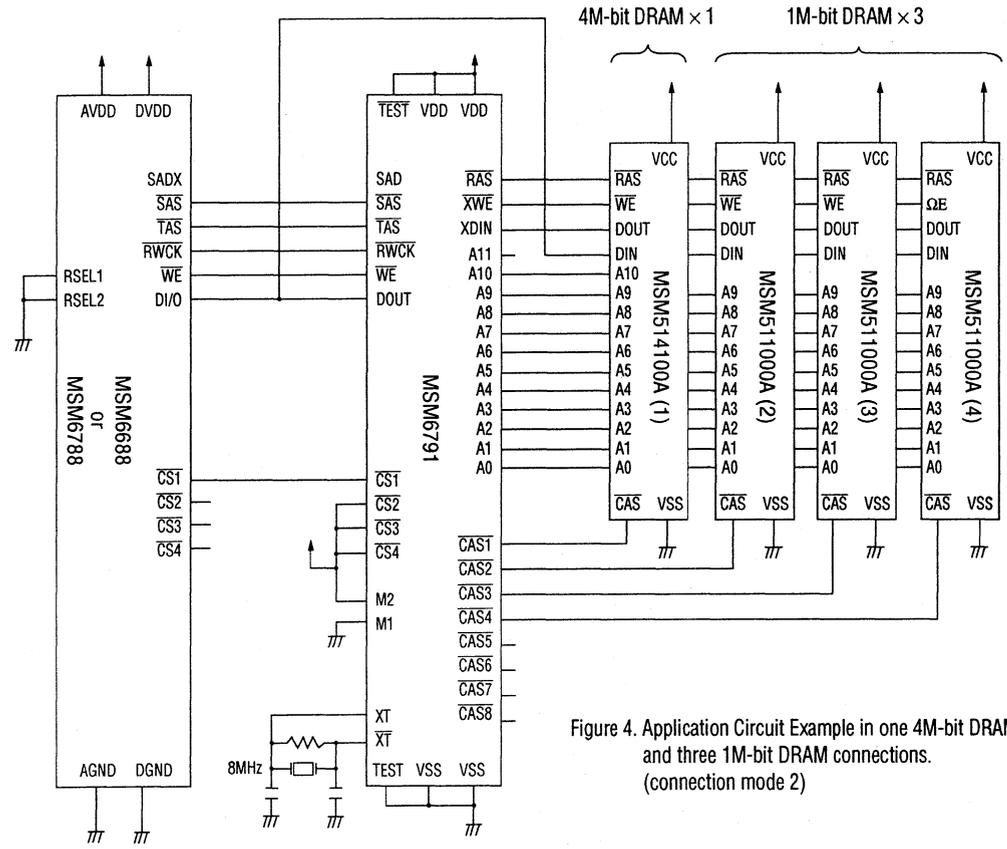
Figure 4. Application Circuit Example in one 4M-bit DRAM and three 1M-bit DRAM connections. (connection mode 2)
