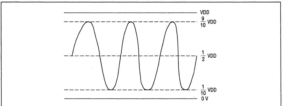
**Figure 6 Waveform When the Maximum Amplitude Level of the Input Waveform is about 80% of the Dynamic Range.**
