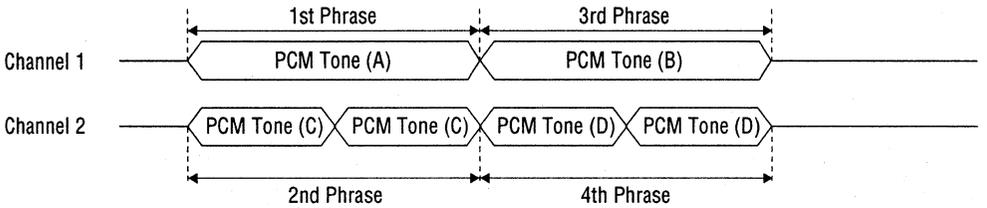
**Figure 13.10 Example of Channel Synthesis between PCM Main Melody Tone (A), (B) and PCM Rhythm Tone (C), (D) with 2 Repeats**
