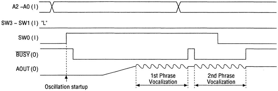
**Figure 4.3 Complete SW Input Interface Repeat Vocalization Timing**
