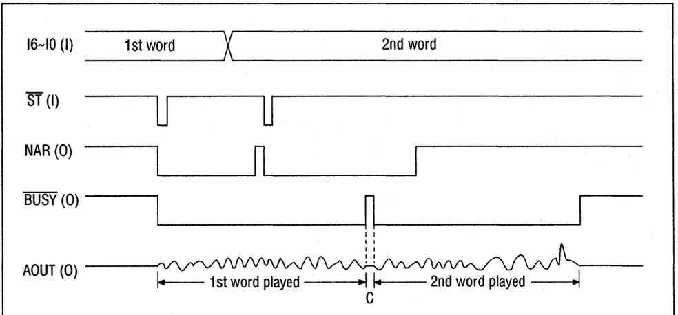
**Figure 1 Timing of CPU Interface ( $\overline{ST} \leq 350 \mu\text{s}$ )**
