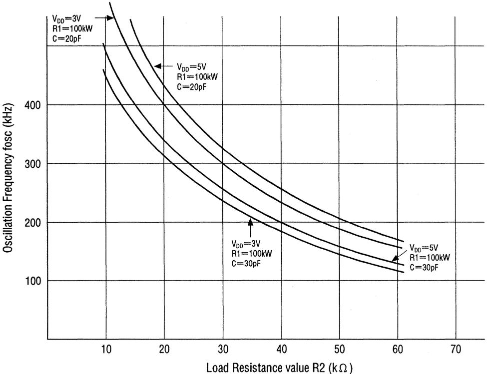
Figure 13.2 RC oscillation Frequency eharacteristics
