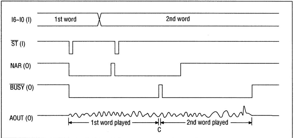
Figure 1 Timing of CPU Interface ( $\overline{ST} \leq 350 \mu s$ )
