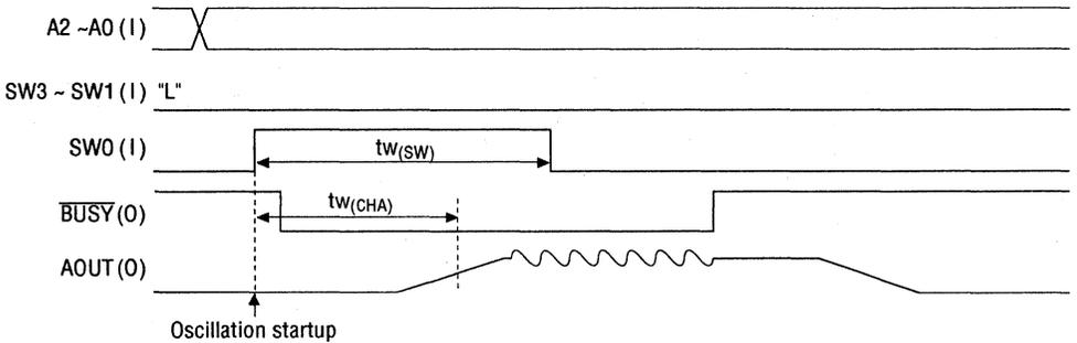
**Figure 4.1 Complete SW Input Interface 1 Phrase Vocalization Timing**
