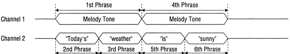
**Figure 9.8 Example of Four Phrase Channel Synthesis Timing with Melody Tone and 1st and 4th Phrases as BGM**
