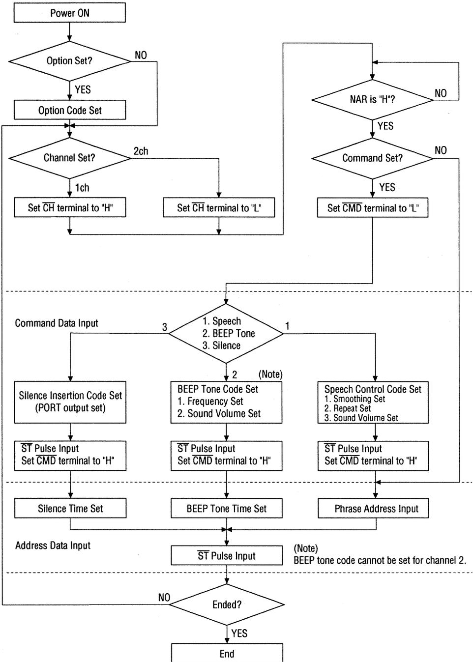
Figure 4.4 Parallel Input Flow Chart when External Command Is Used.
