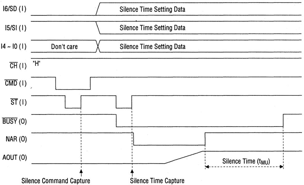
Figure 5.3 Channel 1 Silence Setting Timing (Parallel Input)
