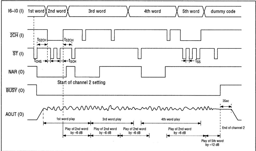
1. Channel 2 starts playing when the  $\overline{ST}$  pulse is input and  $2CH = "L"$ . The sound volume can be changed by the number of the  $\overline{ST}$  pulses using the table below.
