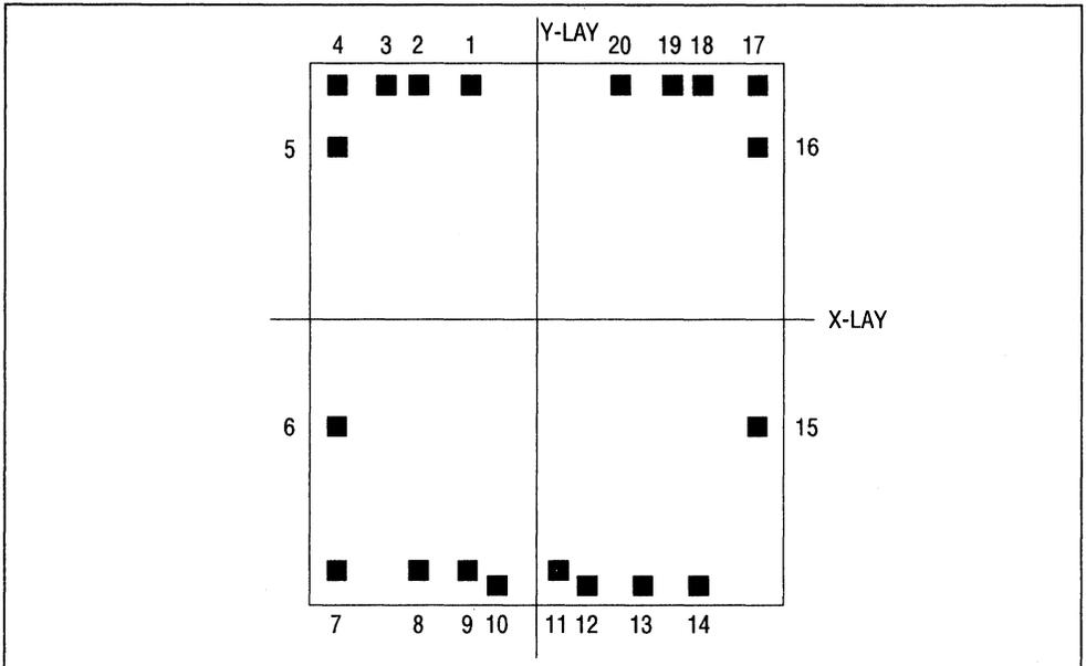
Pad Position (the die center is located at X=0, Y=0)
