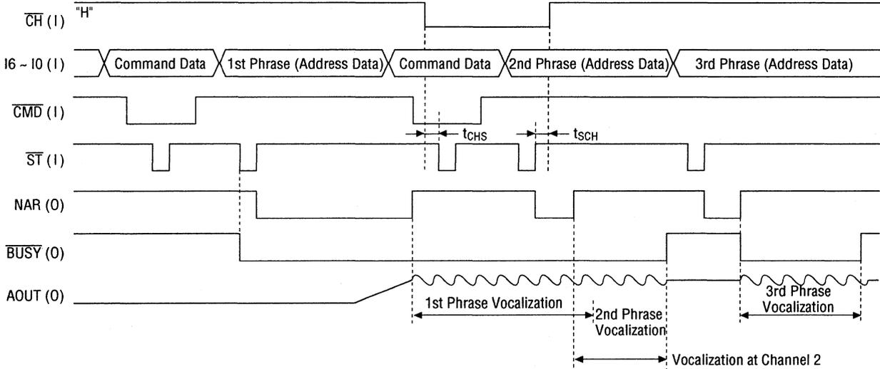
Since command data is maintained independently, if speech is started up at channel 1 without a command setting, speech is vocalized by the same command set at the 1st phase.
