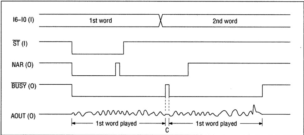
Figure 2 Timing of CPU Interface ( $\overline{ST} > 800 \mu\text{S}$ )
