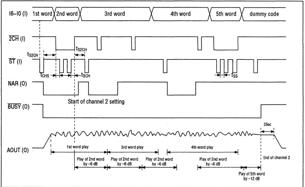
1. Channel 2 starts playing when the  $\overline{ST}$  pulse is input and  $2CH = "L"$ . The sound volume can be changed by the number of the  $\overline{ST}$  pulses using the table below.
