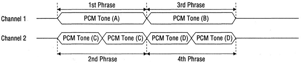
**Figure 12.10 Example of Channel Synthesis between PCM Main Melody Tone (A), (B) and PCM Rhythm Tone (C), (D) with 2 Repeats**
