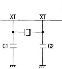
Figure 13.1 External circuit diagram
