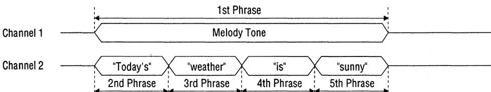
**Figure 12.7 Example of Four Phrase Channel Synthesis Timing with Melody Tone as GBM**
