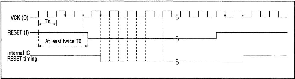
Figure 6 MSM5205 Reset Timing
