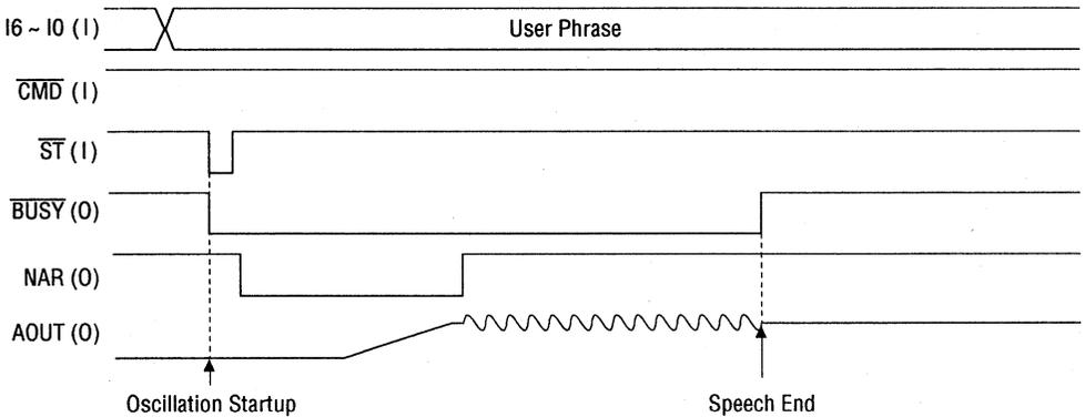
**Figure 6.1 Speech Startup Timing**
