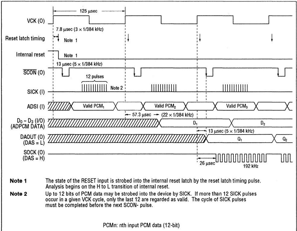
**SYNTHESIS ONLY ( $f_{\text{SAMPLE}} = 8 \text{ kHz}$ )**
