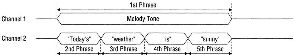
**Figure 9.7 Example of Four Phrase Channel Synthesis Timing with Melody Tone as BGM**
