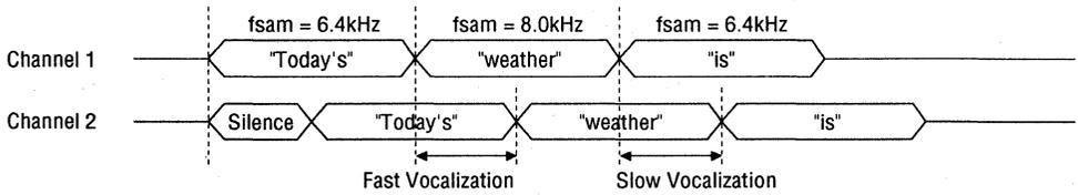
**Figure 9.5 Vocalization Timing of Echo Regenerations with Different Sampling Frequencies**
