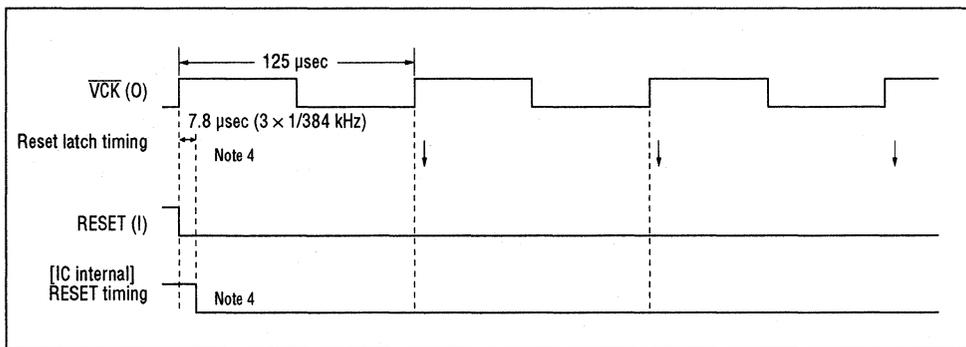
**Figure 9 MSM5218 Reset Timing (8 kHz Sampling Example)**
