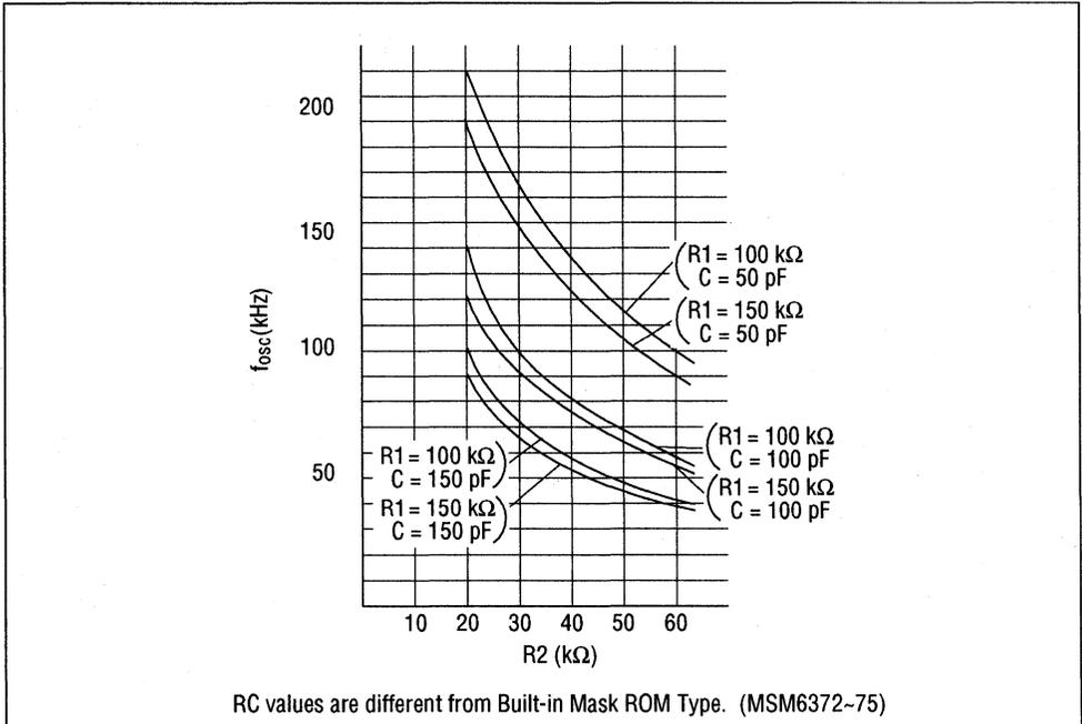
Figure 12 RC Oscillation Frequency
