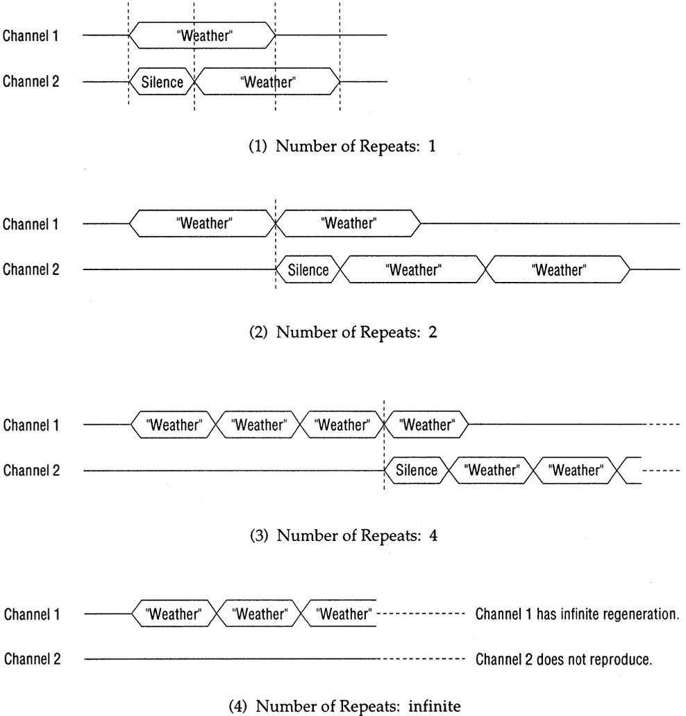
**Figure 13.3 Vocalization Timing of Echo Reproduction According to Number of Repeats**
