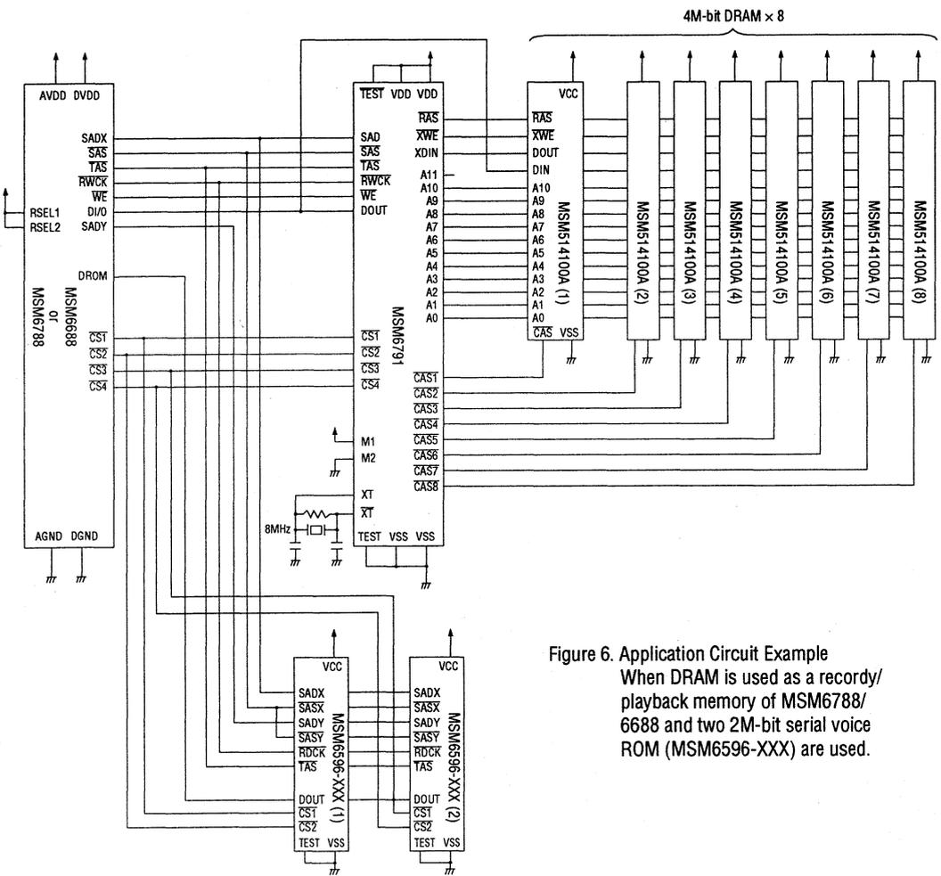
Figure 6. Application Circuit Example
