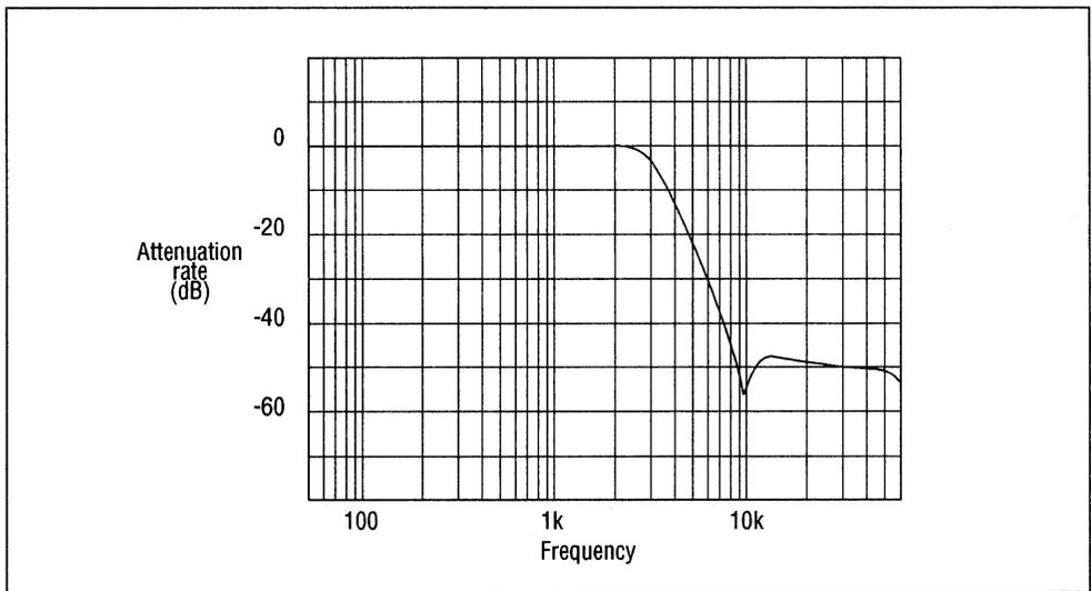
Figure 8 Low-pass Filter Characteristics ( $f_s=8\text{ kHz}$ )
