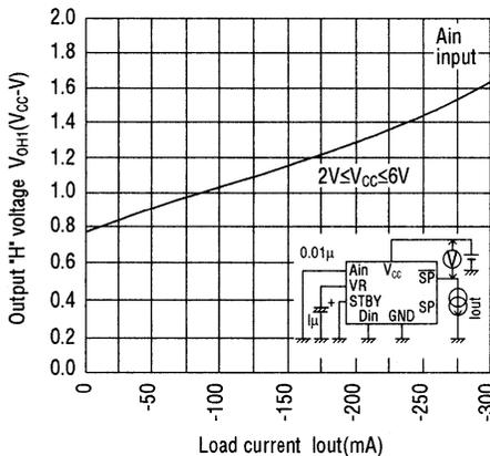
Output voltage vs load current (example)
