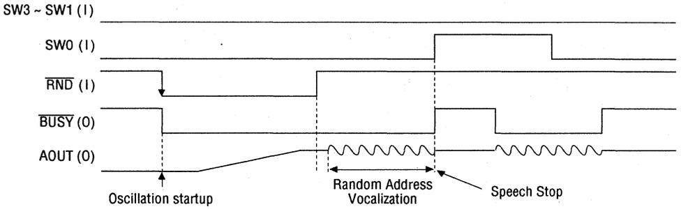
Figure 4.9 Timing when a Pulse Is Input to SW0 Pin during Random vocalization
