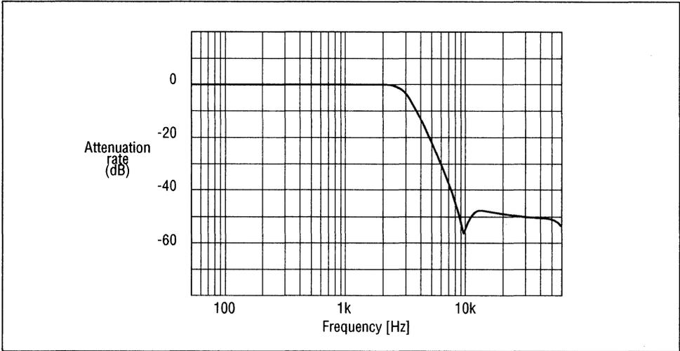
Figure 8 Low-pass Filter Characteristics ( $f_s=8\text{ kHz}$ )
