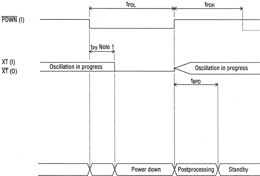
**Note 1:** When an external clock is used, continue to apply the clock input to the XT terminal during  $t_{\text{PX}}$  after the  $\overline{\text{PDWN}}$  pin is set to a low level.
