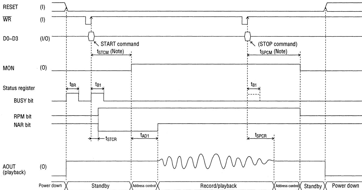
**Note:**  $t_{STCM}$  and  $t_{SPCM}$  vary depending on the control mode for record/playback and on record or playback mode.
