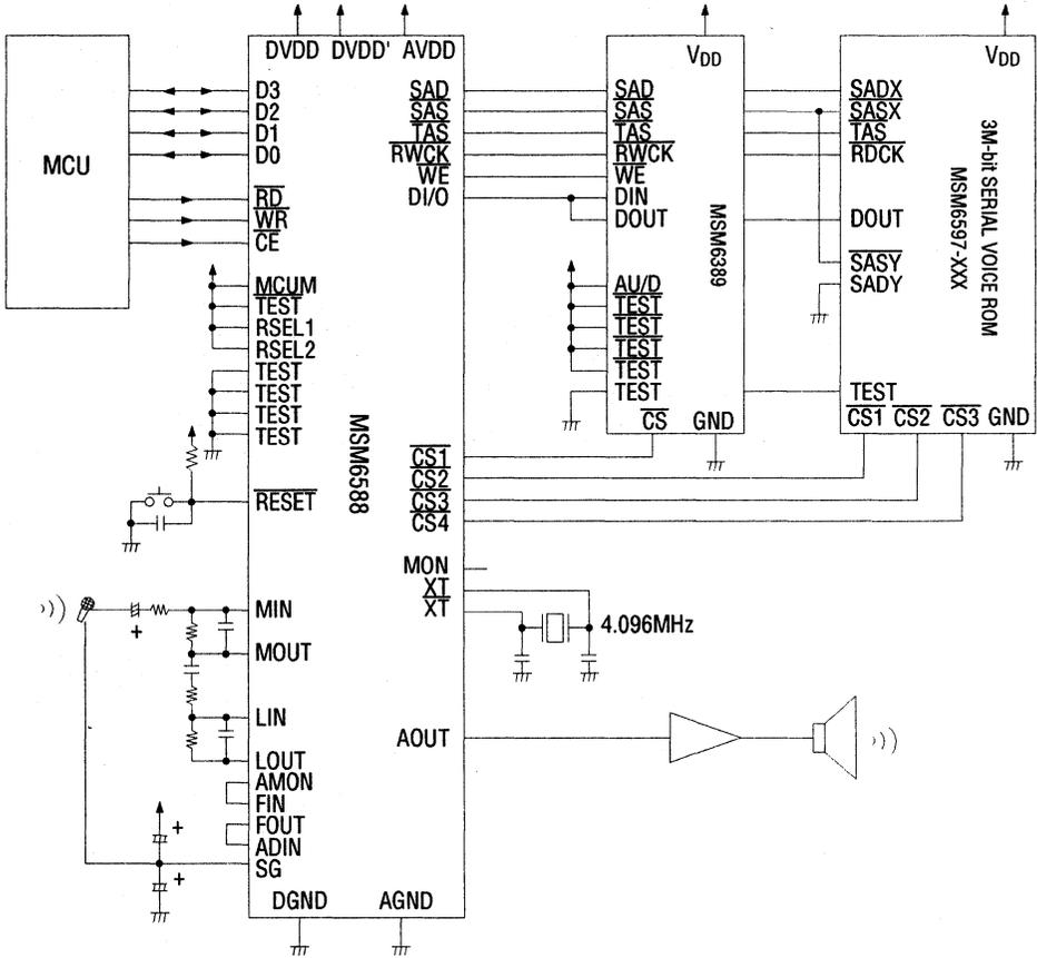
**Note:** When MSM6597 is driven by MSM6388 or MSM6588, a serial register is required.
