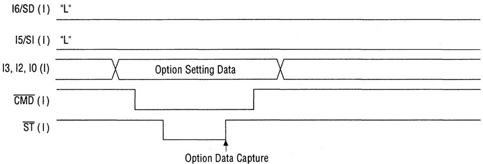
**Figure 4.1 Option Setting Timing (during Parallel Input)**
