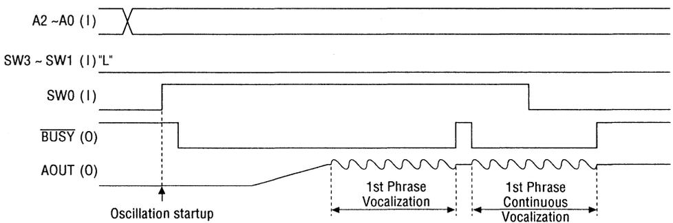
Figure 5.2 Complete SW Input Interface Repeat Vocalization Timing
