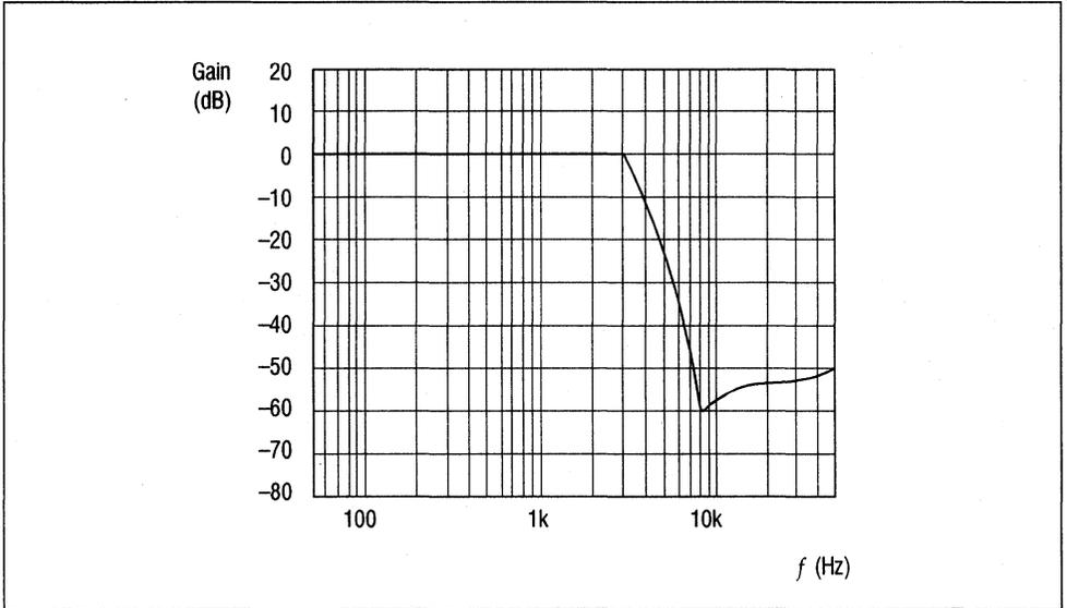
**LPF Frequency Characteristics ( $f_{\text{sam}} = 8.0 \text{ kHz}$ )**
