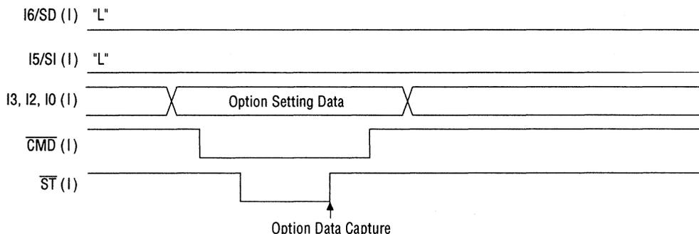
**Figure 3.1 Option Setting Timing (during Parallel Input)**
