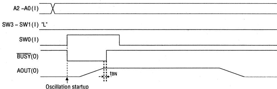
**Figure 4.5 Timing when Speech Is Started up at an Address other than the User-Specified Phrase**
