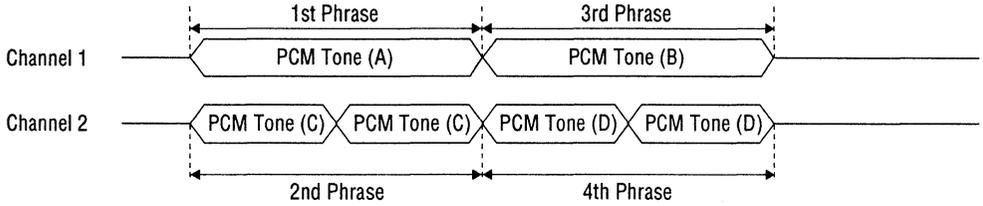
**Figure 10.10 Example of Channel Synthesis between PCM Main Melody Tone (A) (B) and PCM Rhythm Tone (C) (D) with 2 Repeats**
