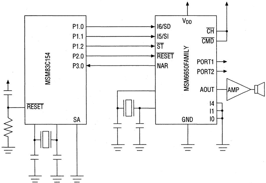
Example of Application Circuit at Serial Input Interface
