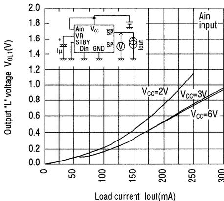
Output voltage vs load current (example)
