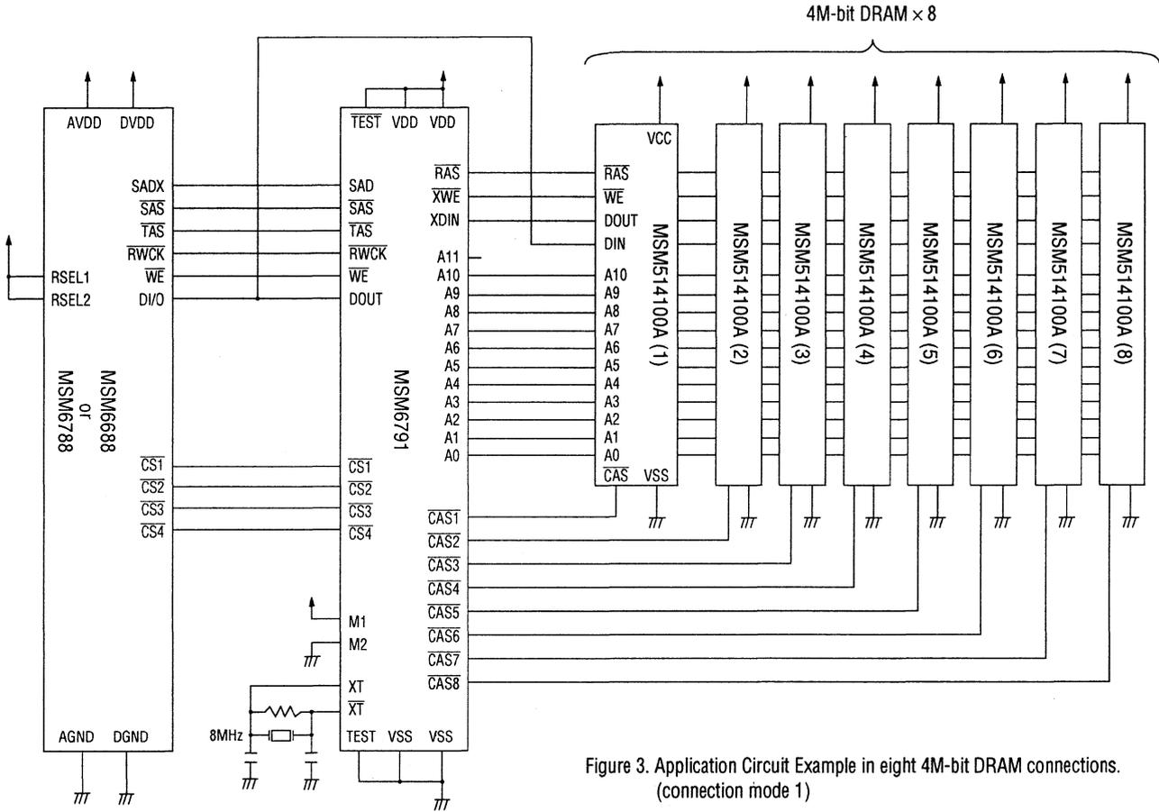
Figure 3. Application Circuit Example in eight 4M-bit DRAM connections. (connection mode 1)
