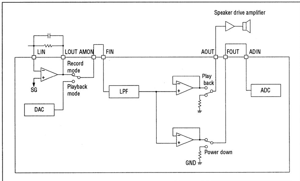
**Note:** Switches in the figure denote the state during record operation.
