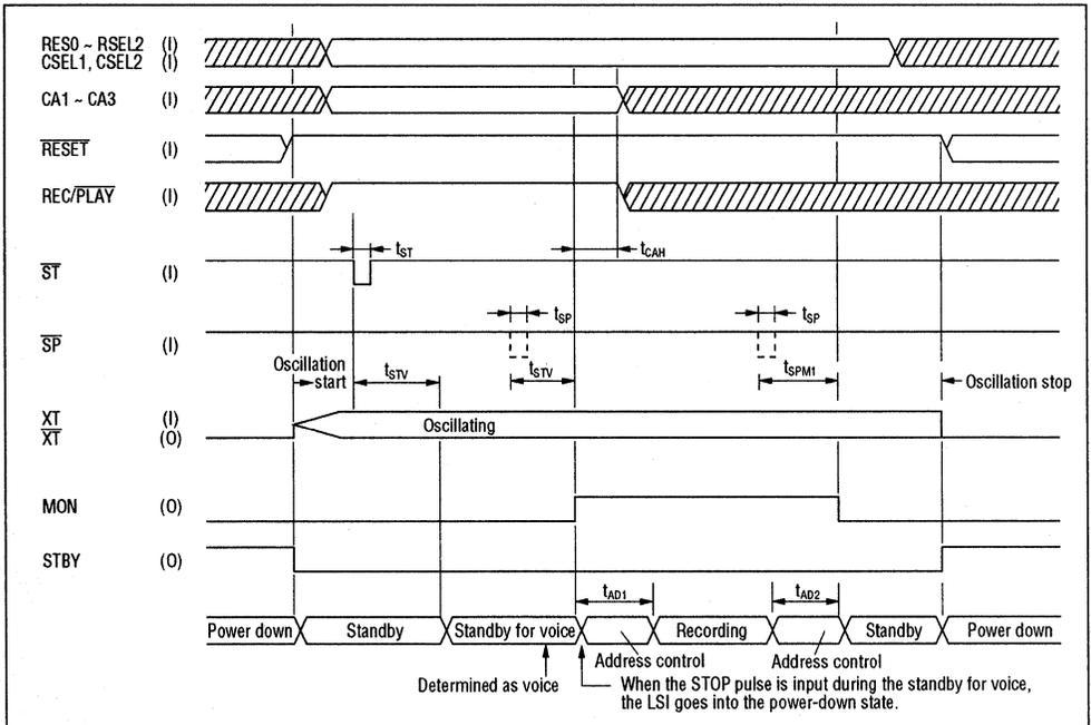
7. Timing during playback (PDMD pin = "H")
