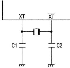
Figure 16.1 External circuit diagram
