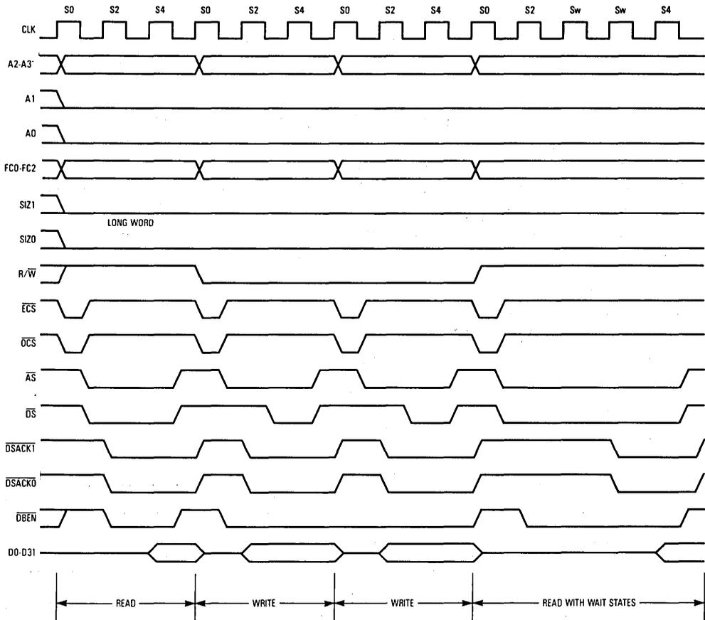
Figure 7-25. Asynchronous Read-Write-Read Cycles — 32-Bit Port
