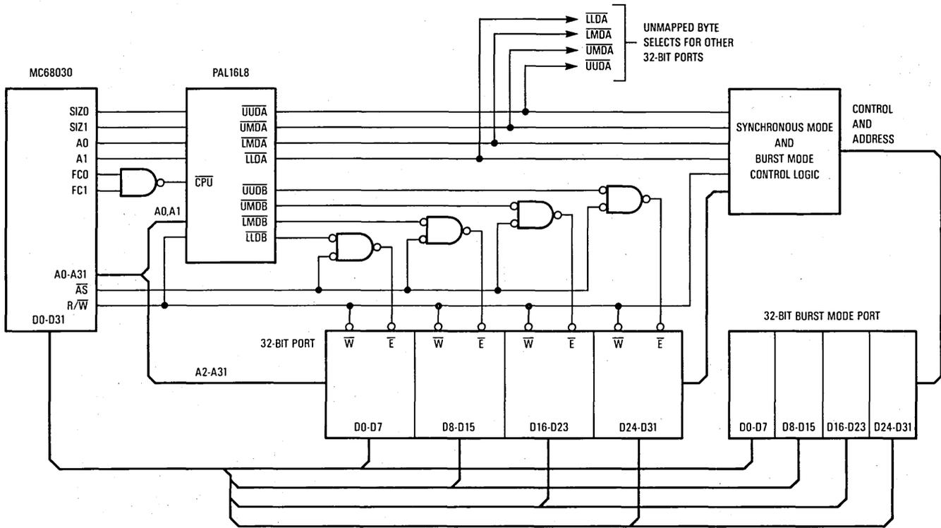
Figure 12-6. Example MC68030 Byte Select PAL System Configuration
