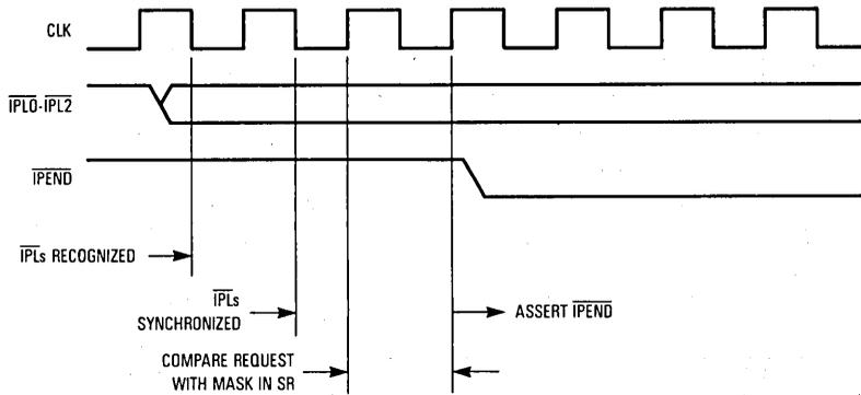
Figure 8-4. Assertion of  $\overline{IPEND}$
