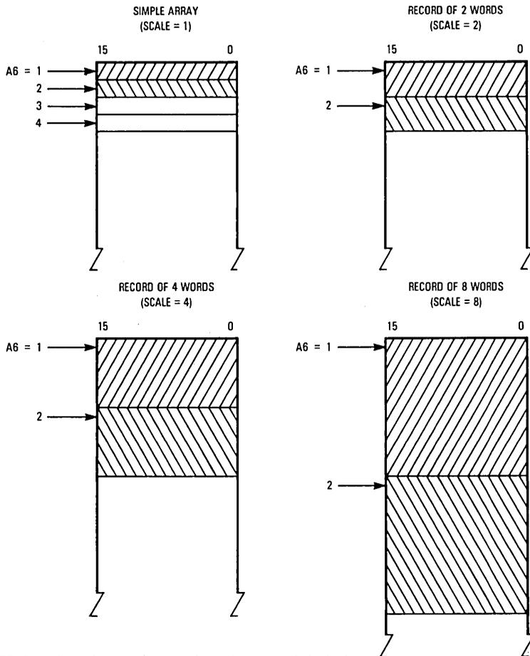
NOTE: Regardless of array structure, software increments index by the appropriate amount to point to next record.
