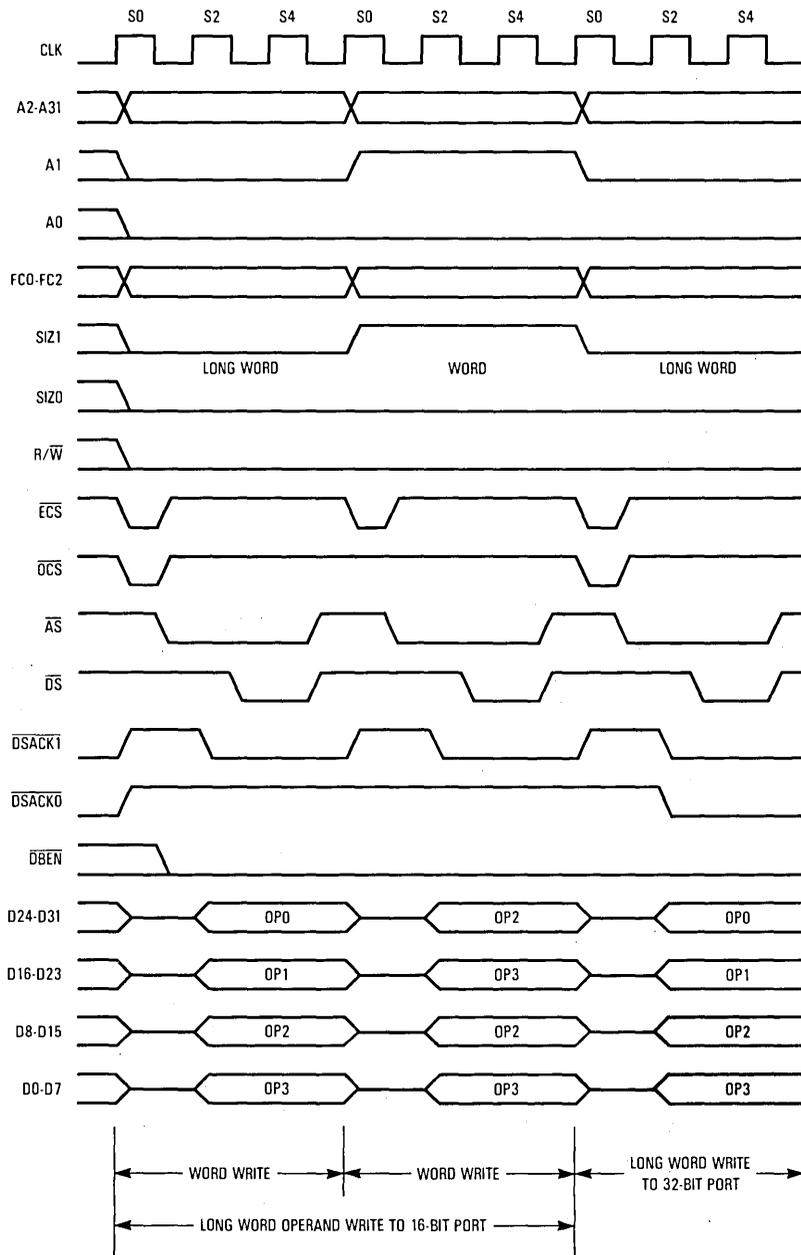
Figure 7-28. Long-Word Operand Write — 16-Bit Port
