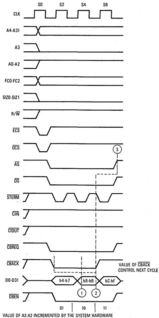
Figure 7-39. Long-Word Operand Request from \$07 with Burst Request —  $\overline{\text{CBACK}}$  Negated Early
