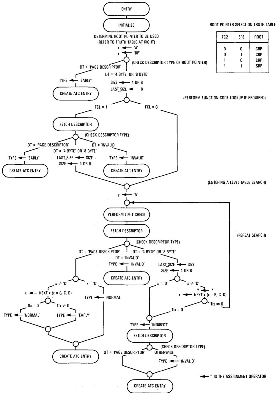
**Figure 9-25. Detailed Flowchart of MMU Table Search Operation**
