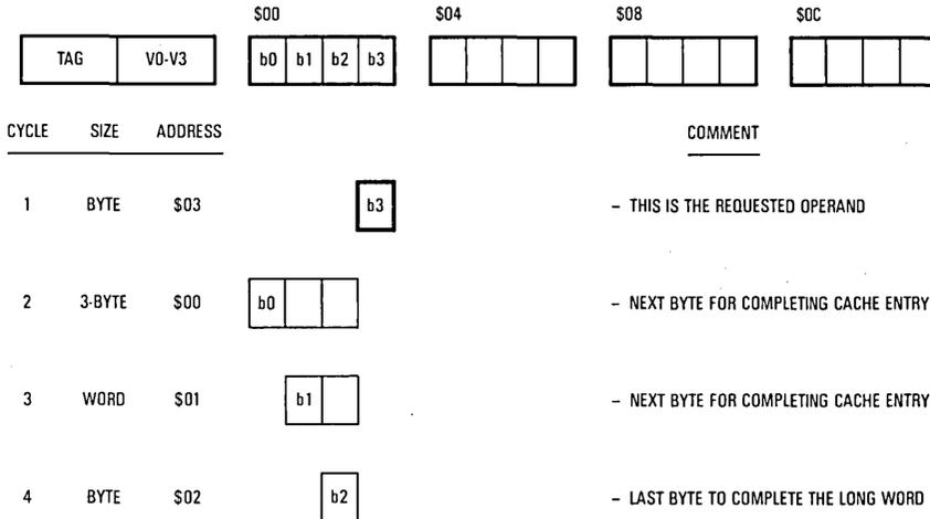
Figure 6-5. Single Entry Mode Operation — 8-Bit Port
