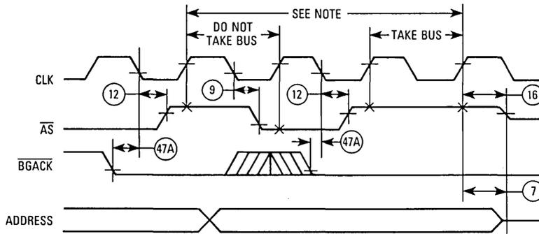
**NOTE:** The alternate bus master must sample  $\overline{AS}$  high on two consecutive rising edges of the clock (after  $\overline{BGACK}$  is recognized low) before taking the bus.
