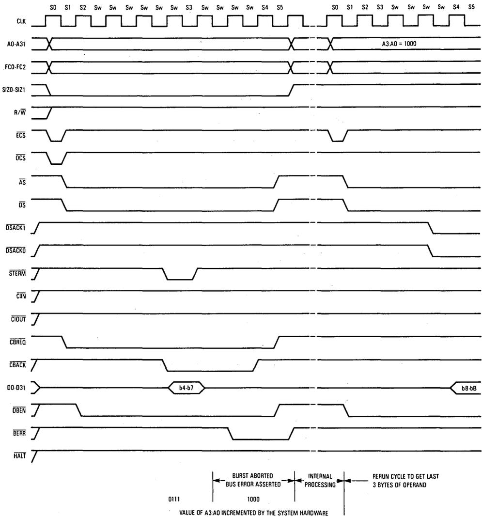
Figure 7-53. Long-Word Operand Request —  $\overline{\text{BERR}}$  on Second Access
