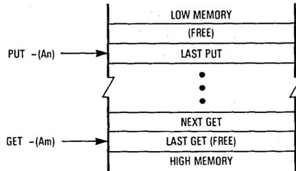
To implement the queue as a circular buffer, the "get" or "put" operation should be performed first, and then the relevant address register should be checked and adjusted, if necessary. The address register is adjusted by adding the buffer length (in bytes) to the register contents.
