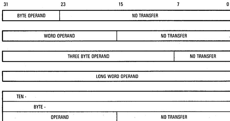
Figure 10-21. Operand Alignment for Operand CIR Accesses
