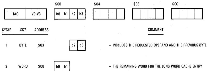
**Figure 6-6. Single Entry Mode Operation — 16-Bit Port**
