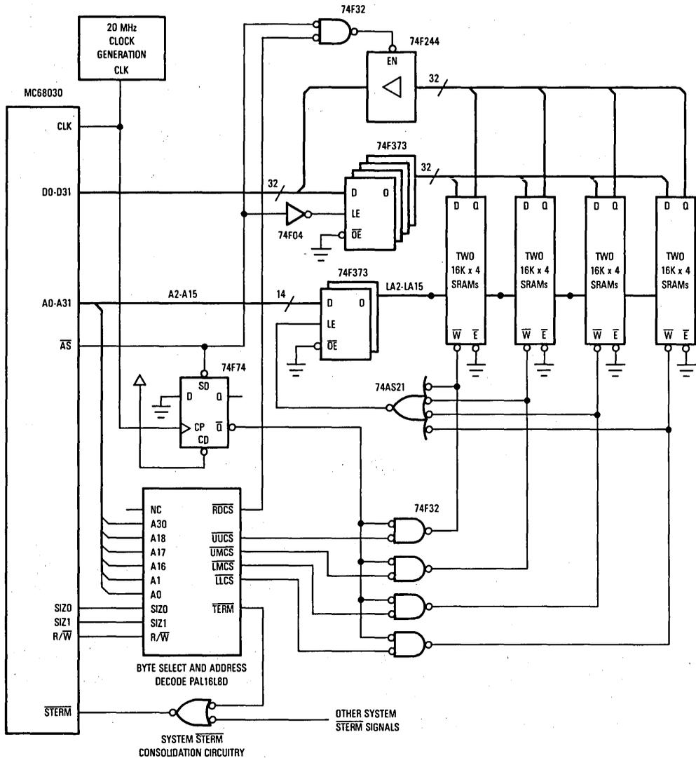
Figure 12-12. Example Two-Clock Read and Write Memory Bank
