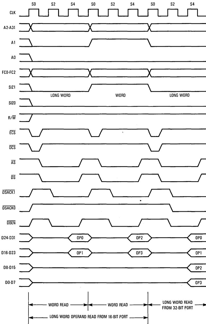
Figure 7-23. Long-Word Read — 16-Bit and 32-Bit Port
