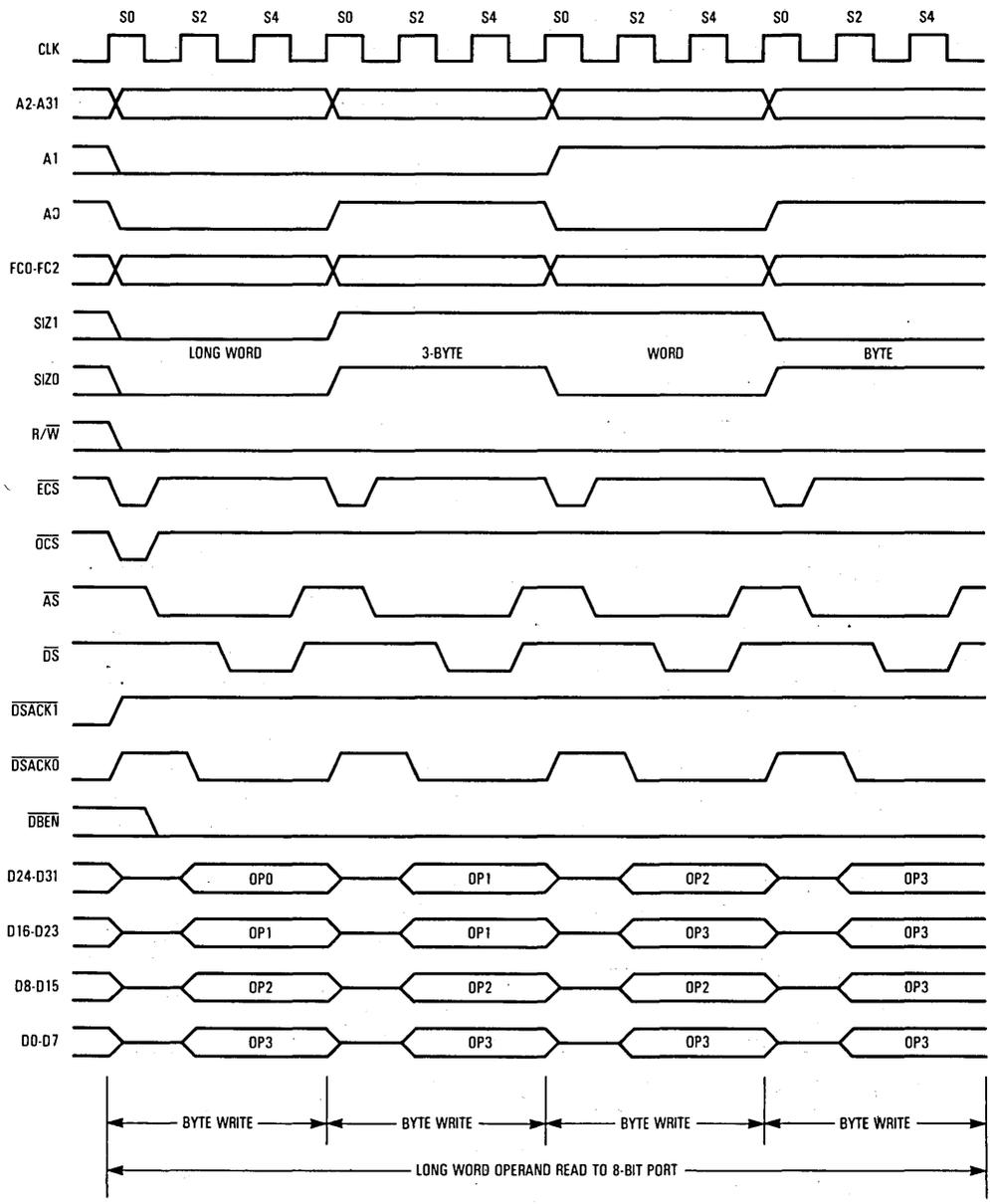
Figure 7-27. Long-Word Operand Write — 8-Bit Port
