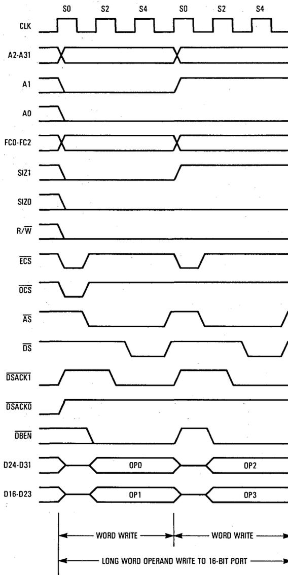
Figure 7-6. Long-Word Operand Write Timing (16-Bit Data Port)
