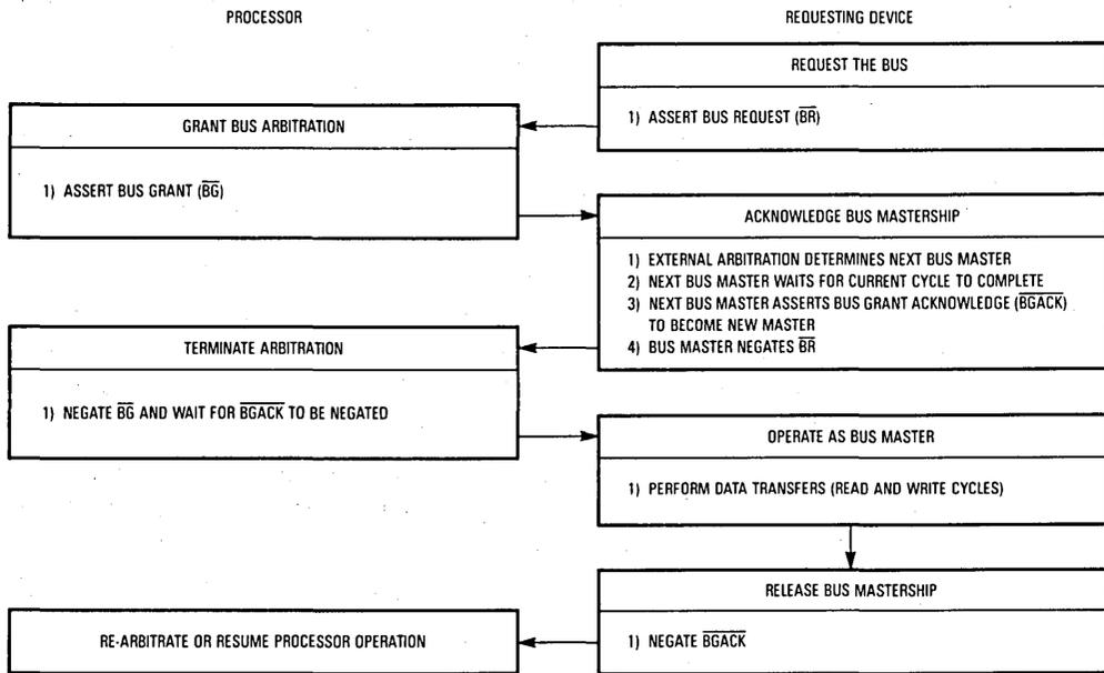
Figure 7-59. Bus Arbitration Flowchart for Single Request
