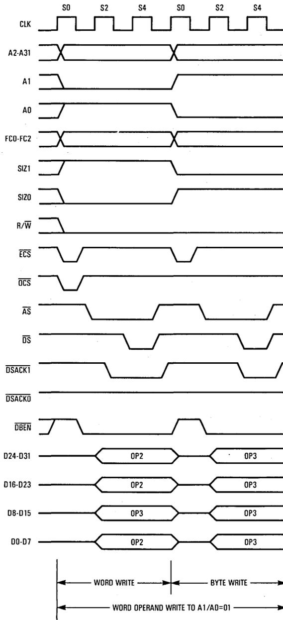
Figure 7-13. Misaligned Word Transfer to Word Port
