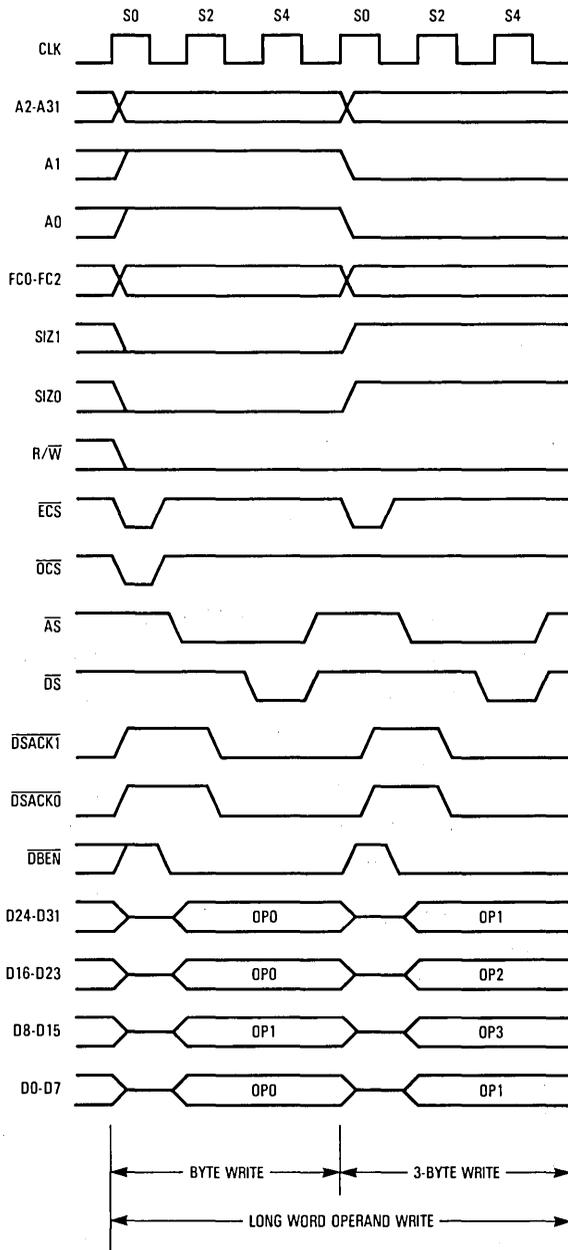
Figure 7-16. Misaligned Write Cycles to Long-Word Port
