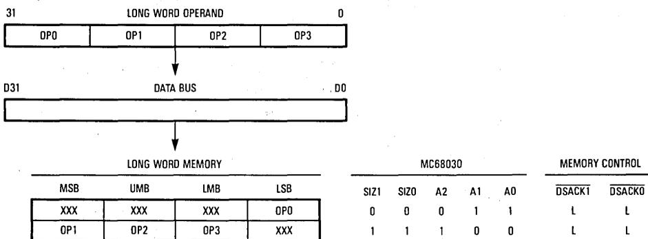
Figure 7-15. Misaligned Long-Word Transfer to Long-Word Port
