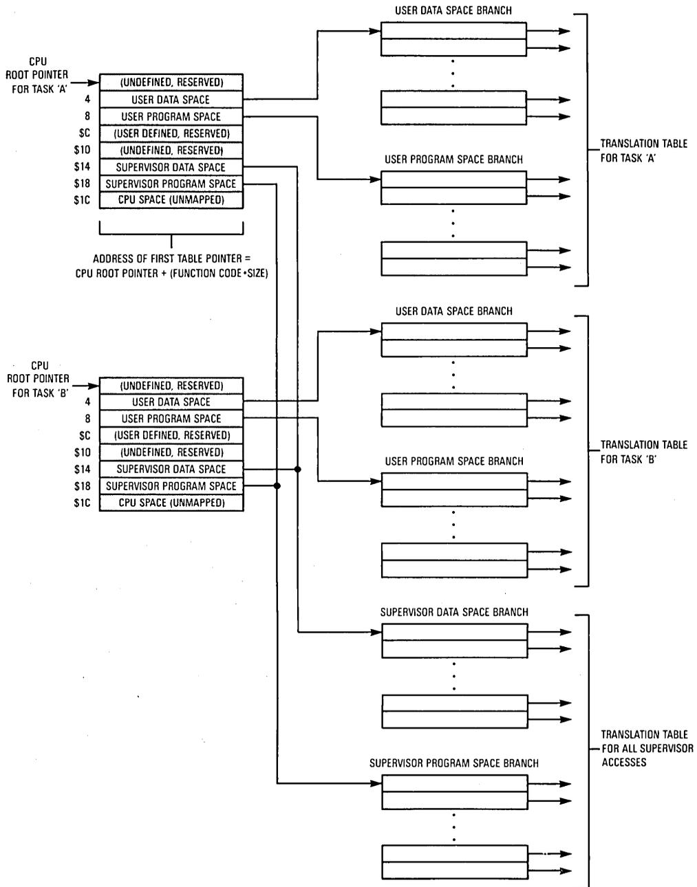
Figure 9-32. Example Translation Tree Structure for Two Tasks
