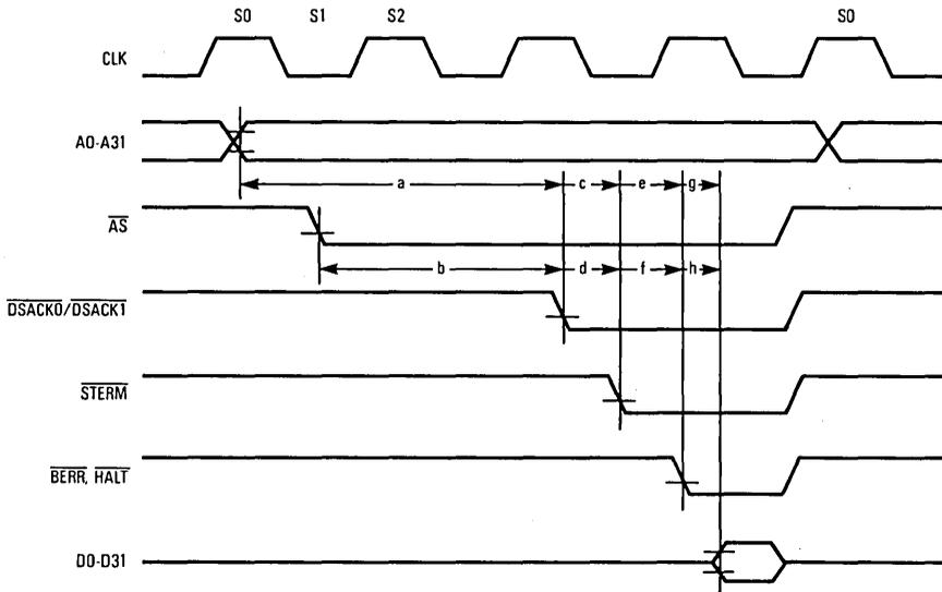
NOTE: This diagram illustrates access time calculations only.  $\overline{DSACK0}/\overline{DSACK1}$  and  $\overline{STERM}$  should never be asserted together during the same bus cycle.
