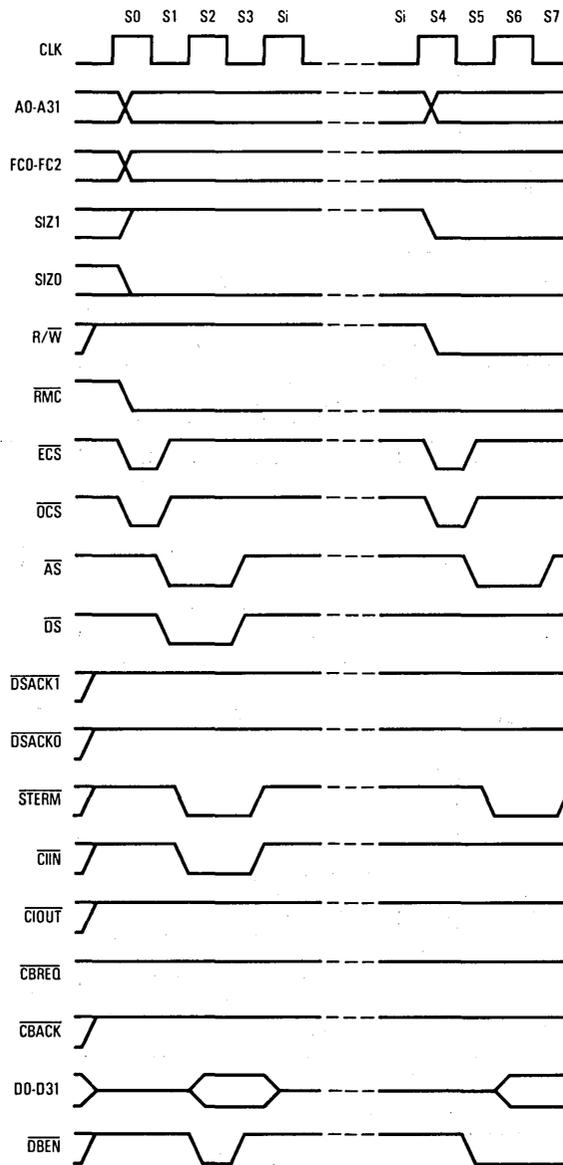
Figure 7-36. Synchronous Read-Modify-Write Cycle Timing —  $\overline{\text{CIIN}}$  Asserted
