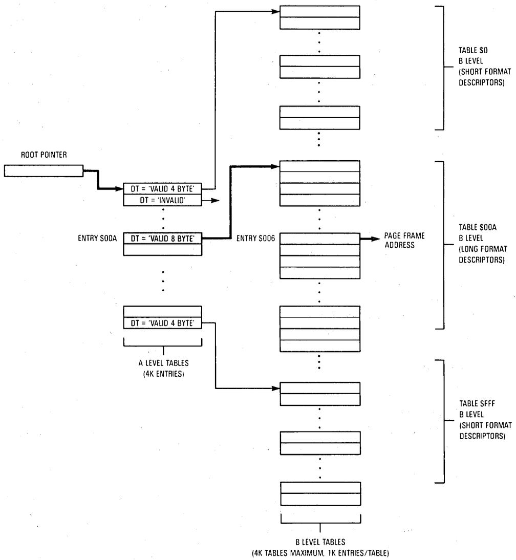
Figure 9-7. Example Translation Tree Using Different Format Descriptors
