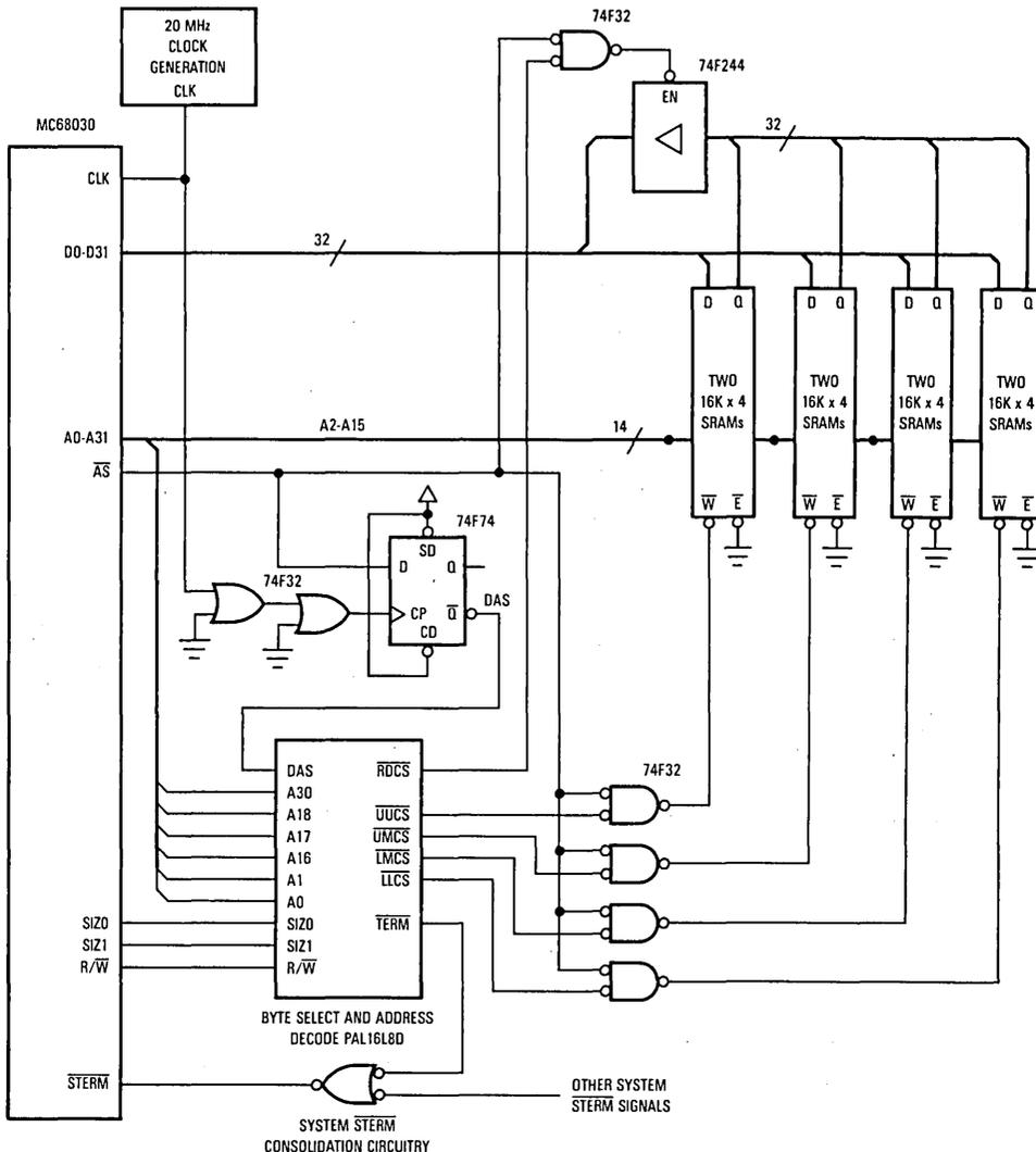
Figure 12-9. Example Two-Clock Read, Three-Clock Write Memory Bank
