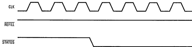
Figure 12-22. Processor Halted
