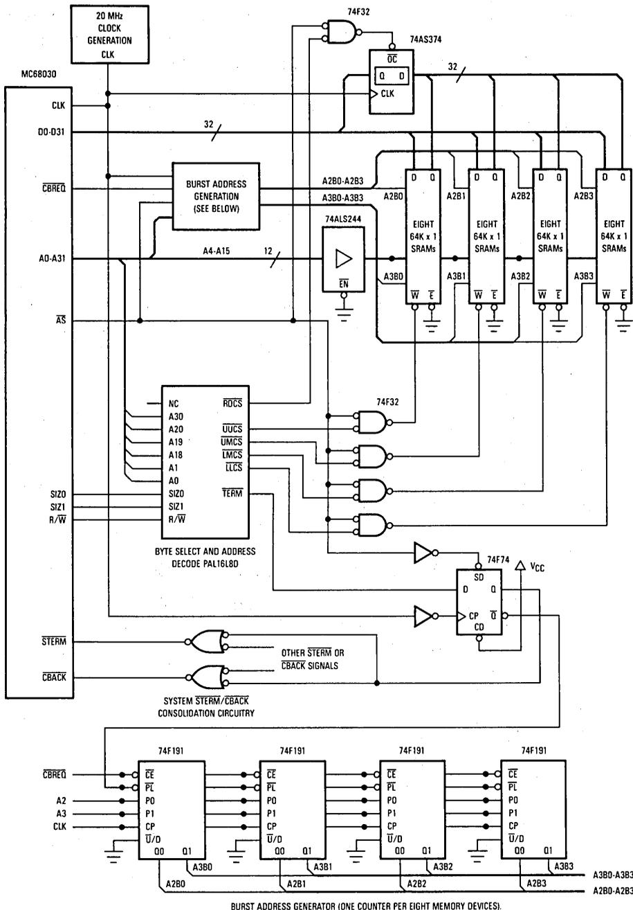
**Figure 12-15. Example 3-1-1 Pipelined Burst Mode Memory Bank at 20 MHz, 256K Bytes**
