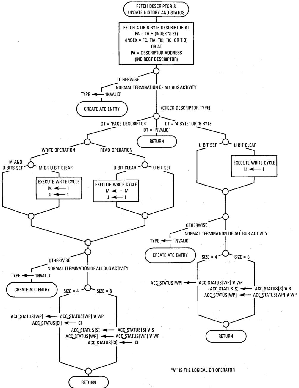
**Figure 9-29. Detailed Flowchart of Descriptor Fetch Operation**
