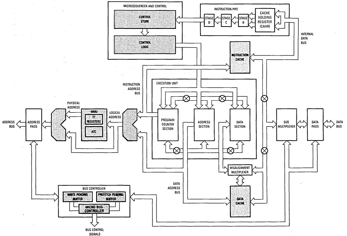
Figure 11-1. Block Diagram — Eight Independent Resources
