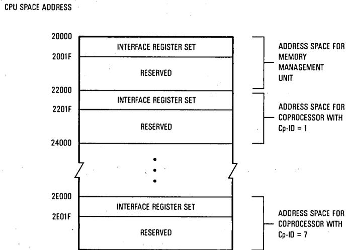
**Figure 10-4. Coprocessor Address Map in MC68030 CPU Space**
