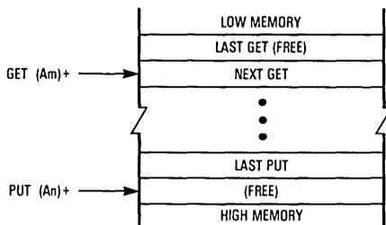
To implement the queue as a circular buffer, the relevant address register should be checked and adjusted, if necessary, before performing the "put" or "get" operation. The address register is adjusted by subtracting the buffer length (in bytes) from the register.
