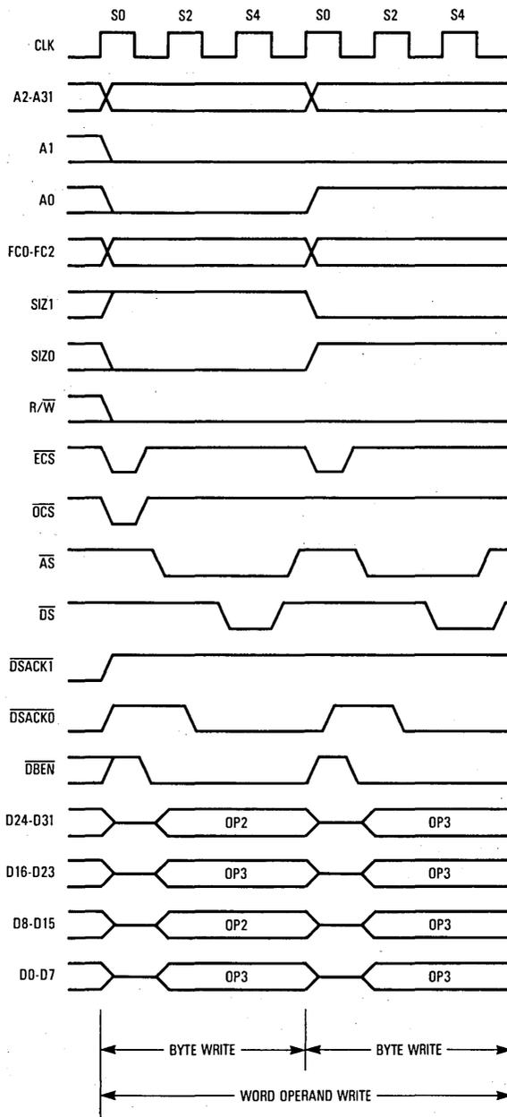
Figure 7-8. Word Operand Write Timing (8-Bit Data Port)
