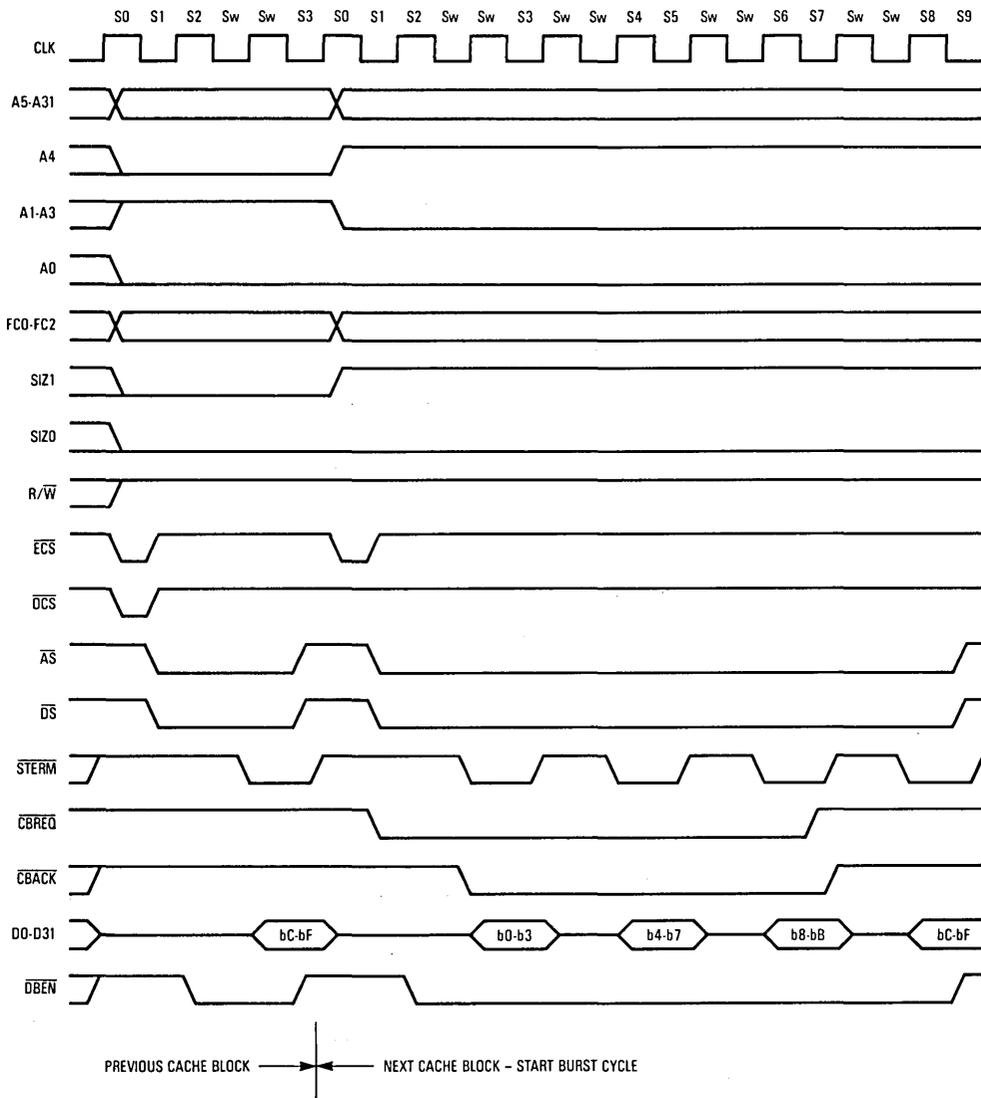
Figure 7-40. Long-Word Operand Request from \$0E — Burst Fill Deferred
