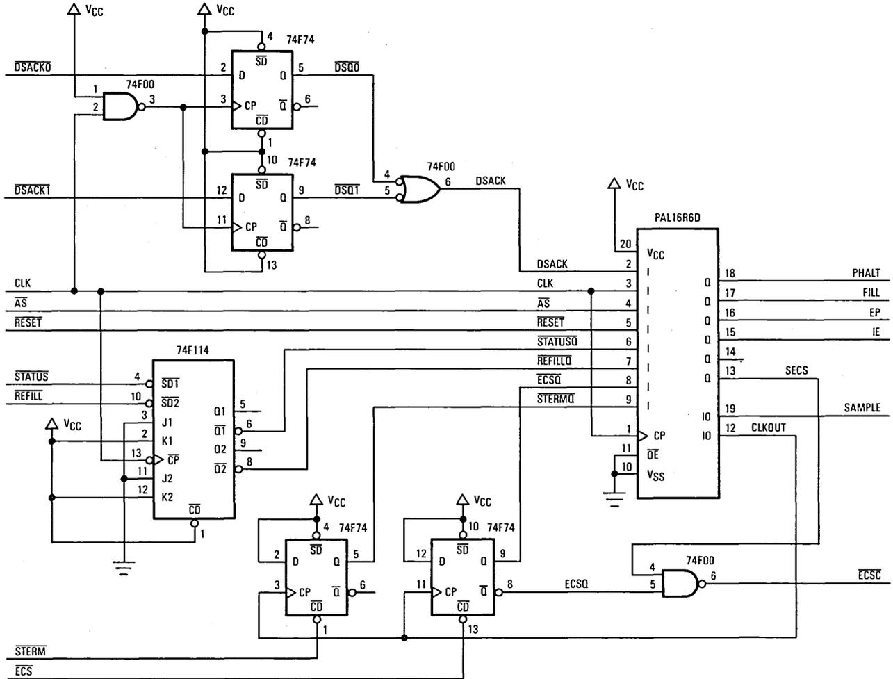
Figure 12-23. Trace Interface Circuit
