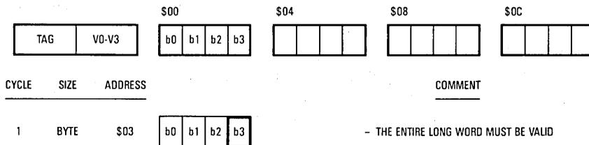
**Figure 6-7. Single Entry Mode Operation — 32-Bit Port**
