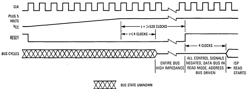
**Figure 7-64. Initial Reset Operation Timing**
