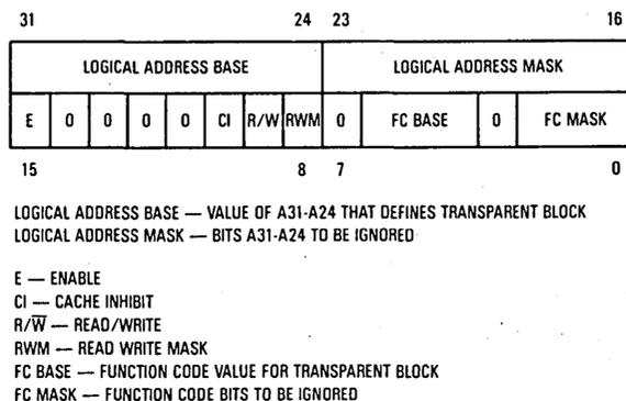
**Figure 9-37. Transparent Translation Register (TT0 and TT1) Format**
