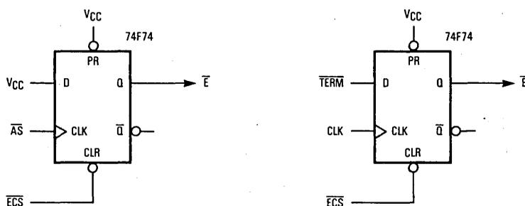
Figure 12-11. Additional Memory Enable Circuits
