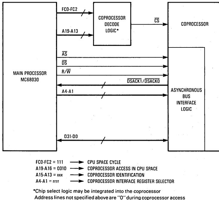
**Figure 10-2. Asynchronous Non-DMA M68000 Coprocessor Interface Signal Usage**
