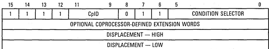
**Figure 10-10. Branch On Coprocessor Condition Instruction (cpBcc.L)**
