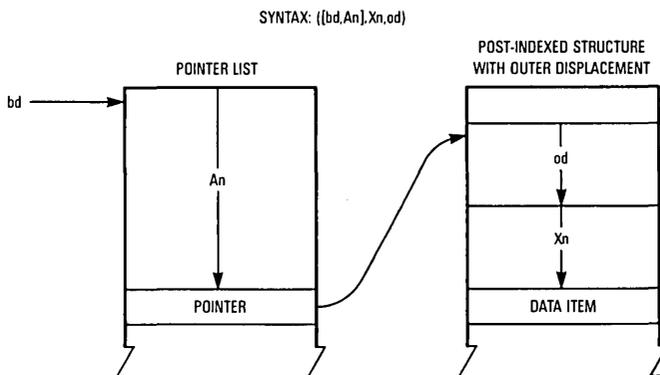
Figure 2-14. Postindexed Indirect Addressing with Outer Displacement
