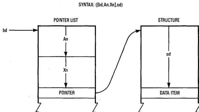
**Figure 2-13. Preindexed Indirect Addressing with Outer Displacement**
