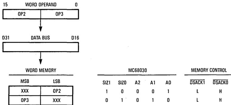
Figure 7-12. Misaligned Word Transfer to Word Port Example
