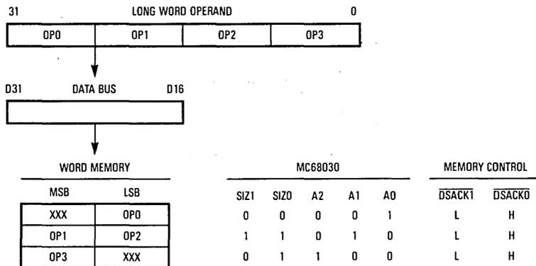
**Figure 7-9. Misaligned Long-Word Transfer to Word Port Example**
