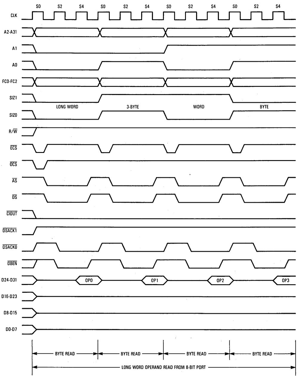
Figure 7-22. Long-Word Read — 8-Bit Port with  $\overline{CIOUT}$  Asserted
