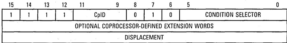
**Figure 10-9. Branch on Coprocessor Condition Instruction (cpBcc.W)**
