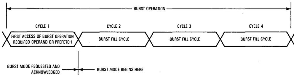
**Figure 6-11. Burst Operation Cycles and Burst Mode**
