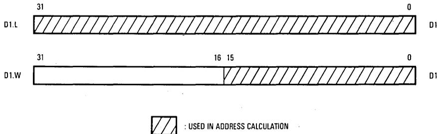
Figure 2-5. Using SIZE in the Index Selection
