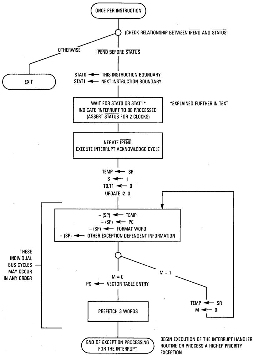
Figure 8-5. Interrupt Exception Processing Flowchart
