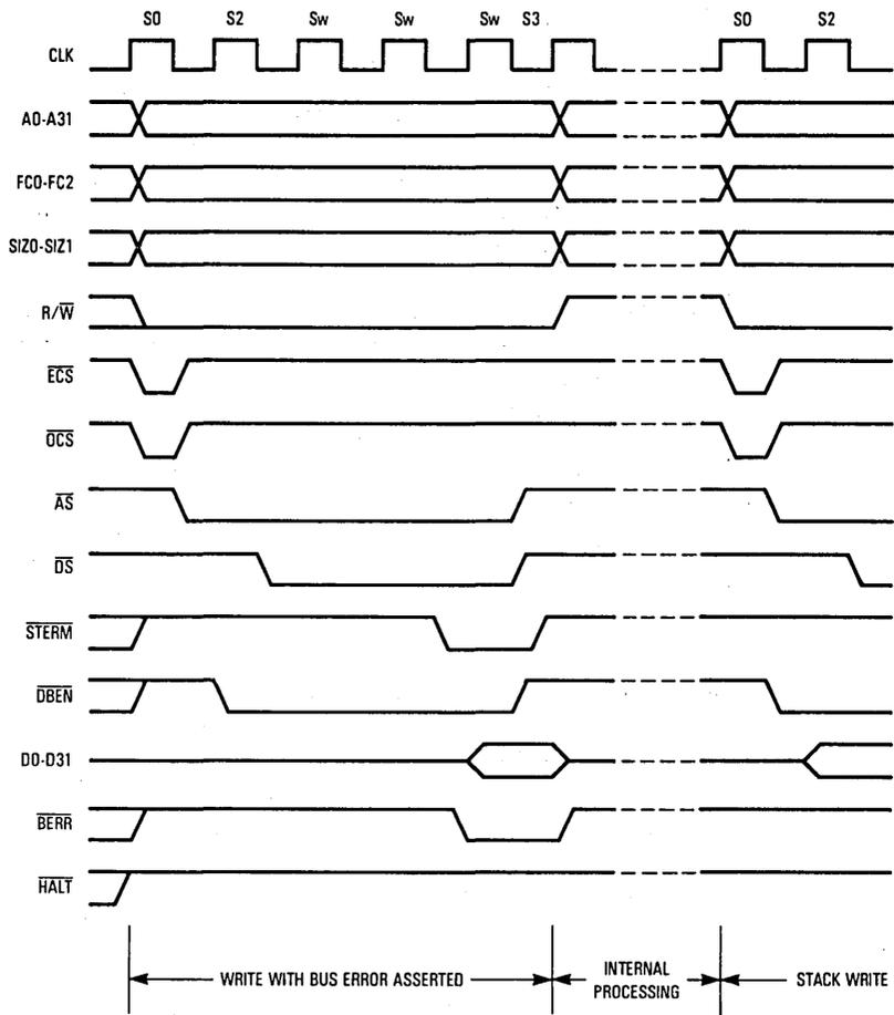
Figure 7-51. Late Bus Error with  $\overline{\text{STERM}}$  — Exception Taken
