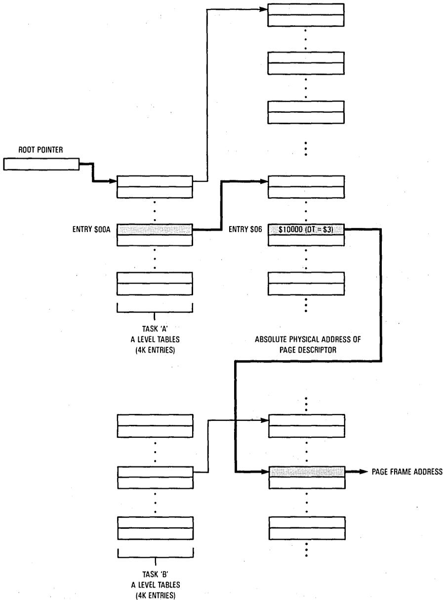
Figure 9-22. Example Translation Tree Using Indirect Descriptors
