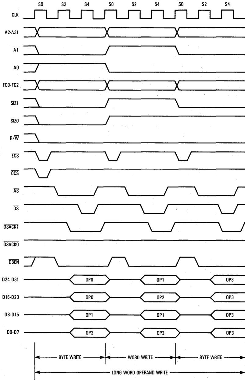
Figure 7-10. Misaligned Long-Word Transfer to Word Port
