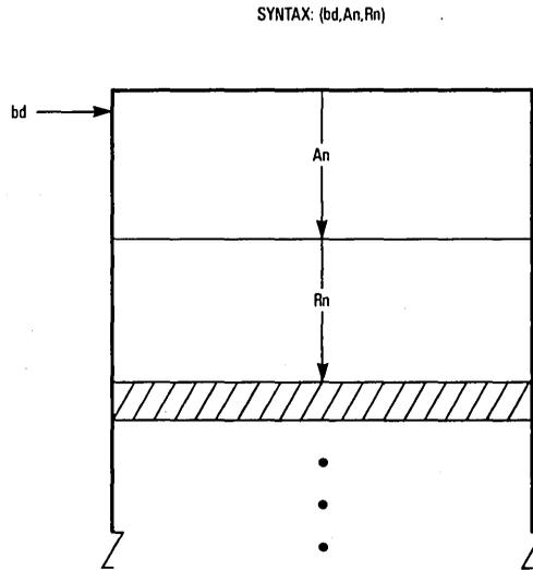
**Figure 2-6. Using Absolute Address with Indexes**
