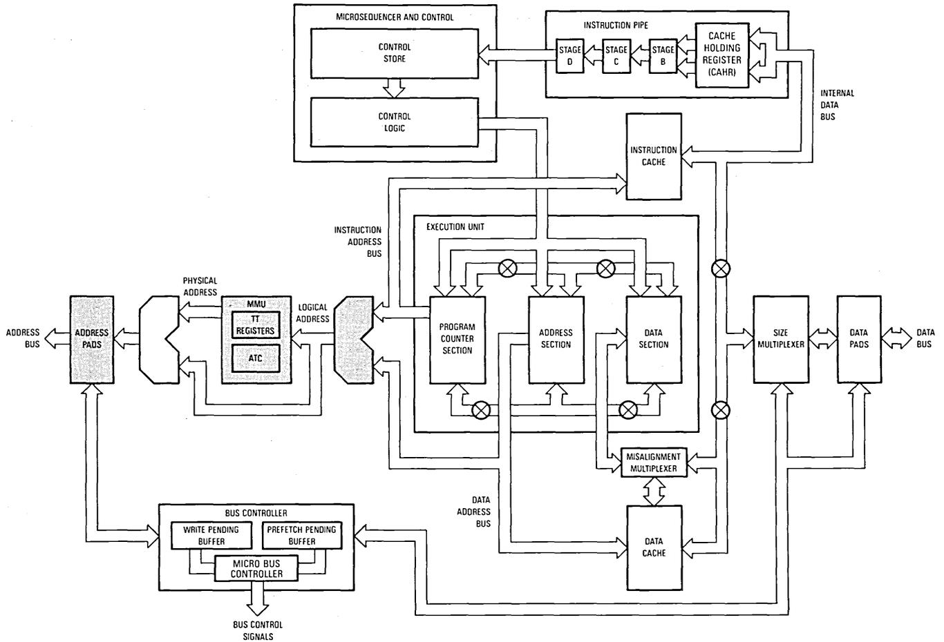
Figure 9-1. MMU Block Diagram
