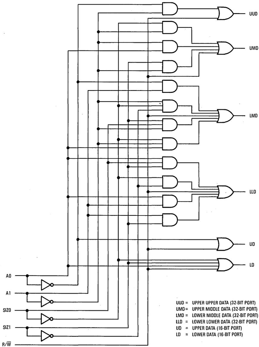
NOTE: These select lines can be combined with the address decode circuitry, or all can be generated within the same programmed array logic unit.
