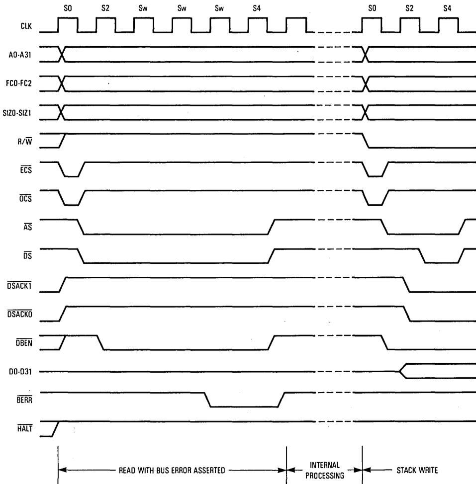
**Figure 7-48. Breakpoint Acknowledge Cycle Timing (Exception Signaled)**
