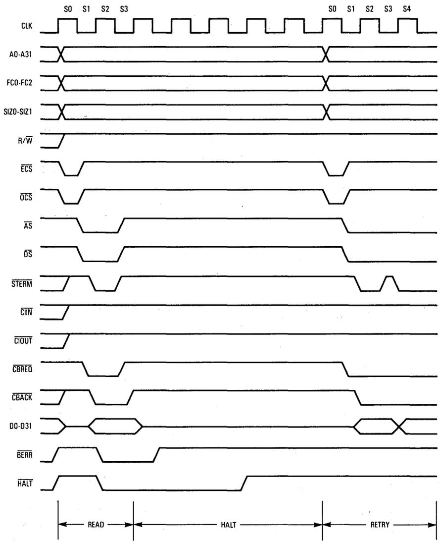
**Figure 7-56. Late Retry Operation for a Burst**
