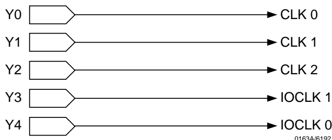
Figure 4. ispLSI and pLSI 6192 Family Global Clock Structure
