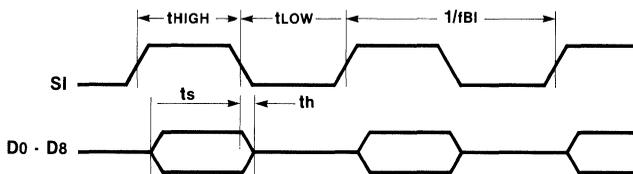
Note:  $\overline{MR}$  is HIGH;  $t_{HIGH} > t_{SIH}$ ;  $t_{LOW} > t_{SIL}$ ;  $t_{HIGH} + t_{LOW} > 1/f_{BI}$ .
