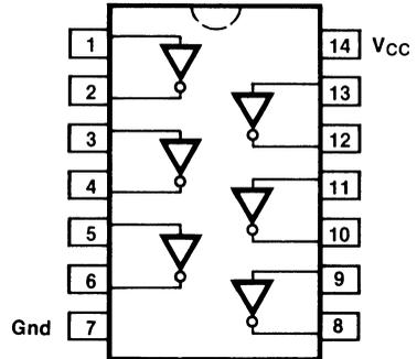
**Pin Assignment for DIP, Flatpak and SOIC**
