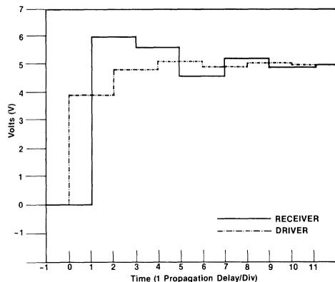
**Figure 2-3a: Resultant Waveforms Driving 50 Ohm Line — Actual**
