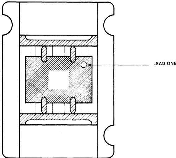
Standard carrier loading locates Lead One of the device adjacent to the side with the double notch, mark side up.
