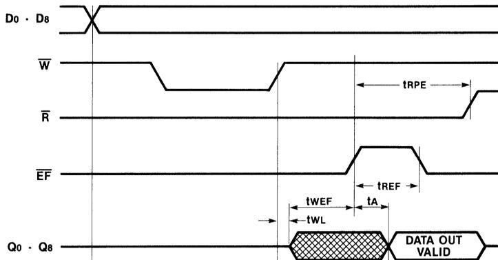
**Figure 16: Write Data Flow-Through Mode**
