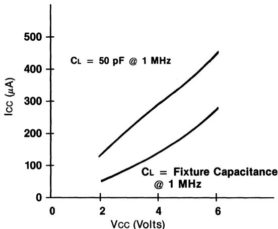
Figure 2-1 illustrates the effects of I<sub>CC</sub> versus power supply voltage (V<sub>CC</sub>) for two load capacitance values: 50 pF and stray capacitance. The clock frequency was 1 MHz for the measurements.
