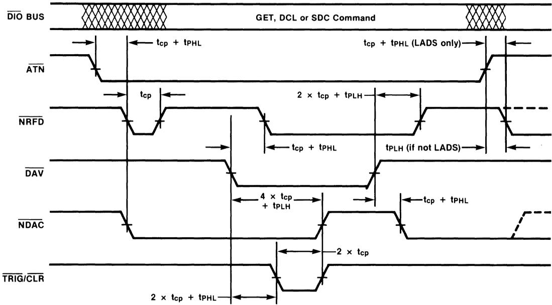
Figure 14: Timing Diagram for Remote/Local Logic (Starting in LOCAL State)
