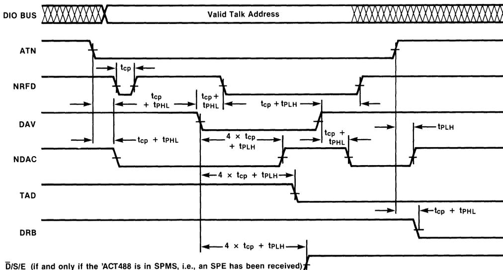
**Figure 11: Timing Diagram for Secondary Address Sequence**
