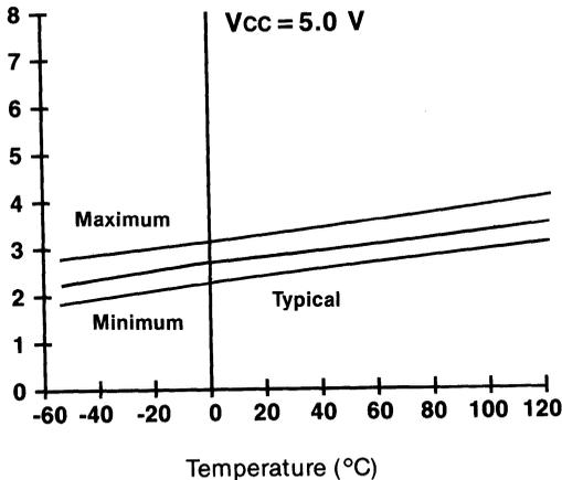
**Figure 2-11c: Voltage Effects on Delay Times**
