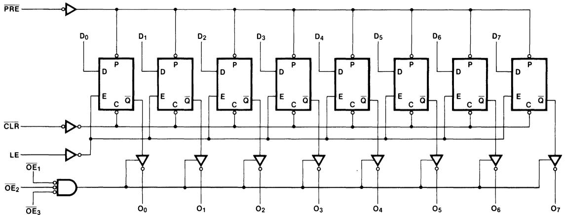
Please note that this diagram is provided only for the understanding of logic operations and should not be used to estimate propagation delays. The 'AC/ACT846 has the same logic diagram with inverting outputs.
