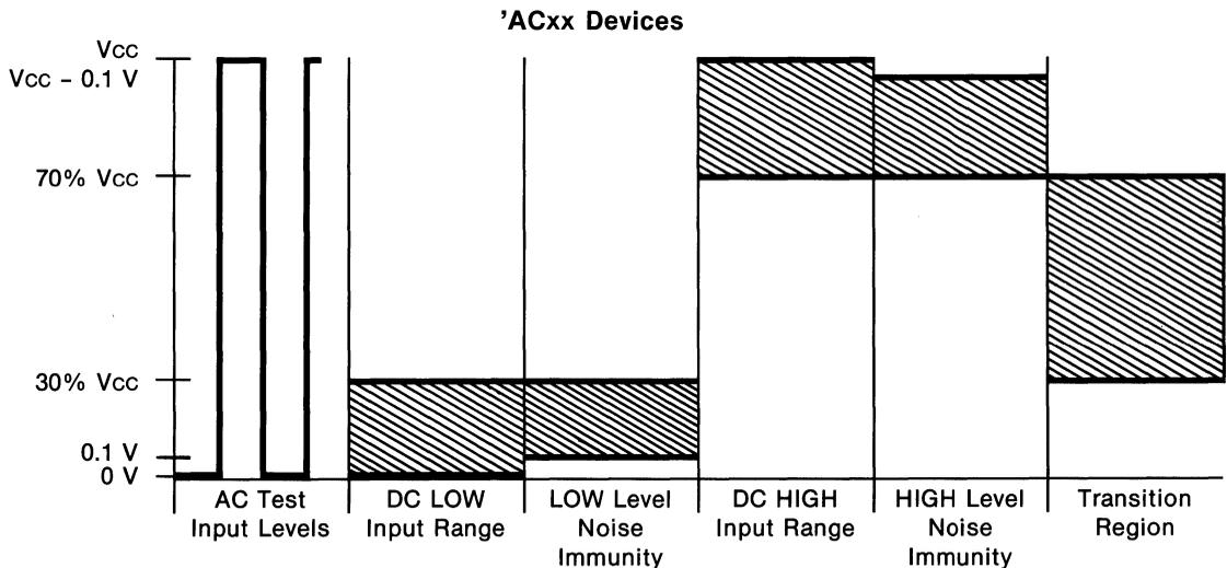
**Figure 3-4b: Test Input Signal Levels**
