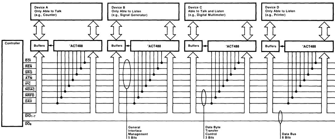
**Figure 2: Source and Acceptor Handshake Logic**
