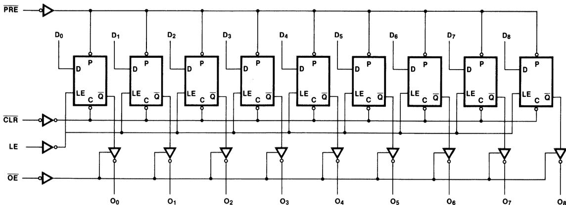
Please note that this diagram is provided only for the understanding of logic operations and should not be used to estimate propagation delays. The 'AC'/ACT844 has the same logic diagram with inverting outputs.
