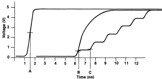
would be required before the comparator would detect the level. It is this added delay time caused by the transmission line environment of the ATE that may cause parts to fail customers' incoming tests, even though the device meets specifications. The figure below graphically shows this stepout.
