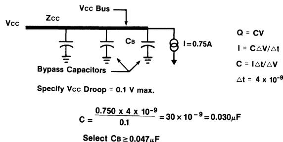
Place one decoupling capacitor adjacent to each package driving any transmission line and distribute others evenly throughout the logic. One capacitor per three packages.
