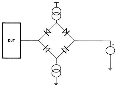
The voltage source provides a pull-up/pull-down voltage while the current sources provide  $I_{OH}$  and  $I_{OL}$ . When devices with slow output slew rates are tested with the ATE load, the resultant waveforms closely approximate the bench waveform, and a
