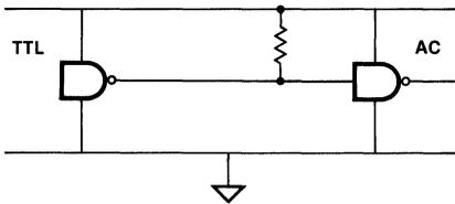
Unfortunately, there will be designs where including a pull-up resistor will not be acceptable. In these cases, such as a terminated TTL bus, Fairchild has designed devices which offer thresholds that are TTL-compatible (Figure 4-3). These interfaces tend to be slightly slower than their CMOS-level counterparts due to an extra buffer stage required for level conversion.
