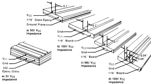
Local high frequency decoupling is required to supply power to the chip when it is transitioning from a LOW to a HIGH value. This power is necessary to charge the load capacitance or drive a line impedance. Figure 4-13 displays various Vcc and ground layout schemes along with associated impedances.
