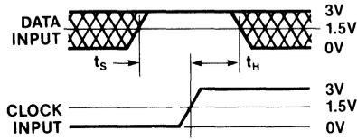
Figure 8: State Control Timing
