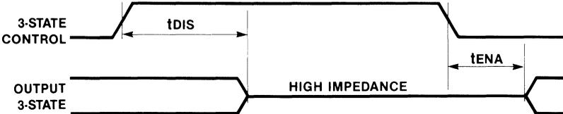
Figure 11: '1016 Timing Diagram
