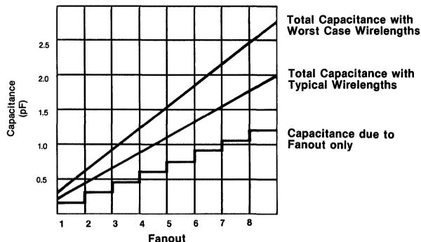
The figure illustrates variations of capacitance due to fanout and wirelength of an estimated average of internal cell macros. Typical wirelengths are based on an assumption of 15 mils length per connection, 30% first-layer and 70% second-layer metal routing. Worst case wirelengths assume 30 mils length per connection with 50% first-layer and 50% second-layer metallization.
