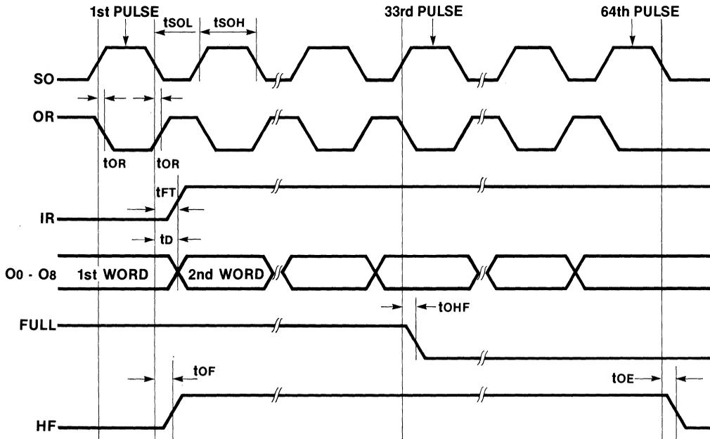
Note:  $\overline{SI}$  and  $\overline{OE}$  are LOW;  $\overline{MR}$  is HIGH;  $D_0 - D_8$  are immaterial.
