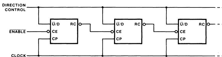
**Figure c: Synchronous N-Stage Counter With Parallel Gated Carry/Borrow**
