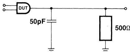
Figure 6: Output 3-State Delay Load
