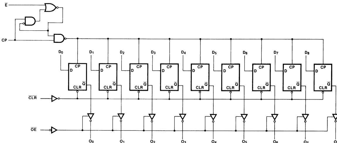
Please note that this diagram is provided only for the understanding of logic operations and should not be used to estimate propagation delays. The 'AC'/ACT824 also has the same logic diagram with inverting outputs.
