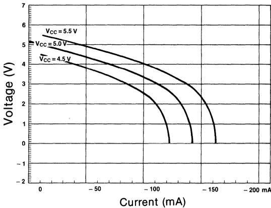
**Figure 2-5: Output Characteristics  $V_{OL}/I_{OL}$ , 'AC00**
