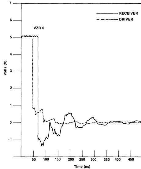
**Figure 2-3b: Resultant Waveforms Driving 50 Ohm Line — Theoretical**
