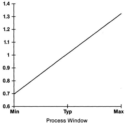
**Figure 2-11e:  $t_{PHL}$ , A to B, with Voltage and Process Variation**
