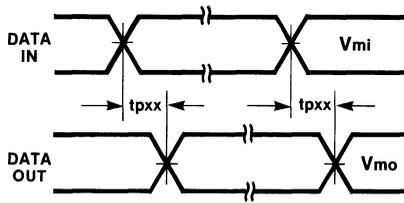
**Figure 3-6: Propagation Delay, Pulse Width and  $t_{rec}$  Waveforms**
