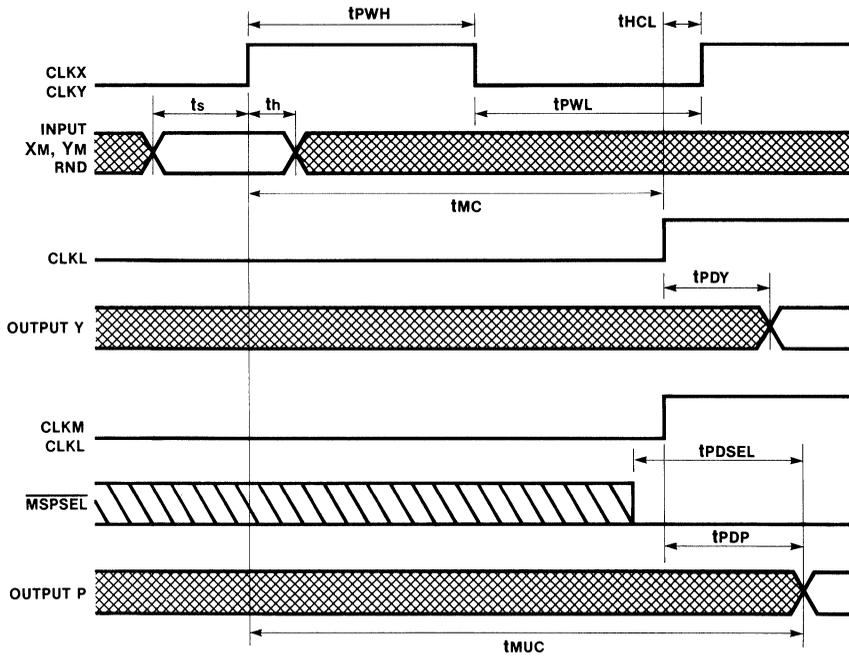
Figure 12: Simplified Timing Diagram — Typical Application
