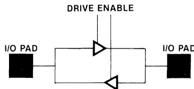
Each I/O pin is connected to both an input device and an output device. The pin can be viewed as having three states: input, output and output disabled. However, only two states actually exist.
