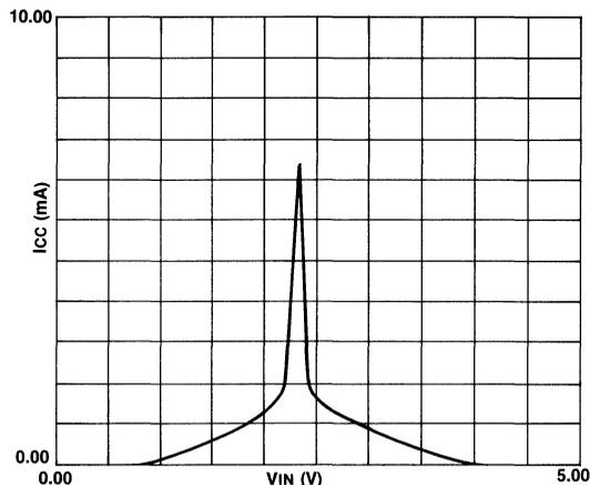
When testing the  $I_{CC}$  of a CMOS '245, problems can arise depending upon how the test is conducted. Note the structure of the '245's I/O pins illustrated below.
