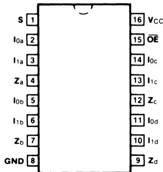
Pin Assignment for DIP, Flatpak and SOIC
