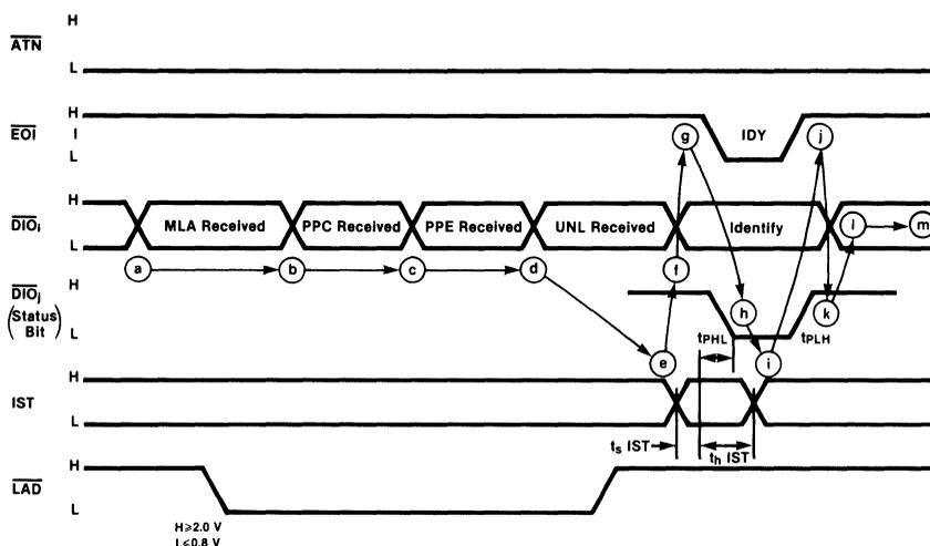
**Figure 18: IFC Timing Diagram**
