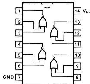
Pin Assignment for DIP, Flatpak and SOIC
