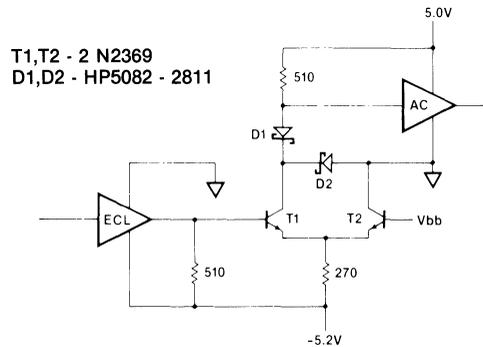
**Figure 4-4c: Differential Output ECL-to-'AC Circuit**
