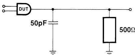
Figure 8: Output 3-State Delay Load
