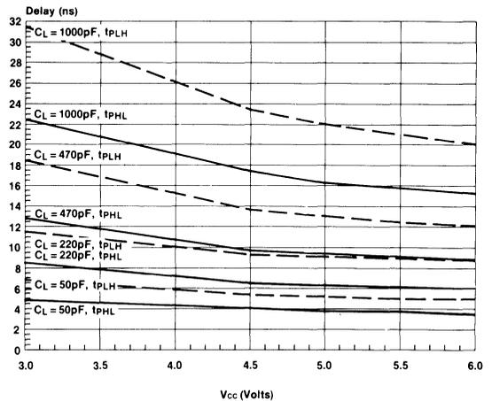
**Figure 2-13: Propagation Delay vs. CL (AC00)**
