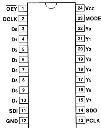
Pin Assignment for DIP, Flatpak and SOIC
