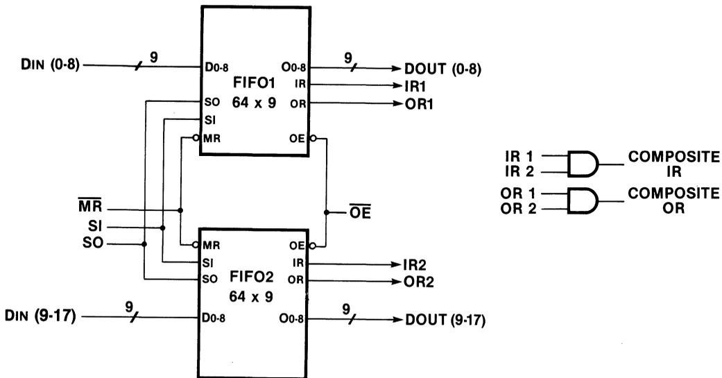
Note: Monitor flags from any one FIFO or AND the corresponding flags to obtain a composite signal.
