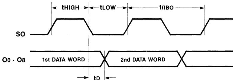
Note:  $\overline{OE}$  is LOW;  $\overline{MR}$  is HIGH;  $t_{HIGH} > t_{SOH}$ ;  $t_{LOW} > t_{SOL}$ ;  $t_{HIGH} + t_{LOW} \geq 1/f_{BO}$ .
