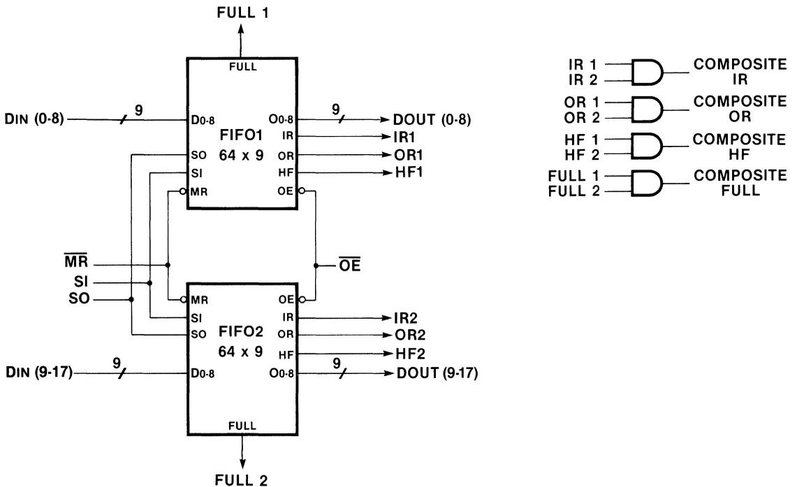
Note: Monitor flags from any one FIFO, or AND the corresponding flags to obtain a composite signal.
