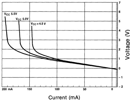
**Figure 2-6: Input Characteristics  $V_{IN}/I_{IN}$**
