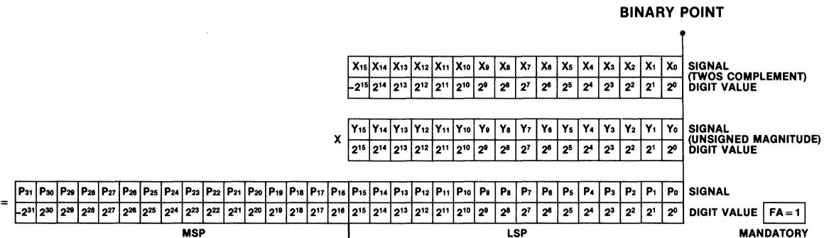
\*In this format an overflow occurs in the attempted multiplication of the twos complement number 1000...0 with 1000.00 yielding an erroneous product of -1 in the fraction case and -2<sup>30</sup> in the integer case.
