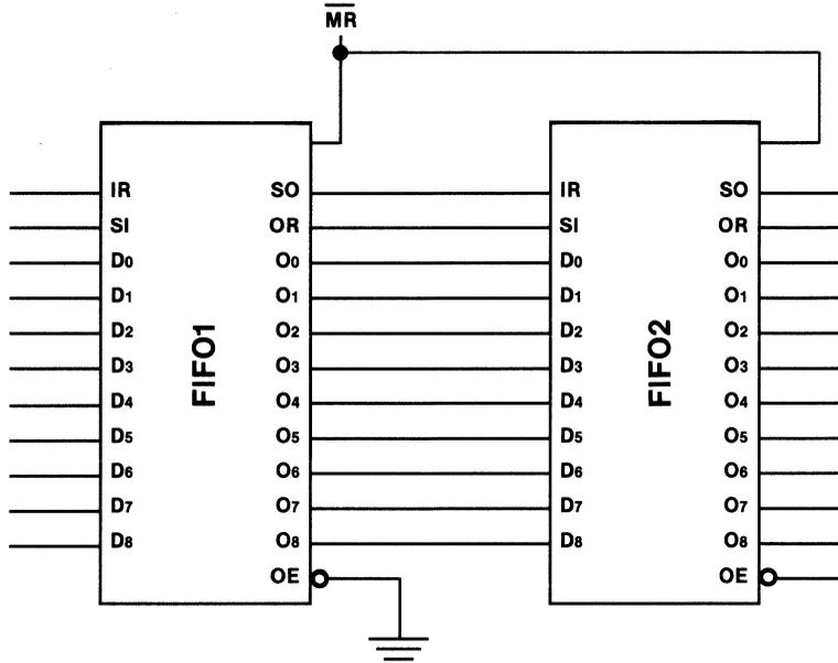
**Figure 10: Handshaking for Depth Expansion Mode — 128 x 9 FIFO**
