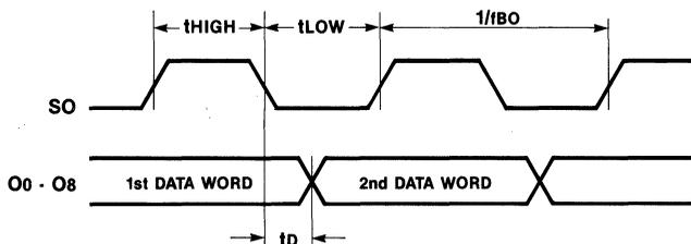
Note:  $\overline{OE}$  is LOW;  $\overline{MR}$  is HIGH;  $t_{HIGH} > t_{SOH}$ ;  $t_{LOW} > t_{SOL}$ ;  $t_{HIGH} + t_{LOW} > 1/f_{BO}$ .
