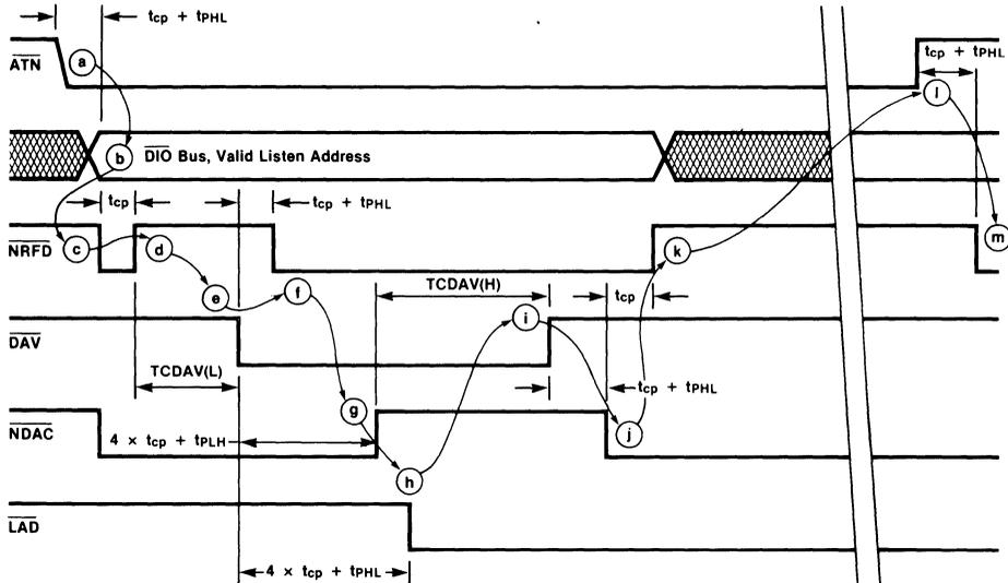
Note:  $\overline{ATN}$ ,  $\overline{DIO}$  bus and  $\overline{DAV}$  driven by controller;  $\overline{NRFD}$ ,  $\overline{NDAC}$  driven by 'ACT488.
