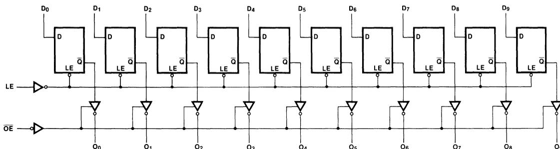
Please note that this diagram is provided only for the understanding of logic operations and should not be used to estimate propagation delays. The 'AC/ACT842 has the same logic diagram with inverting outputs.
