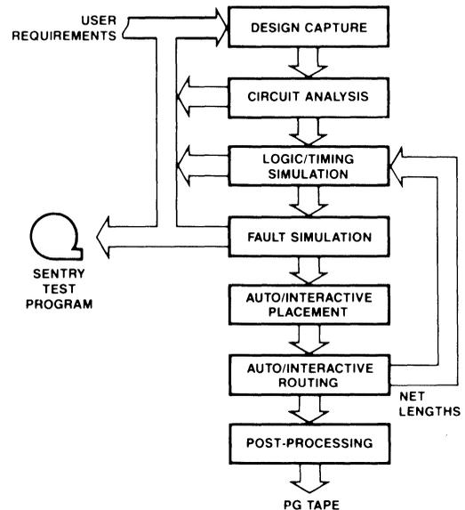
**Figure 7-7: Typical Engineering Workstation Design Flow**
