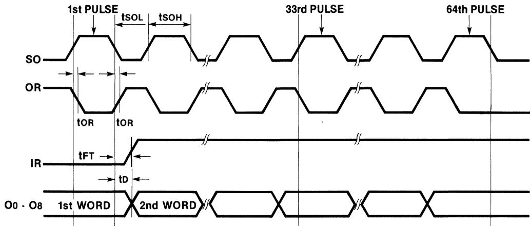
Note:  $\overline{SI}$  and  $\overline{OE}$  are LOW;  $\overline{MR}$  is HIGH;  $D_0 - D_8$  are immaterial.
