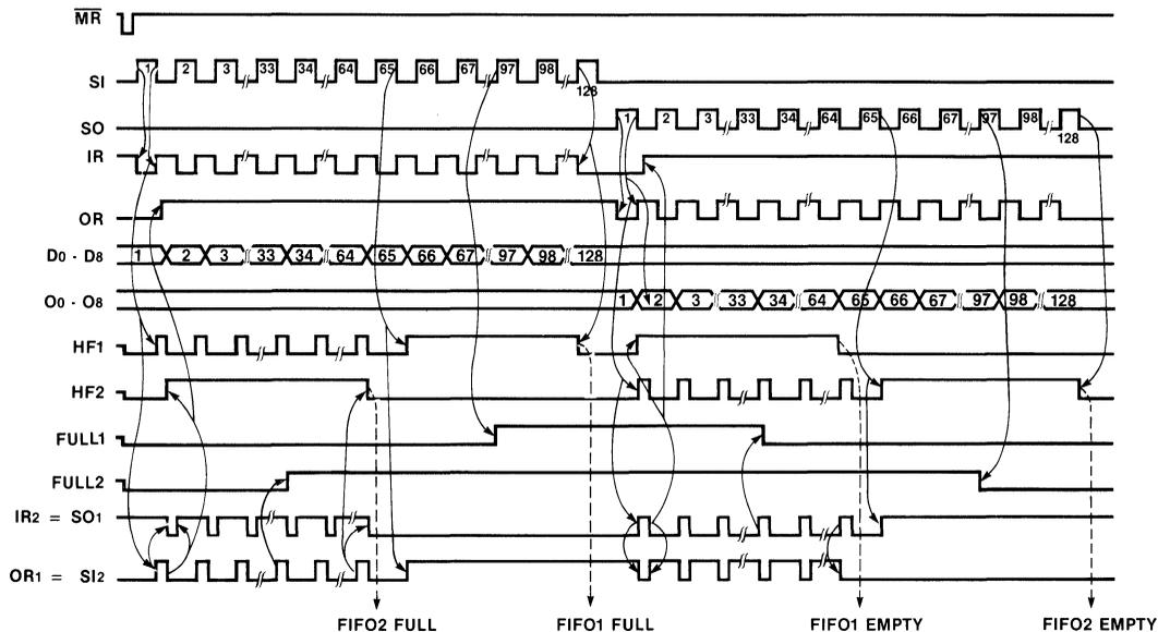
Note: The numbers for SI and SO indicate the pulse numbers. The numbers for data in and data out indicate data words: 1 is first data word, 2 is second data word, etc.
