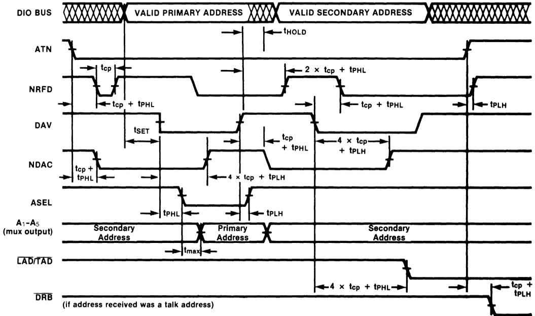
**Figure 12: Timing Diagram for 'ACT488 Receiving Bus Commands**
