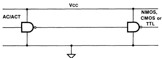
FACT devices can be directly driven by both NMOS and CMOS families, as shown in Figure 4-1, operating at the same rail potential without special considerations. This is possible due to the low input loading of FACT product, guaranteed to be less than 1  $\mu$ A per input.
