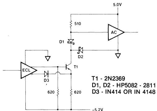
It should be understood that for FACT, as with other CMOS technologies, input levels that are between specified input values will cause both transistors in the CMOS structure to be conducting. This will cause a low resistive path from the supply rail to ground, increasing the power consumption by several orders of magnitude. It is important that CMOS inputs are always driven as close as possible to the rail.
