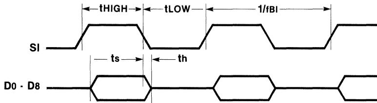
Note:  $\overline{MR}$  is HIGH;  $t_{HIGH} > t_{SIH}$ ;  $t_{LOW} > t_{SIL}$ ;  $t_{HIGH} + t_{LOW} \geq 1/f_{BI}$ .
