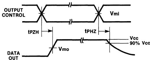
**Figure 3-8: 3-State Output Low Enable and Disable Times**
