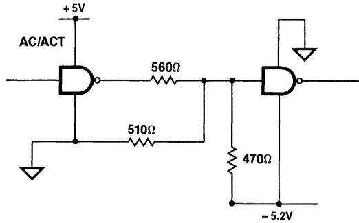
**Figure 4-4b: Single-Ended ECL-to-'AC Circuit**
