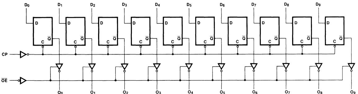
Please note that this diagram is provided only for the understanding of logic operations and should not be used to estimate propagation delays. The 'AC/'ACT822 also has the same logic diagram with inverting outputs.
