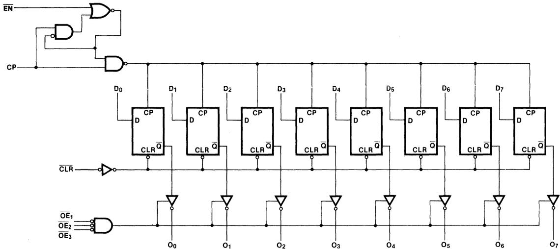
Please note that this diagram is provided only for the understanding of logic operations and should not be used to estimate propagation delays. The 'AC/'ACT826 also has the same logic diagram with inverting outputs.
