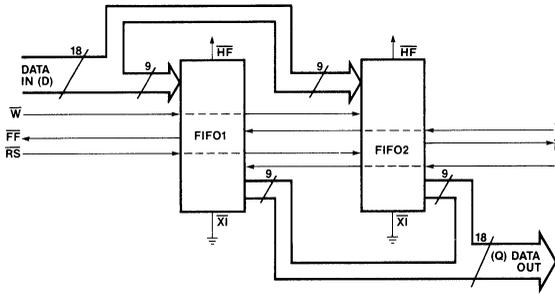
Notes: Flag detection is accomplished by monitoring  $\overline{FF}$ ,  $\overline{EF}$  and  $\overline{HF}$  on any device used in the width expansion configuration. Output signals should not be connected together.
