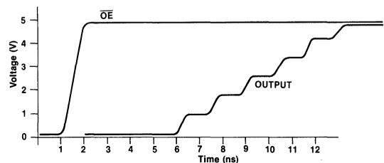
Transmission line theory states the voltage level of this current wave is equal to the current in the line times the impedance of the line. With typical currents as low as 5 mA and impedances of 50 to 60 ohms, this voltage step can be as minimal as 250 mV. If the comparator was programmed to the 10% point, it would be looking for a step of 550 mV at 5.5 V Vcc. Three reflections of the current pulse
