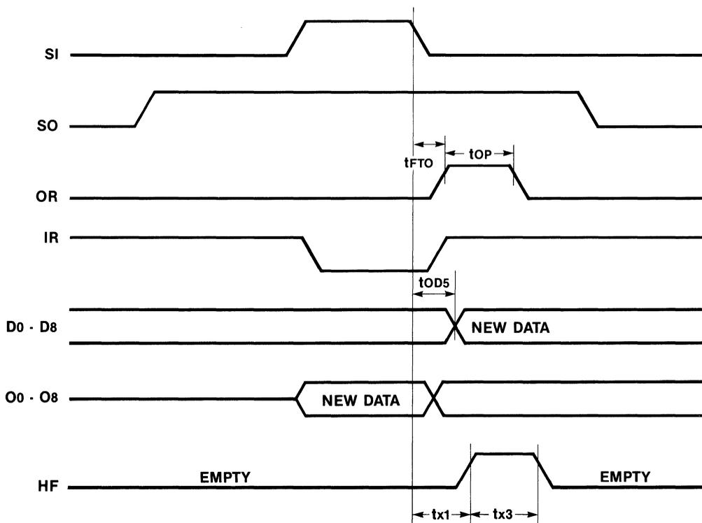
Note: FULL is LOW;  $\overline{MR}$  is HIGH;  $\overline{OE}$  is LOW;  $t_{DOF} = t_{FTO} - t_{OD5}$ . Data output transition—valid data arrives at output stage  $t_{DOF}$  after OR is HIGH.
