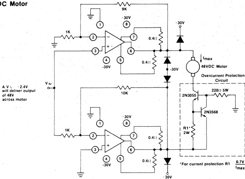
Figure 15: Power Amp Driving 48 VDC Motor
