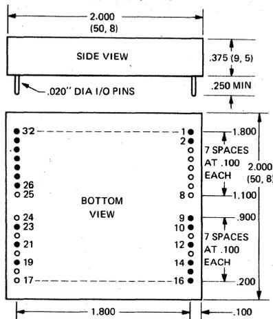
NOTE: OPEN DOTS INDICATE OMITTED PINS. PIN POSITION TOLERANCE IS  $\pm 0.005$ " FROM DATUM, NON-ACCUMULATIVE. WEIGHT: 1.8 OZ. (51 G)
