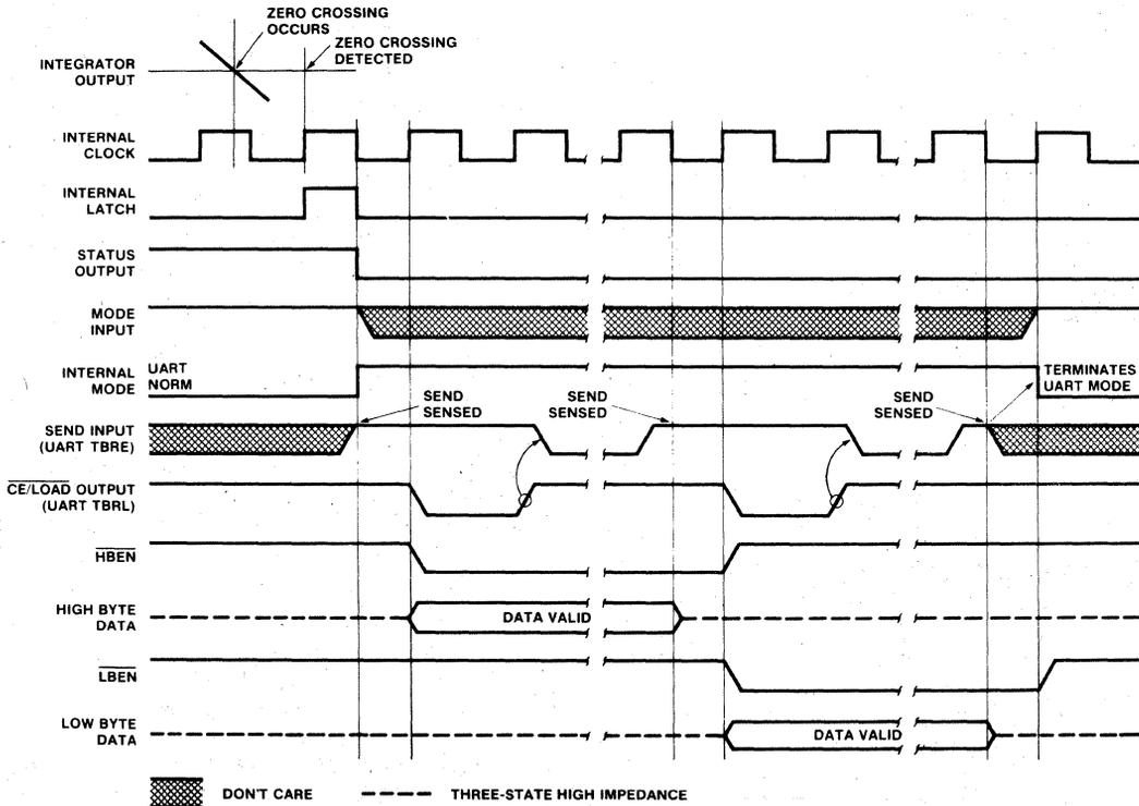
Figure 8: Handshake - Typical UART Interface Timing
