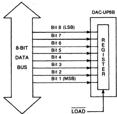
This illustrates the connection for loading parallel data into the input register. The register circuit is a static latch and is controlled by the **LOAD**, active low. When the data is stable on the data inputs (bits 1-8), it can be transferred on the positive edge of the **LOAD** pulse. The voltage levels on the data bus should be stable for at least 200 nsec before **LOAD** goes HI. The minimum pulse width of the **LOAD** command is 200 nsec.
