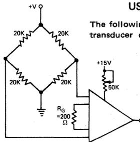
The following errors are computed for an AM-201C operated from a bridge transducer over a  $\pm 10^\circ C$  ambient temperature range at a gain of 1000.
