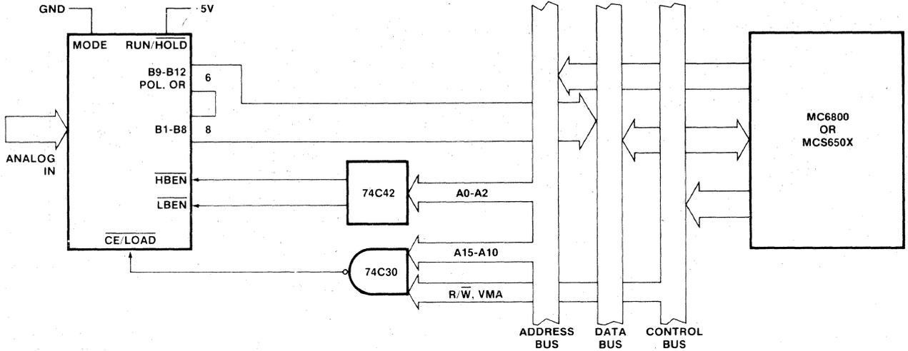
Figure 19: Direct ADC-7109 — MC6800 Bus Interface
