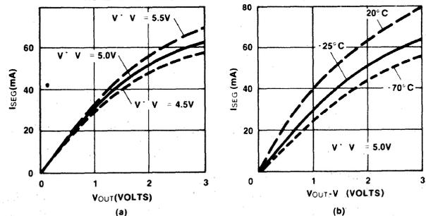
**Figure 7:** 7226B Typical I<sub>SEG</sub> Vs. V<sup>+</sup>-V<sub>out</sub>
