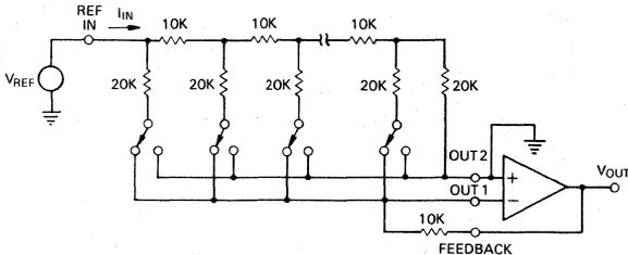
**Figure 1. PRECISION DAC-HA CIRCUIT**
