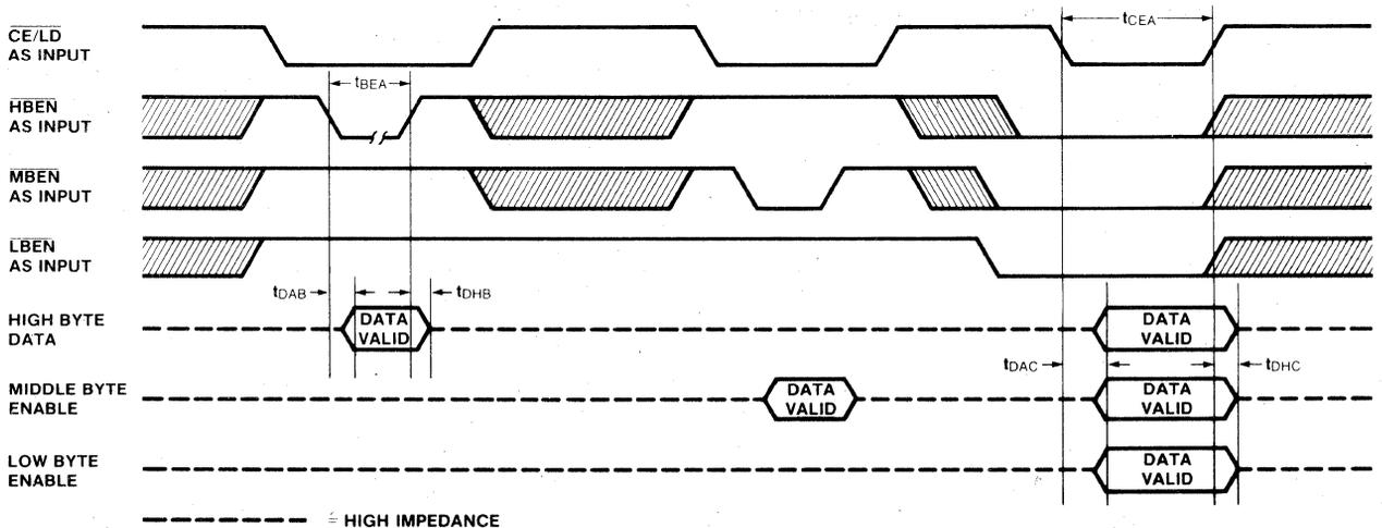
Figure 2: Direct Mode Output Timing
