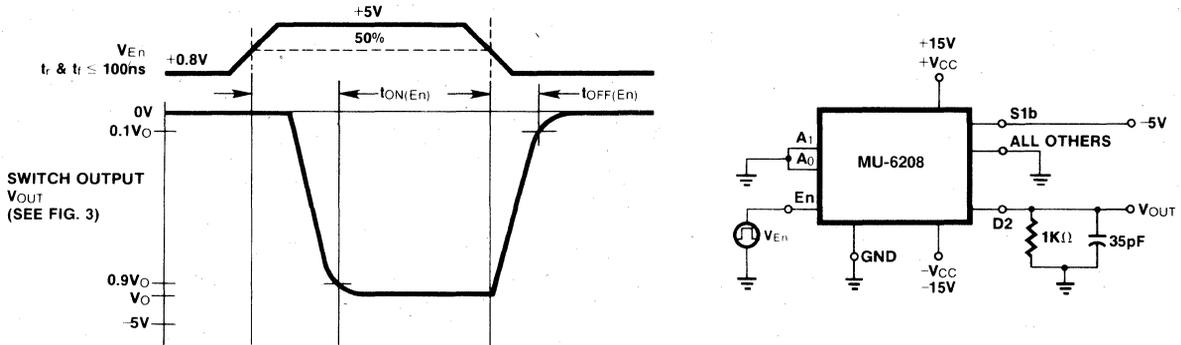
Figure 3.  $t_{on}$  and  $t_{off}$  Switching Test
