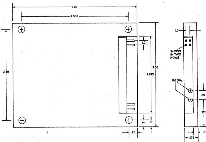
Ultra-Linear 8 Bit A/D Converter Model ADC-881
