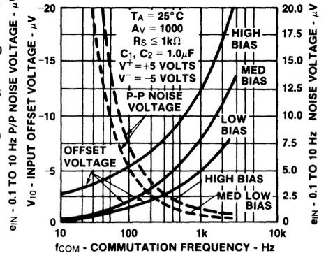
INPUT OFFSET VOLTAGE AND PK TO PK NOISE VOLTAGE AS A FUNCTION OF COMMUTATION FREQUENCY (C1, C2 = 0.1 μF)
