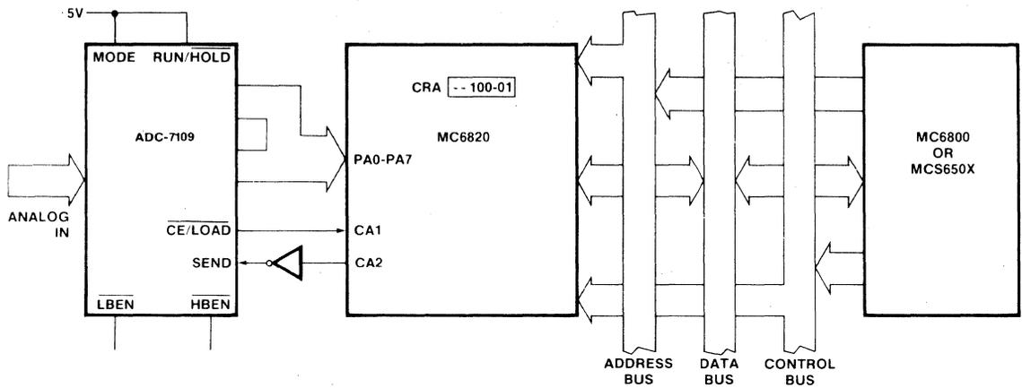
Figure 21: Handshake Interface — ADC-7109 to MC6800, MCS650X
