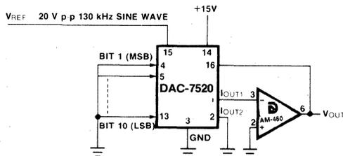
Figure 5. Feedthrough Error
