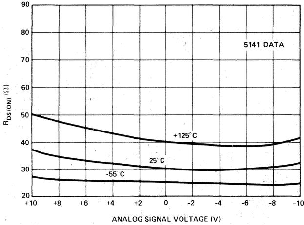
FIGURE 2.  $R_{DS(ON)}$  vs. Temp., @  $\pm 15V$ ,  $+5V$  Supplies.
