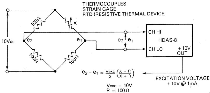
Remote monitoring of low level signals can be difficult, especially when analog signals pass through an environment with high levels of electrical noise. One solution is to use an instrumentation amplifier to extract the common mode voltage and amplify the voltage difference. The HDAS-8, an eight channel differential input system,
