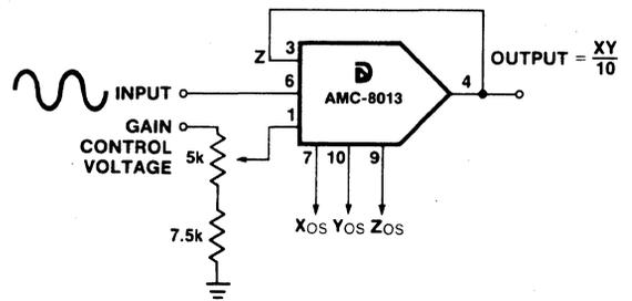
DATTEL-INTERISL'S AMC-8013 ALLOWS ANALOG MULTIPLICATION, DIVISION AND EXPONENTIATION, OR MAY BE CONFIGURED AS A VARIABLE GAIN AMPLIFIER.
