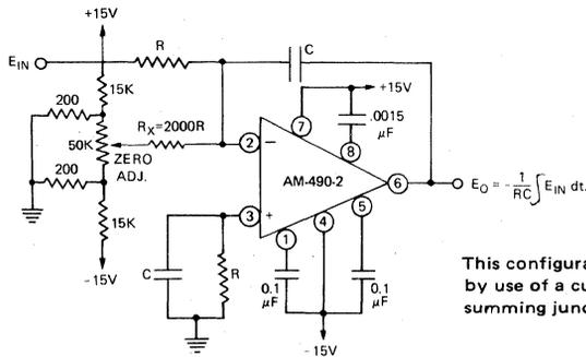
This configuration shows zeroing by use of a current into the summing junction.
