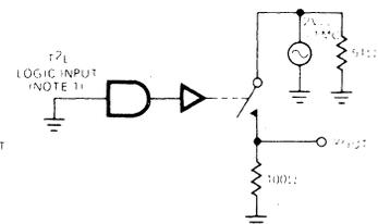
**NOTE 1:** Some channels are turned on by high "1" logic inputs and other channels are turned on by low "0" inputs; however 0.8V to 2.4V describes the min. range for switching properly. Refer to logic diagrams to see absolute value of logic input required to produce "ON" or "OFF" state.
