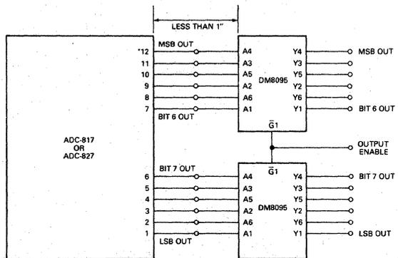
\*FOR TWO'S COMPLEMENT OUTPUT CODING THIS CONNECTION IS PIN 13 (MSB)
