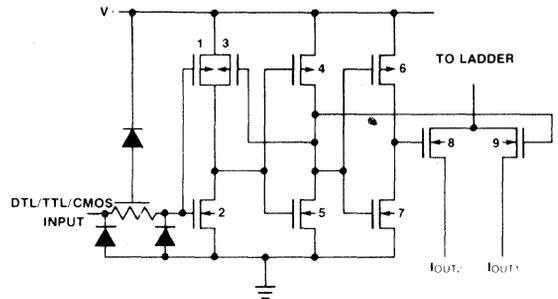
Figure 8. CMOS Switch
