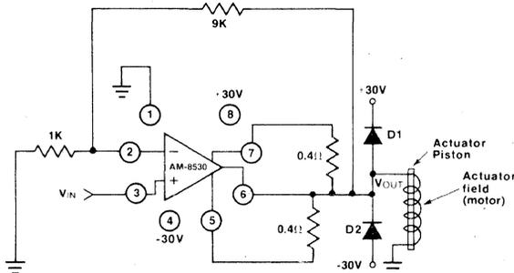
Figure 13: Power Amp Driving Actuator
