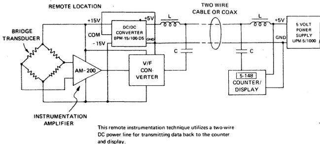
This remote instrumentation technique utilizes a two-wire DC power line for transmitting data back to the counter and display.
