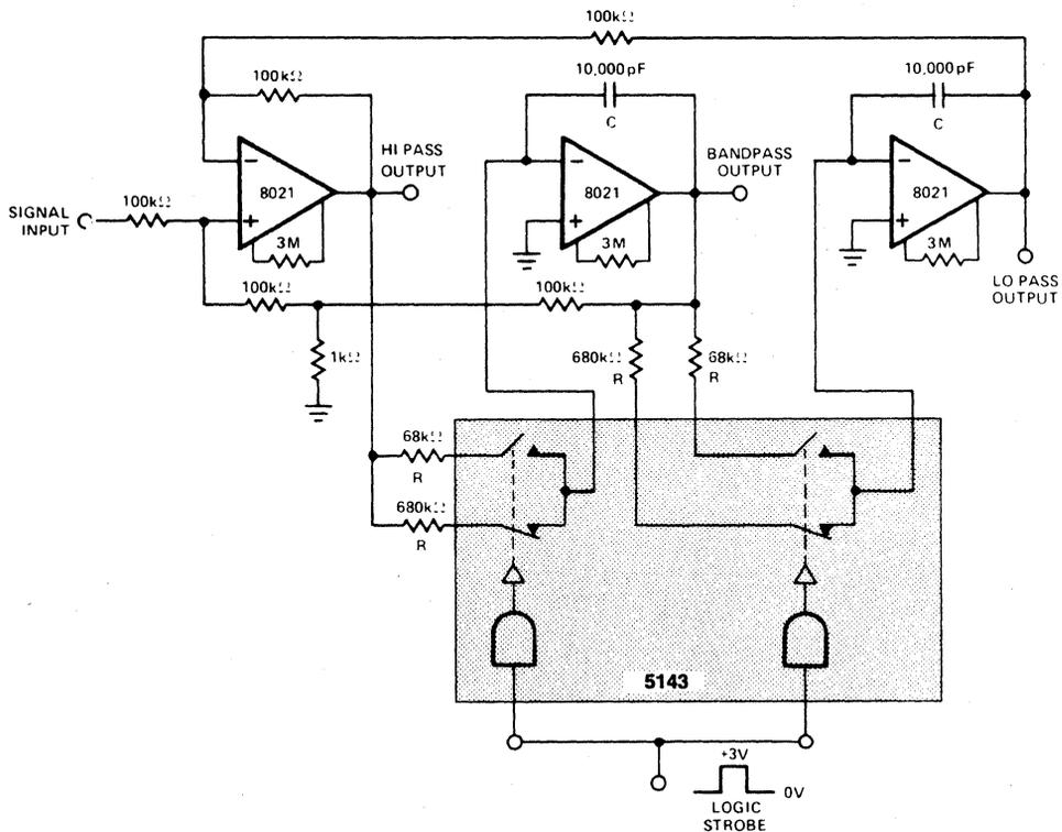
CONSTANT GAIN, CONSTANT Q, VARIABLE FREQUENCY FILTER WHICH PROVIDES SIMULTANEOUS LOWPASS, BANDPASS, AND HIGHPASS OUTPUTS. WITH THE COMPONENT VALUES SHOWN, CENTER FREQUENCY WILL BE 235Hz AND 23.5Hz FOR HIGH AND LOW LOGIC INPUTS RESPECTIVELY,  $Q = 100$ , AND GAIN = 100.
