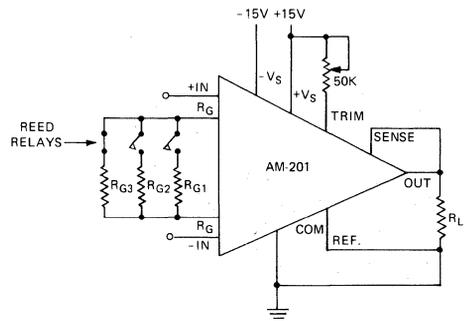
Gain is inversely proportional to  $R_G$ . Thus if  $R_G$  is halved the gain is exactly doubled. Input offset voltage does not change with  $R_G$ .
