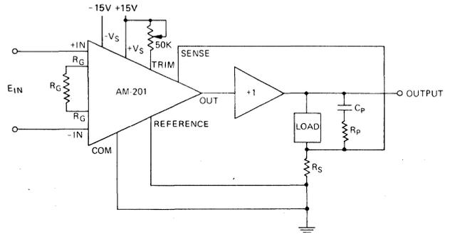
**NOTE:** The output voltage using the gain equation will appear across  $R_S$ . The load impedance and output of the current booster must be compatible with this. Highly inductive loads may cause ringing or oscillation. In this case add  $R_p$  and  $C_p$  as shown.
