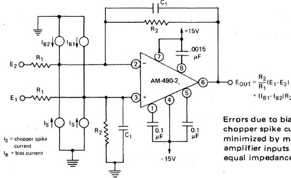
Errors due to bias current and chopper spike current are minimized by making both amplifier inputs look back into equal impedances to ground.
