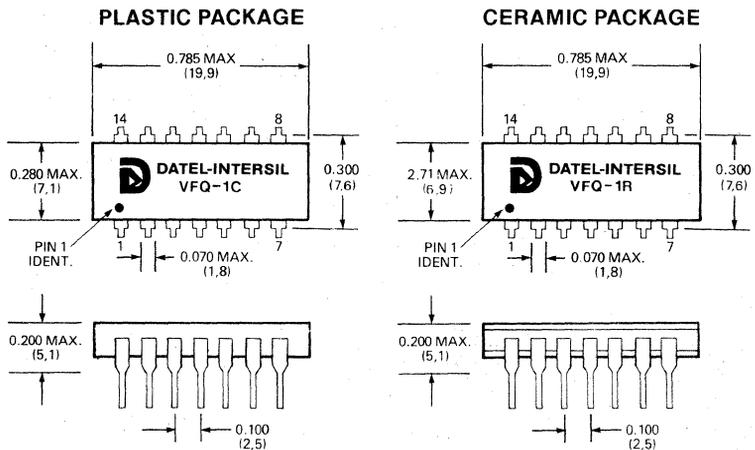
Low Cost Monolithic Voltage To Frequency Converters Models VFQ-1C, VFQ-1R
