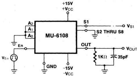
Figure 3.  $t_{on}$  and  $t_{off}$  Switching Test
