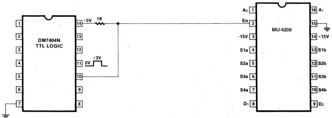
Figure 4. Enable Input Strobing from TTL Logic
