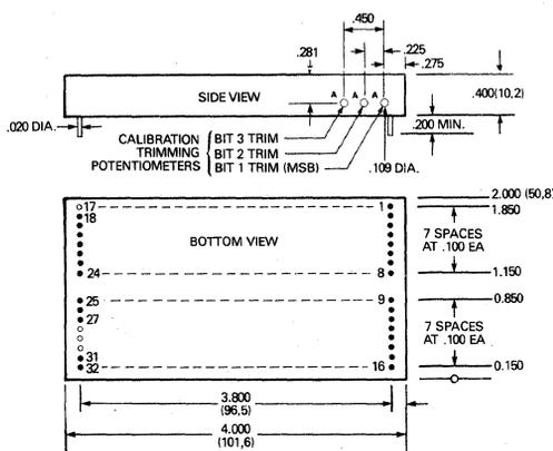
NOTE: OPEN DOTS INDICATE OMITTED PINS.
