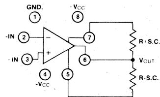
In general, for a given VOUT, Isc limit, and case temperature TC, Rs.c. can be calculated from the equation below (VOUT in Volts):
