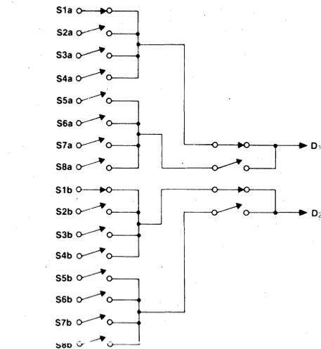
TO DECODE LOGIC CONTROLLING BOTH TIERS OF MUXING
