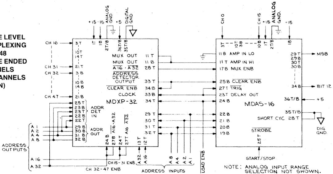
**SINGLE LEVEL MULTIPLEXING UP TO 24 DIFFERENTIAL CHANNELS (24 CHANNELS SHOWN)**
