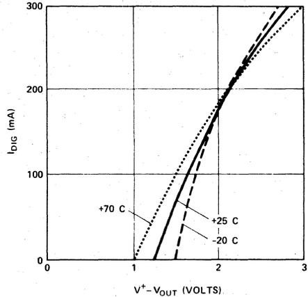
**FIGURE 4. CD-7216A & C Typical I<sub>DIG</sub> vs. V<sup>+</sup> - V<sub>OUT</sub>, 4.5V ≤ V<sup>+</sup> - V<sup>-</sup> ≤ 6.0V**
