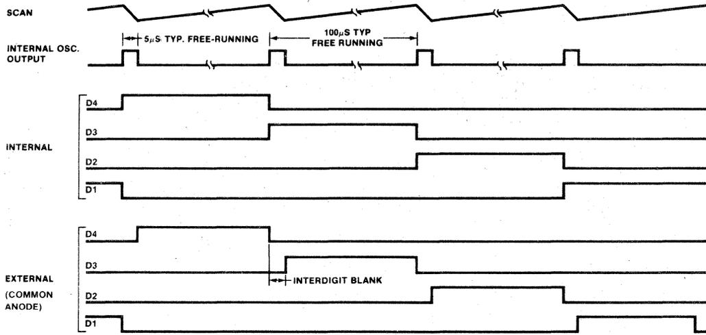
Figure 3: Multiplex Timing
