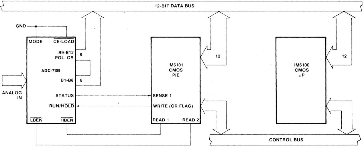
Figure 17: ADC-7109-IM6100 Interface Using IM6101 PE
