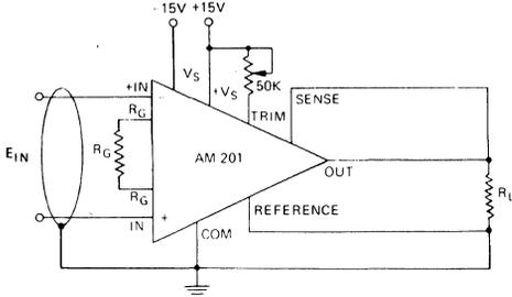
**INPUT OFFSET TRIMMING:** Short input terminals together and connect to ground or to common mode voltage at which input will be used. Adjust 50K trimming pot for zero output voltage. For critical applications  $R_G$  should be a Vishay type S102 and the trimming pot should be a Vishay type 1203. See technical notes.
