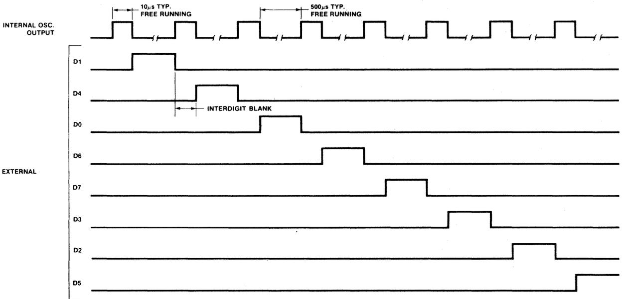
Figure 1: Multiplex Timing
