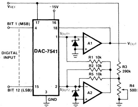
Note: R1 and R2 should be 0.01%, low-TCR resistors.
