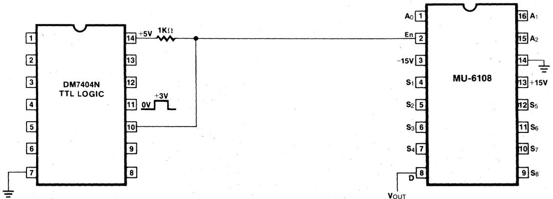
Figure 4. Enable Input Strobing from TTL Logic
