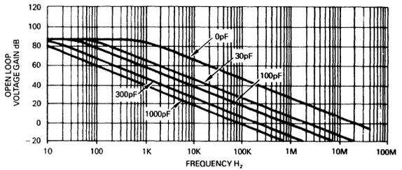
NOTE: EXTERNAL COMPENSATION IS REQUIRED FOR CLOSED LOOP GAIN < 3.
