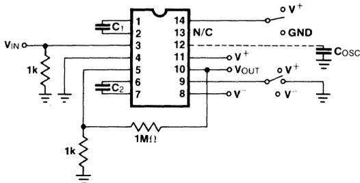
Test Circuit 1: Voltage Gain = 1000
