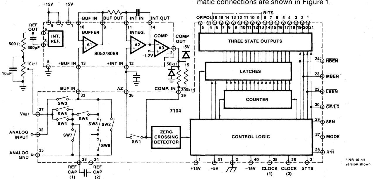
Figure 1: 8068A/7104 16/14 Bit A/D Converter Functional Block Diagram
