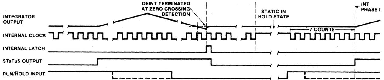
Figure 8: Run/Hold Operation
