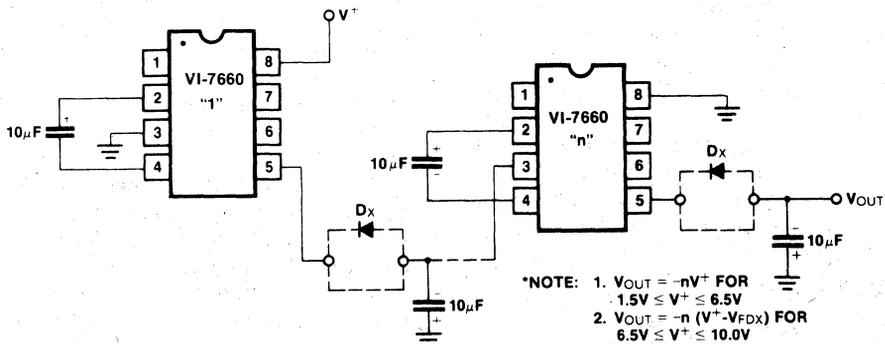
Figure 6: Cascading Devices for Increased Output Voltage
