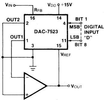
$$V_{OUT} = -V_{IN}/D$$
