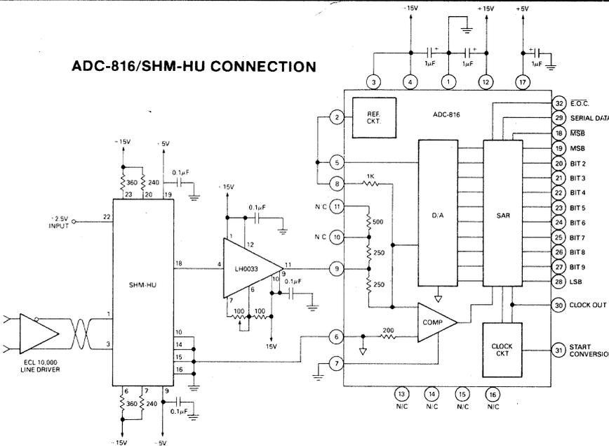
When the ADC-816 or ADC-826 is configured as shown here with Datal-Intersil's SHM-HU hybrid sample-and-hold, a  $\pm 2.5V$  input step can be acquired to 0.1% accuracy in 30 nsec and held to within  $40 \mu V$  while the A/D conversion takes place. Use of the SHM-HU reduces the time over which the input signal is averaged to a few nanoseconds (an A/D converter without a sample-and-hold averages the analog input signal over the total conversion time of the A/D).
