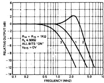
CURVE 1:  $C_C = 15\text{pF}$ ,  $V_{IN} = 2.0\text{V}_{pp}$  CENTERED AT  $+1.0\text{V}$ .
