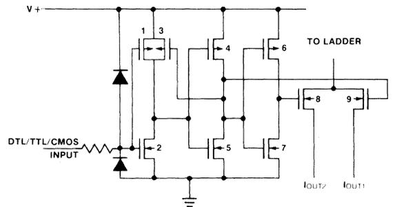
Figure 8. CMOS Switch
