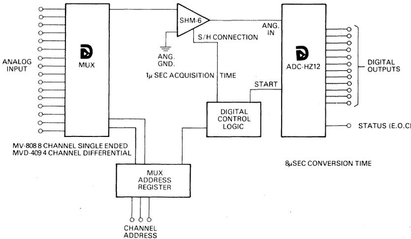
A high speed data acquisition system employing the SHM-6. This system is capable of a 110 KHz throughput rate with 12 bit resolution. In this system the SHM-6 is used with Datel-Intersil's ADC-HZ12, a high-speed hybrid 12 bit A/D converter, and Datel's MV-808, a low cost monolithic analog multiplexer. Use of a low on-resistance MUX is recommended, so that the time constant formed by MUX on-resistance and bus capacitance does not limit the acquisition performance of the SHM-6.
