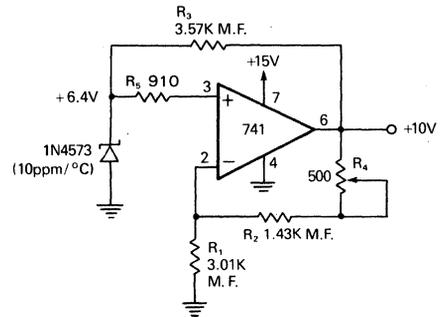
Adjust  $R_4$  for +10.000V output. For best stability  $R_1$  &  $R_2$  should track each other closely with temperature.  $R_4$  should be a low tempco trimming pot or else a selected metal film trim resistor.
