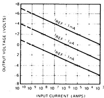
TRANSFER FUNCTION FOR VOLTAGE INPUTS
