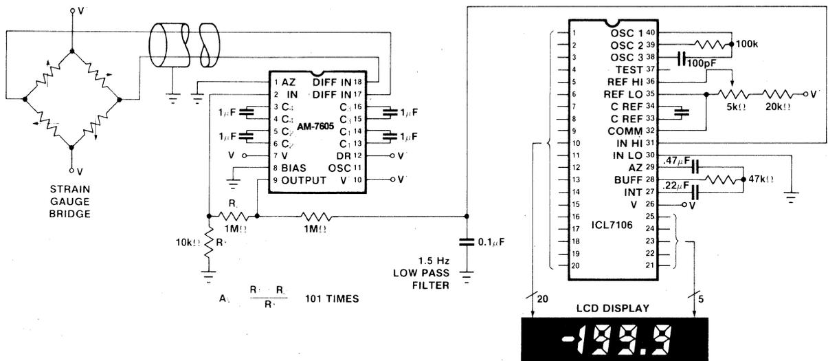
Figure 6: 3-1/2 Digit Digital Readout Torque Wrench
