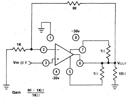
Figure 6: Large Signal Power Band Width
