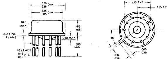
NOTE: Pin 5 connected to case.
