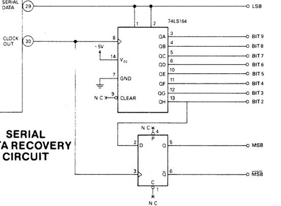
The Unconditional Start Circuit, shown for the ADC-816/826 insures the initiation of a conversion cycle upon the application of one start pulse of 40 nsec minimum pulse width regardless of converter status. The serial data output of the ADC-816/826 is converted into parallel form, with the addition of an MSB output, by the Serial Data Recovery circuit. Users should refer to technical note No. 2 on the loading of the ADC-816/826 digital outputs when using these circuits.
