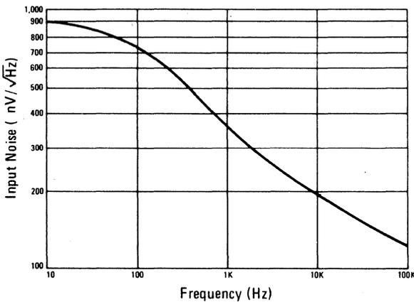
EQUIVALENT INPUT NOISE VS. CLOSED LOOP BANDWIDTH
