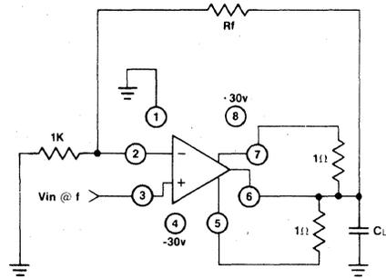
Figure 7: Small Signal Frequency Response
