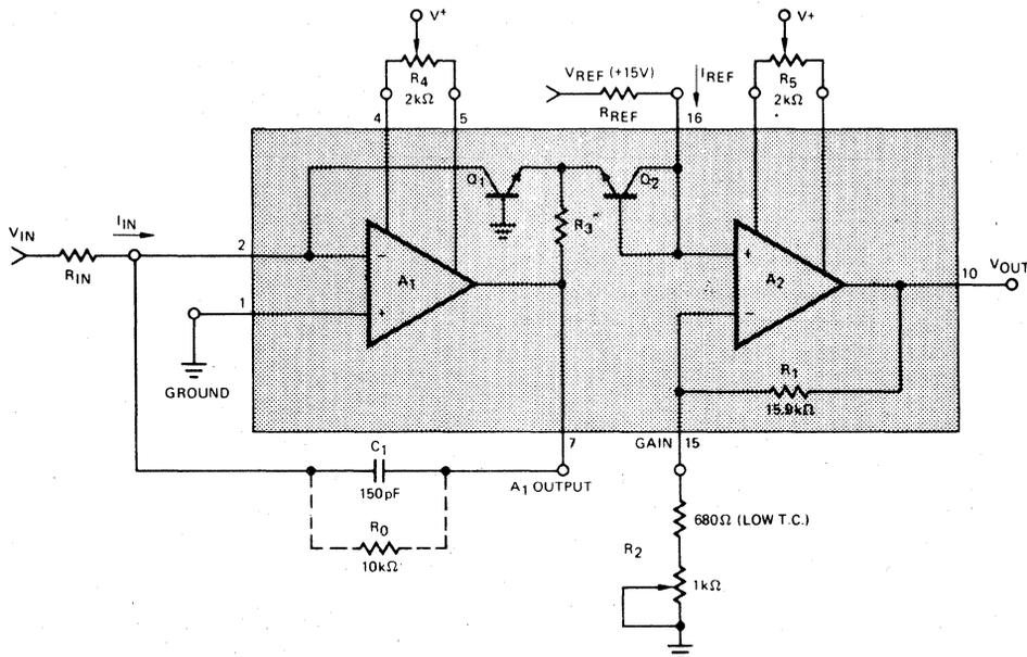
FIGURE 1. 8048 OFFSET AND SCALE FACTOR ADJUSTMENT
