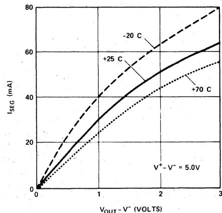
**FIGURE 5. CD-7216A & C Typical I<sub>SEG</sub> vs. V<sub>OUT</sub> - V<sup>-</sup>**
