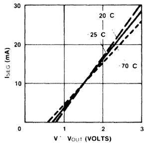
Figure 9: 7226B Typical  $I_{seg}$  Vs.  $V^+ - V_{out}$
