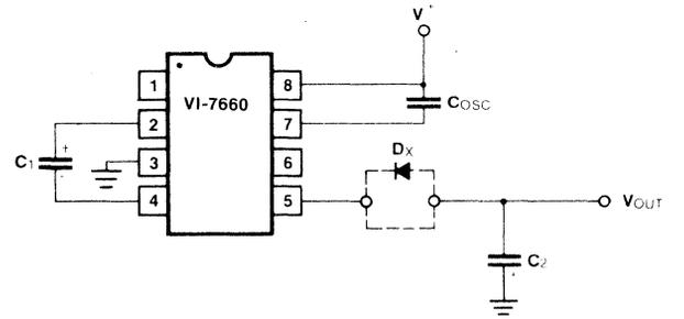
Figure 8: Lowering Oscillator Frequency
