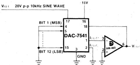
Figure 5. Feedthrough Error
