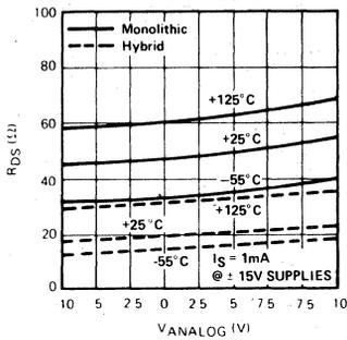
$R_{DS(ON)}$  vs POWER SUPPLY VOLTAGE
