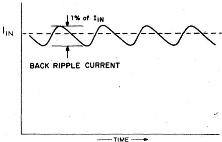
Figure 1. Back Ripple Current of a DC-DC Converter.
