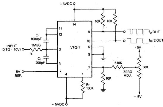
NOTE: FOR 100kHz FULL SCALE,  $C_1 = 100\text{pF}$  AND  $C_2 = 20\text{pF}$
