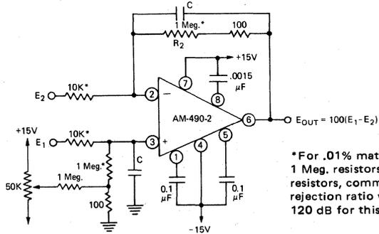
\*For .01% match between 1 Meg. resistors and 10K resistors, common mode rejection ratio will be approx. 120 dB for this circuit.
