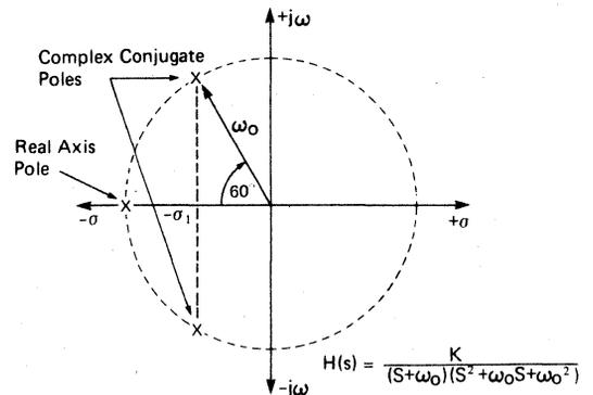
Figure 7. S-Plane Diagram of 3-Pole Butterworth Lowpass Filter
