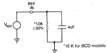
**Figure 3. EQUIVALENT INPUT IMPEDANCE OF DAC-HA REFERENCE INPUT**
