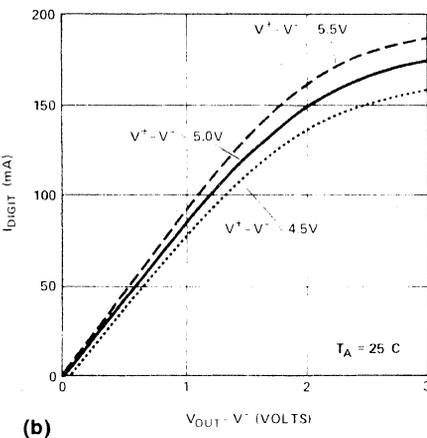
FIGURE 6. CD-7216B & D Typical  $I_{DIGIT}$  vs.  $V_{OUT} - V^-$
