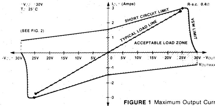
FIGURE 1 Maximum Output Current for Given Rs.c.
