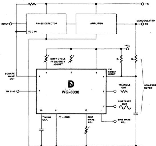
THE WG-8038 PRODUCES A VARIETY OF WAVEFORM OR PULSE OUTPUTS WITH HIGH ACCURACY, USING A MINIMUM OF EXTERNAL COMPONENTS.
