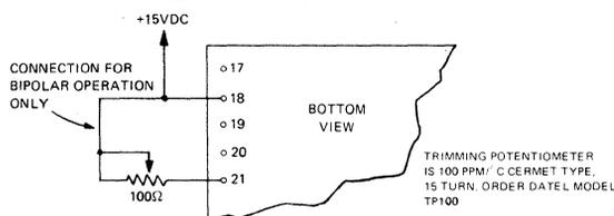
1. UNIPOLAR - No adjustments are necessary and 100Ω trimming pot is not used. Full scale and zero are internally set to better than 1/2 LSB. Pin 21 is left open.
