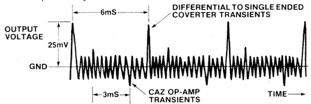
**Figure 9:** Output waveform from Test Circuit 1.
