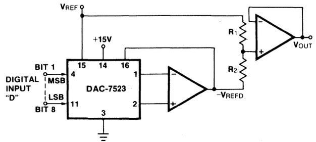
$$V_{OUT} = V_{REF} \left[ \left( \frac{R_2}{R_1 + R_2} \right) - \left( \frac{R_1 D}{R_1 + R_2} \right) \right]$$
