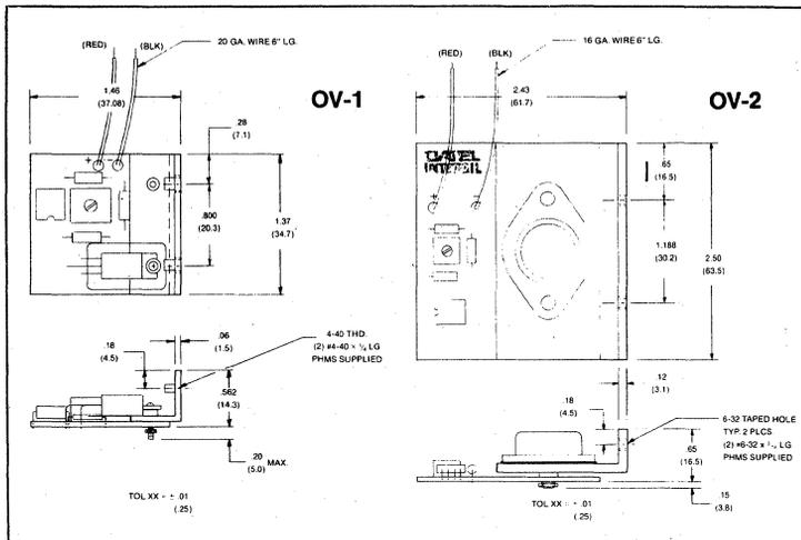
Mounting holes are provided in the PC series open frames for the OV modules
