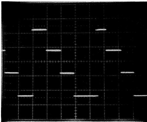
**Fig. 1** The output of a non-linearized 8 bit A/D converter is shown above. The display shows the 4 least significant bits at the major carry transition, demonstrating differential nonlinearity. This is a property of all non-linearized A/D converters. (The unit used for this example is a typical non-linearized A/D with  $\pm 1/2$  LSB of integral linearity and  $\pm 1/2$  LSB of differential nonlinearity).
