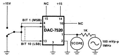
Figure 4. Output Capacitance
