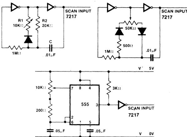
Figure 6: Brightness Circuits
