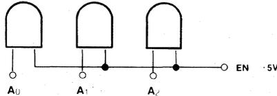
3 LINE BINARY STROBE INPUTS (0 0 0) AND EN = 5V
