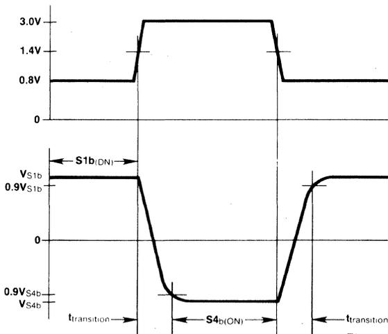
Figure 1. t<sub>transition</sub> Switching Test
