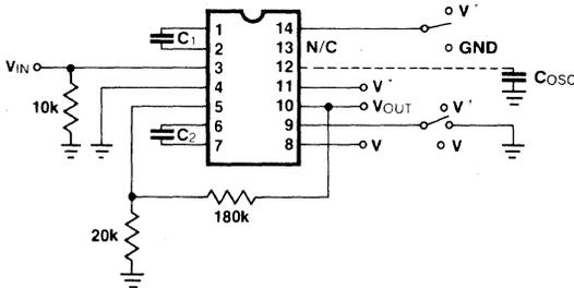
Test Circuit 3: Voltage Gain = 10
