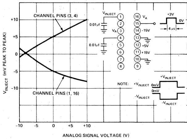
FIGURE 4. Charge Injection vs. Analog Signal.
