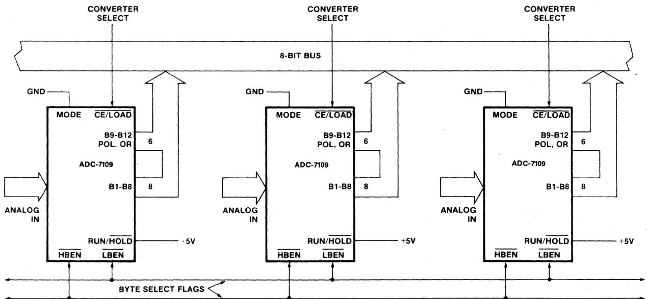
Figure 13: Three-stating Several 7109's to a Small Bus
