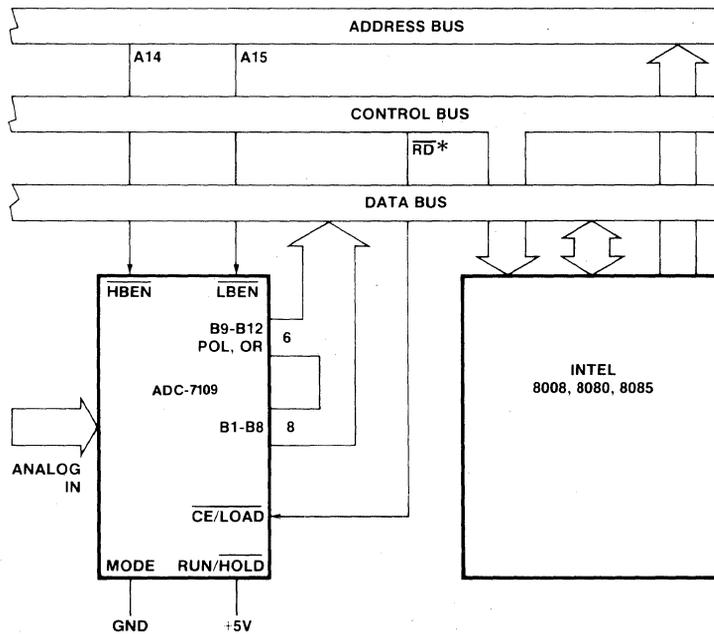
Figure 18: Direct ADC-7109-INTEL 8080/8085 Interface
