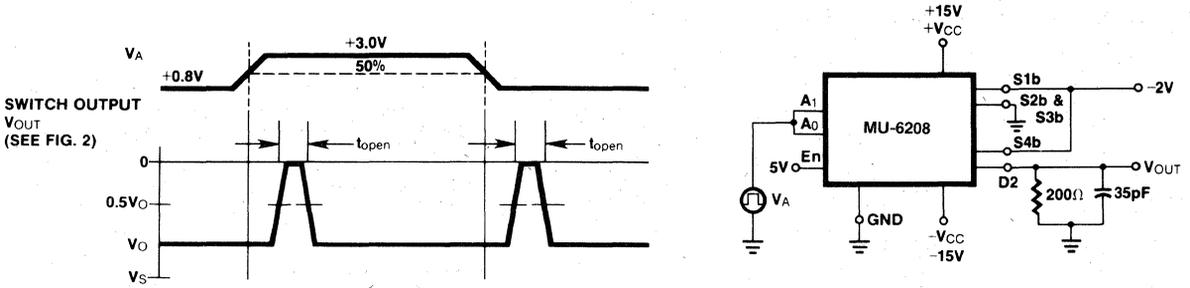
Figure 2.  $t_{open}$  'Break-Before-Make' Switching Test
