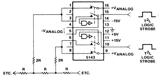
EXAMPLE: If  $-VANALOG = -10VDC$  and  $+VANALOG = +10VDC$  then Ladder Legs are switched between  $\pm 10VDC$ , depending upon state of Logic Strobe.
