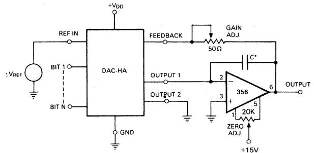
\*Use 3 to 30pF trim capacitor and adjust for optimum step response.
