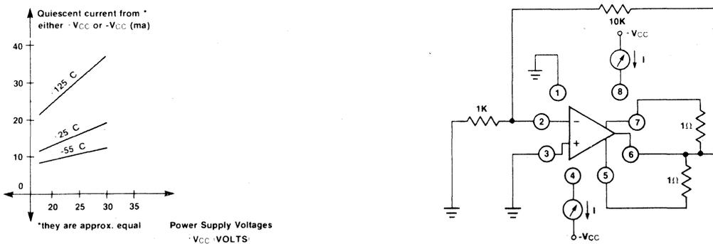
Figure 5: Quiescent Current vs Power Supply Voltage
