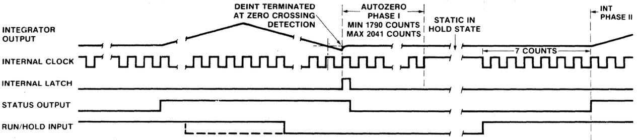
Figure 5: Run/Hold Operation
