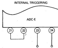
TO DECREASE TRIGGERING RATE CONNECT CAPACITOR ACROSS PINS 23 AND 24
