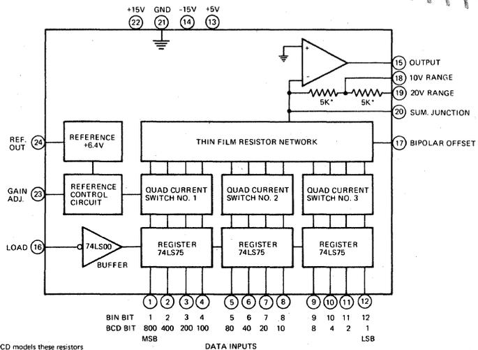
\*For BCD models these resistors are 4K ohms.
