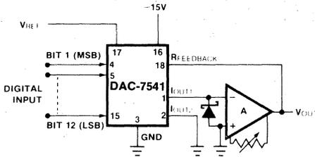
Figure 9. Unipolar Binary Operation (2-Quadrant Multiplication)
