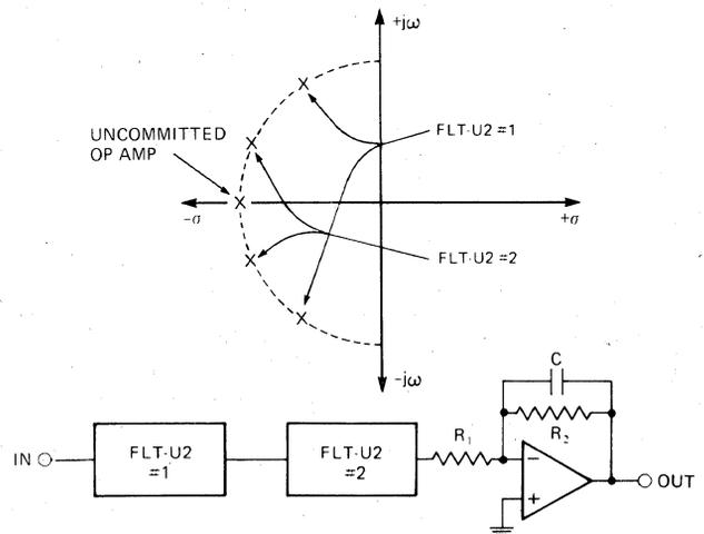
Figure 11. Realization of a Complex Multipole Filter
