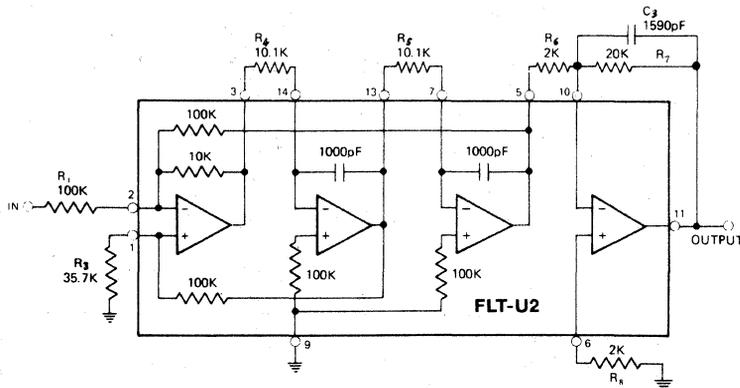
DATEL-INTERSil'S FLT-U2 ALLOWS A VARIETY OF FILTER FUNCTIONS WITH A MINIMUM OF EXTERNAL COMPONENTS; FOR EXAMPLE, THIS THREE POLE BUTTERWORTH LOW PASS FILTER.
