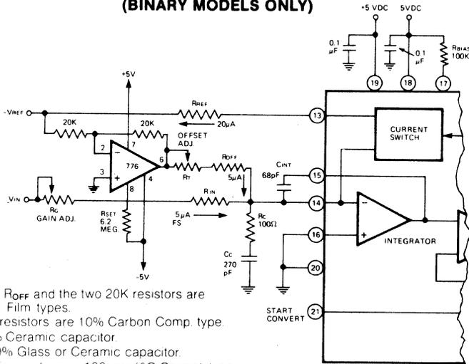
$R_{IN}$ ,  $R_{REF}$ ,  $R_{OFF}$  and the two 20K resistors are 1% Metal Film types.
