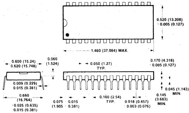
28 Pin Plastic Dual-In-Line Package
