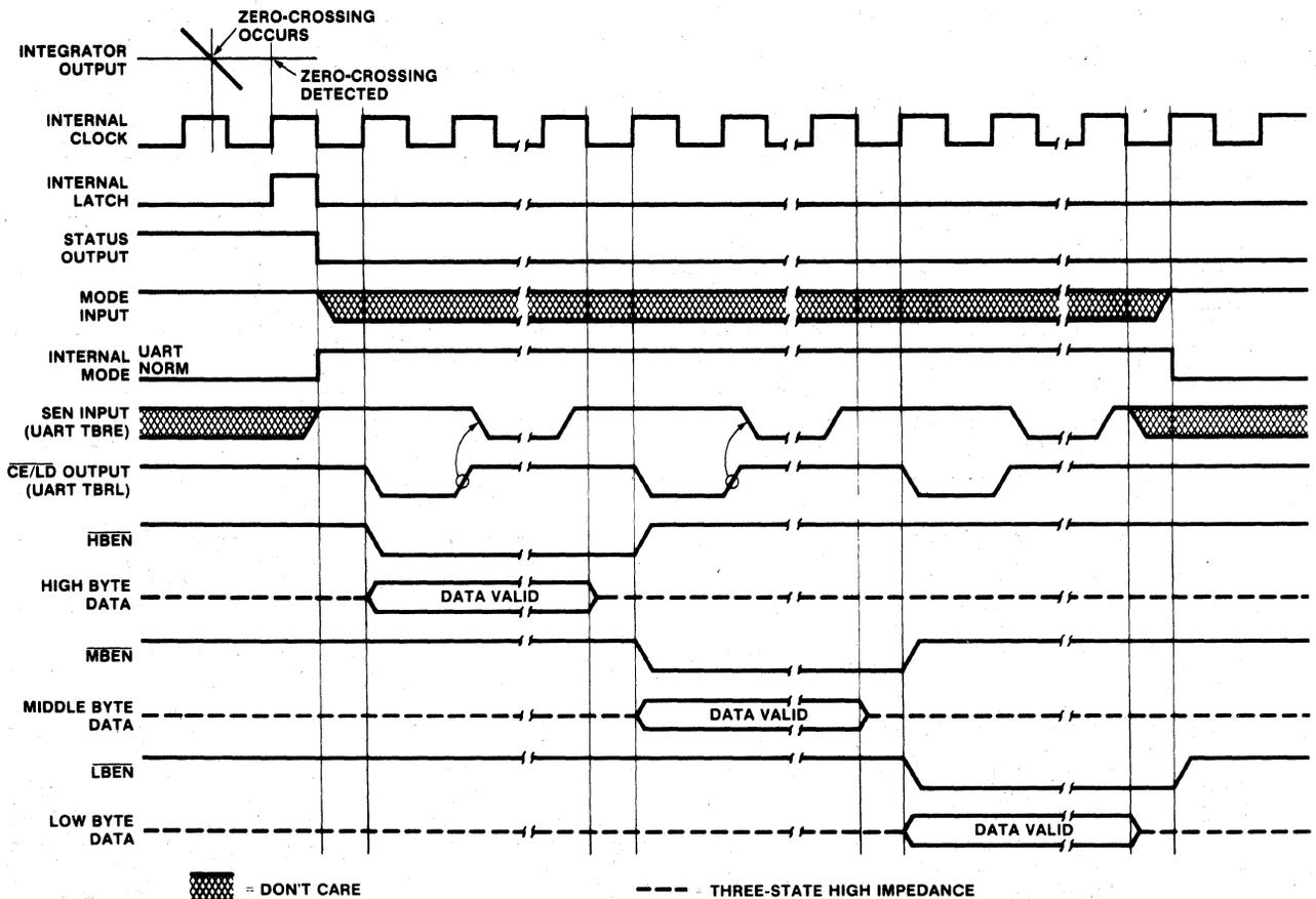
Figure 10: Handshake - Typical UART Interface Timing
