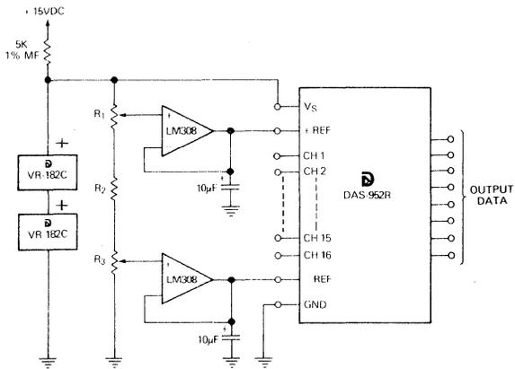
NOTE: VALUES OF  $R_1$ ,  $R_2$  and  $R_3$  ARE SELECTED TO YIELD THE DESIRED FULL SCALE CONVERSION RANGE. SEE TECHNICAL NOTE 1.
