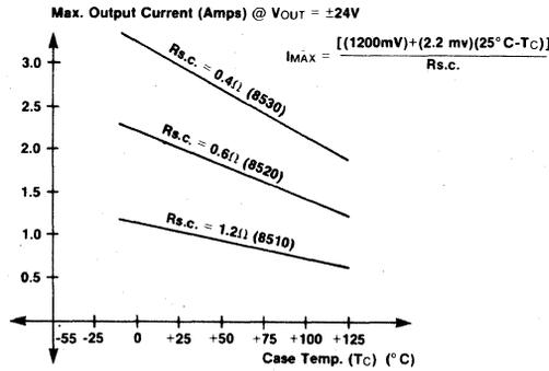
Figure 8: Maximum Output Current vs. Case Temperature
