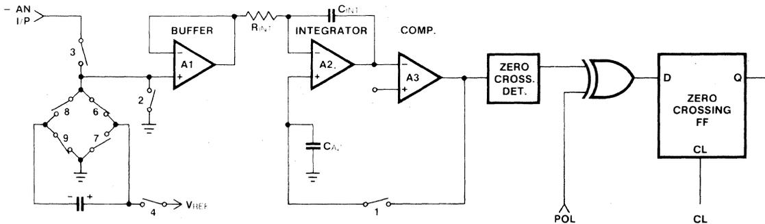
Figure 4D: Phase III - Deintegrate
