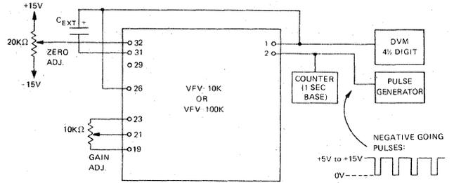
Trimming potentiometers are 100ppm/°C, 15 turn type, available from Datel-Intersil
