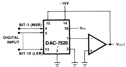
Figure 12. Analog/Digital Divider
