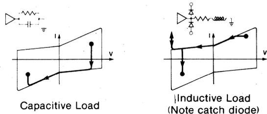
Thus the limiting circuitry protects the load and avoids needless damage to the driver during abnormal conditions. For any 24Vdc-28Vdc motor/actuator, the Rs.c. resistors must be calculated to get proper power delivered to the motor (up to a maximum of 2.7 amps) and ±VCC set at ±30V. For lower supply and/or output voltages, the maximum output current will follow graphs of Figures 1 and 10.
