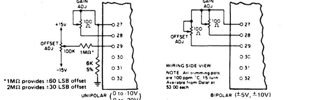
**Adjustment Procedure - Unipolar Input**
