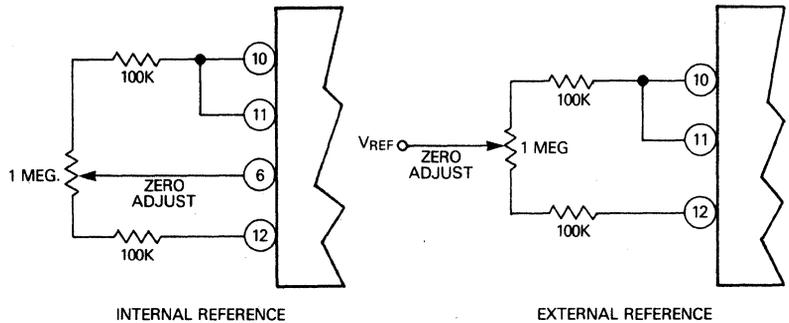
FOR UNIPOLAR OPERATION WHERE  $R_4$  APPROACHES  $\infty$  AND A ZERO ADJUSTMENT IS REQUIRED, THIS CIRCUIT MAY BE USED TO REPLACE  $R_4$
