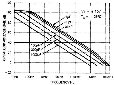
NOTE: EXTERNAL COMPENSATION COMPONENTS ARE NOT REQUIRED FOR STABILITY, BUT MAY BE ADDED TO REDUCE BANDWIDTH IF DESIRED IF EXTERNAL COMPENSATION IS USED, ALSO CONNECT 100pF CAPACITOR FROM OUTPUT TO GROUND.
