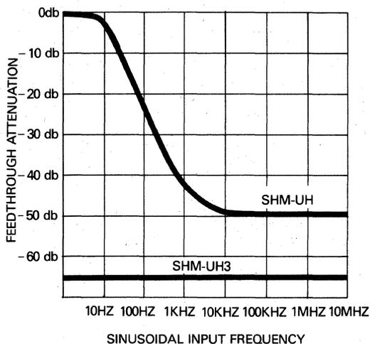
HOLD-MODE FEEDTHROUGH IS A PHENOMENA THAT OCCURS AFTER THE SWITCH HAS BEEN OPENED AND THE SIGNAL IS BEING HELD. A SMALL PART OF THE SIGNAL ON THE INPUT WILL BE COUPLED TO THE OUTPUT.
