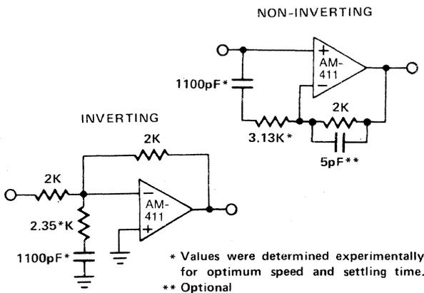
EXTERNAL OFFSET ADJUST AND BANDWIDTH COMPENSATION FOR AM-410 AND AM-411
