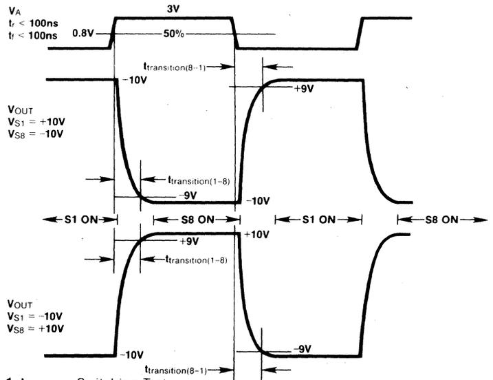
Figure 1. t<sub>transition</sub> Switching Test
