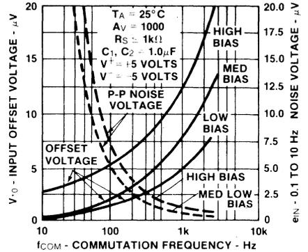
**INPUT OFFSET VOLTAGE AND PK-TO-PK NOISE VOLTAGE AS A FUNCTION OF COMMUTATION FREQUENCY (C1, C2 = 0.1 μF)**
