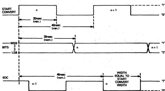
**ADC-UH8B TIMING DIAGRAM**
