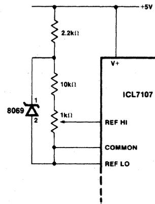
(c) Double regulated 100mV reference for ICL7107 one-chip DPM circuit.
