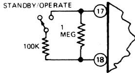
This reduces power consumption to about 200uA during Standby
