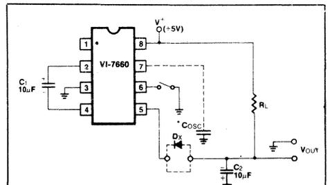
NOTES: 1. For large value of  $C_{OSC}$  ( $> 1000pF$ ) the values of  $C_1$  and  $C_2$  should be increased to  $100\mu F$ .
