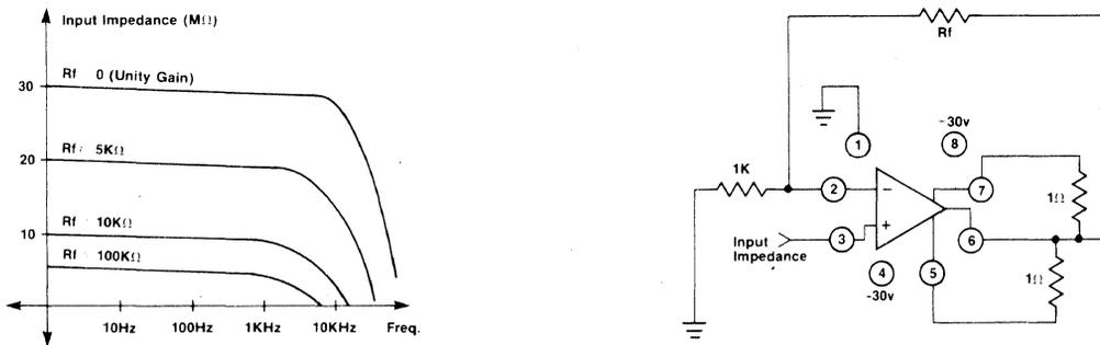
Figure 4: Input Impedance vs Gain vs Frequency
