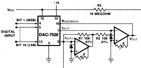
Figure 10. Bipolar Operation
