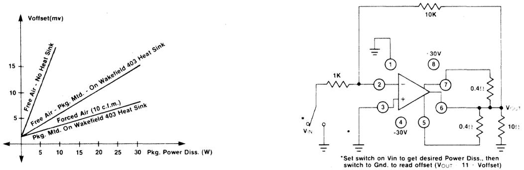
Figure 3: Input Offset Voltage vs Power Dissipation
