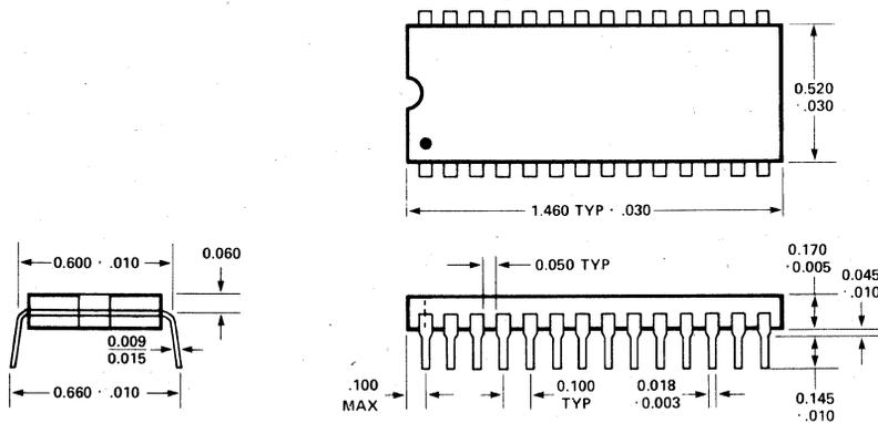
28 PIN CERDIP DUAL IN LINE PACKAGE
