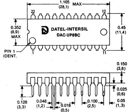
8-Bit Monolithic D/A Converter with Input Register Model DAC-UP8B
