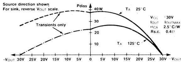
Figure 12: Power Dissipation under Short Circuit Conditions
