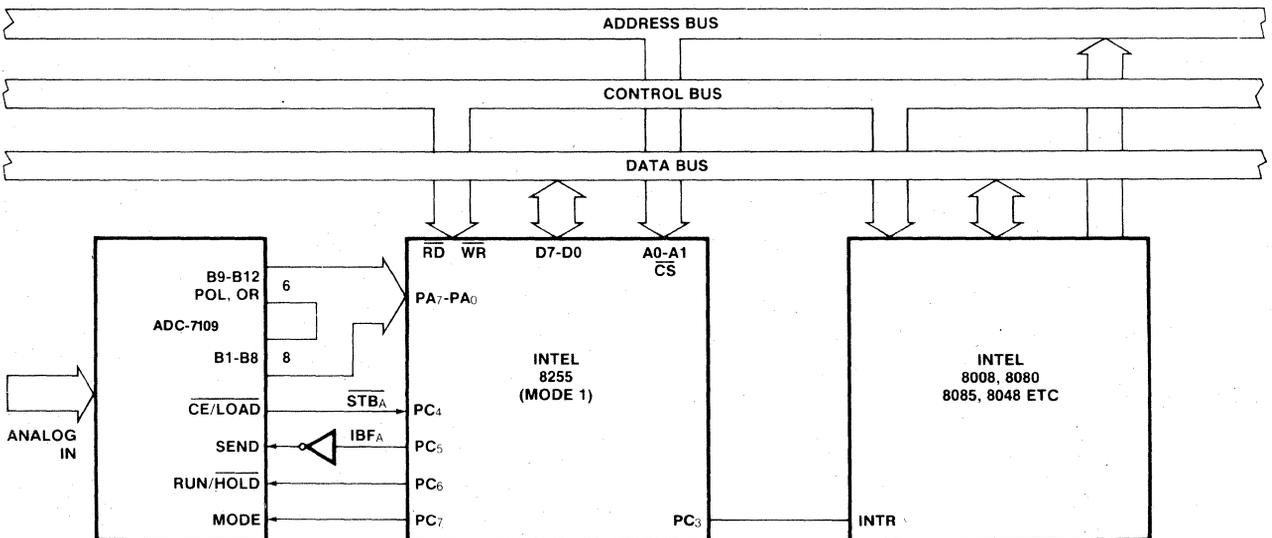
Figure 20: Handshake Interface — ADC-7109 to INTEL MCS-48, -80, 85
