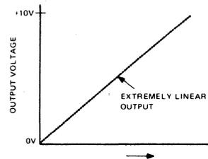
THIS CIRCUIT DEVELOPS A HIGHLY LINEAR (.01%) OUTPUT VOLTAGE RAMP FROM 0 TO +10V. THE RAMP CAN BE MADE AS SLOW AS DESIRED WITHOUT AFFECTING LINEARITY BY SETTING THE PULSE RATE OF THE TIMING CIRCUIT TO THE PROPER VALUE. THE OUTPUT RAMP IS GENERATED IN DISCRETE STEPS OF .024% FS (4096 STEPS FOR FS CHANGE).
