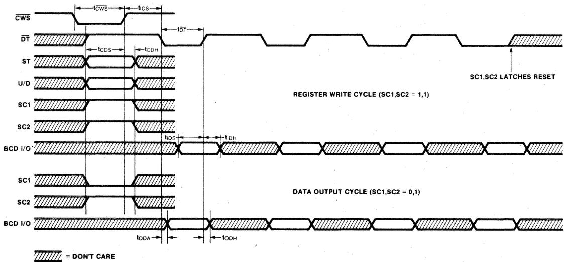
Figure 5: CD-7227 I/O Timing (See Table 2)
