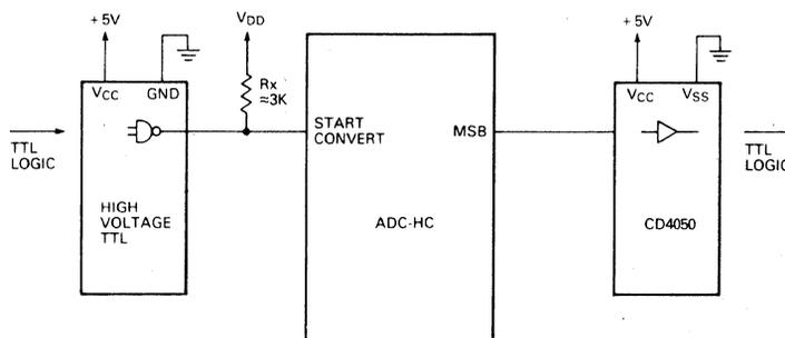
CMOS and TTL logic are not compatible due to different threshold levels. They can, however, be interfaced by simple techniques.
