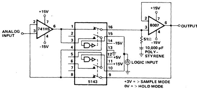
FIGURE 12. Improved Sample and Hold Using 5143
