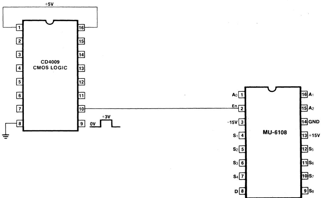
Figure 5. Enable Input Strobing from CMOS Logic
