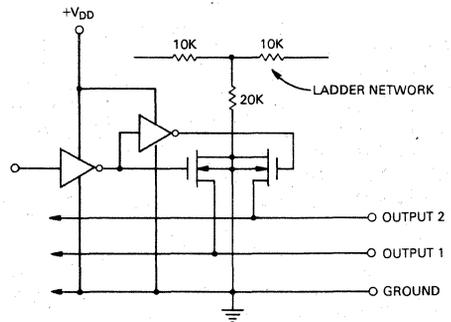
**Figure 2. SINGLE POLE DOUBLE THROW CMOS SWITCH**
