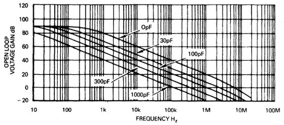
NOTE: EXTERNAL COMPENSATION COMPONENTS ARE NOT REQUIRED FOR STABILITY, BUT MAY BE ADDED TO REDUCE BANDWIDTH IF DESIRED.
