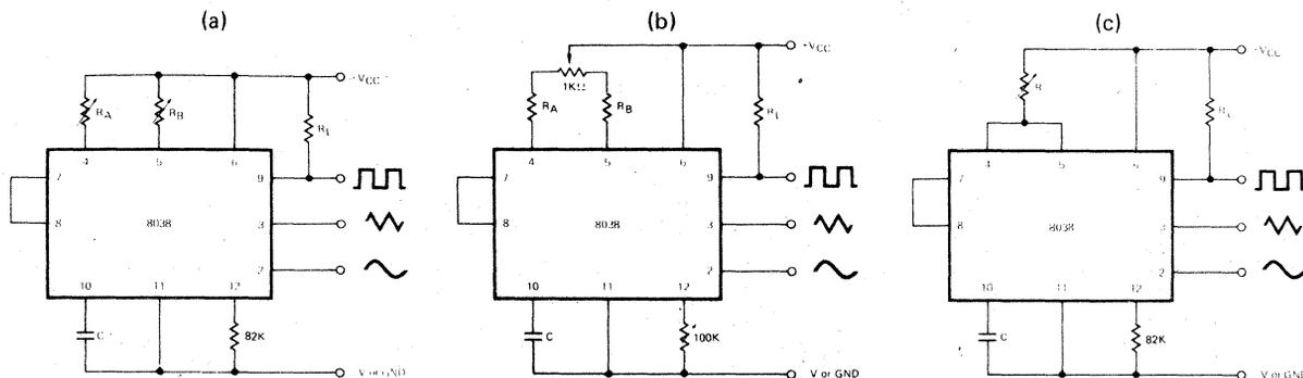
FIGURE 8. POSSIBLE CONNECTIONS FOR THE EXTERNAL TIMING RESISTORS.
