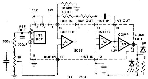
Figure 6: Adding Buffer Gain to 8068
