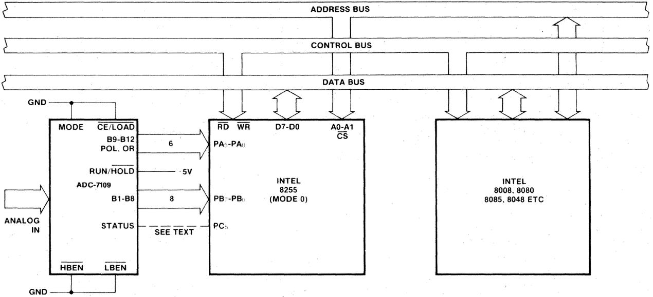
Figure 14: Full-time Parallel Interface to INTEL Microcomputer Systems
