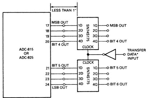
\*TRANSFER DATA INPUT MAY BE TIED TO EOC OUTPUT (PIN 2) OR EXTERNALLY DRIVEN. WHEN TRANSFER DATA IS EXTERNALLY CONTROLLED TIMING OF CONTROL PULSE SHOULD BE AS SHOWN
