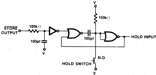
Figure 20: Circuit for Reducing Time Between Measurements
