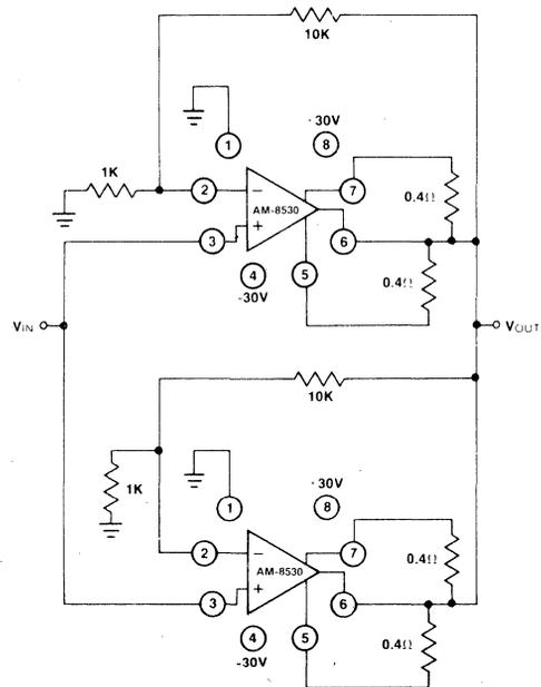
Figure 14: Paralleling Power Amps for Increased Current Capability
