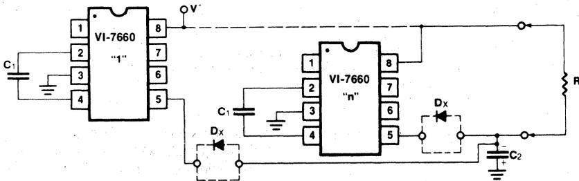
Figure 5: Paralleling Devices
