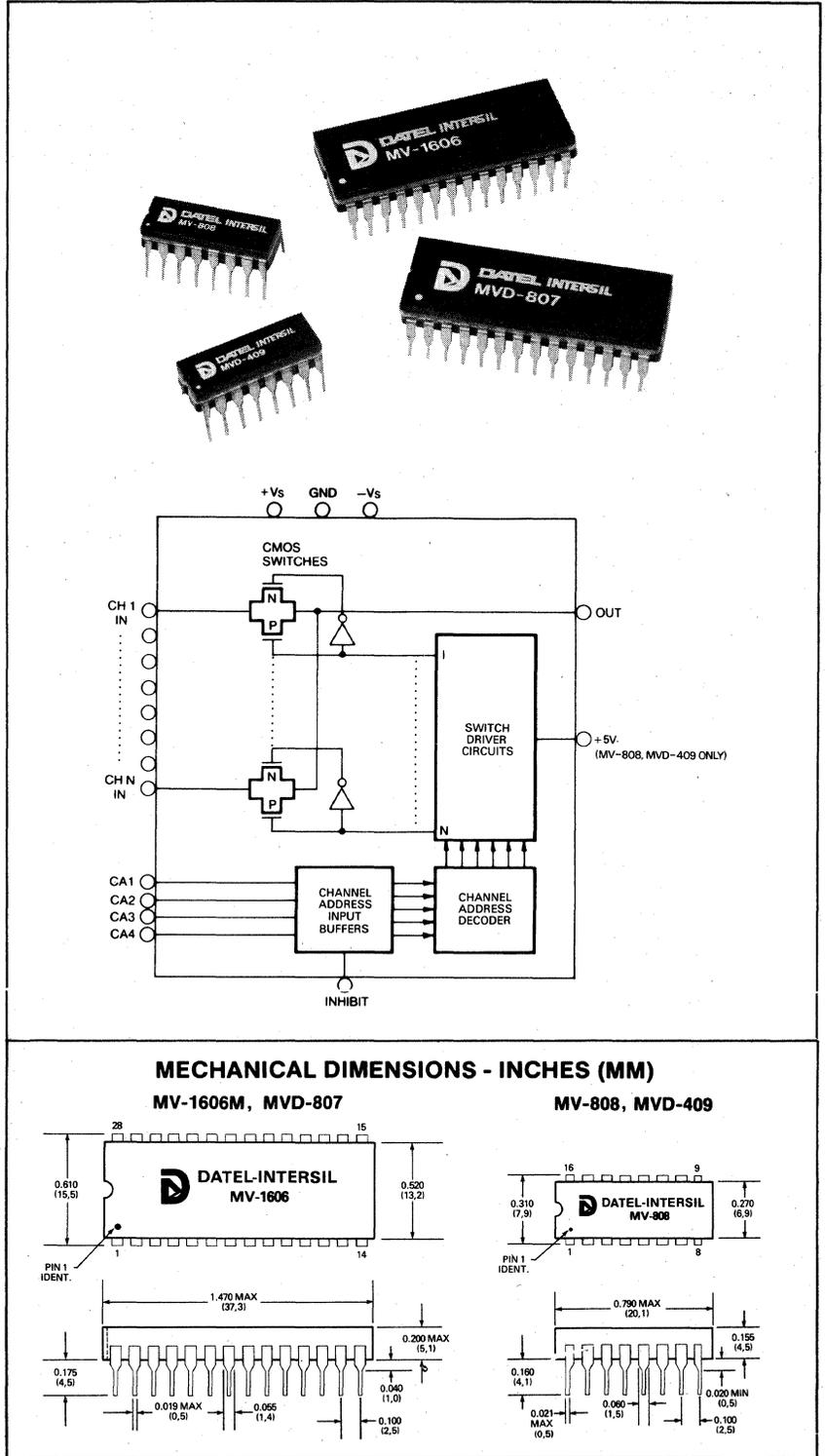
Low On Resistance CMOS Analog Multiplexers MV Series
