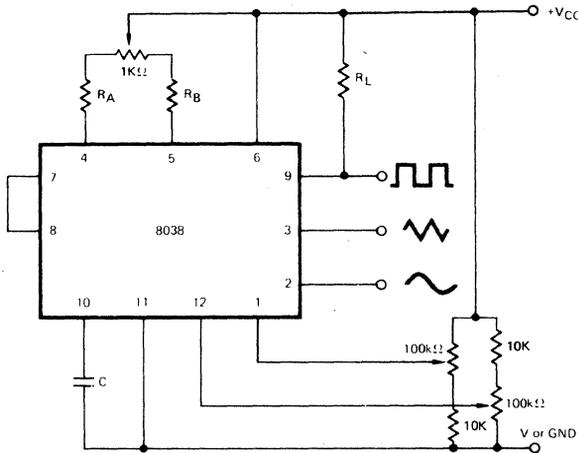
FIGURE 9. CONNECTION TO ACHIEVE MINIMUM SINE-WAVE DISTORTION.
