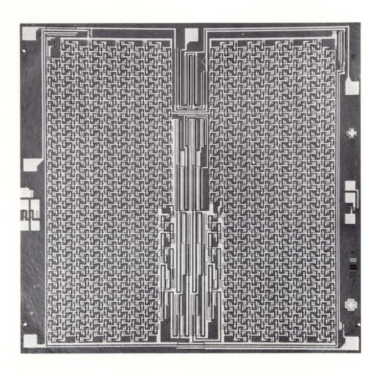
426-Bit Register with 2567 transistors on a 105 x 106 mil chip.
