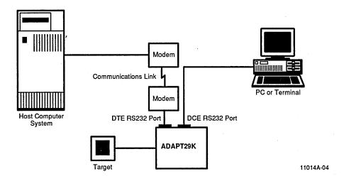
Figure 4. Connections to the ADAPT29K
