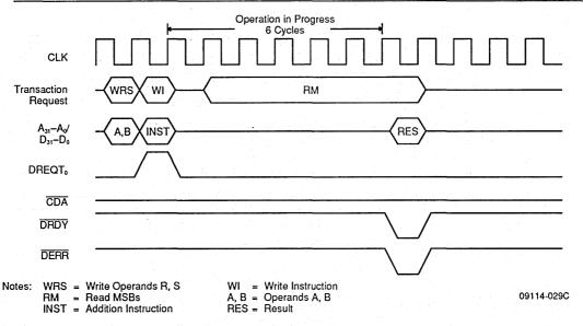
Figure D13. Typical Timing for Single-Precision Operation in Flow-Through Mode, with DRDY Advanced—Perform the Operation A PLUS B, Read the Result; Mode Register Field PLTC=6
