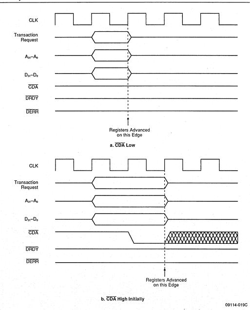
Figure D3. Timing for the Advance Temp. Registers Transaction Request
