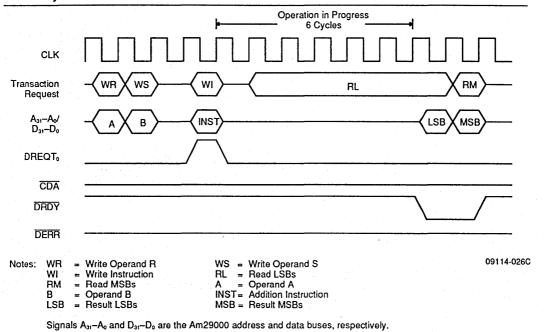
Figure D10. Typical Timing for the Double-Precision Operation in Flow-Through Mode—Perform the Operation A PLUS B, Read the Result; Mode Register Field PLTC = 6
