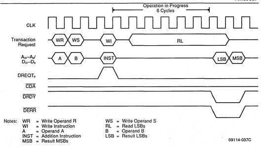
Figure D16. Typical Timing for Double-Precision Operation in Flow-Through Mode, with DRDY Advanced and Unmasked Exception Present—Perform the Operation A PLUS B, Read the Result;
