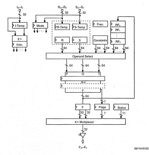
Figure 16. Programmer's Model for Pipeline Mode
