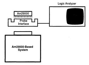
Figure 16. Connection of the Probe Interface
