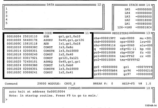
Figure 14. The Standard Assembly-Level Mode Screen
