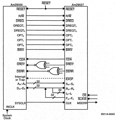
Figure 2. Am29000/Am29027 Hardware Interface
