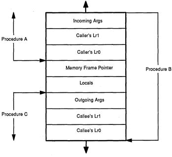
Figure 5. The Register Stack
