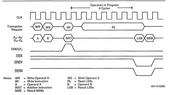
Figure D12. Typical Timing for Double-Precision Operation in Flow-Through Mode, with Unmasked Exception Present—Perform the Operation A PLUS B, Read the Result; Mode Register Field PLTC=6
