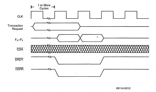
Figure D5. Timing for Read Result LSBs Transaction Request, Unmasked Exception Present
