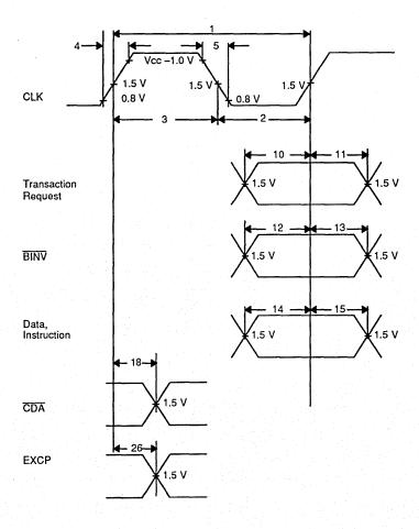
Input Signal Timing; CDA, EXCP Timing
