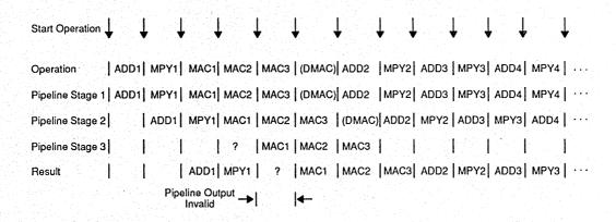
b. Pipeline invalidation timing for multiply-accumulate operations in pipeline mode.
