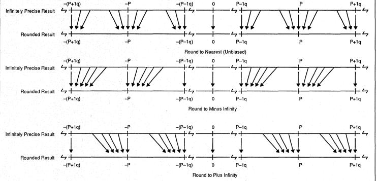
Figure B1. Graphical Interpretation of Round-to-Nearest (Unblased), Round-to-Minus-Infinity, and Round-to-Plus-Infinity Rounding Modes
