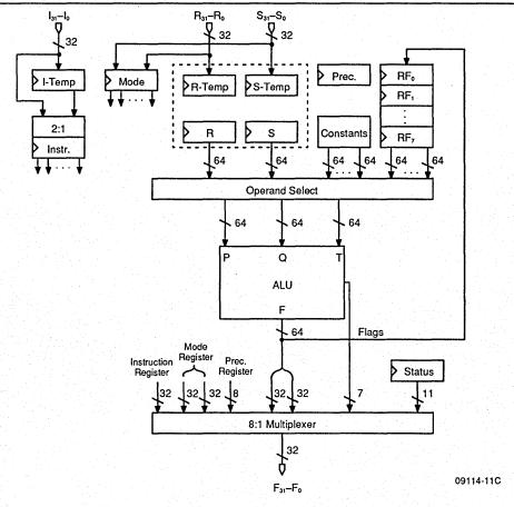
Figure 15. Programmer's Model for Flow-Through Mode
