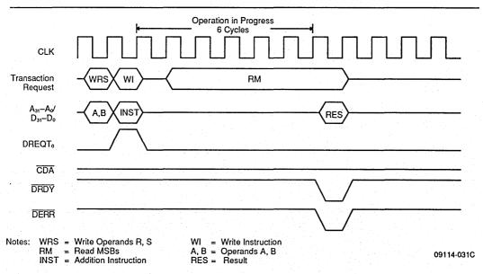
Figure D15. Typical Timing for Single-Precision Operation in Flow-Through Mode, with DRDY Advanced and Unmasked Exception Present—Perform the Operation A PLUS B, Read the Result;
