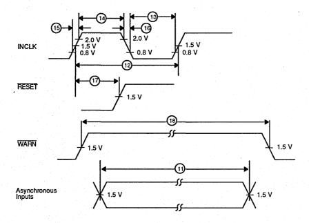
**INCLK** and Asynchronous Inputs
