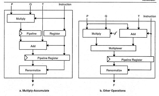
Figure 17. ALU Configuration for Pipeline Mode
