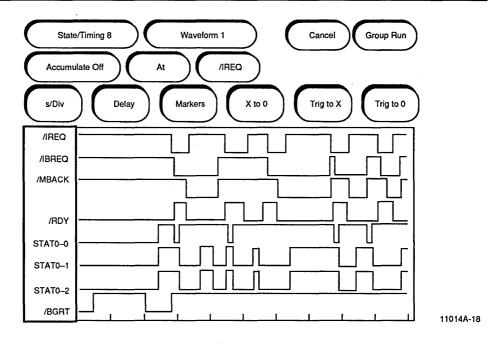
Figure 18. HP 16500 Signal and Timing Display
