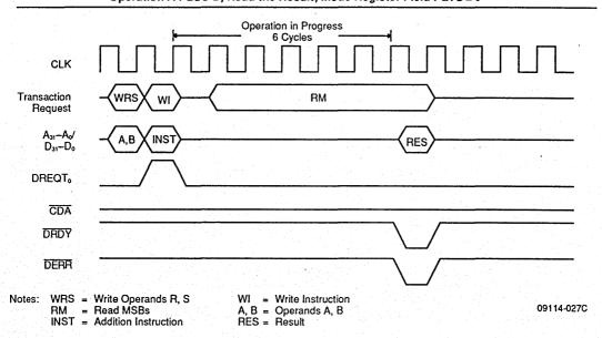
Figure D11. Typical Timing for Single-Precision Operation in Flow-Through Mode, with Unmasked Exception Present—Perform the Operation A PLUS B, Read the Result; Mode Register Field PLTC=6
