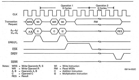
Figure D17. Typical Timing for Overlapped Single-Precision Operations in Flow-Through Mode; Perform the Compound Operation (A PLUS B)  $\times$  C by Performing Operations: (1) RF $_0$   $\leftarrow$  A PLUS B, (2) RF $_0$   $\times$  C Mode Register Field PLTC=6
