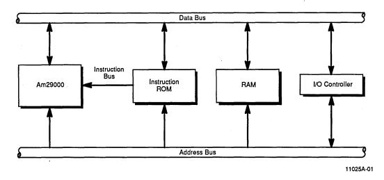
Figure 1. A Typical Am29000 System
