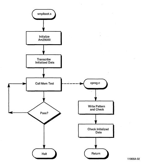
Figure 2. Flow Chart of the Example Application
