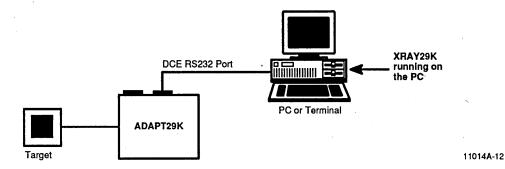
Figure 12. XRAY29K System Connections
