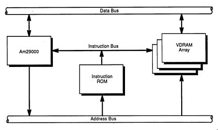
Figure 3. An Am29000 System with VDRAM
