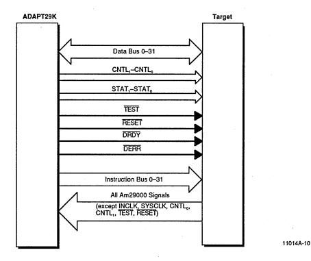
Figure 10. The ADAPT29K-to-Target Interface
