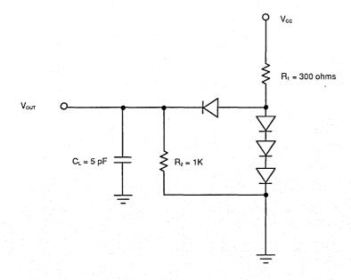
**Three-State Output Inactive Test**
