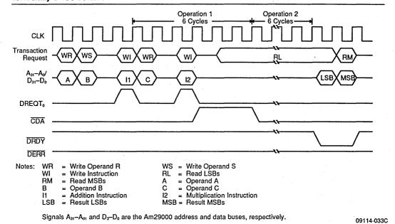
Figure D18. Typical Timing for Overlapped Double-Precision Operations in Flow-Through Mode;
