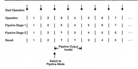
a. Pipeline invalidation timing for switch from flow-through to pipeline mode. Operations shown incur two pipe-line delays in pipeline mode [all base operations except  $F' = (P' \times Q') + T'$ ].
