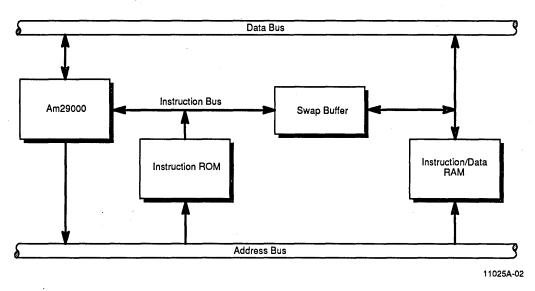
Figure 2. An Am29000 System with Swap Buffers
