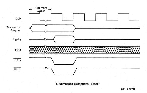
Figure D6. Timing for Read Result MSBs, Read Flags, and Read Status Transaction Requests
