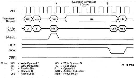
Figure D14. Typical Timing for Double-Precision Operation in Flow-Through Mode, with DRD Advanced—Perform the Operation A PLUS B, Read the Result; Mode Register Field PLTC=6
