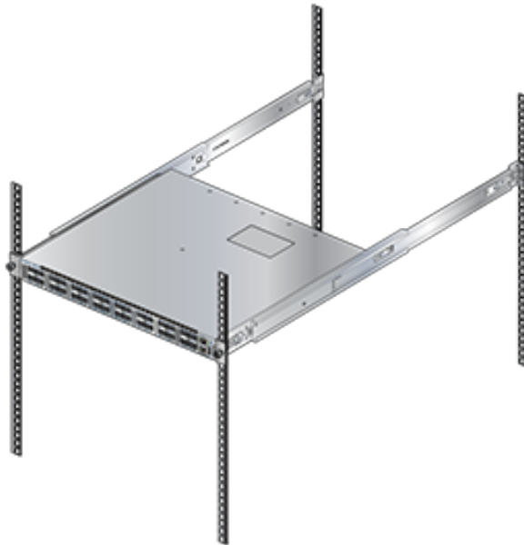
Figure 3-14: Attaching the Switch to the Rack Posts
