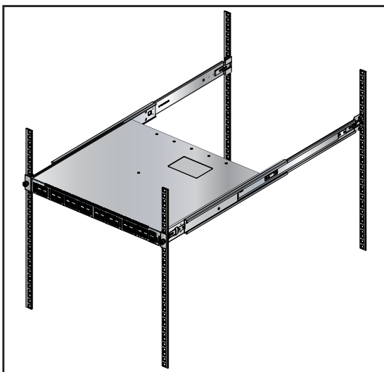
Figure 3-12: Attaching the Switch to the Rack Posts
