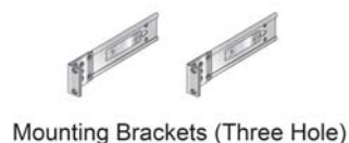
Figure B-2: Two-Post Rack Mount Parts
